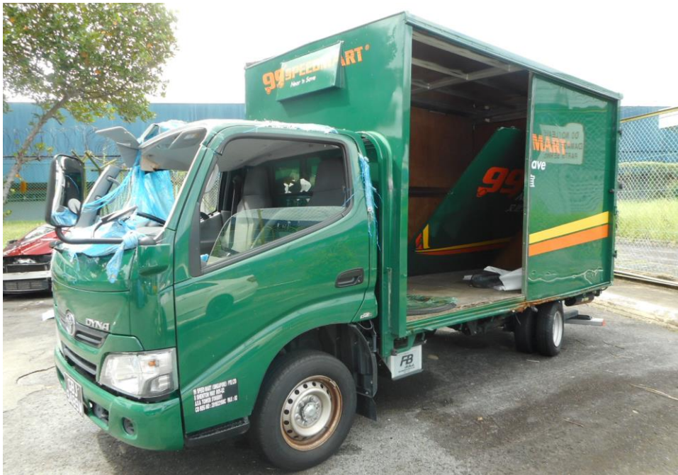
Photo 6 shows a general view of the left body of the Motor Lorry at the time of our inspection. The Motor Lorry was observed to have sustained damages to its rear cabin body panel as a result of the accident.
