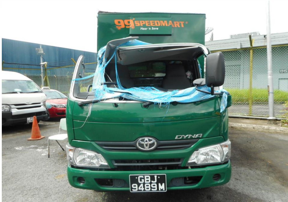
Photo 1 shows a general view of the front windscreen and front cabin body panel of the Motor Lorry at the time of our inspection. The Motor Lorry was observed sustained extensive damage as a result of the accident.
