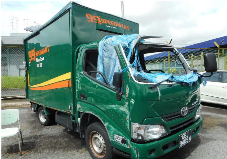
Photo 3 shows a general view of the right body of the Motor Lorry at the time of our inspection. The Motor Lorry was observed to have sustained damages to its doors and rear cabin body panel as a result of the accident.
