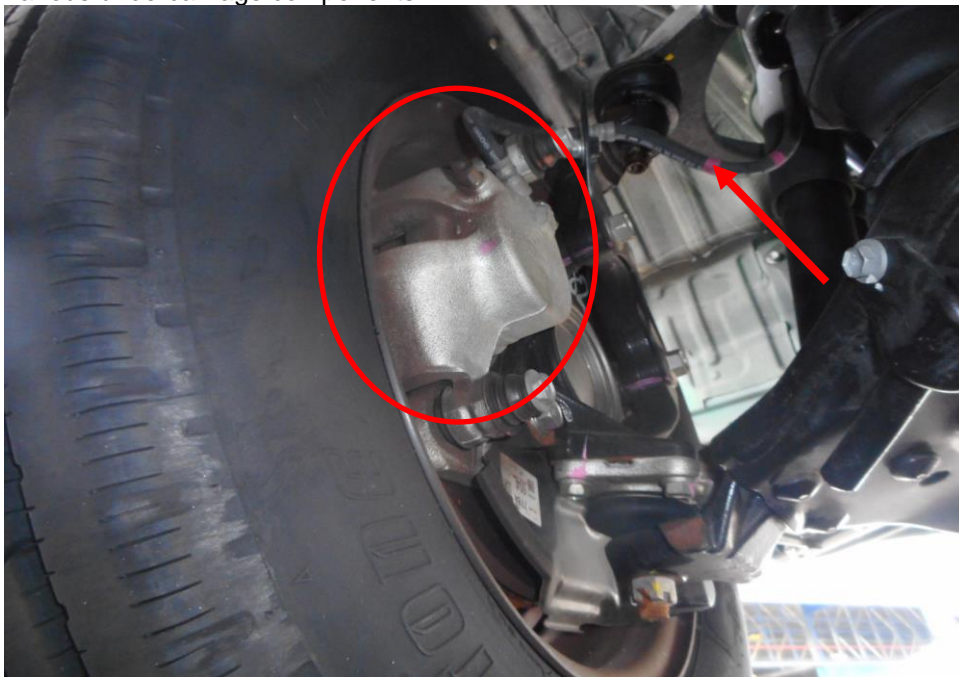
Photo 24 shows the brake hose/pipe (arrowed) at the front left wheel of the Motor Lorry. No leakage of brake fluid was observed. Visual examination of the various components of the braking system like the brake caliper (circled), brake booster, brake pedal etc had revealed all to be intact and without visible damage at the time of accident. There was also no sign of fluid stain(s) observed on the various undercarriage components.
