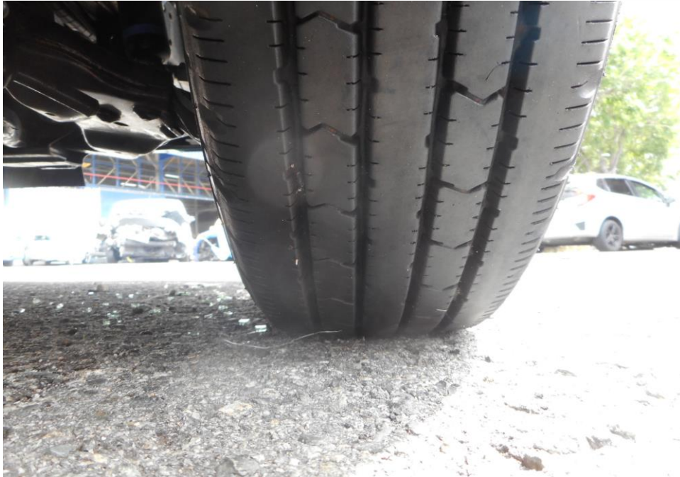
Photo 9 shows the condition of the front right tyre of the Motor Lorry, which was observed to be in serviceable condition with remaining tread depth of approximately 8.3mm. The tyre, which was wrapped around standard steel wheel rim, was also observed to be sufficiently inflated for vehicular operation.
