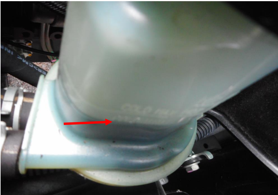
Photo 17 shows the power steering fluid dip stick of the Motor Lorry at the time of my inspection. The steering fluid oil was observed to be of sufficient level (arrowed) and without any visible contamination.
