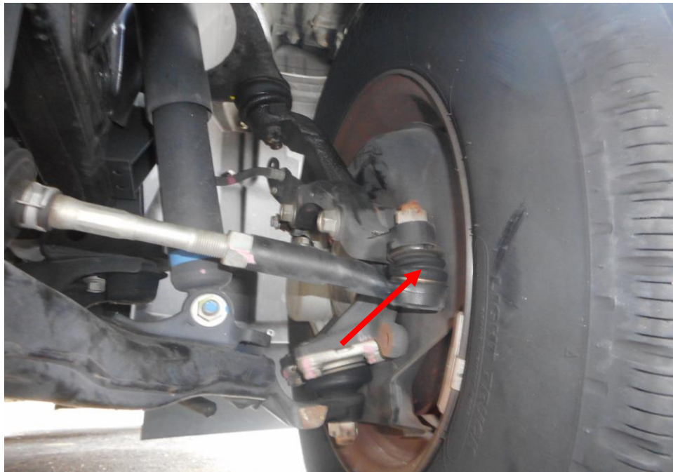
Photo 20 shows the various undercarriage components at the front left wheel of the Motor Lorry, in particular the steering tie rod end (arrowed). The various undercarriage components of the Motor Lorry were all found to be intact without any visible damage. There was also no sign of fluid stain(s) observed on the various undercarriage components.
