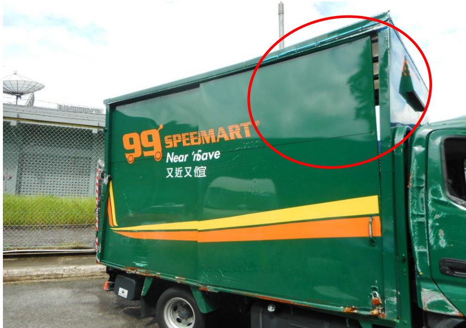
Photo 5 shows a close up view of the right body of the Motor Lorry at the time of our inspection. The Motor Lorry was observed to have sustained damages to its rear cabin body panel (circled) as a result of the accident.
