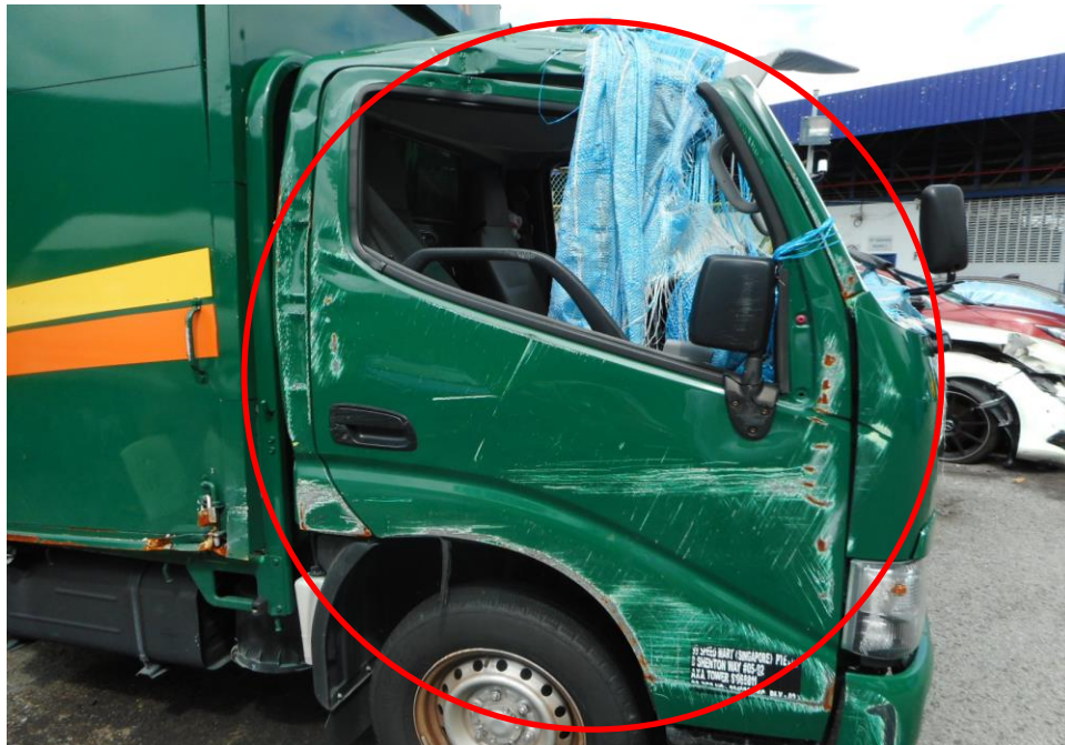
Photo 4 shows a close up view of the right body of the Motor Lorry at the time of our inspection. The Motor Lorry was observed to have sustained damages to its right door (circled) as a result of the accident.
