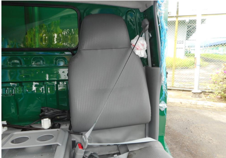
Photo 26 shows that the seat belt on the left seat was tested and all the seat belts were able to be fastened securely into the respective pre-tensioners that were fitted at the sides of each seat.
