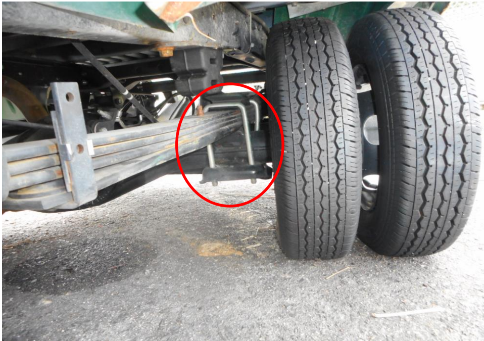
Photo 25 shows the undercarriage chassis (circled) of the Motor Lorry. It was observed to shift out of position due to the impact it had sustained as a result of the accident.
