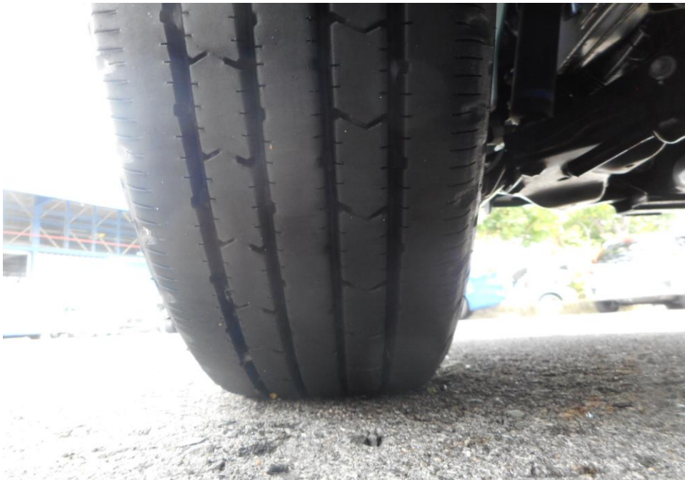
Photo 12 shows the condition of the front left tyres of the Motor Lorry, which observed to be in serviceable condition with remaining tread depth of approximately 7.9mm. The tyres, which were wrapped around standard steel wheel rim, were also observed to be sufficiently inflated for vehicular operation.
