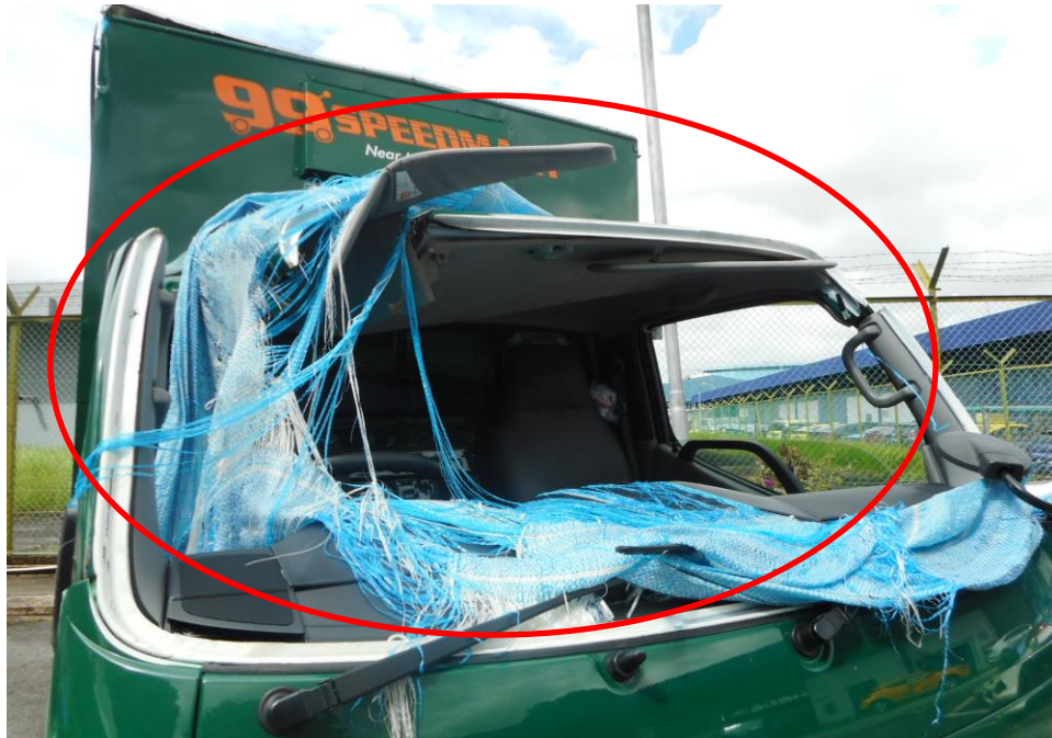
Photo 2 shows a close up view of the front body of the Motor Lorry at the time of our inspection. The Motor Lorry was observed to have sustained extensive damages to its front windscreen and front cabin body panel (circled) as a result of the accident.
