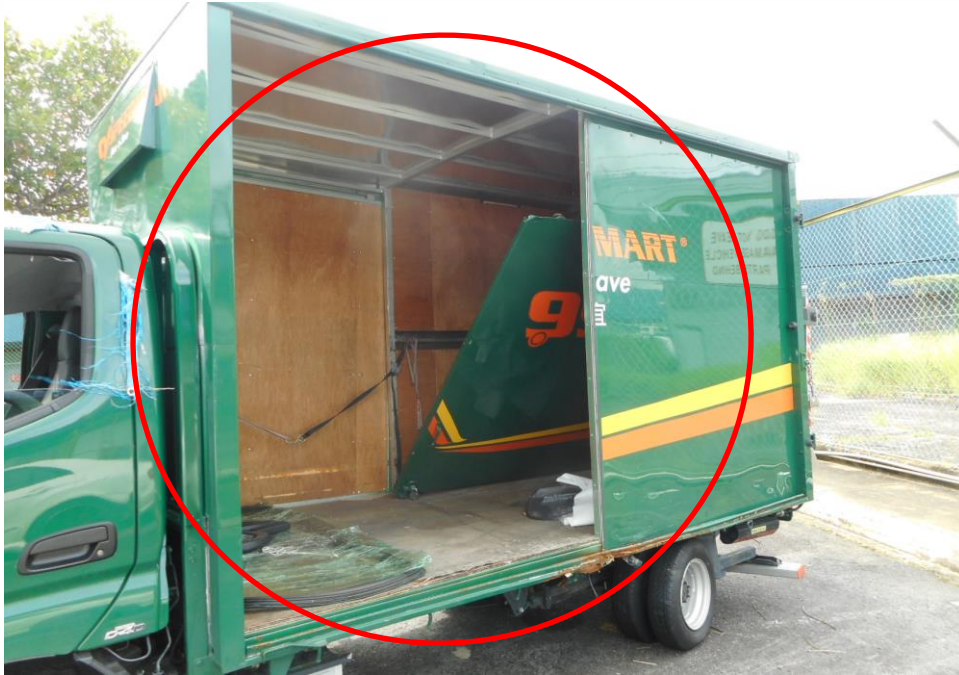
Photo 7 shows a close up view of the left body of the Motor Lorry at the time of our inspection. The Motor Lorry was observed to have sustained damages to its rear cabin body panel (circled) as a result of the accident.
