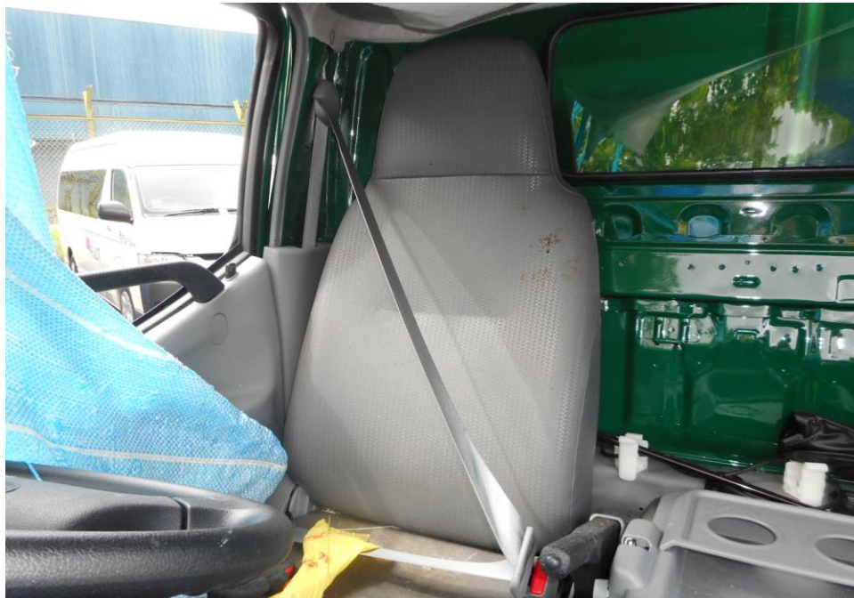
Photo 27 shows that the seat belt on the right seat was tested and all the seat belts were able to be fastened securely into the respective pre-tensioners that were fitted at the sides of each seat.
