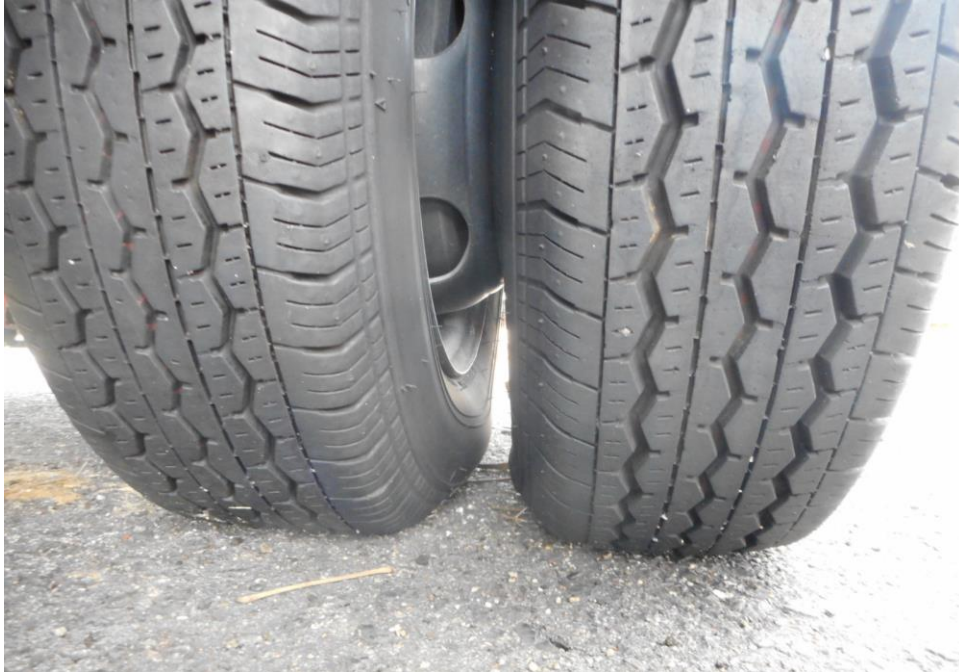
Photo 11 shows the condition of the rear left tyre of the Motor Lorry, which was observed to be in serviceable condition with remaining tread depth of approximately 5mm. The tyre, which was wrapped around standard steel wheel rim, was also observed to be sufficiently inflated for vehicular operation.
