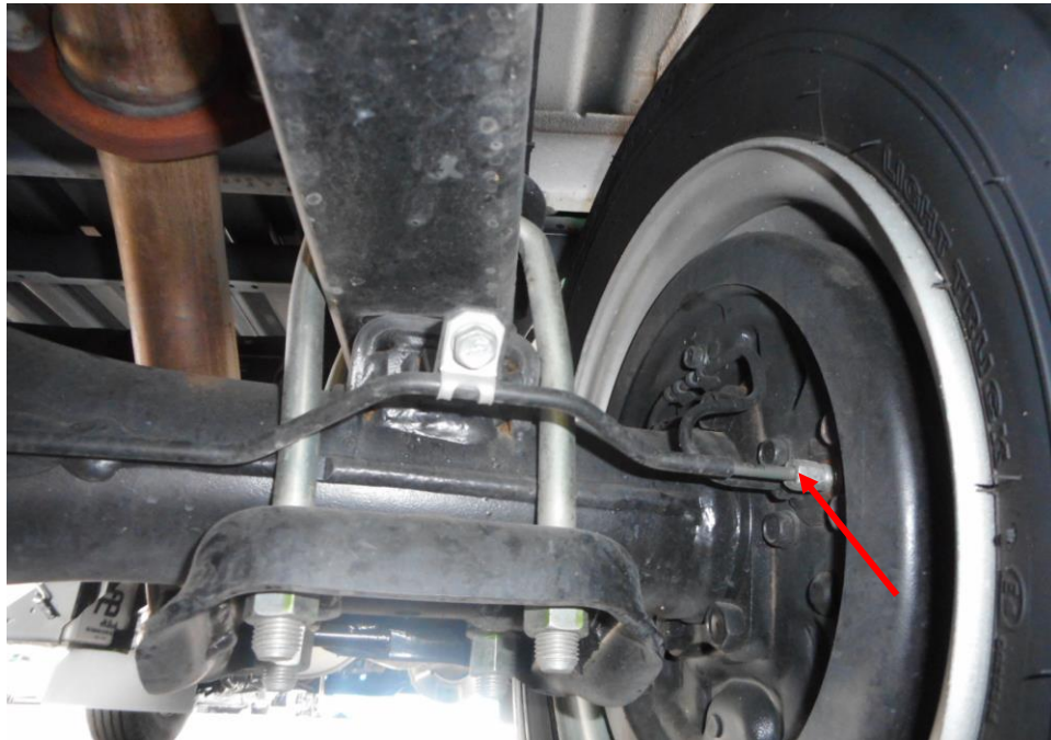
Photo 21 shows the brake pipe (arrowed) at the rear right wheel of the Motor Lorry. I did not observe any leakage of brake fluid at the time of my inspection of the Motor Lorry. My static tests of the Motor Lorry's braking system, along with my visual examination of the various mechanical components in the braking system, had indicated that there was no internal leakage of pressure/vacuum.
