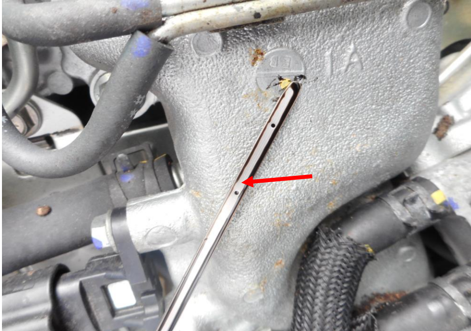
Photo 16 shows the engine oil dip stick of the Motor Lorry at the time of my inspection. The engine oil was observed to be of sufficient level (arrowed) and without any visible contamination.
