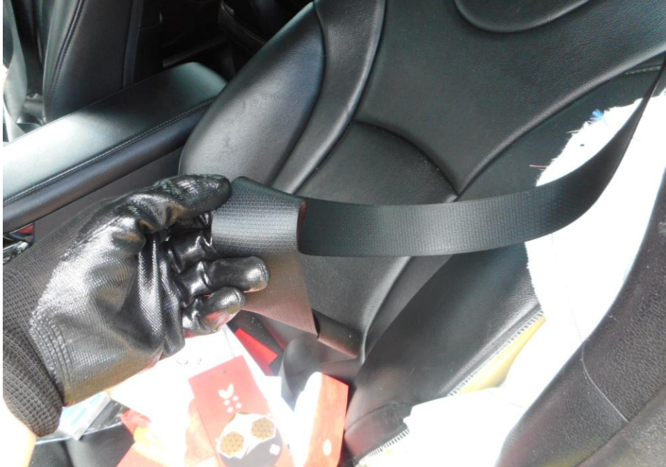
Photo 20 shows that the seat belt on the left seat was worn at the material time of accident as the safety pre-tensioners was activated at the moment of impact and caused the seat belt to be locked into the last position.
