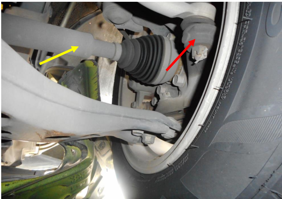
Photo 18 shows the various undercarriage components at the front right wheel of the Motor Taxi, in particular the steering tie rod end (arrowed) and drive shaft (yellow arrow). The various steering components were all found to be intact, suggesting that the steering system of the Motor Taxi was likely to be in serviceable condition at the material time of accident. There was also no sign of fluid stain(s) observed on the various undercarriage components.
