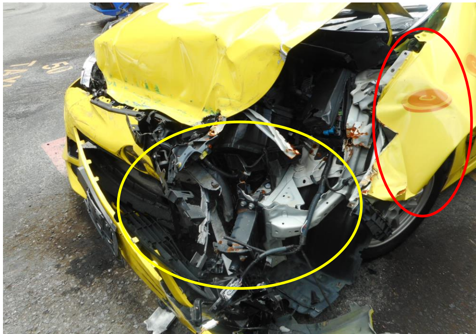
Photo 4 shows a general view of the Motor Taxi's engine compartment at the time of my inspection. The Motor Taxi was observed to have sustained damage at its front portion. Its front left fender (red circle) was amongst the body parts and various components (yellow circle) in the engine compartments were also damaged as a result of the accident.
