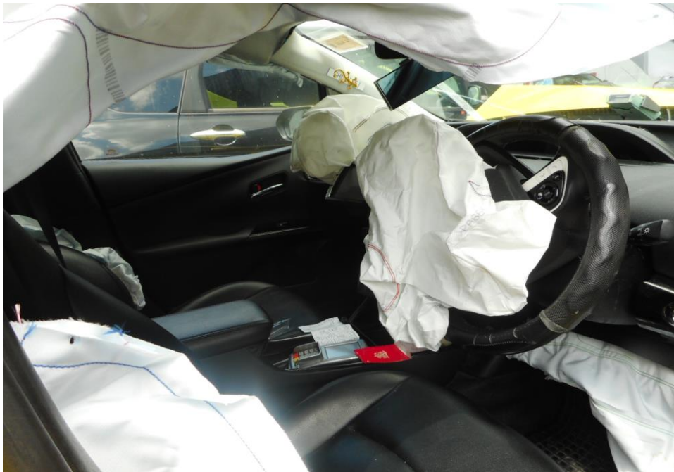
Photo 12 shows the deployment of the Supplemental Restraint System (SRS) airbag (arrowed) in the Motor Taxi as a result of the accident.
