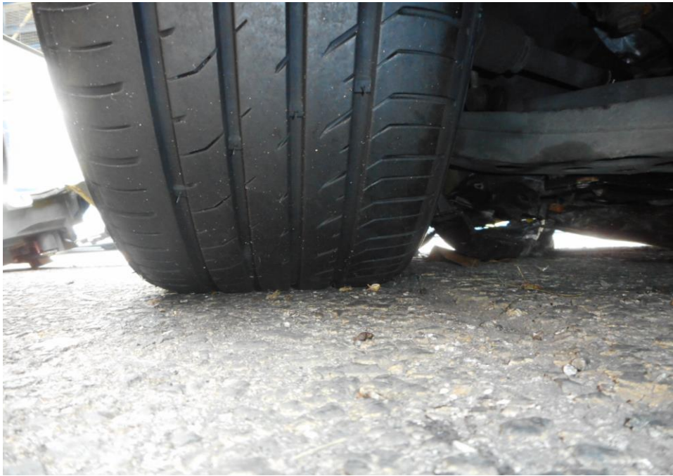
Photo 11 shows the condition of the front left tyre of the Motor Taxi, which was observed to be in serviceable condition with remaining tread depth of approximately 5.6mm. The tyre was also observed to be sufficiently inflated for vehicular operation with no tear, cut or burst mark(s).
