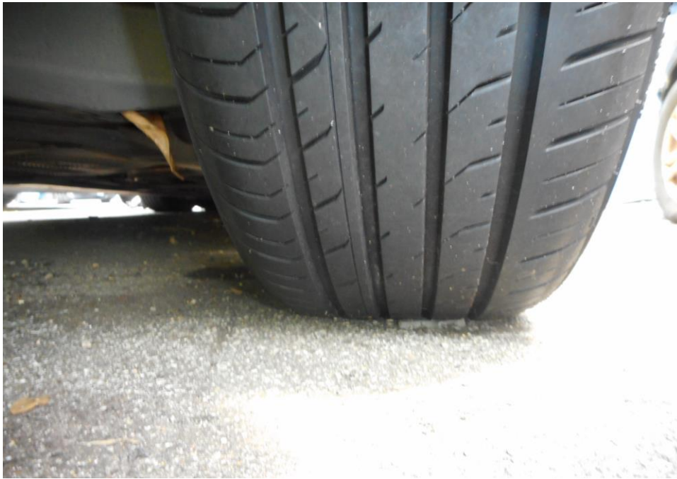
Photo 9 shows the condition of the rear right tyre of the Motor Taxi, which was observed to be in serviceable condition with remaining tread depth of approximately 6.7mm. The tyre was also observed to be sufficiently inflated for vehicular operation with no tear, cut or burst mark(s).
