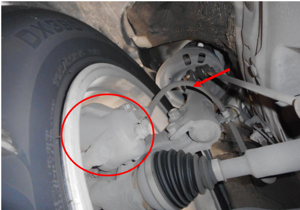
Photo 16 shows the brake hose/pipe (arrowed) at the front right wheel of the Motor Taxi. No leakage of brake fluid was observed. Visual examination of the various components of the braking system like the brake caliper (circled), brake booster, brake pedal etc. had revealed all to be intact and without visible damage at the time of accident. There was also no sign of fluid stain(s) observed on the various undercarriage components.
