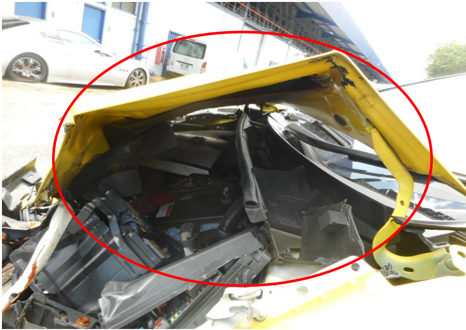
Photo 13 shows a close up view of the damaged front bonnet lock mechanism and the structure of the engine compartment of the Motor Taxi at the time of my inspection resulting it unable to open a result of the accident (circled) (Unable to open)
