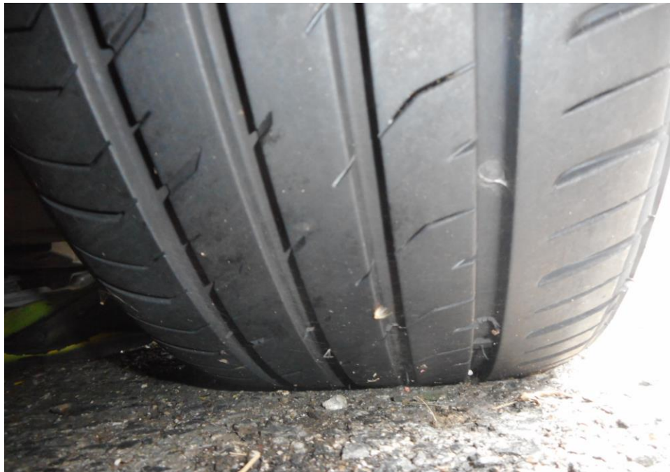
Photo 8 shows the condition of the front right tyre of the Motor Taxi, which was observed to be in serviceable condition with remaining tread depth of approximately 5.5mm. The tyre, which was wrapped around alloy wheel rim, was also observed to be sufficiently inflated for vehicular operation.
