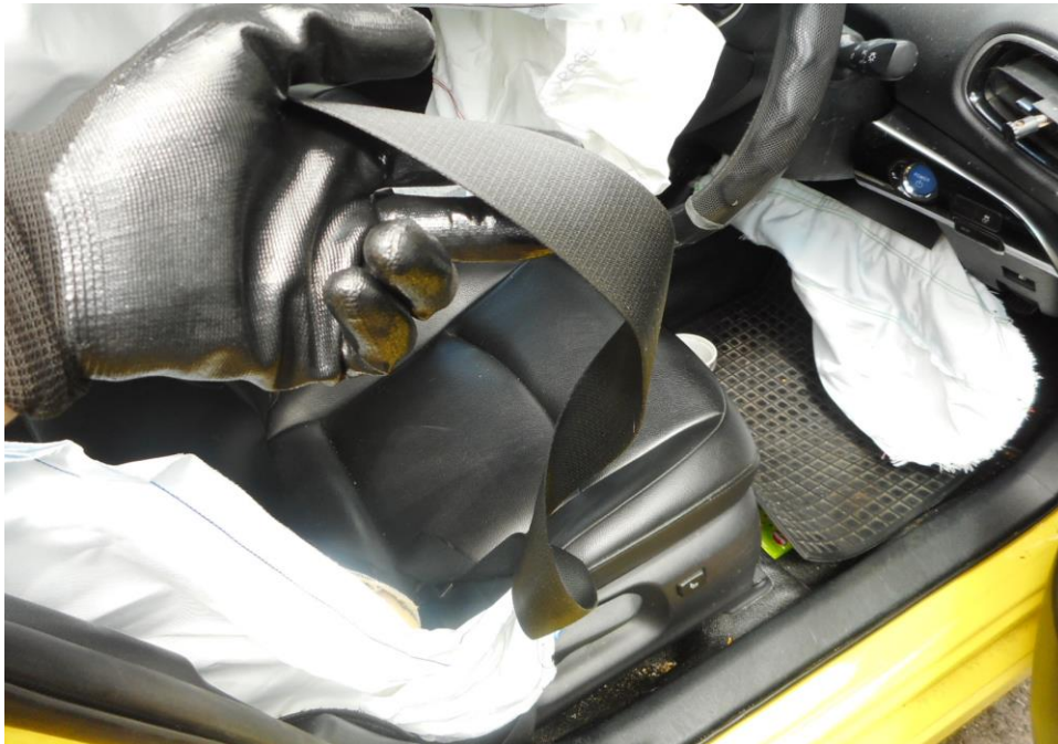
Photo 21 shows that the seat belt on the right seat was worn at the material time of accident as the safety pre-tensioners was activated at the moment of impact and caused the seat belts to be locked into the last position of the user.
