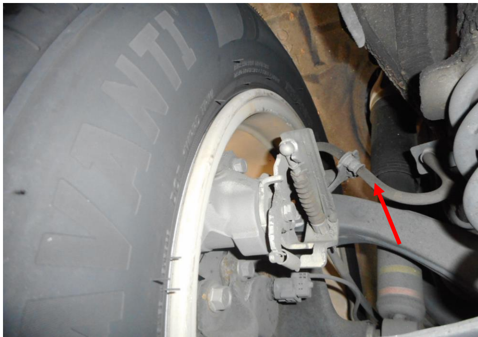
Photo 14 shows the brake hose/pipe (arrowed) at the rear left wheel of the Motor Taxi. No leakage of brake fluid was observed. Visual examination of the various components of the braking system like the drum brake, brake booster, brake pedal etc. had revealed all to be intact and without visible damage.
