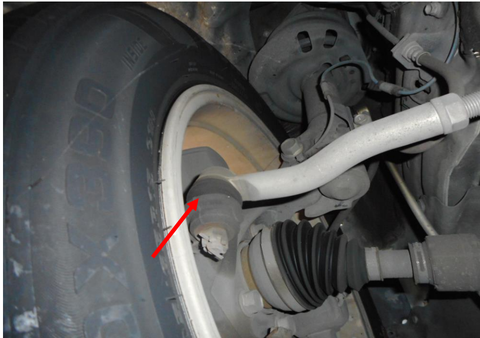
Photo 19 shows the various undercarriage components at the front left wheel of the Motor Taxi, in particular the steering tie rod end (arrowed). The various Undercarriage components of the Motor Taxi were all found to be intact without any visible damage. There was also no sign of fluid stain(s) observed on the various undercarriage components.
