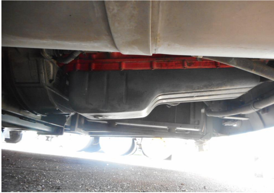
Photo 10 shows the undercarriage of the Motor Bus, at the area where the engine housing located. I did not find any sign(s) or indication(s) of fluid leak and/or fluid stain(s) on the underside of the Motor Bus.
