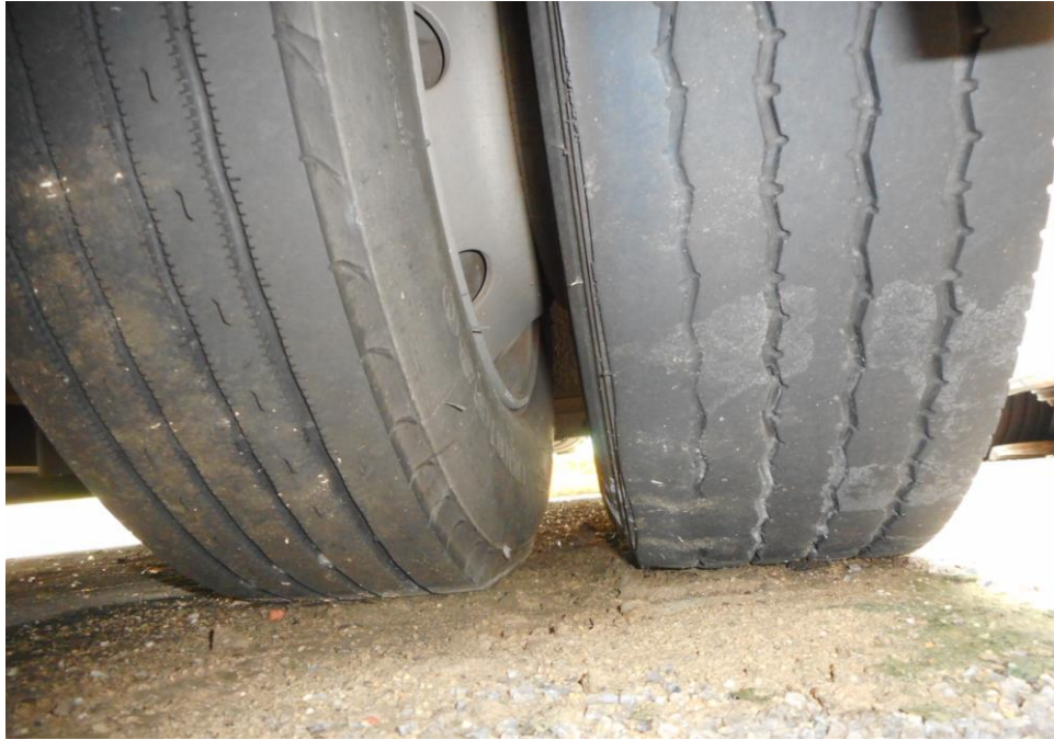
Photo 8 shows the condition of the rear left tyres of the Motor Bus, which was observed to be in serviceable condition with remaining tread depth of approximately 5.2mm. The tyres, which were wrapped around standard steel wheel rim, were also observed to be sufficiently inflated for vehicular operation. There was also no damage found on all 6 steel wheel rims of the Motor Bus.
