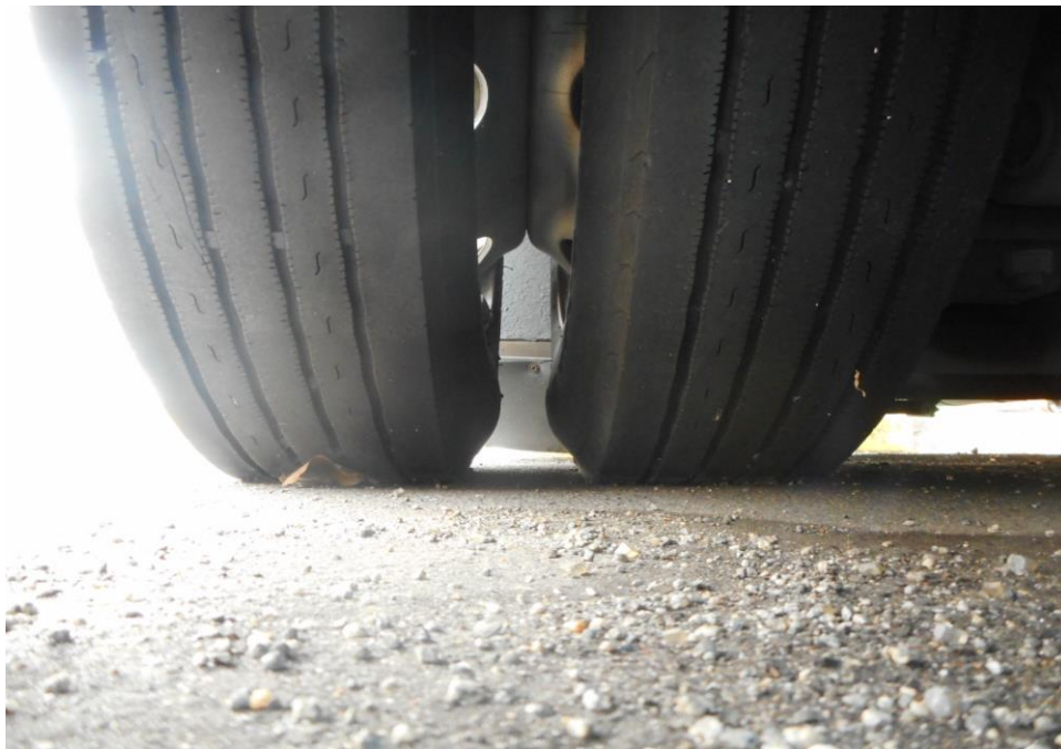
Photo 7 shows the condition of the rear right tyre of the Motor Bus, which was observed to be in serviceable condition with remaining tread depth of approximately 5.8mm. The tyre, which was wrapped around standard steel wheel rim, was also observed to be sufficiently inflated for vehicular operation.
