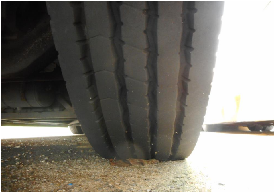
Photo 9 shows the condition of the front left tyres of the Motor Bus, which were observed to be in serviceable condition with remaining tread depth of approximately 12.2mm. There was also no tear, cut or burst mark(s) on the outer and the inner sidewalls as well as across the tread of the 6 tyres that were fitted on the Motor Bus.
