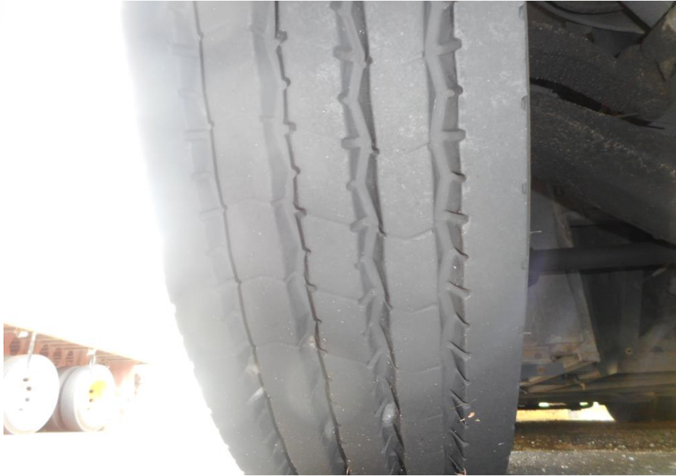
Photo 6 shows the condition of the front right tyre of the Motor Bus, which was observed to be in serviceable condition with remaining tread depth of approximately 12.1 mm. The tyre, which was wrapped around standard steel wheel rim, was also observed to be sufficiently inflated for vehicular operation. There was no tear, cut or burst mark(s) on the outer and the inner sidewalls as well as across the tread of the 6 tyres that were fitted on the Motor Bus.
