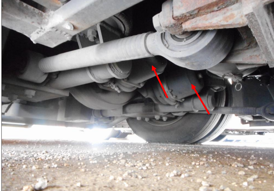
Photo 11 shows the brake air cylinder of both the rear left & right wheel (arrowed) of the Motor Bus. My visual inspection of the mechanical components of the Motor Bus braking system & i did not observe any leakage to suggest that its braking system was in serviceable condition at the material time of accident.
