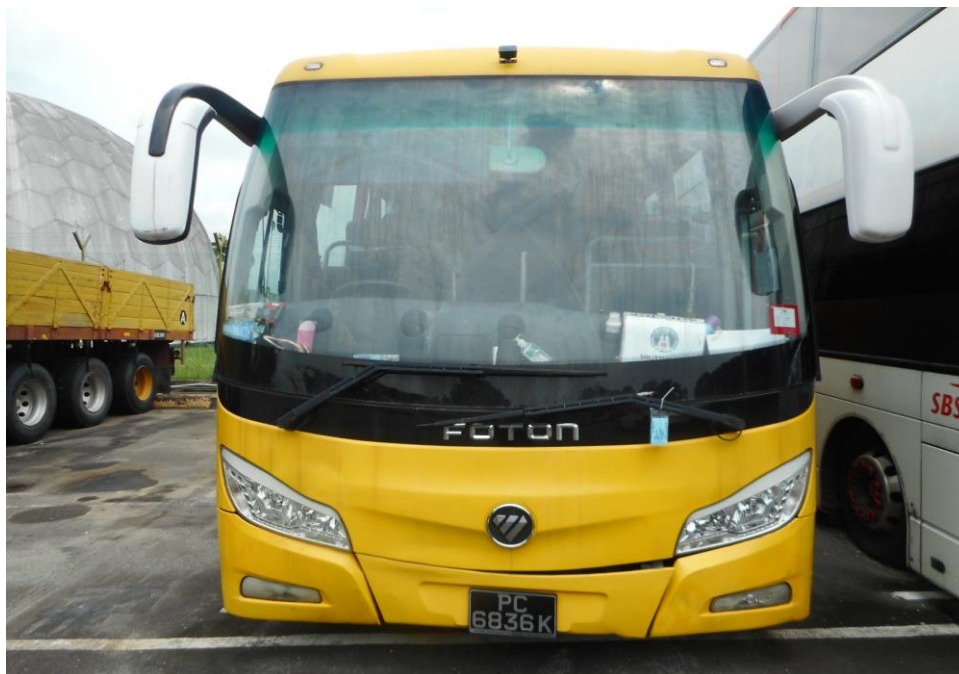
Photo 3 shows a general view of the front body of the Motor Bus front body at the time of my inspection. The front was observed to have been unaffected by the accident.
