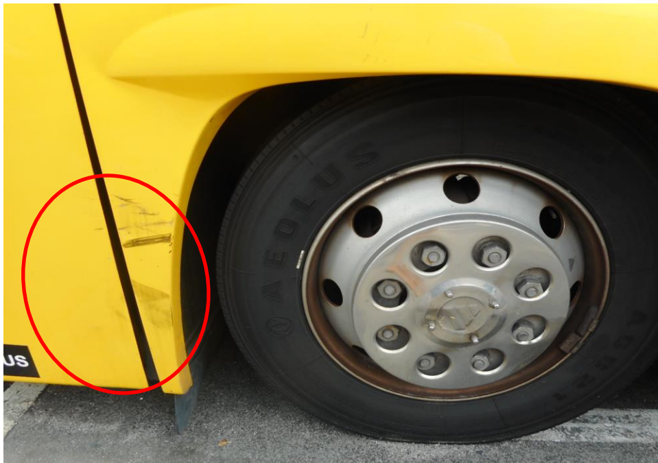
Photo 2 shows a close up view of the front right body of the Motor Bus at the time of my inspection. The Motor Bus was observed to have sustained damage at its right portion. Its right body panel (circled) were amongst the body parts that were damaged as a result of the accident.
