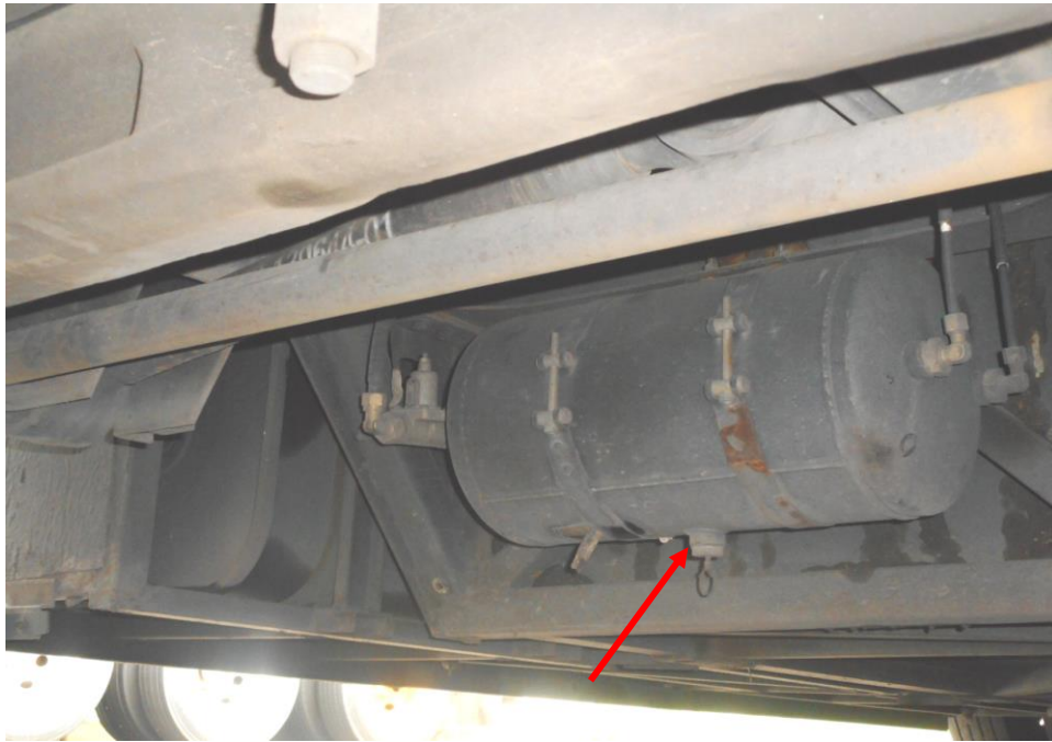
Photo 15 shows the air brake cylinders (arrowed) at the undercarriage of the Motor Bus. I did not observe any leakage of air brake fluid at the time of my inspection of the Motor Bus. My visual examination of the various mechanical components in the braking system had indicated that there was no internal leakage of pressure/vacuum. Hence the braking system of the Motor Bus was likely to be in serviceable condition at the material time of accident.
