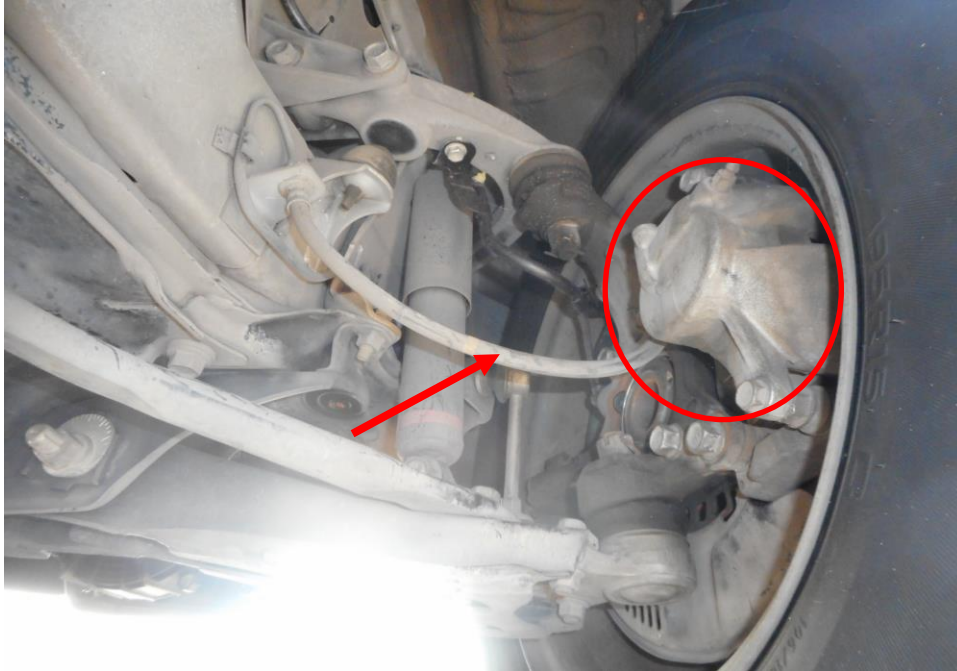
Photo 20 shows the brake hose/pipe (arrowed) at the front right wheel of the Motor Van. No leakage of brake fluid was observed. Visual examination of the various components of the braking system like the brake caliper (circled), brake booster, brake pedal etc had revealed all to be intact and without visible damage at the time of accident. There was also no sign of fluid stain(s) observed on the various undercarriage components.
