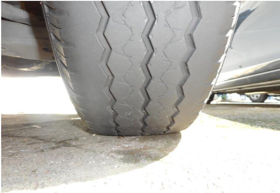
Photo 6 shows the condition of the front right tyre of the Motor Van, which was observed to be in serviceable condition with remaining tread depth of approximately 5.5mm. The tyre, which was wrapped around standard alloy wheel rim, was also observed to be sufficiently inflated for vehicular operation. There was no tear, cut or burst mark(s) on the outer and the inner sidewalls as well as across the tread of the 4 tyres that were fitted on the Motor Van.
