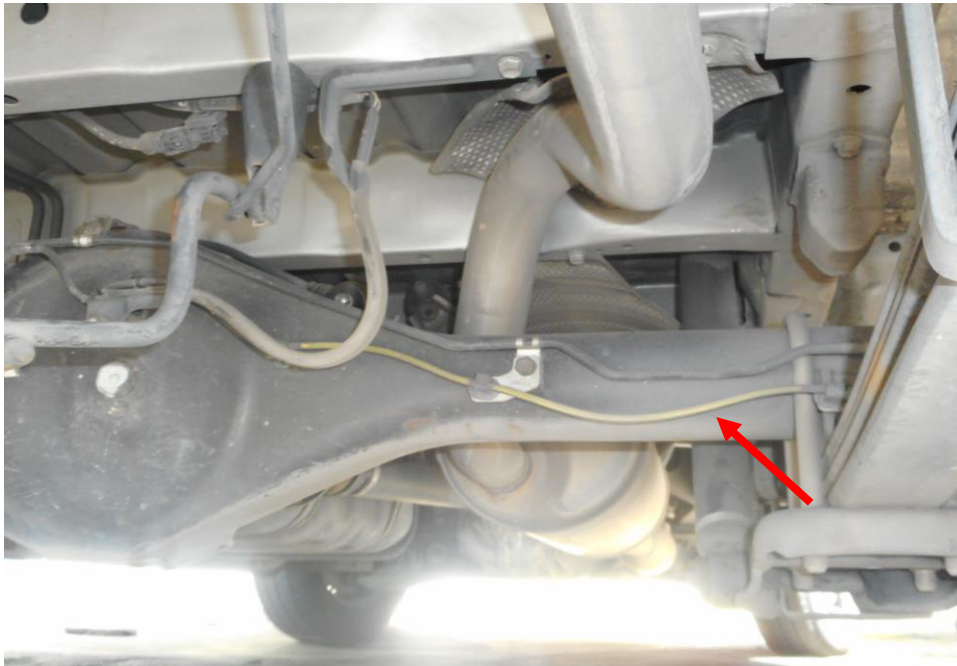
Photo 22 shows the various undercarriage components at the rear right wheel of the Motor Van, in particular the drive shaft (arrowed). The various steering components were all found to be intact, suggesting that the steering system of the Motor Van was likely to be in serviceable condition at the material time of accident. There was also no sign of fluid stain(s) observed on the various undercarriage components.
