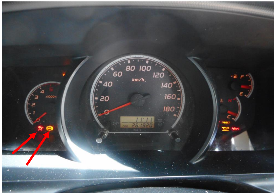
Photo 24 shows the warning light for Anti-Lock Brake System (ABS) and Supplemental Restraint System (SRS) appearing on the instrument panel of the Motor Van during the self-test of its various electronic operating systems when its engine was cranked.
