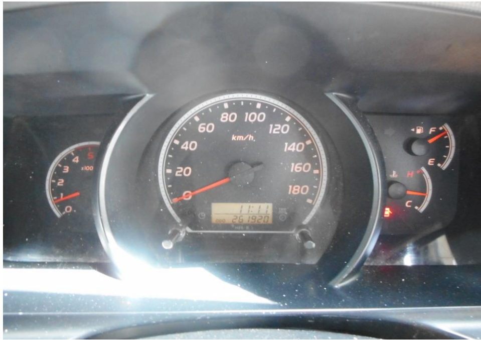
Photo 25 shows no warning lights illuminated on the instrument panel of the Motor Van after the engine was cranked. This would suggest that there was no abnormality to the various electronic operating systems of the Motor Van, like the ABS and SRS.
