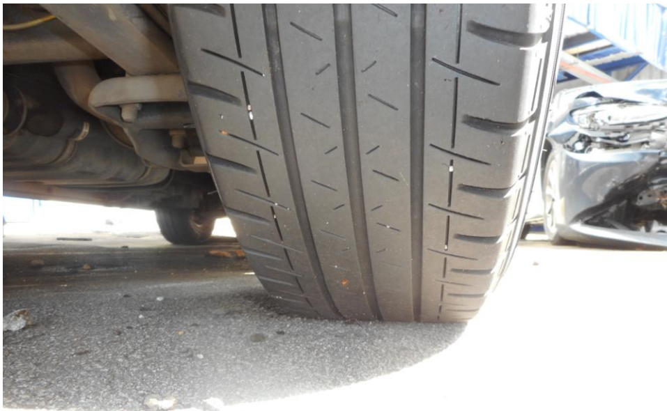
Photo 6 shows the condition of the front right tyre of the Motor Van, which was observed to be in serviceable condition with remaining tread depth of approximately 5.5mm. The tyre, which was wrapped around standard alloy wheel rim, was also observed to be sufficiently inflated for vehicular operation. There was no tear, cut or burst mark(s) on the outer and the inner sidewalls as well as across the tread of the 4 tyres that were fitted on the Motor Van.
