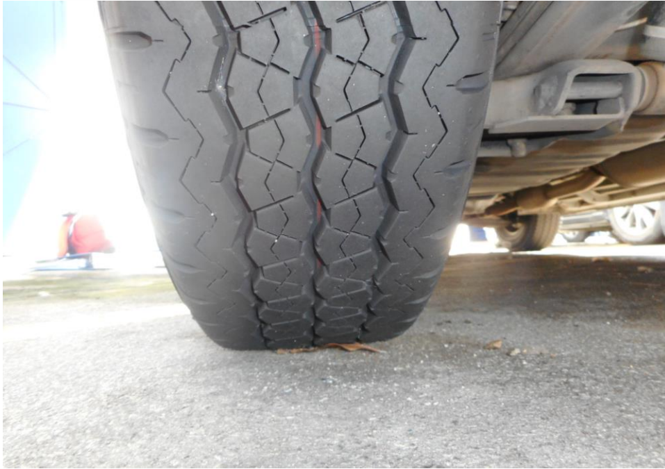
Photo 8 shows the condition of the rear left tyres of the Motor Van, which was observed to be in serviceable condition with remaining tread depth of approximately 8.1mm. The tyres, which were wrapped around standard alloy wheel rim, were also observed to be sufficiently inflated for vehicular operation. There was also no damage found on all 4 alloy wheel rims of the Motor Van.
