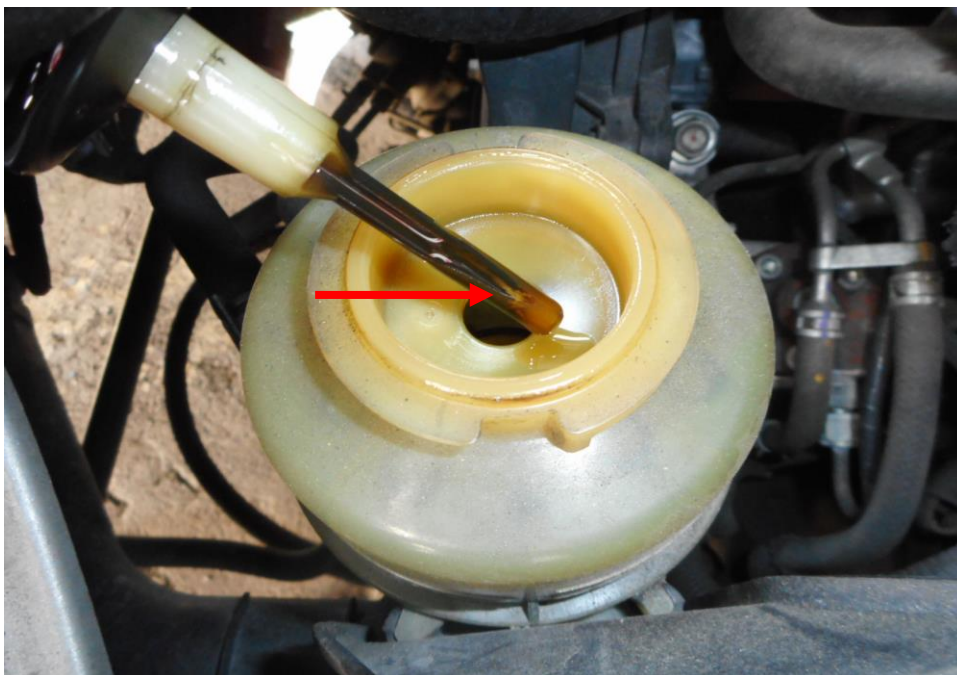
Photo 14 shows the power steer fluid reservoir of the Motor Van at the time of my inspection. The power steering fluid was observed to be of sufficient level (arrowed) and without any visible contamination.
