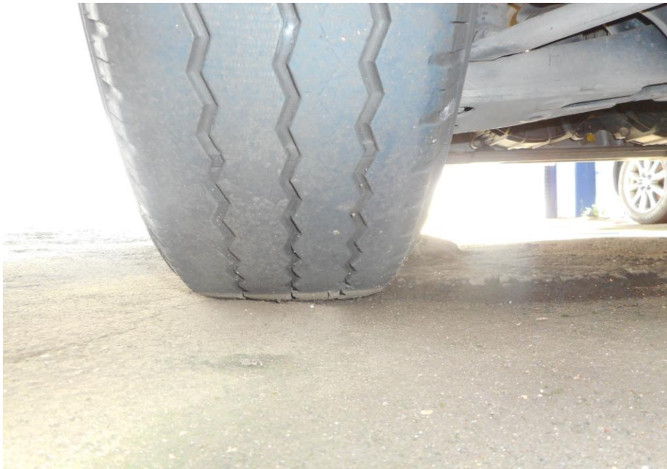
Photo 9 shows the condition of the rear right tyres of the Motor Van, which were observed to be in serviceable condition with remaining, tread depth of approximately 4.9mm. There was also no tear, cut or burst mark(s) on the outer and the inner sidewalls as well as across the tread of the 4 tyres that were fitted on the Motor Van.
