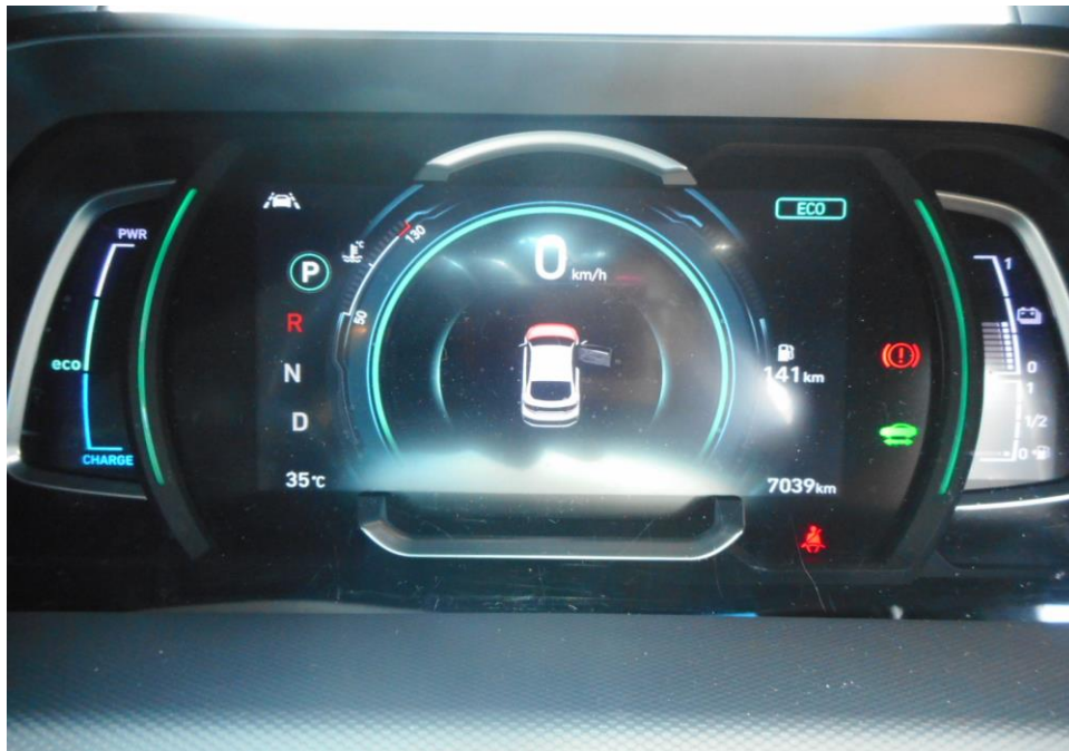
Photo 24 shows no warning lights illuminated on the instrument panel of the Motor Taxi after the engine was cranked. This would suggest that there was no abnormality to the various electronic operating systems of the Motor Taxi, like the ABS, SRS, TC and EPS.
