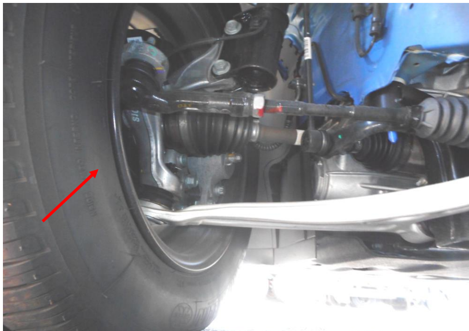
Photo 17 shows the various undercarriage components at the front left wheel of the Motor Taxi, in particular the steering tie rod end (arrowed). The various Undercarriage components of the Motor Taxi were all found to be intact without any visible damage. There was also no sign of fluid stain(s) observed on the various undercarriage components.
