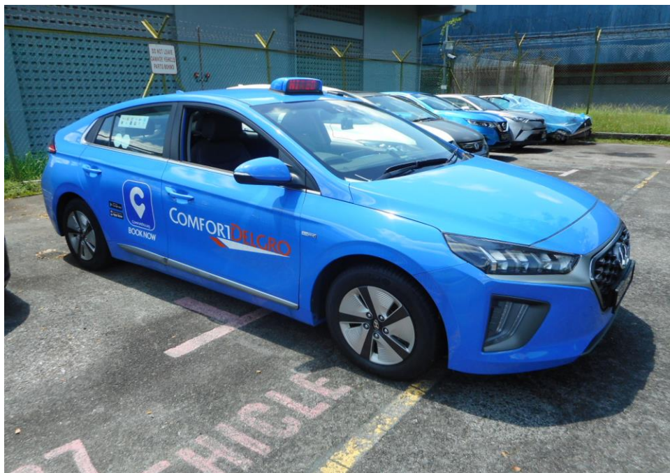
Photo 3 shows a general view of the right body of the Motor Taxi at the time of my inspection. The Motor Taxi was observed to visually sustain damage at its front right door and fender portion which had caused difficult in opening the door.
