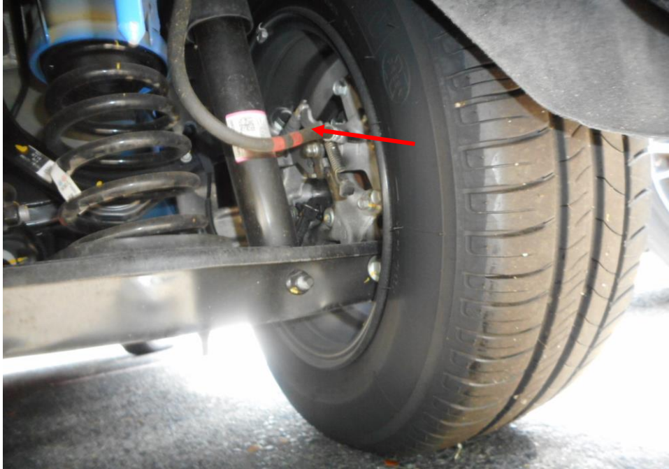
Photo 18 shows the brake pipe (arrowed) at the rear right wheel of the Motor Taxi. I did not observe any leakage of brake fluid at the time of my inspection of the Motor Taxi. My static tests of the Motor Taxi's braking system, along with my visual examination of the various mechanical components in the braking system, had indicated that there was no internal leakage of pressure/vacuum. Hence the braking system of the Motor Taxi was likely to be in serviceable condition at the material time of accident.
