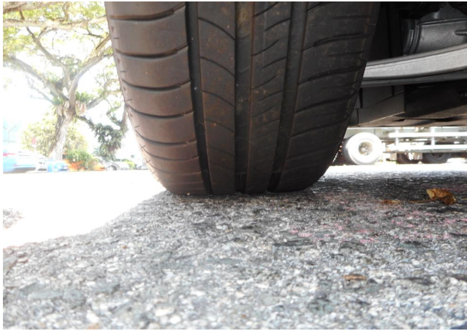
Photo 10 shows the condition of the rear right tyres of the Motor Taxi, which were observed to be in serviceable condition with remaining, tread depth of approximately 5.2mm. There was also no tear, cut or burst mark(s) on the outer and the inner sidewalls as well as across the tread of the 4 tyres that were fitted on the Motor Taxi.
