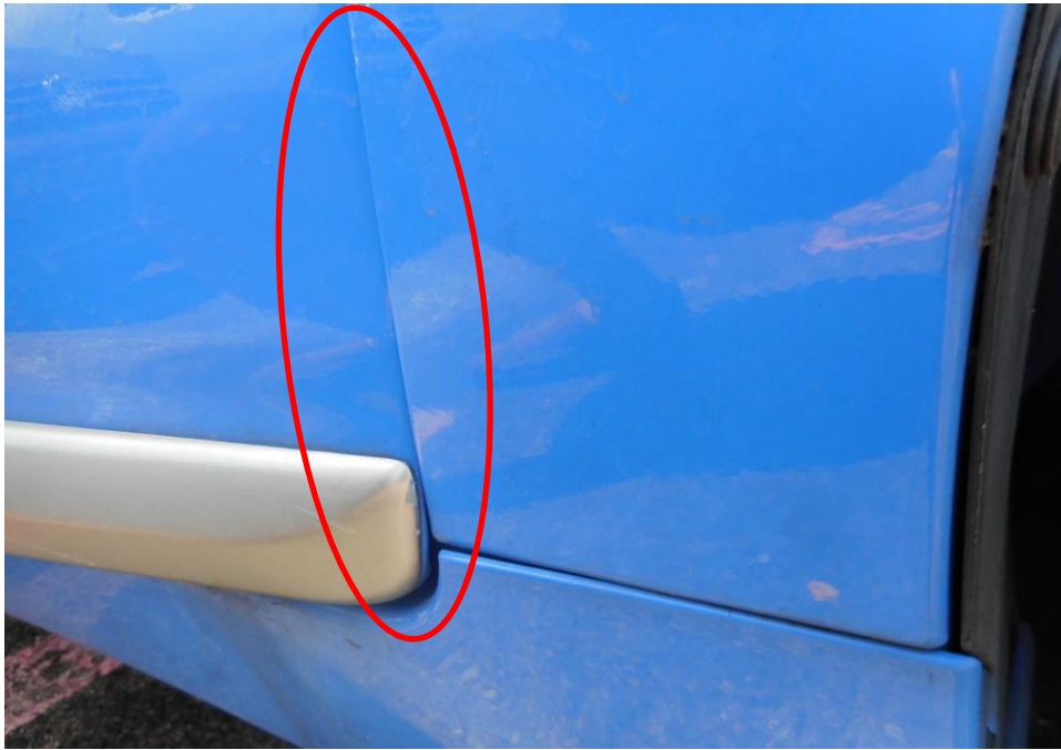
Photo 4 shows a close up view of the right body of the Motor Taxi at the time of my inspection. The Motor Taxi was observed to visually sustain damage at its front right bumper and fender portion (circled) which had cause difficult in opening the door.
