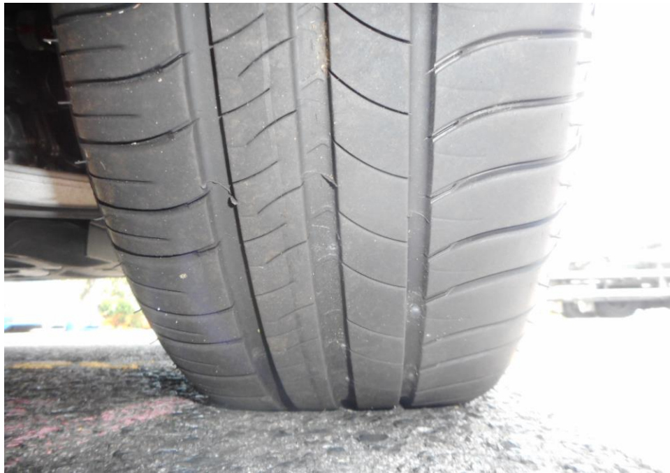
Photo 7 shows the condition of the front right tyre of the Motor Taxi, which was observed to be in serviceable condition with remaining tread depth of approximately 5.4mm. The tyre, which was wrapped around standard alloy wheel rim, was also observed to be sufficiently inflated for vehicular operation. There was no tear, cut or burst mark(s) on the outer and the inner sidewalls as well as across the tread of the 4 tyres that were fitted on the Motor Taxi.
