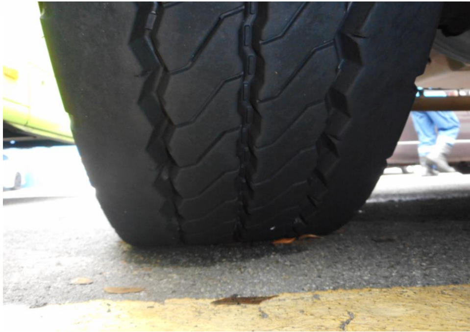
Photo 14 shows the condition of the front left tyre of the Motor Lorry, which were observed to be in serviceable condition with remaining, tread depth of approximately 14.4mm. There was also no tear, cut or burst mark(s) on the outer and the inner sidewalls as well as across the tread of the 6 tyres that were fitted on the Motor Lorry.
