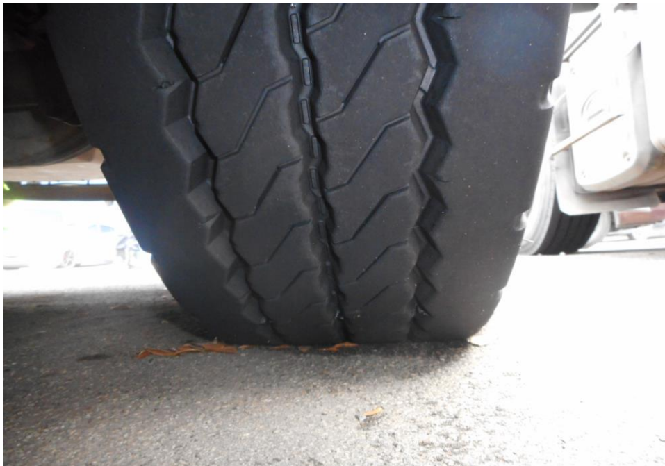
Photo 11 shows the condition of the front right tyre of the Motor Lorry, which was observed to be in serviceable condition with remaining tread depth of approximately 13.7mm. The tyre, which was wrapped around standard steel wheel rim, was also observed to be sufficiently inflated for vehicular operation. There was no tear, cut or burst mark(s) on the outer and the inner sidewalls as well as across the tread of the 6 tyres that were fitted on the Motor Lorry.
