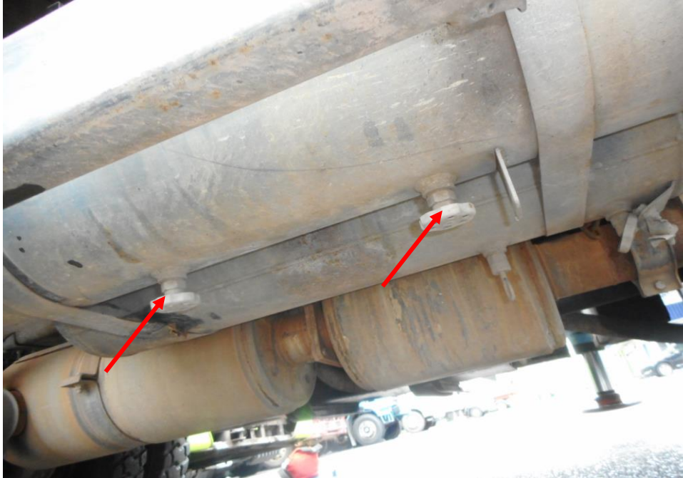
Photo 26 shows the air brake cylinders (arrowed) at the undercarriage of the Motor Lorry. I did not observe any leakage of air brake fluid at the time of my inspection of the Motor Lorry. My static tests of the Motor Lorry's braking system, along with my visual examination of the various mechanical components in the braking system had indicated that there was no internal leakage of pressure/vacuum. Hence the braking system of the Motor Lorry was likely to be in serviceable condition at the material time of accident.
