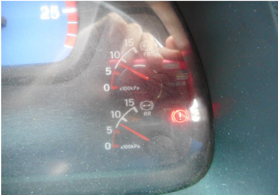
Photo 16 shows the air in the air brake cylinders of the Motor Lorry at the time of my inspection. The air in the cylinder was observed to be of sufficient level & serviceable at the time of the accident.
