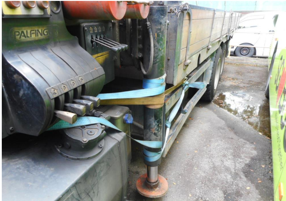
Photo 6 shows a general view of the left hydraulic arm of the Motor Lorry at the time of my inspection. The left hydraulic arm was observed to be damaged as a result of the accident, it was strapped in by ropes as the hydraulic arm will extend out of place when not strapped in.
