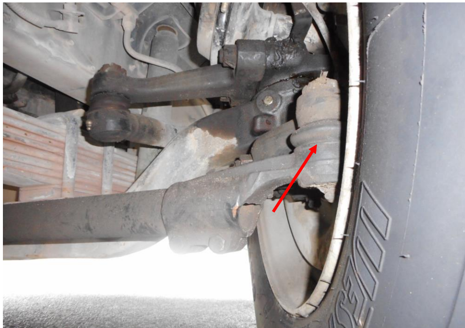
Photo 21 shows the various undercarriage components at the front right wheel of the Motor Lorry, in particular the steering tie rod end (arrowed). The various steering components were all found to be intact, suggesting that the steering system of the Motor Lorry was likely to be in serviceable condition at the material time of accident. There was also no sign of fluid stain(s) observed on the various undercarriage components.
