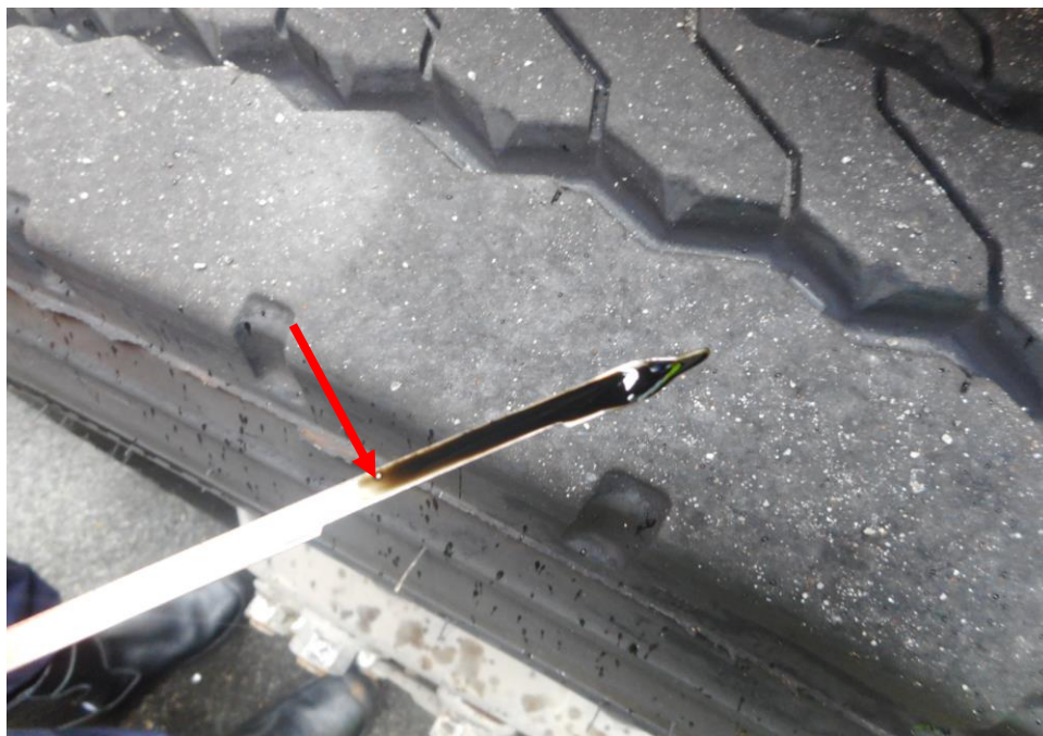
Photo 18 shows the engine oil dip stick of the Motor Lorry at the time of my inspection. The engine oil was observed to be of sufficient level (arrowed) and without any visible contamination.
