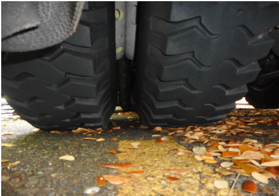
Photo 13 the condition of the rear left tyres of the Motor Lorry, which was observed to be in serviceable condition with remaining, tread depth of approximately 12.6mm. The tyres, which were wrapped around standard steel wheel rim, were also observed to be sufficiently inflated for vehicular operation. There was also no damage found on all 6 steel wheel rims of the Motor Lorry.
