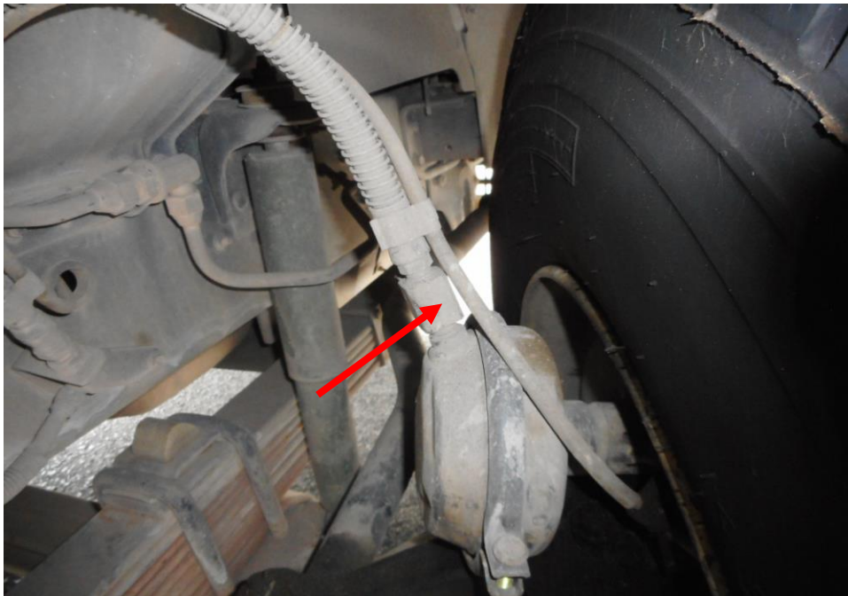
Photo 27 shows the brake hose/pipe (arrowed) at the front right wheel of the Motor Lorry. I did not observe any leakage of brake fluid at the time of my inspection of the Motor Lorry. My static tests of the Motor Lorry's braking system, along with my visual examination of the various mechanical components in the braking system had indicated that there was no internal leakage of pressure/vacuum. Hence the braking system of the Motor Lorry was likely to be in serviceable condition at the material time of accident.
