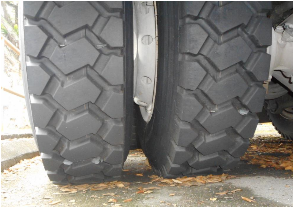
Photo 12 shows the condition of the rear right tyres of the Motor Lorry, which was observed to be in serviceable condition with remaining, tread depth of approximately 14.7mm. The tyres, which were wrapped around standard steel wheel rim, were also observed to be sufficiently inflated for vehicular operation. There was also no damage found on all 6 steel wheel rims of the Motor Lorry.
