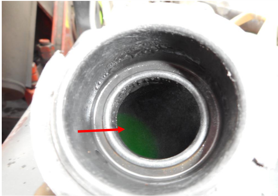
Photo 17 shows the engine coolant reservoir of the Motor Lorry at the time of my inspection. The engine coolant was observed to be of sufficient level (arrowed) and without any visible contamination.
