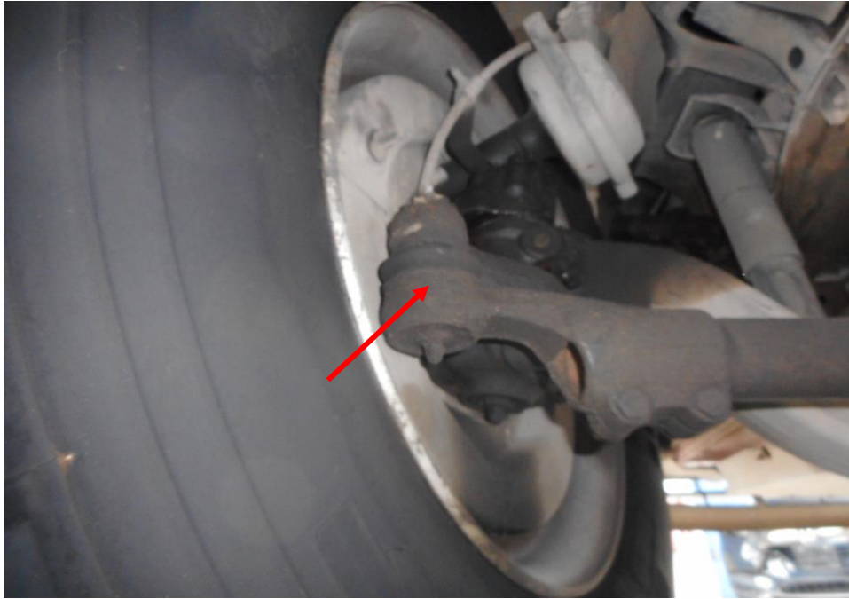
Photo 22 shows the various undercarriage components at the front left wheel of the Motor Lorry, in particular the steering tie rod end (arrowed). The various Undercarriage components of the Motor Lorry were all found to be intact without any visible damage. There was also no sign of fluid stain(s) observed on the various undercarriage components.
