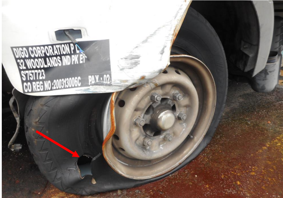
Photo 10 shows the condition of the front left tyre of the Motor Lorry, which was observed to be in unserviceable condition as it was observed with a cut on the sidewall (arrowed) with remaining tread depth of approximately 4.8mm. The tyre, which was wrapped around standard steel wheel rim.
