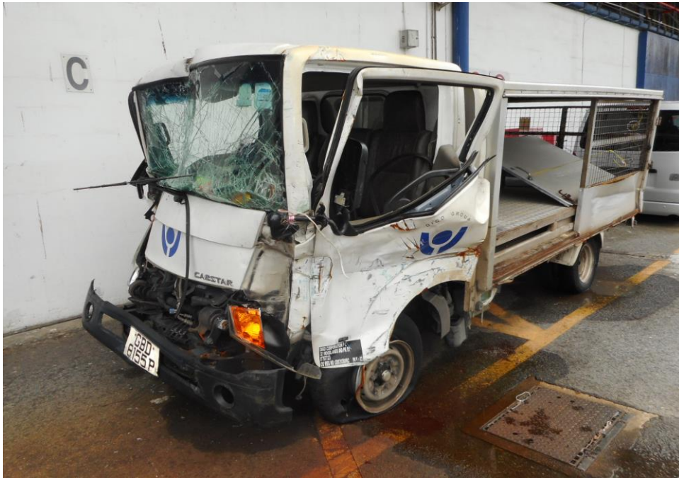
Photo 4 shows a general view of the left body of the Motor Lorry at the time of our inspection. The Motor Lorry was observed to have sustained major damages to its doors that was crushed and dislodged due to the accident's impact.
