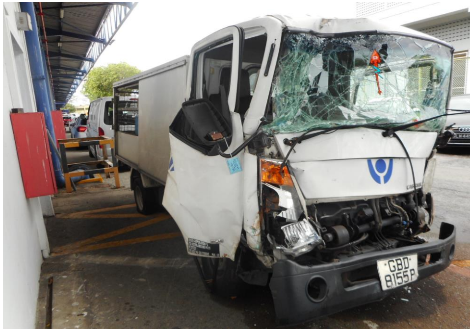
Photo 5 shows a general view of the right body of the Motor Lorry at the time of our inspection. The Motor Lorry was observed to have sustained major damages to its doors that was crushed and dislodged due to the accident's impact.
