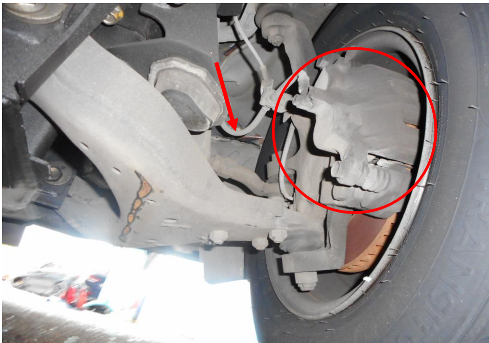
Photo 19 shows the various undercarriage components at the front right wheel of the Motor Lorry, in particular the brake hose (arrowed) and callipers (circled). The various undercarriage components of the Motor Lorry were all found to be intact without any visible damage. There was also no sign of fluid stain(s) observed on the various undercarriage components.
