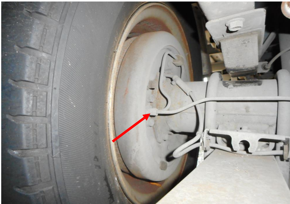
Photo 21 shows the various undercarriage components at the rear left wheel of the Motor Lorry, in particular the brake hose and drum brake (arrowed). The various undercarriage components of the Motor Lorry were all found to be intact without any visible damage. There was also no sign of fluid stain(s) observed on the various undercarriage components.
