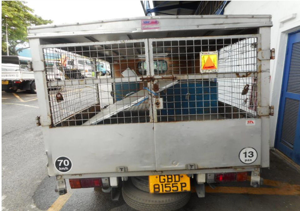
Photo 8 shows the number plate and the general view of the rear portion of the Motor Lorry at the time of our inspection. The Motor Lorry was observed sustained major damages to its rear which the tailgate was shifted out of place, likely due to the accident's impact.
