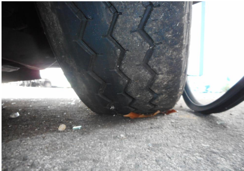
Photo 11 shows the condition of the front right tyre of the Motor Lorry, which was observed to be in serviceable condition with remaining tread depth of approximately 4.7mm. The tyre, which was wrapped around standard steel wheel rim, was also observed to be sufficiently inflated for vehicular operation.
