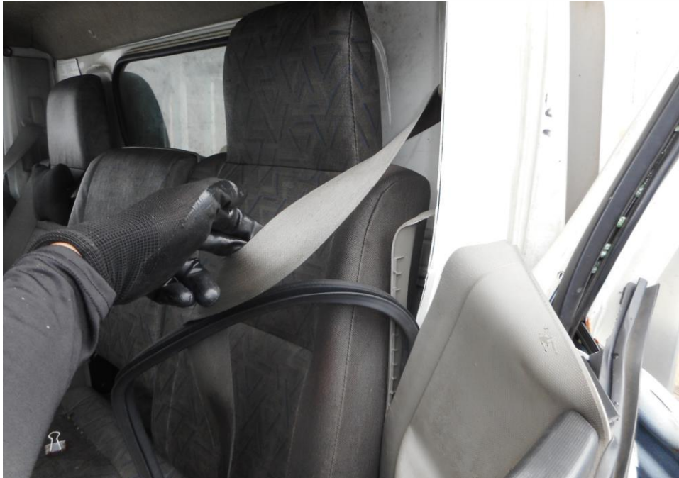
Photo 23 shows that the seat belt on the left seat was worn at the material time of accident as the safety pre-tensioners was activated at the moment of impact and caused the seat belts to be locked into the last position of the user.
