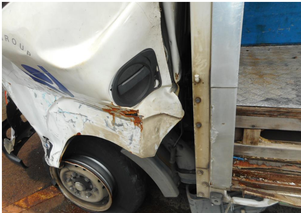
Photo 14 shows the induced damage to the cabin of the Motor Lorry's which immobilised the opening and viewing of the various parts and components inside the engine compartment, a result of the accident.
