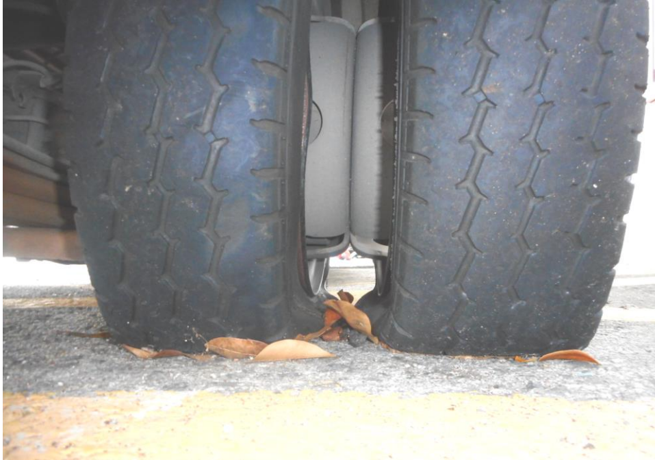
Photo 12 shows the condition of the rear left tyres of the Motor Lorry, which observed to be in serviceable condition with remaining tread depth of approximately 1.7mm. The tyres, which were wrapped around standard steel wheel rim, were also observed to be sufficiently inflated for vehicular operation.
