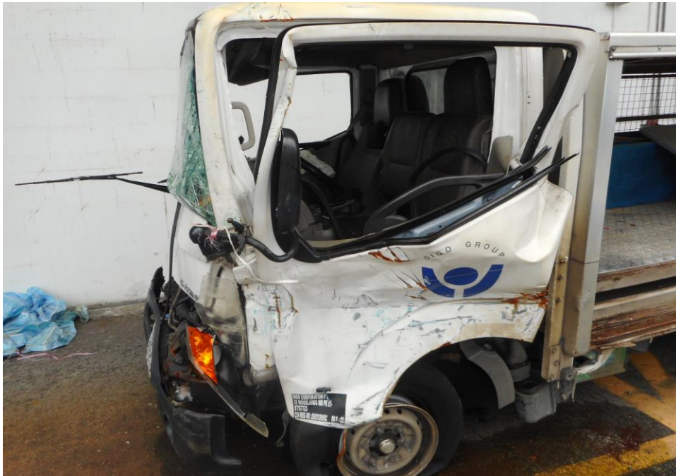
Photo 6 shows the close up view of the left door of the Motor Lorry at the time of our inspection. The Motor Lorry was observed to have sustained major damages to its doors that was crushed and dislodged due to the accident's impact.
