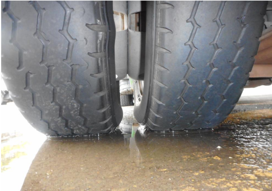
Photo 13 shows the condition of the rear right tyres of the Motor Lorry, which were observed to be in serviceable condition with remaining, tread depth of approximately 1.7mm. See above.
