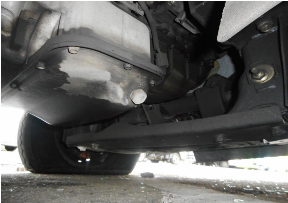
Photo 16 shows the undercarriage of the engine of the Motor Lorry at the time of our inspection. There was also sign(s) and indication(s) of old fluid stain within the engine undercarriage area.
