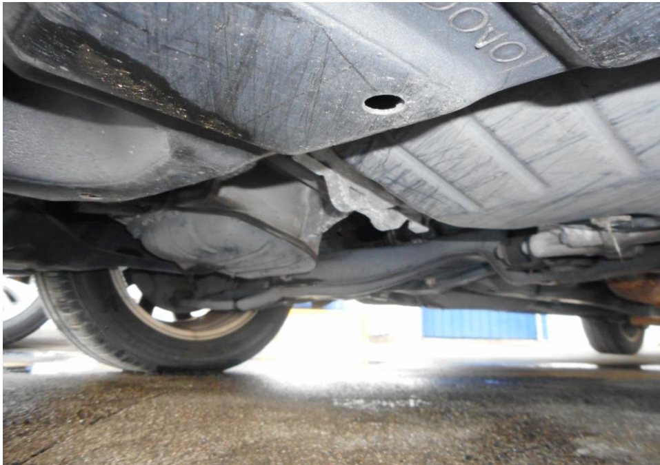
Photo 16 shows the undercarriage of the Motor Car, at the area where the engine housing and transmission housing are located. . I did not find any sign(s) or indication(s) of fluid leak and/or fluid stain(s) on the underside of the Motor Car.
