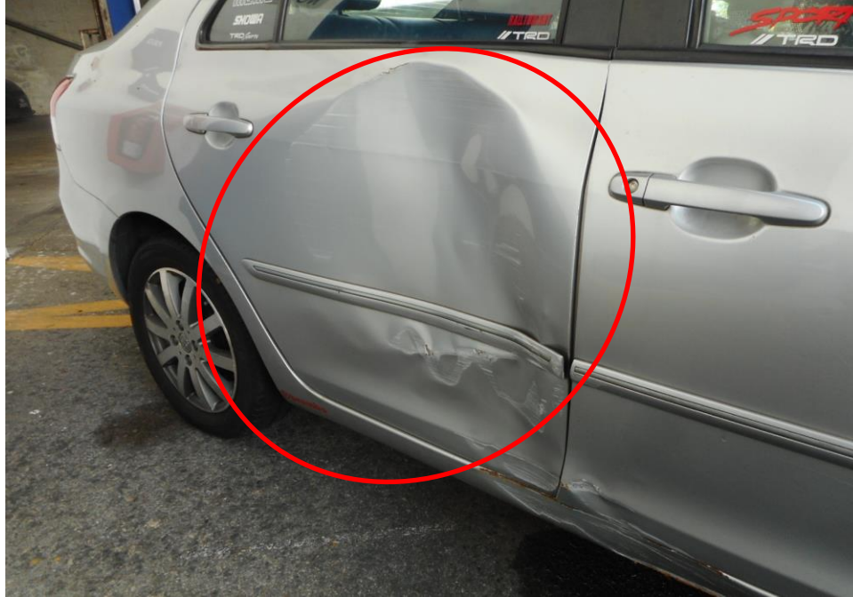
Photo 5 shows a close up view of the Motor Car's right body at the time of my inspection. The right portion of the Motor Car was observed to have been damaged, its right body panel (circled) was damaged as a result of the accident.
