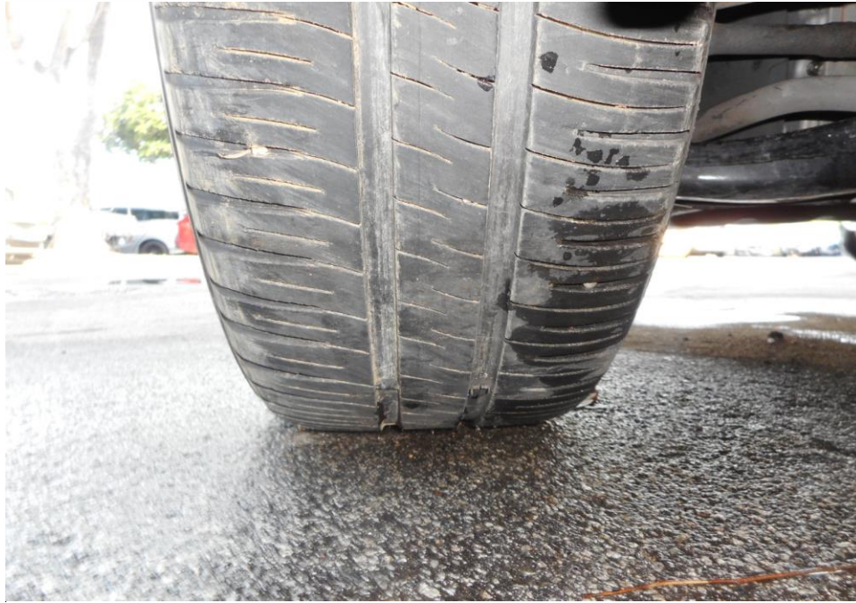
Photo 11 shows the condition of the front left tyre of the Motor Car, which was observed to be in serviceable condition with remaining tread depth of approximately 4.1mm. The tyre was also observed to be sufficiently inflated for vehicular operation with no tear, cut or burst mark(s).
