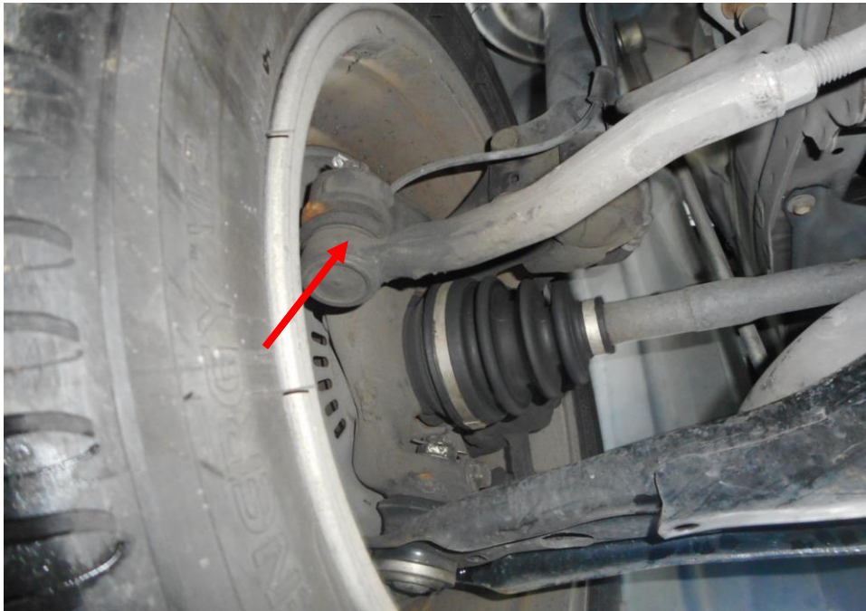
Photo 23 shows the various undercarriage components at the front left wheel of the Motor Car, in particular the steering tie rod end (arrowed). The various Undercarriage components of the Motor Car were all found to be intact without any visible damage. There was also no sign of fluid stain(s) observed on the various undercarriage components.
