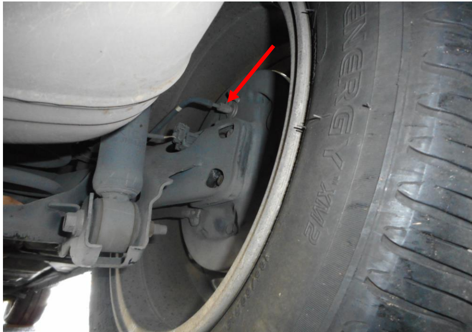
Photo 19 shows the brake hose/pipe (arrowed) at the rear right wheel of the Motor Car. No leakage of brake fluid was observed. Visual examination of the various components of the braking system like the drum brake, brake booster, brake pedal etc. had revealed all to be intact and without visible damage.
