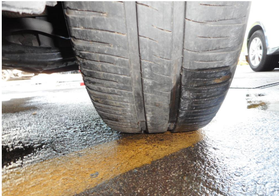
Photo 8 shows the condition of the front right tyre of the Motor Car, which was observed to be in serviceable condition with remaining tread depth of approximately 4.2mm. The tyre, which was wrapped around alloy wheel rim, was also observed to be sufficiently inflated for vehicular operation.
