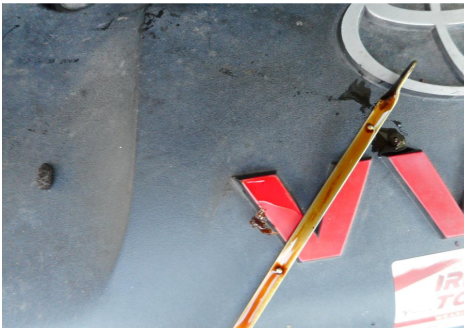
Photo 15 shows the engine oil dip stick of the Motor Car at the time of my inspection. The engine oil was observed to be of sufficient level and without any visible contamination.
