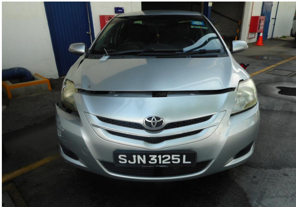
Photo 2 shows a general view of the Motor Car's front body at the time of my inspection. The Motor car was observed to have sustained damage at its front right portion. Its front bumper, front right fender, front right headlamp and right door panel was amongst the body parts and various components in the engine compartments were also damaged as a result of the accident.
