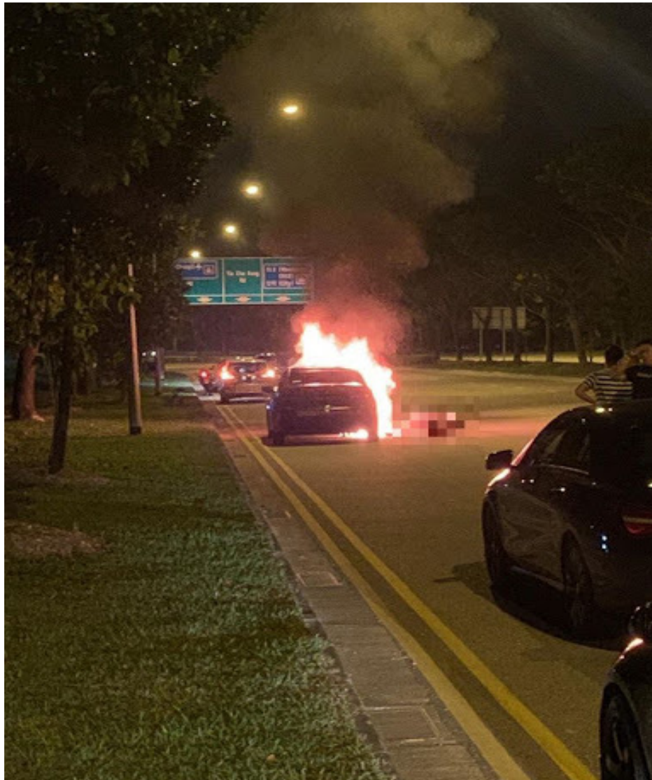
Photo 8 shows the Insured Vehicle on fire before the arrival of the SCDF (as taken from the rear portion). In general, based on the information that could be gathered from this photograph, the fire seems to have originated from the frontal portion of the Insured Vehicle.
