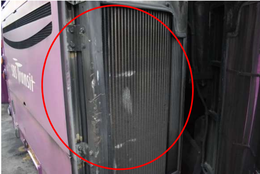
Damaged of Hydraulic oil cooler, cooling unit, (Close-up), located behind/after the radiator assembly.
