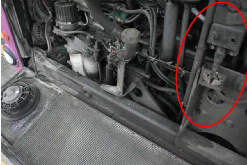
Damaged of door microswitch – adjustable RR engine DR, (close-up)
