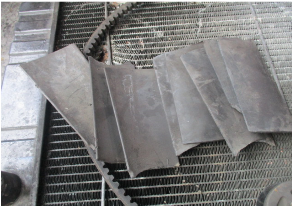
Photo 17 shows a close up view of the broken blades of the radiator fan of the Motor Bus which was replaced at GSH on 3 March 2020.
