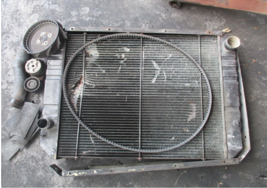
Photo 13 shows the deformed radiator, broken radiator fan blades as well as torn radiator hose of the Motor Bus which were replaced on 3 March 2020 at GSH.
