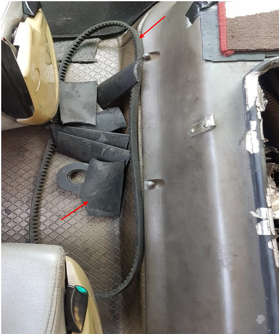
Photo 5 shows the faulty components of the Motor Bus post- incident. We observed the broken blades of the radiator fan as well as the fan belting (arrowed).
