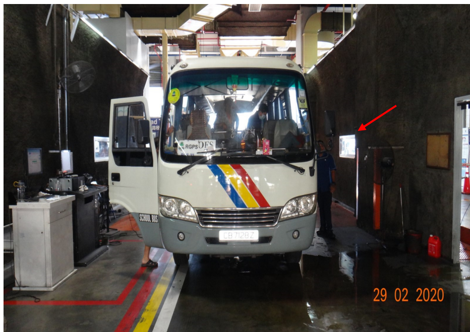
Photo 1 shows the Motor Bus post- incident. The Motor Bus passed the above-carriage check but failed the Chassis Dynamometer Smoke Test (herein referred to as “CDST”) (arrowed) which are the 2 components for the 1st stage of the inspection.
