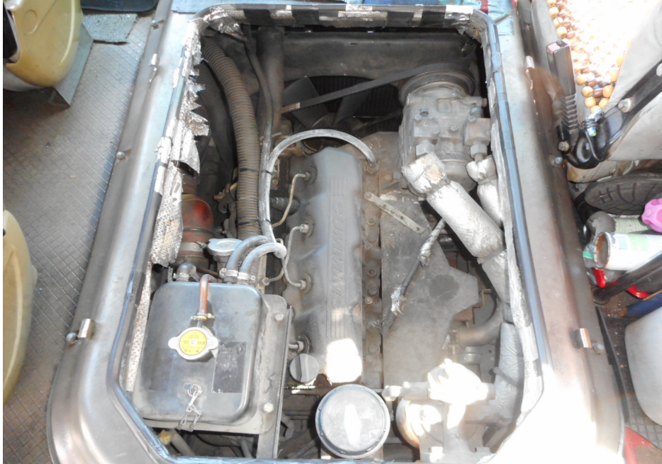
Photo 9 shows the engine compartment of the Motor Bus upon our inspection. The engine components were all in working condition. We were also informed by Mr Loo that the faulty parts of the Motor Bus which included the fan belting, radiator fan blades as well as the radiator were replaced on 3 March 2020.
