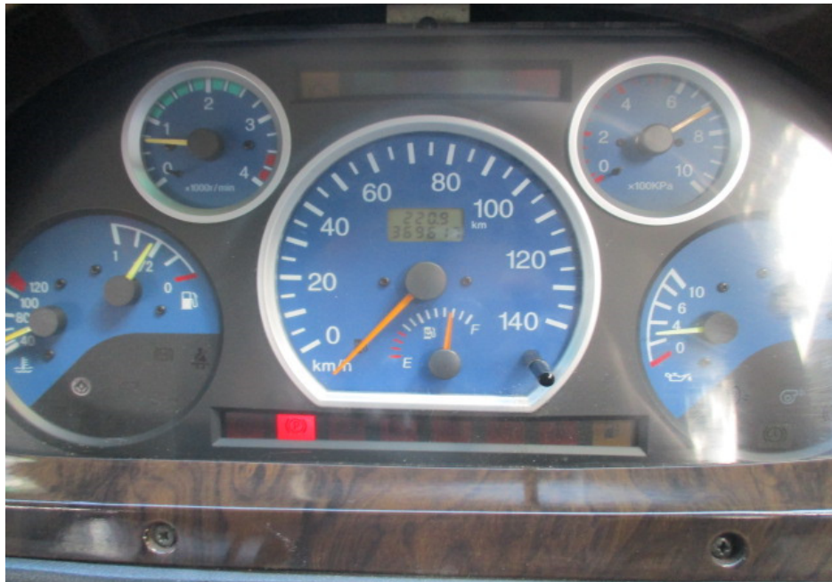
Photo 7 shows no warning lights illuminated on the instrument panel of the Motor Bus after the engine was cranked. This would suggest that there was no abnormality to the various electronic/electrical components of the Motor Bus.
