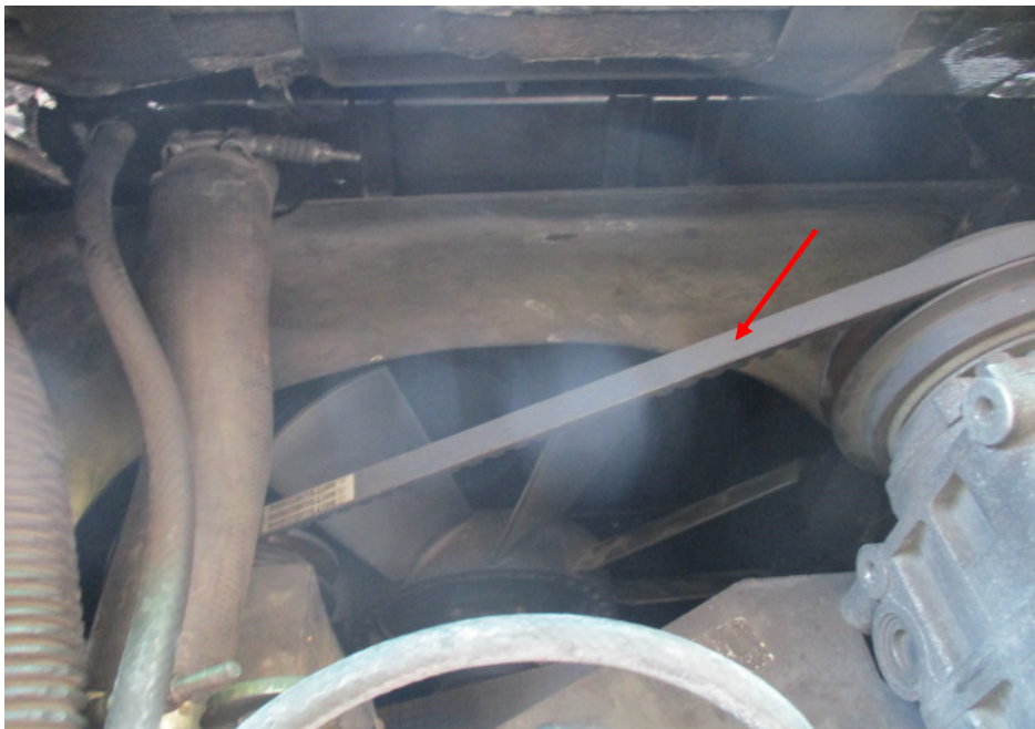
Photo 10 shows the fan belting of the Motor Bus which was replaced on 3 March 2020 (arrowed).
