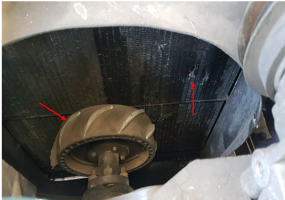
Photo 4 shows the faulty components of the Motor Bus post- incident. We observed the broken radiator fan as well as the deformed radiator (arrowed).
