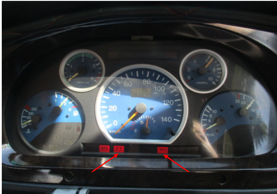
Photo 6 shows the warning lights for the various electronic/electrical components of the Motor Bus appearing on its instrument panel before the engine is cranked, in particular the 'Battery' warning light and 'Oil Pressure' warning light (arrowed).
