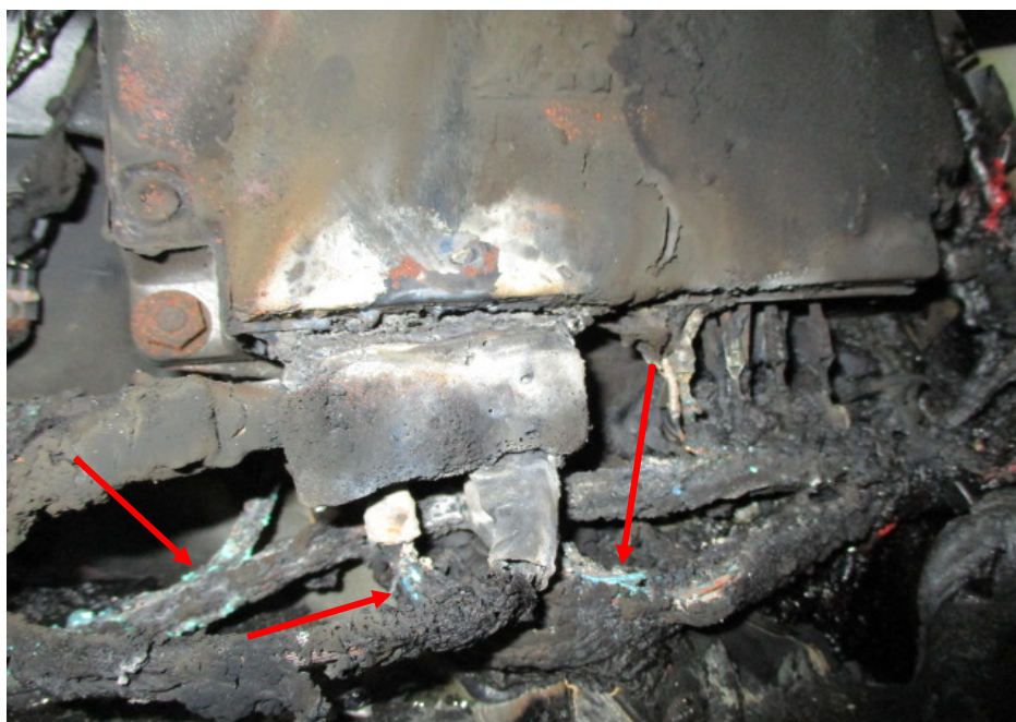
Photo 6 shows the greenish residue (arrowed) that was found on the wirings leading to the burnt connector socket. The presence of greenish residue suggests occurrence of an electrical short circuit, indicating that the cause of fire to the Insured Vehicle was due to electrical in nature.
