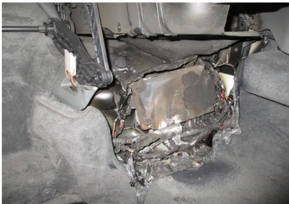
Photo 4 shows a closer view of the burnt carpet upholstery, wirings and control module unit at the right side of the rear boot compartment.
