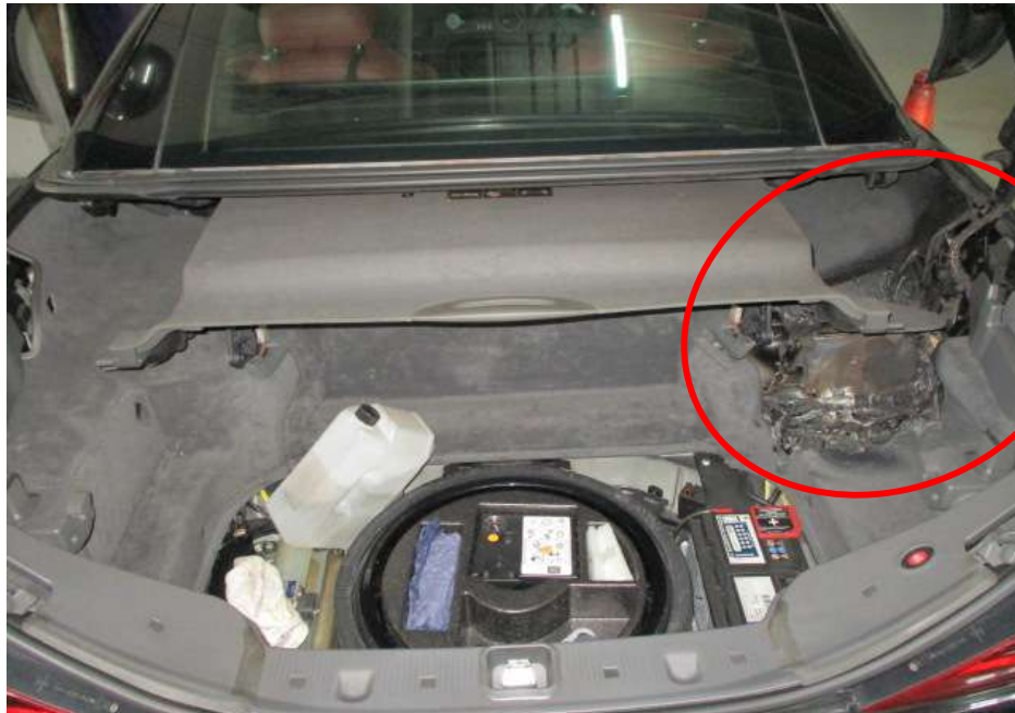
Photo 3 shows the rear boot compartment of the Insured Vehicle. Upon checking the rear boot compartment of the Insured Vehicle, I had found fire damage that was confined to the right side (circled) of the rear boot compartment. The carpet upholstery, wirings and a control module unit at the right side of the rear boot compartment were amongst the parts that were observed to be burnt.
