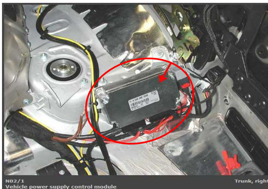
Photo 8 shows the “vehicle power supply control module” (circled), which was found to be burnt on the Insured Vehicle.
