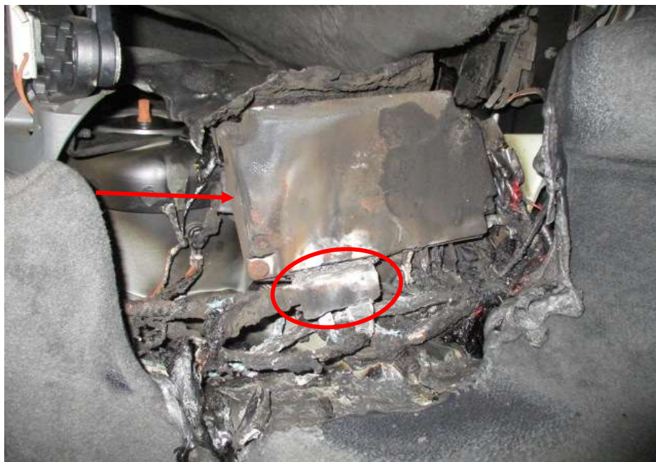
Photo 5 shows the burnt control module unit (arrowed) at the right side of the Insured Vehicle's rear boot compartment. Upon my close examination of the burnt area, I had found greenish residue on the stretch of wirings leading to the connector socket of the burnt control module unit. The connector socket (circled) was found with whitish burnt marks, which are a result of prolong exposure to heat intensity.
