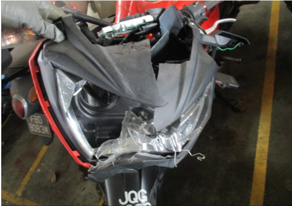
Photo 4 shows a close up view of the head cowl and headlight assembly which were amongst the body parts at the front of the Motorcycle that had sustained damage as a result of the accident.
