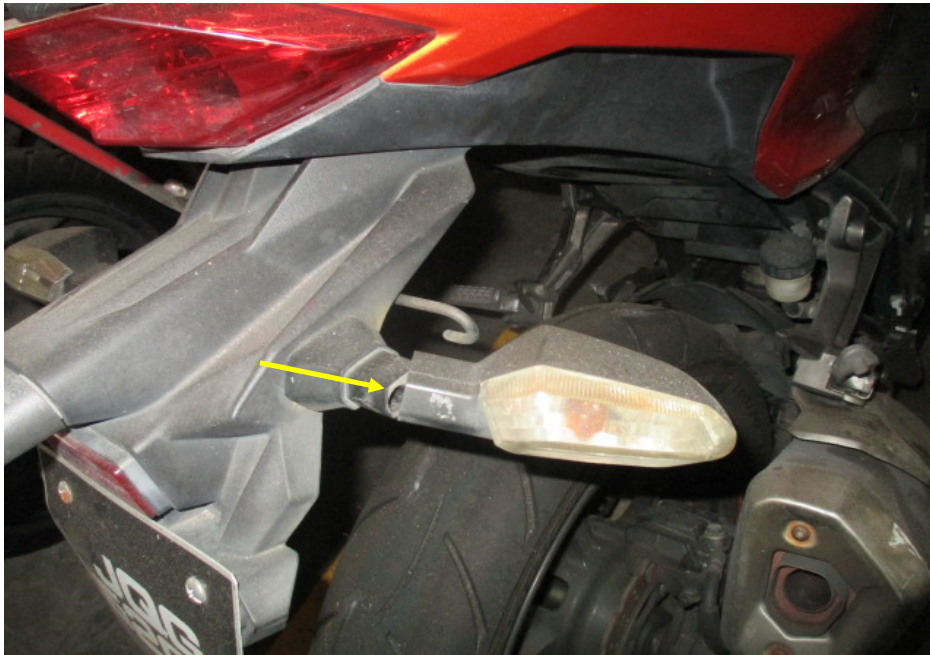
Photo 12 shows the right rear signal lamp of the Motorcycle that had sustained damage as a result of the accident (arrowed).
