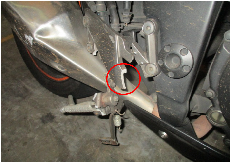
Photo 11 shows a closer view of the broken right front footrest bracket of the Motorcycle as a result of the accident (circled).
