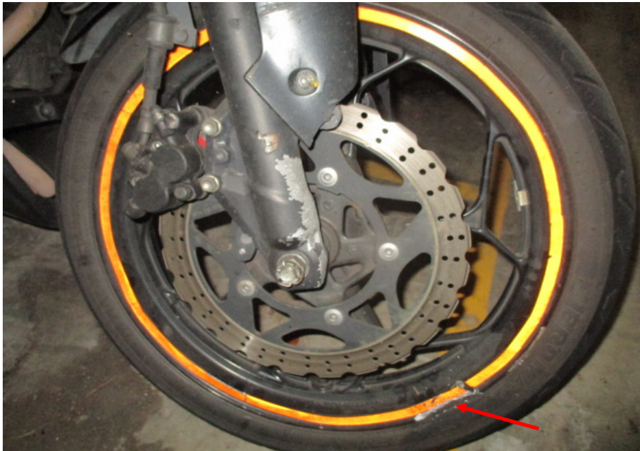
Photo 16 shows the front wheel rim of the Motorcycle which was observed to be chipped as a result of the accident (arrowed).
