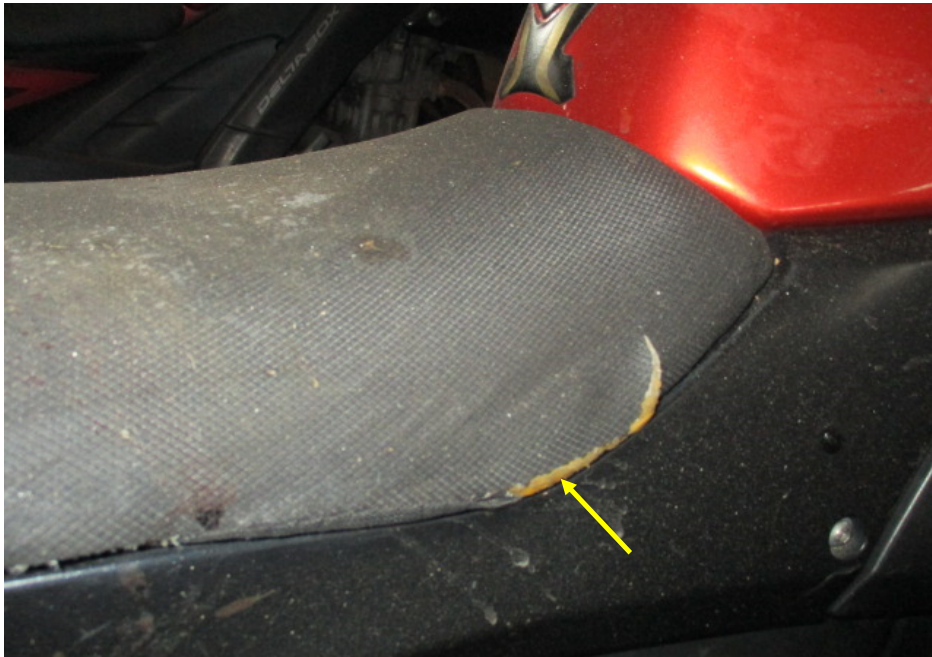
Photo 14 shows the torn seat of the Motorcycle as a result of the accident (arrowed).
