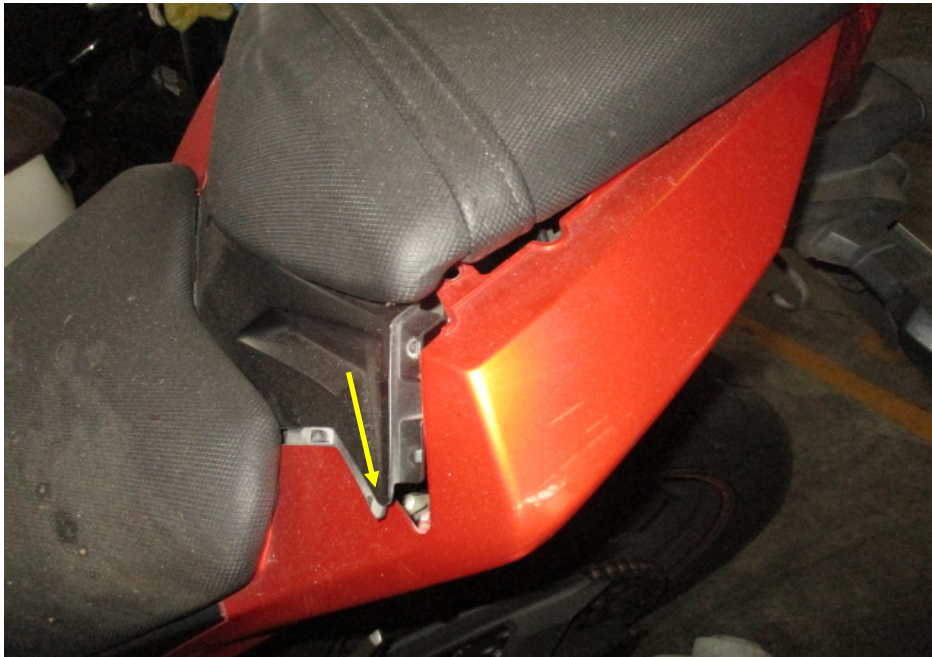
Photo 10 shows a closer view of the cracked left rear side cover of the Motorcycle as a result of the accident (arrowed).
