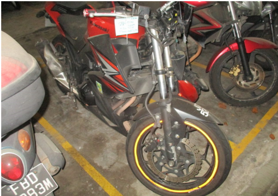
Photo 3 shows a general view of the right front body of the Motorcycle at the time of our inspection. The Motorcycle was observed to have sustained damages all around body. Amongst the body parts that were found to have been damaged include its headlight assembly, head cowl, front mudguard, right cowl, front brake lever, clutch lever, right footrest bracket and left rear side cover, amongst others.
