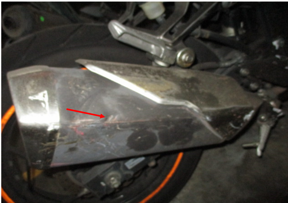
Photo 13 shows the dented exhaust muffler of the Motorcycle as a result of the accident (arrowed).
