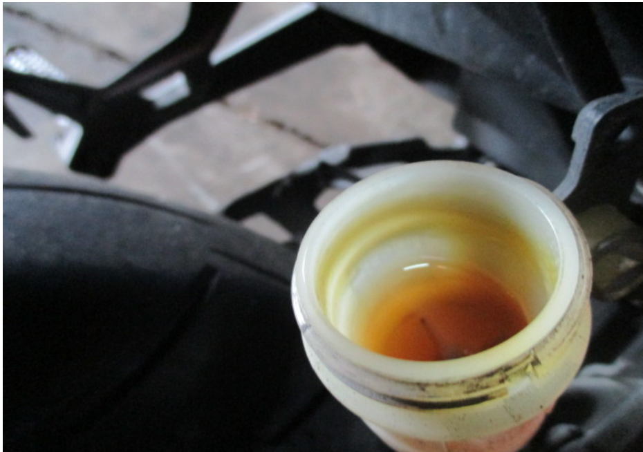
Photo 28 shows the brake fluid reservoir for the rear brake of the Motorcycle. The brake fluid was found to be without contamination and of sufficient level for operating purposes.
