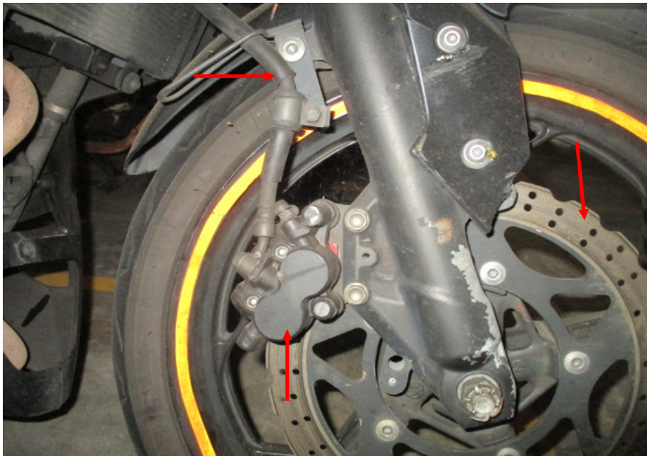
Photo 24 shows a close up view of the front brake caliper, front brake disc and front brake hose (arrowed) of the Motorcycle, which are all part of the components in the hydraulic front brake system of the Motorcycle. Our visual checks of these various components had revealed all to be intact with no visible damage. No leakage of brake fluid was also observed.
