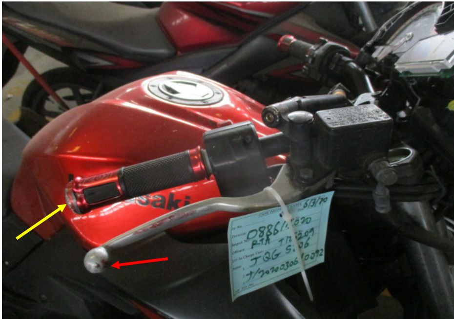
Photo 8 shows the right handlebar end and front brake lever (arrowed), which were amongst the body parts of the Motorcycle that had sustained damage as a result of the accident.
