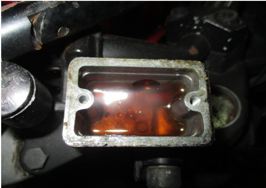
Photo 25 shows the brake fluid reservoir for the front brake of the Motorcycle. The brake fluid was found to be without contamination and of sufficient level for operating purposes.
