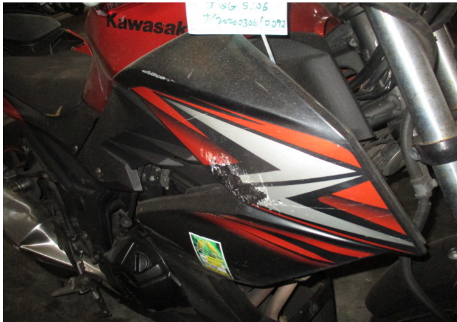
Photo 6 shows a closer view of the right cowling of the Motorcycle which had sustained damages of grazing nature as a result of the accident.
