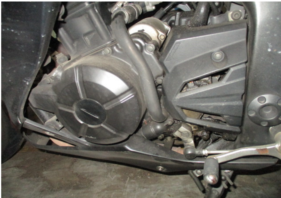
Photo 18 shows the left side of the engine of the Motorcycle at the time of our inspection. The various engine related parts and components were found to be intact with no visible damage. There was also no sign(s) or indication(s) of fluid leak observed around the left engine area of the Motorcycle.
