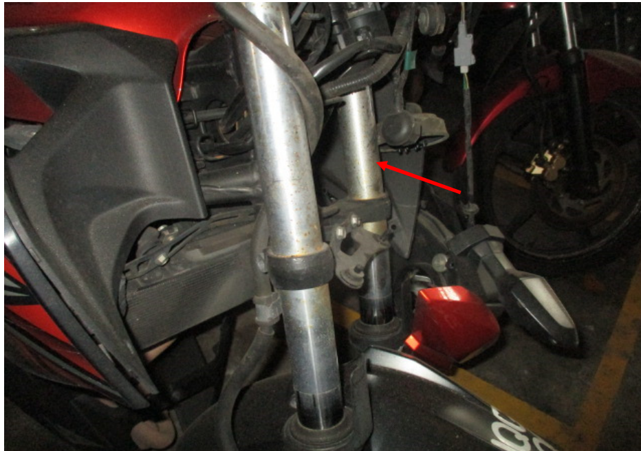
Photo 22 shows the front forks of the Motorcycle. The left front fork was found to be bent inwards as a result of the accident (arrowed). We were hence not able to conduct any tests on the steering system of the Motorcycle.
