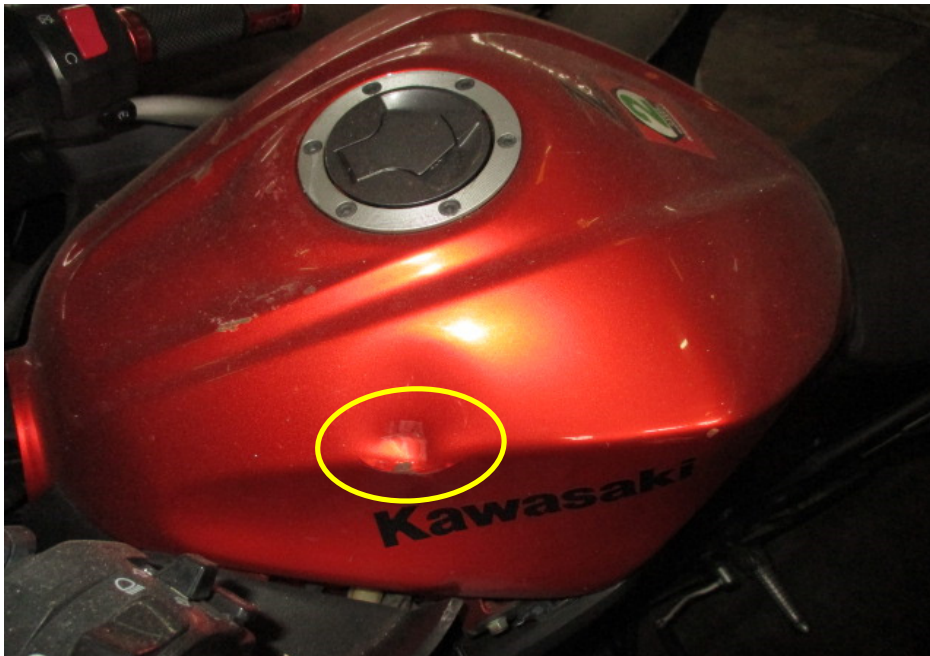
Photo 9 shows a closer view of the dented petrol tank (circled) which was amongst the body parts of the Motorcycle that had sustained damage as a result of the accident.
