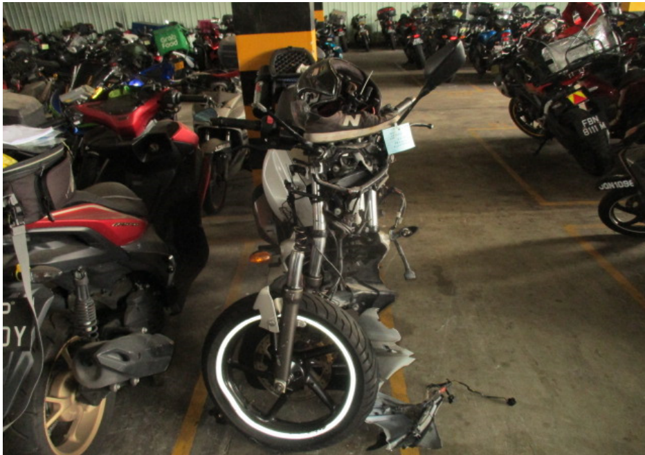
Photo 3 shows a general view of the frontal portion of the Motorcycle at the time of our inspection. The Motorcycle had sustained damages all around. Body parts that were found to have been damaged include its headlight assembly, front fork assembly, front mudguard, petrol tank, side mirrors, front brake lever, clutch lever, handlebar ends, gear shift pedal, exhaust header and right rear signal lamp, amongst others.
