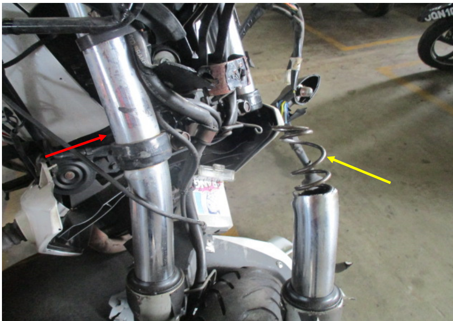
Photo 19 shows the front forks of the Motorcycle. The front right fork was observed to be bent inwards (red arrow) and the left front fork was observed to be dislodged (yellow arrow) as a result of the accident. We were hence not able to conduct any tests on the steering system of the Motorcycle.
