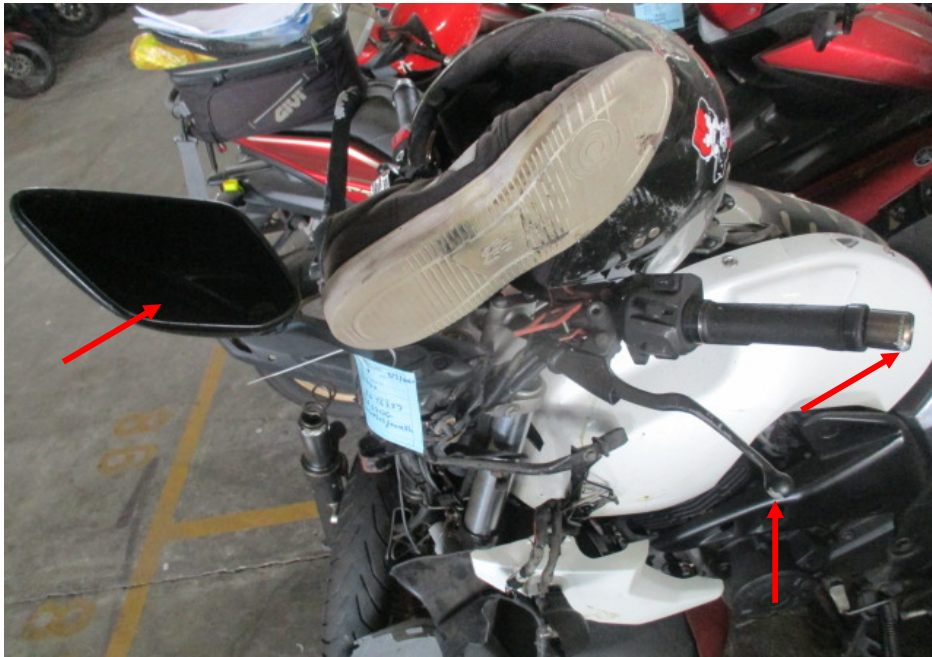
Photo 5 shows a closer view of the clutch lever, left side mirror and left handlebar end (arrowed) of the Motorcycle. These parts were amongst the body parts of the Motorcycle which were damaged as a result of the accident.
