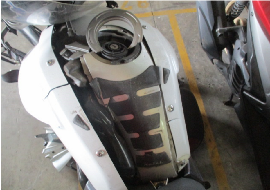
Photo 7 shows a closer view of the deformed petrol tank which was amongst the body parts of the Motorcycle that had sustained damages as a result of the accident.
