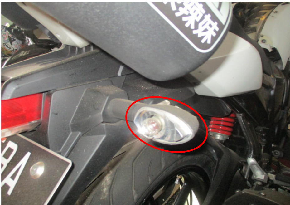
Photo 8 shows a closer view of the cracked right rear signal lamp which was amongst the body parts at the rear body of the Motorcycle that had sustained damages as a result of the accident (circled).
