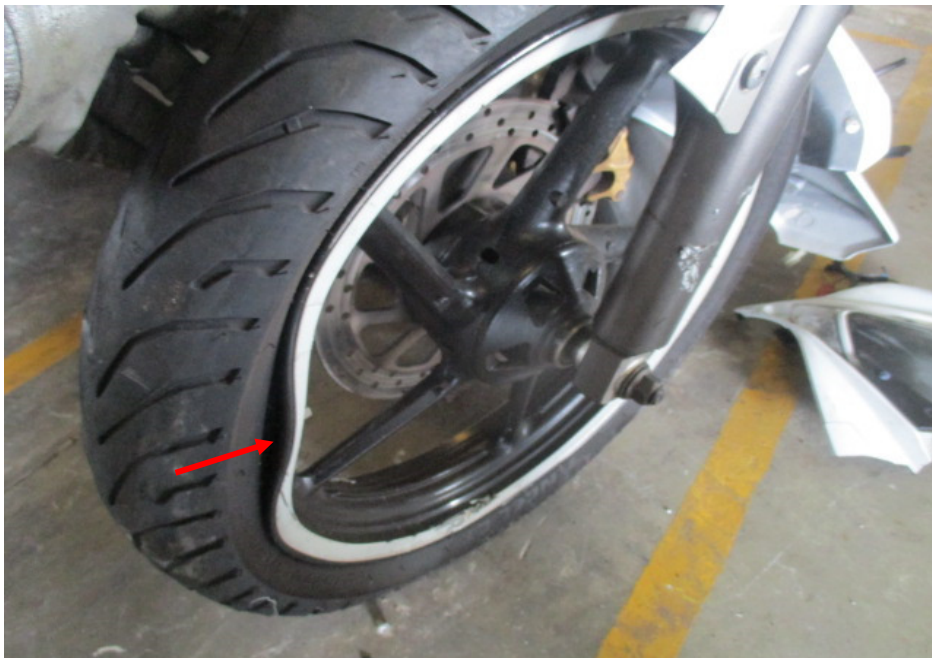
Photo 12 shows the bent front wheel rim of the Motorcycle as a result of the accident at the time of our inspection (arrowed).
