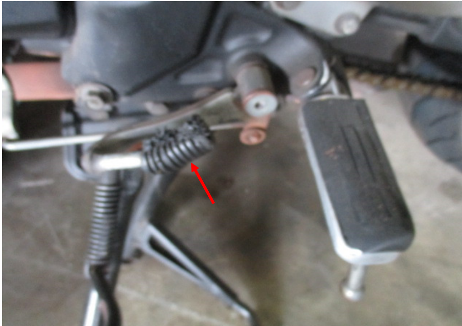
Photo 11 shows the bent gear shift pedal of the Motorcycle as a result of the accident (arrowed).
