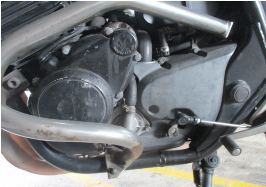
Photo 8 shows the left side of the engine of the Motorcycle at the time of our inspection. The various engine related parts and components were found to be intact with no visible damage. There was also no sign(s) or indication(s) of fluid leak observed around the left engine area of the Motorcycle.
