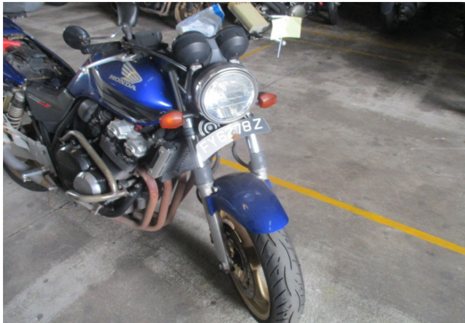
Photo 15 shows the front wheel of the Motorcycle turned towards its full right. Turning the Motorcycle's handle bar towards the left and right did not produce any abnormal free play and/or resistance. This would indicate that the steering system of the Motorcycle was in serviceable condition at the time of our inspection.
