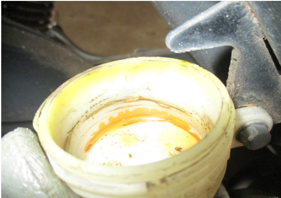
Photo 22 shows the brake fluid reservoir for the rear brake of the Motorcycle. The brake fluid was observed to be of insufficient level for operational purposes.
