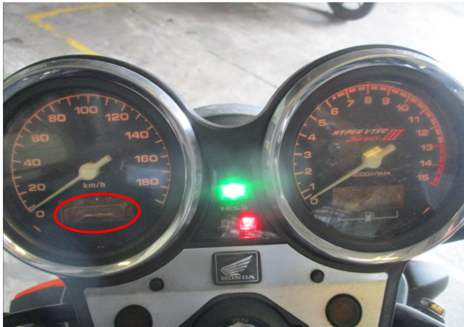
Photo 1 shows the mileage of the Motorcycle which could not be recorded at the time of our inspection due to the damage sustained to the speedometer gauge (circled).
