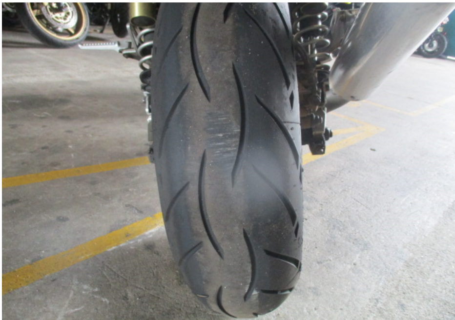
Photo 7 shows the condition of the Motorcycle's rear tyre. The rear tyre was observed to be in serviceable condition with remaining tread depth of approximately 4mm. The tyre was also observed to be sufficiently inflated for vehicular operation. We did not observe any tear, burst mark(s) and/or punctured hole(s) on the sidewalls as well as across the tread of the rear tyre.
