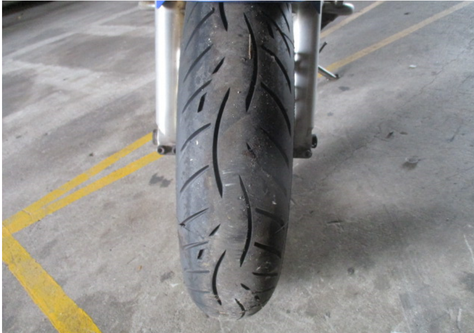
Photo 6 shows the condition of the Motorcycle's front tyre. The front tyre was observed to be in serviceable condition with remaining tread depth of approximately 4mm. There was no tear, burst mark(s) and/or punctured hole(s) on the sidewalls as well as across the tread of the front tyre.
