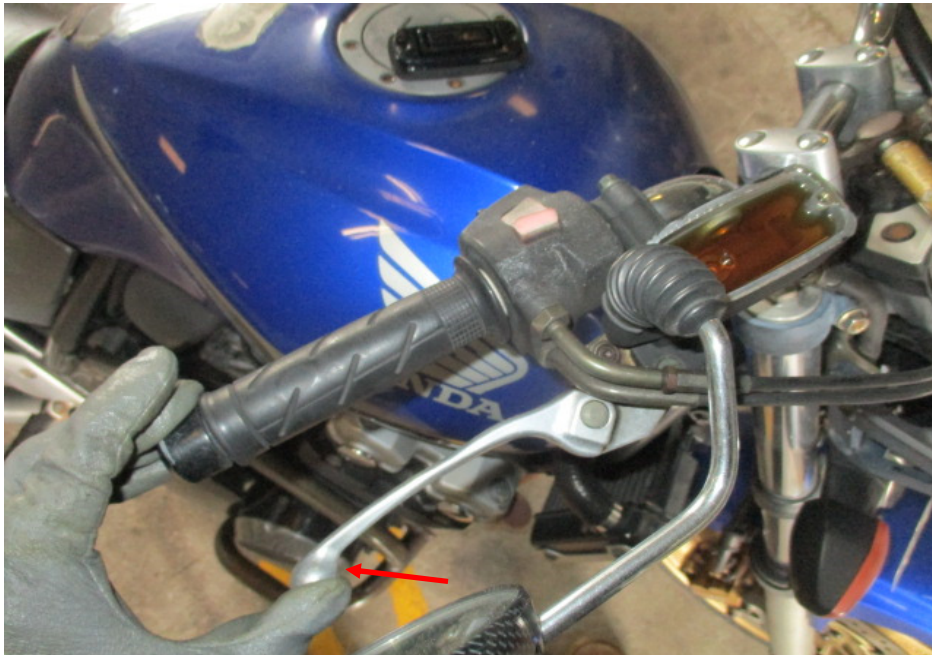
Photo 20 shows the front brake lever being depressed. There was some resistance felt (spongy like feel) upon pressing the front brake lever (arrowed). This would indicate that there is no leakage of pressure/vacuum in the brake system.
