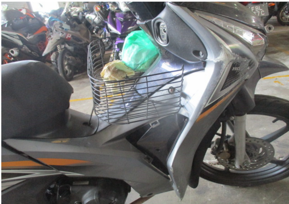
Photo 8 shows a closer view of the right cowling which was amongst the body parts of the Motorcycle that had sustained damages as a result of the accident.
