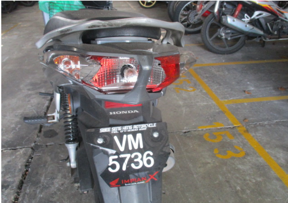
Photo 11 shows the broken tail light assembly and cracked rear number plate of the Motorcycle as a result of the accident.
