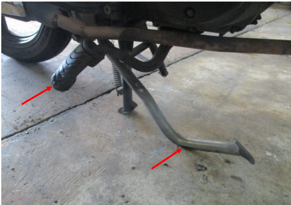
Photo 10 shows the bent brake foot pedal and right front footrest (arrowed), which were amongst the body parts of the Motorcycle that had sustained damage as a result of the accident.
