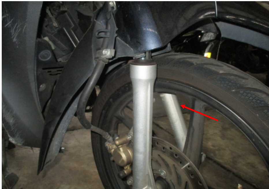
Photo 19 shows the front forks of the Motorcycle. The front left fork (arrowed) was observed to be bent as a result of the accident. We were hence not able to conduct any tests on the steering system of the Motorcycle.
