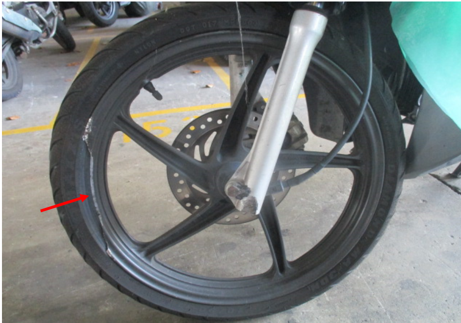
Photo 12 shows the broken front wheel rim (arrowed) of the Motorcycle as a result of the accident at the time of our inspection.
