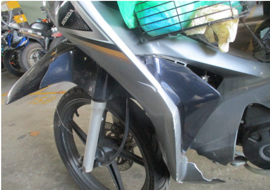
Photo 9 shows a closer view of the left cowling which was amongst the body parts of the Motorcycle that had sustained damages as a result of the accident.
