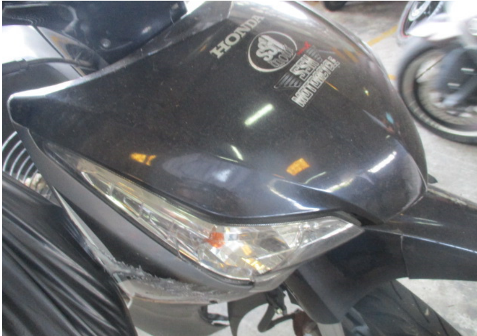
Photo 7 shows a closer view of the front cowling which was amongst the body parts at the front body of the Motorcycle that had sustained damages as a result of the accident.
