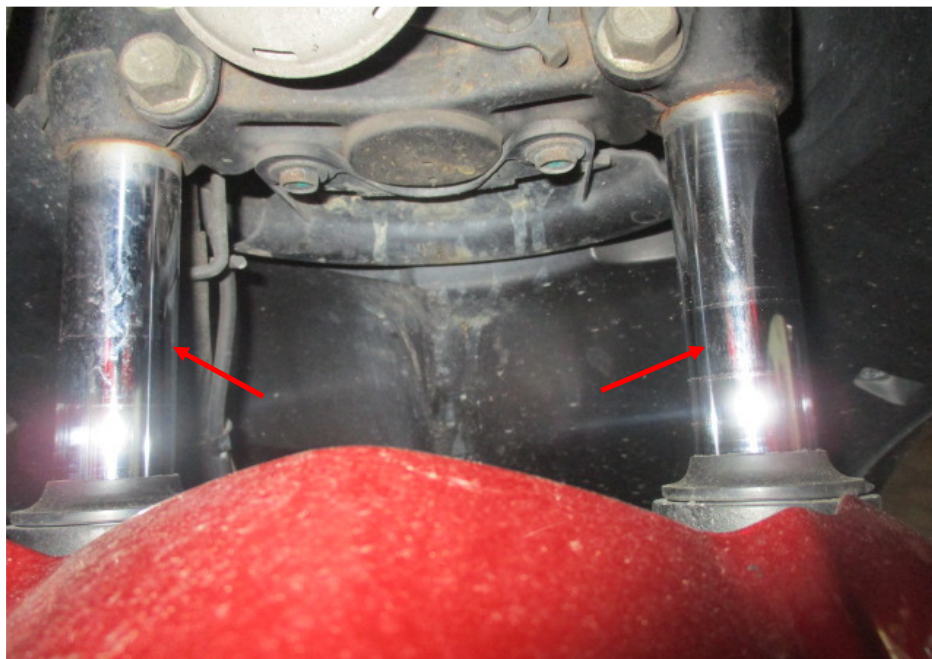
Photo 21 shows the front forks (arrowed) of the Motorcycle. The front forks and fork brackets of the Motorcycle were both found to be intact and undamaged. Turning the Motorcycle's handle bar towards the left and right did not produce any abnormal free play and/or resistance. The steering system of the Motorcycle was in serviceable condition at the time of our inspection.
