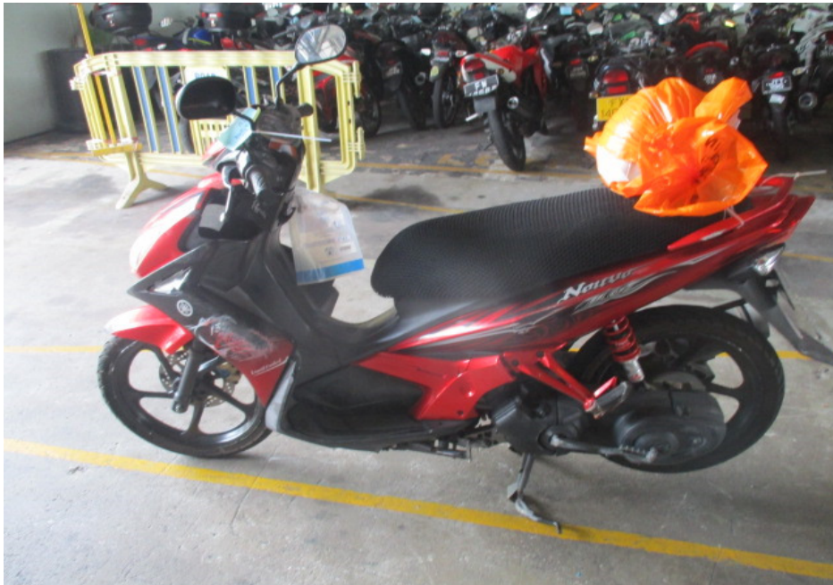
Photo 3 shows a general view of the left body of the Motorcycle at the time of our inspection. The body parts that were found to have been damaged include its front cowling, front mudguard, rear brake lever, left side mirror, left handlebar grip, left side cowling, left side cover, left rear side cover, left pillion footpeg and left rear signal lamp, amongst others as a result of the accident.
