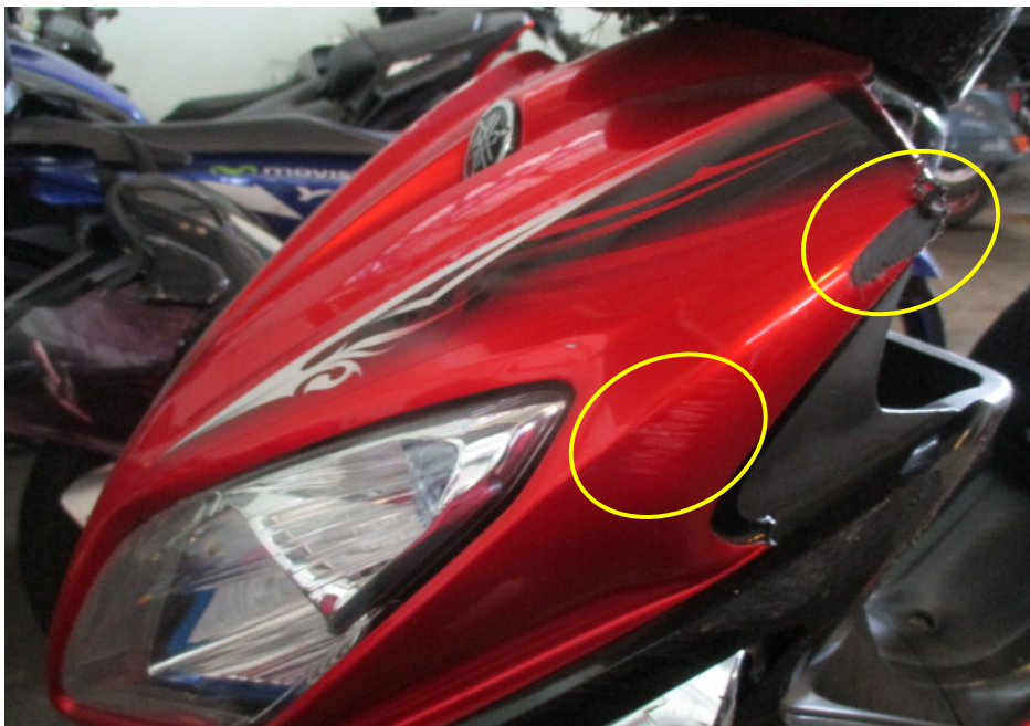
Photo 4 shows a closer view of the damaged front cowling of the Motorcycle at the time of our inspection (circled).
