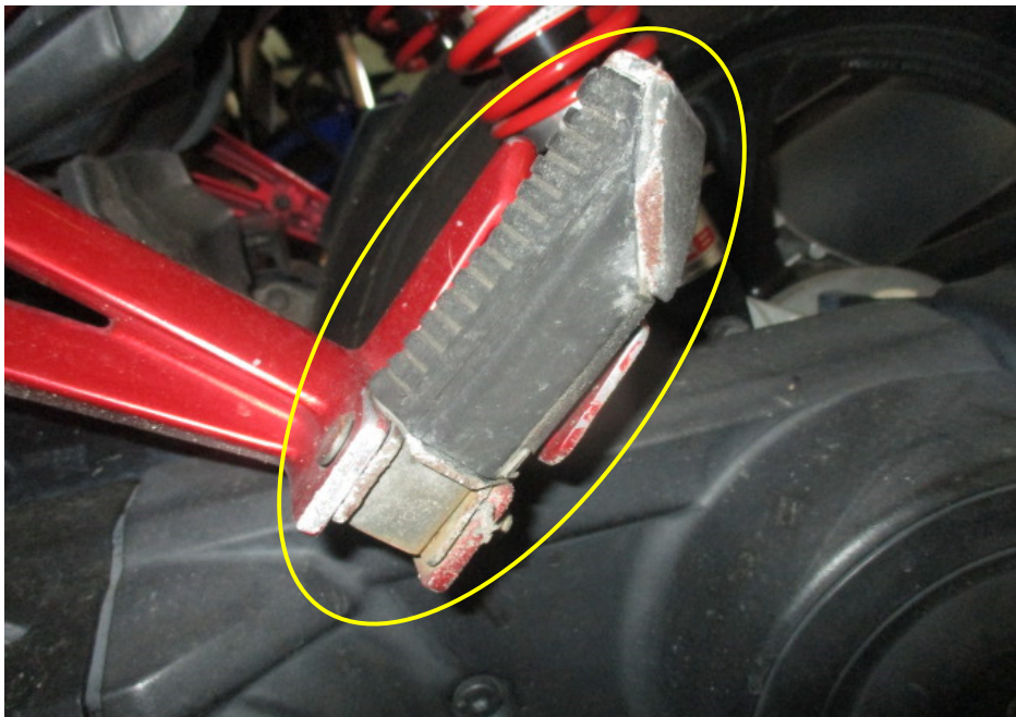
Photo 12 shows a closer view of the damaged left pillion footpeg of the Motorcycle at the time of our inspection (circled).
