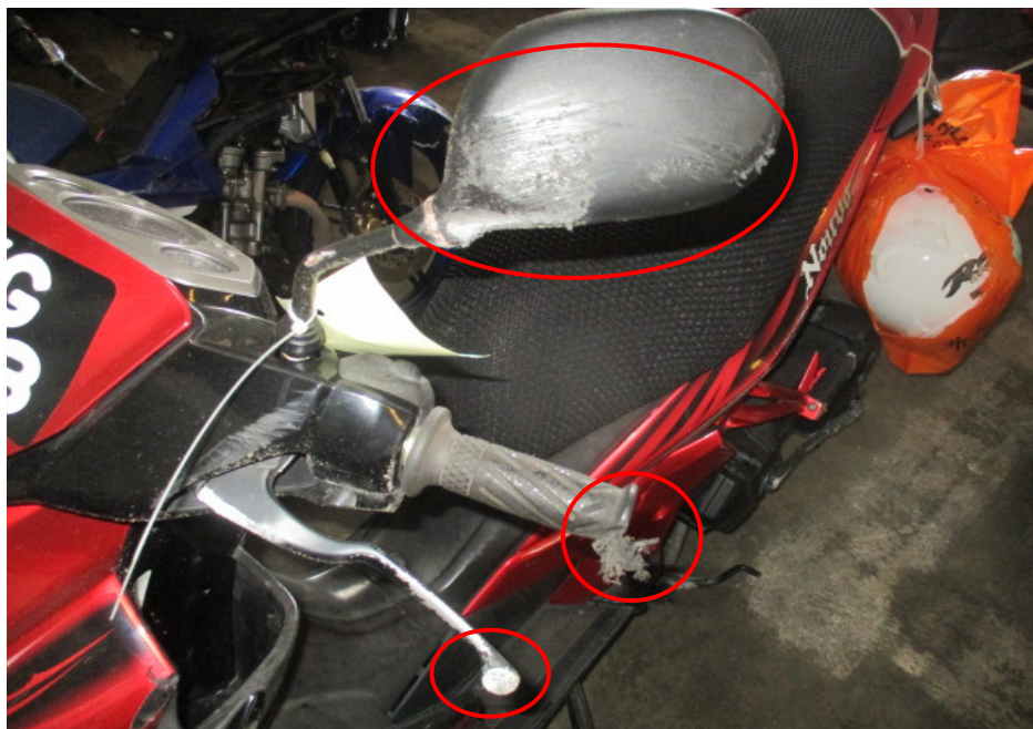
Photo 6 shows a closer view of the left side mirror, left handlebar grip and rear brake lever of the Motorcycle which were observed to be damaged due to the accident (circled).
