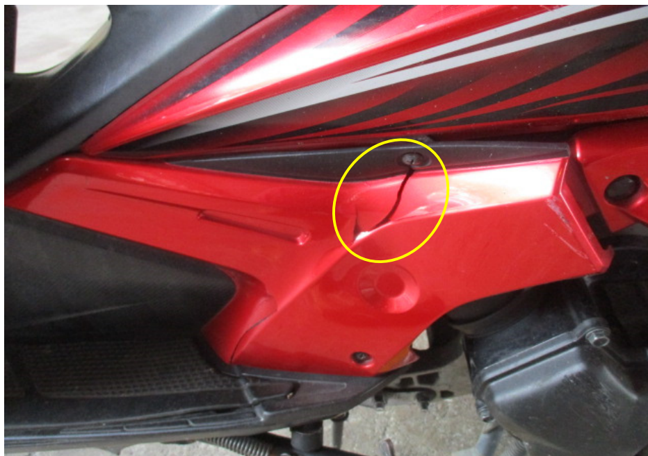
Photo 9 shows a close-up view of the cracked left side cover of the Motorcycle at the time of our inspection (circled).
