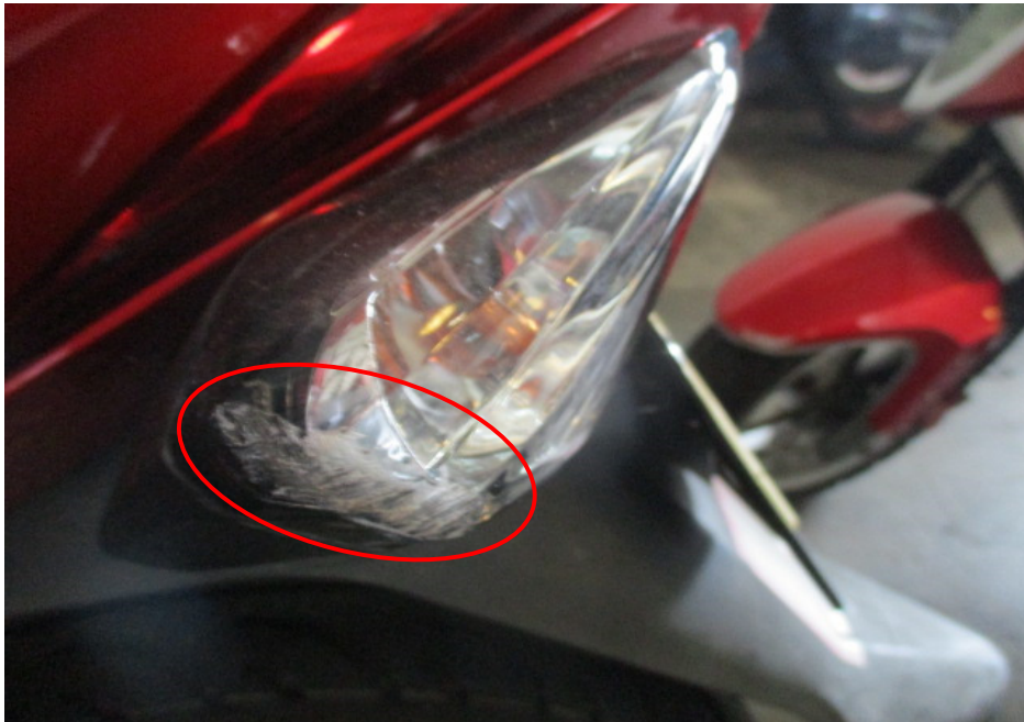
Photo 11 shows a closer view of the grazed left rear signal lamp of the Motorcycle at the time of our inspection (circled).
