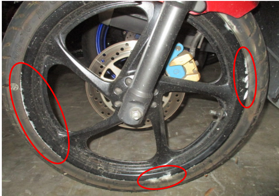
Photo 15 shows the left front wheel rim and tyre of the Motorcycle at the time of our inspection. The front tyre was observed to be in serviceable condition and sufficiently inflated for vehicular operation. Some relatively minor marks of grazing nature were observed on the edges of the front wheel rim (circled), at the left side of the Motorcycle.
