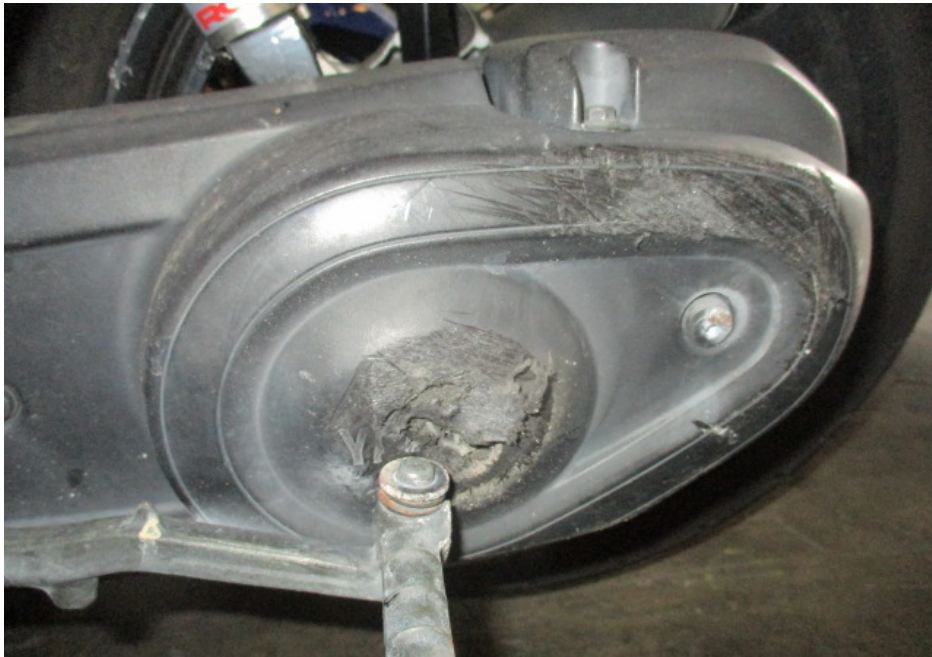
Photo 18 shows the drive train of the Motorcycle which was found to be intact without any misalignment. However the drive train cover had sustained damages of grazing nature as a result of the accident.
