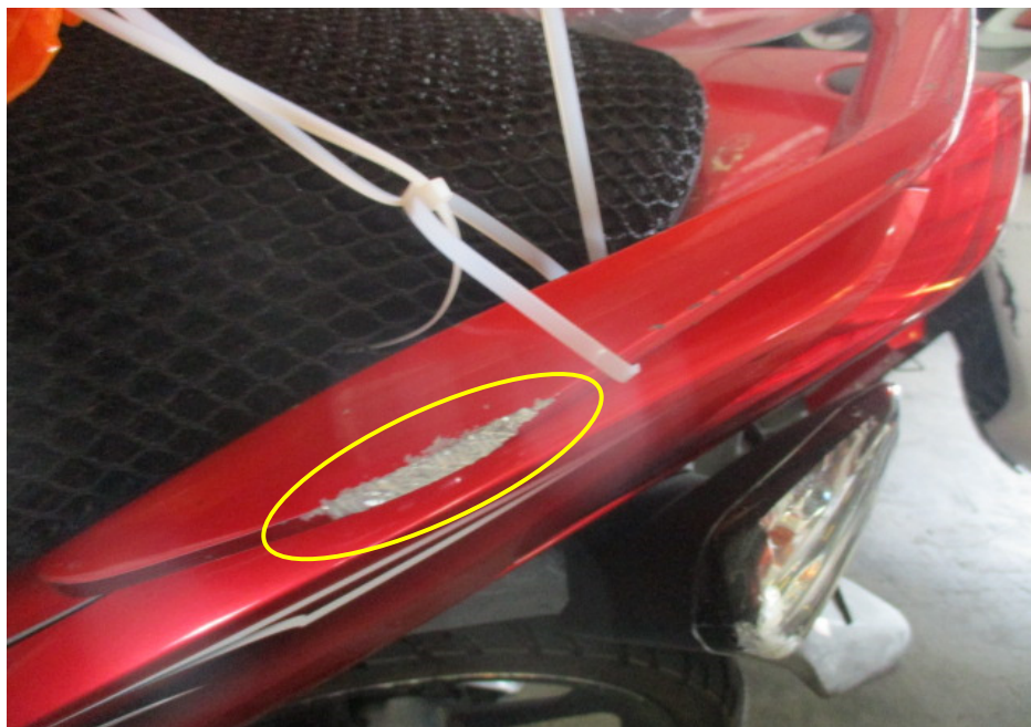
Photo 13 shows a closer view of the left grab bar of the Motorcycle which had sustained damage due to the accident (circled).
