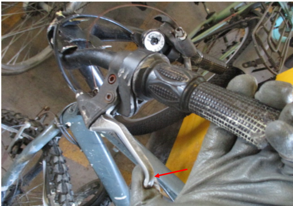
Photo 17 shows the jammed front brake lever as a result of the accident (arrowed). Hence a static brake test could not be conducted on the Bicycle's front braking system.
