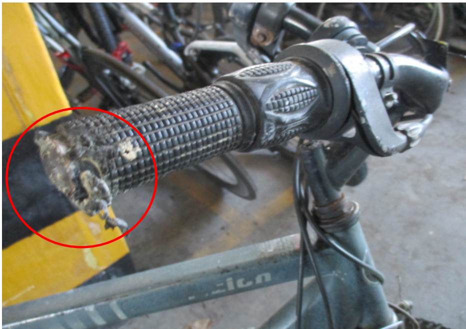
Photo 6 shows the damaged right handlebar end of the Bicycle at the time of our inspection (circled).
