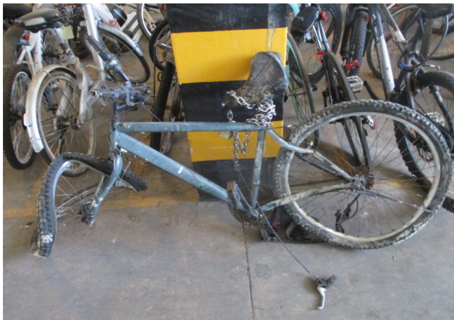
Photo 3 shows the left portion of the Bicycle at time of our inspection. The Bicycle had sustained damages all around. The Bicycle had sustained damages all around. The body parts that were found to have been damaged include its front forks, handlebar, frame and braking components, amongst others as a result of the accident.
