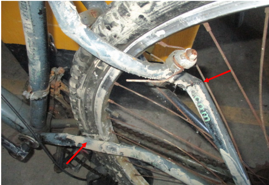
Photo 9 shows a close-up view of the bent rear frame which was observed to be pushed against the rear tyre of the Bicycle as a result of the accident (arrowed).
