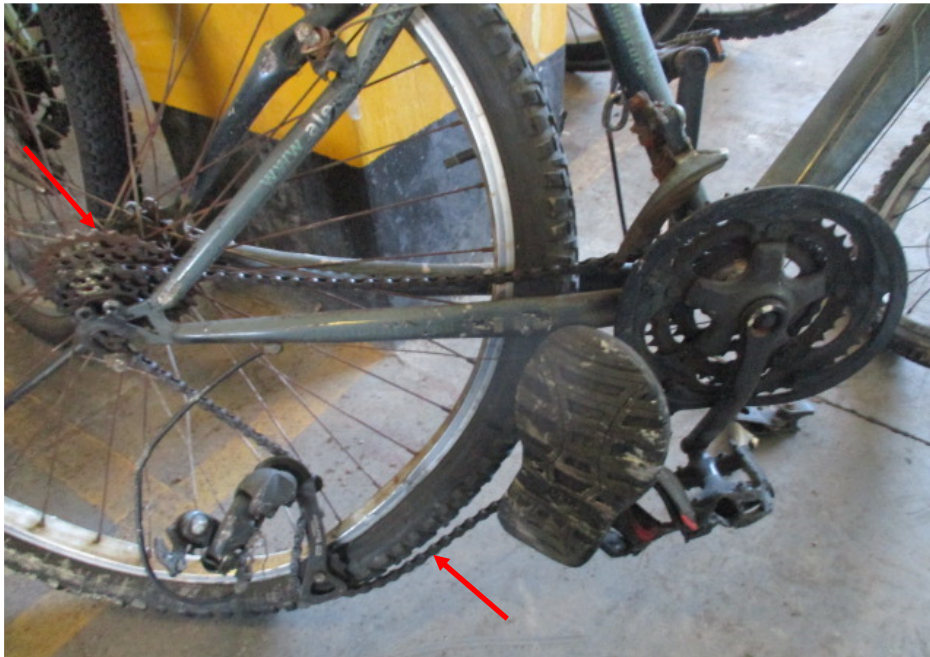
Photo 13 shows the general view of the gear train of the Bicycle, which was observed to have sustained severe damages as a result of the accident (arrowed).
