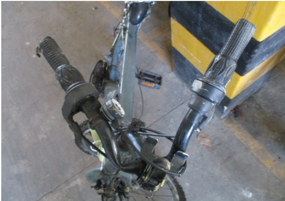
Photo 5 shows the deformed handlebar of the Bicycle at the time of our inspection.
