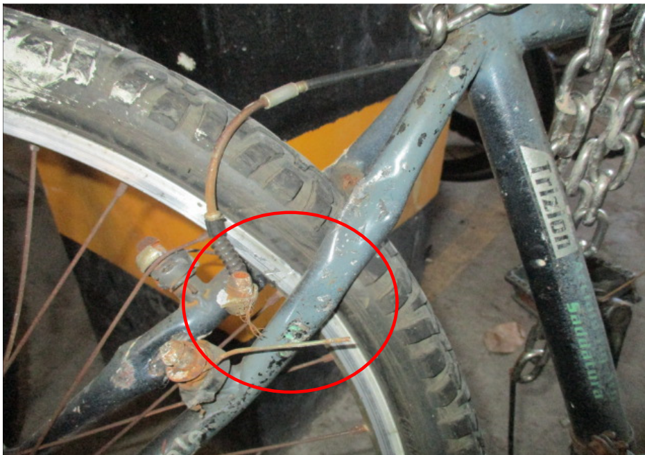
Photo 19 shows the rear connecting cable which had been disconnected from the rear hand brake lever as a result of the accident (circled).
