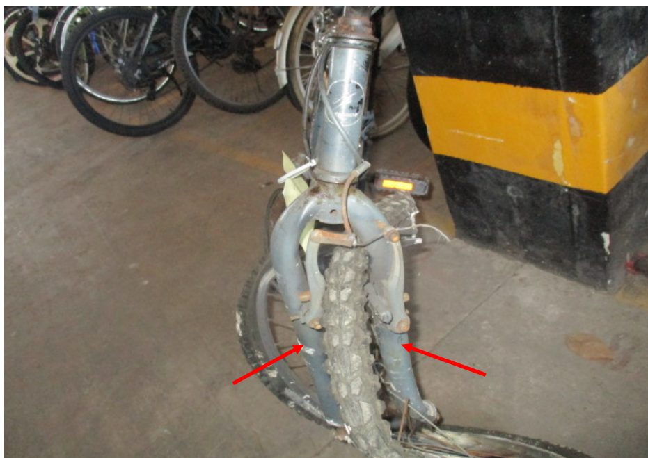
Photo 15 shows the front fork (arrowed) of the Bicycle. The front fork and fork bracket of the Bicycle were both found to be bent as a result of the accident, hence causing the whole steering system to be out of alignment and rendering the Bicycle immobile for any static or operational tests.
