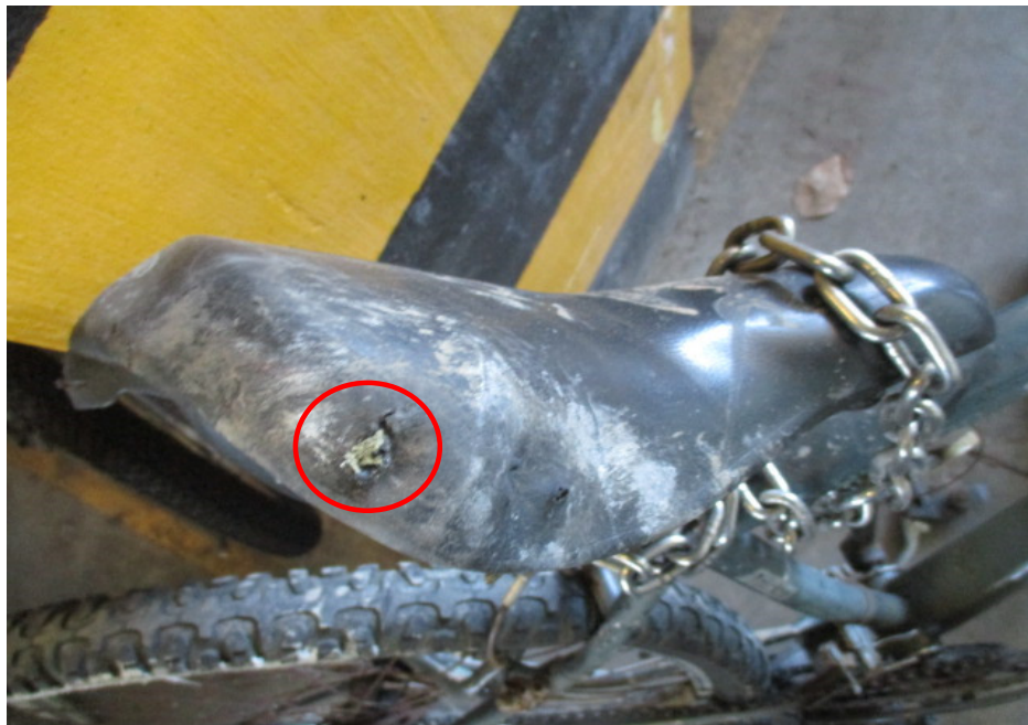
Photo 7 shows a close-up view of the torn seat of the Bicycle due to the accident.
