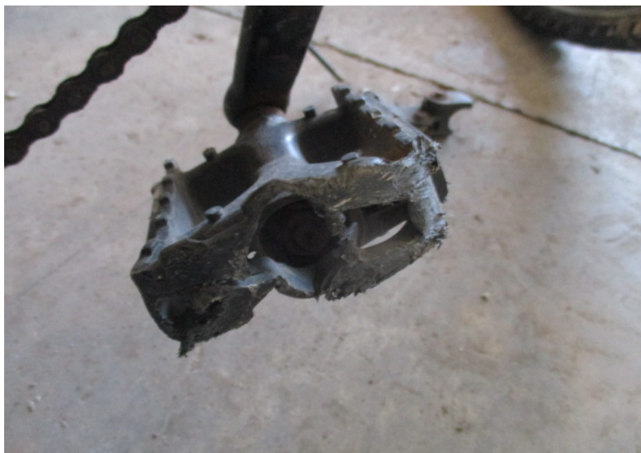
Photo 8 shows the right pedal of the Bicycle which sustained damage as a result of the accident.
