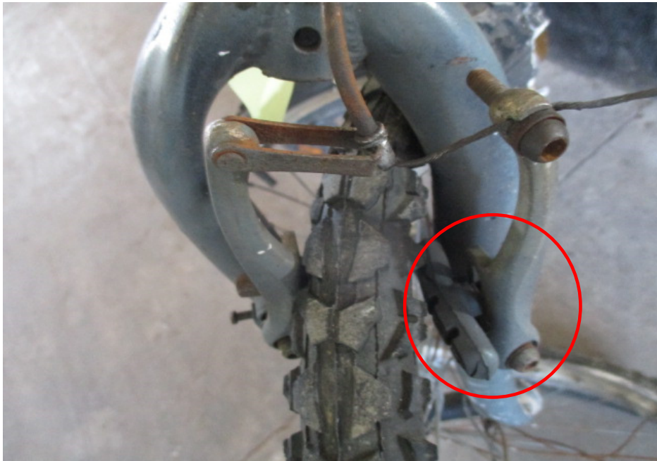
Photo 16 shows the front brake clamp assembly of the Bicycle which was intact however it was observed to be misaligned (circled).
