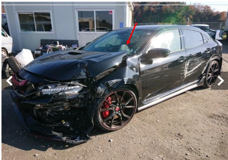
Photo 1 shows the front left body of the Motor Car prior to any repairs being carried out (photograph provided to me). The Motor Car was observed to have sustained damages along its left side. The body parts observed to be damaged had included its front bumper, front left headlamp, front left fender, front bonnet and front left door amongst others. The front left passenger airbag was also observed to be deployed (arrowed).
