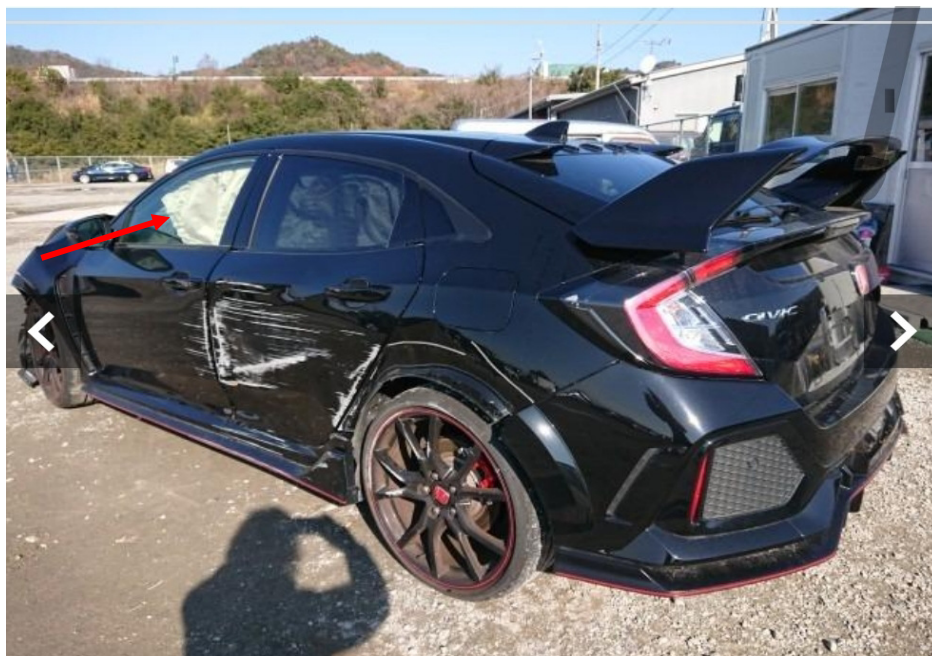
Photo 2 shows the rear left body of the Motor Car prior to any repairs being carried out (photograph provided to me). The Motor Car was observed to have sustained damages along its left side. The rear left door and rear left fender were amongst the body parts that were observed to be damaged. The left side roof airbag was also observed to be deployed (arrowed).
