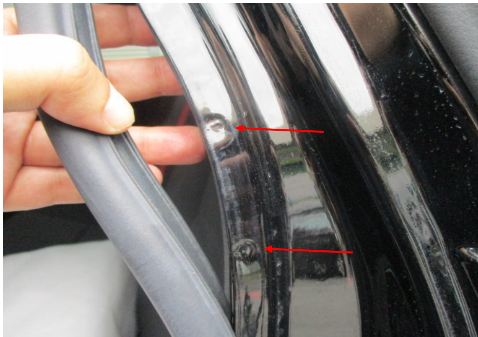
Photo 20 shows the left "C" pillar of the Motor Car. I did not find any weld marks other than original spot weld marks (arrowed) on the non-detachable body panels of the Motor Car, indicating that there was no re-welding works carried out; and that the non-detachable body panels of the Motor Car were originally fitted.
