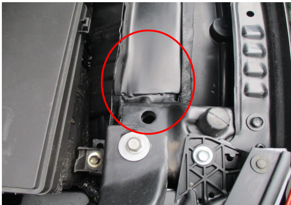
Photo 9 shows the front left fender inner panel of the Motor Car. Signs of repair was observed (circled). Generally, the repair/restoration works carried out to the damaged area of the Motor Car (refer photograph 1 to 3 above) were reasonably adequate and in order.
