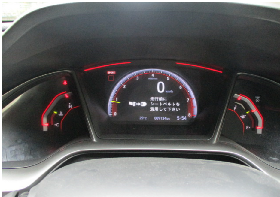
Photo 12 shows the respective warning lights no longer illuminated after the engine was started, indicating that there was no fault detected to the ABS, SRS, VSA and EPS systems of the Motor Car during the self-test. These electronic systems were hence in working condition at the time of my inspection.
