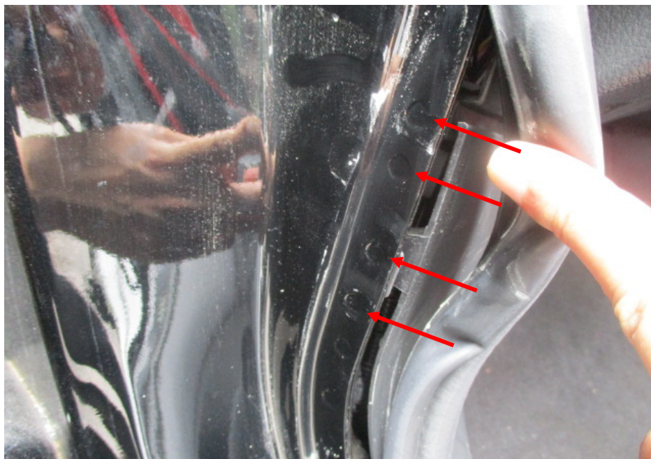
Photo 21 shows the left "A" pillar of the Motor Car. I did not find any weld marks other than original spot weld marks (arrowed) on the non-detachable body panels of the Motor Car, indicating that there was no re-welding works carried out; and that the non-detachable body panels of the Motor Car were originally fitted.
