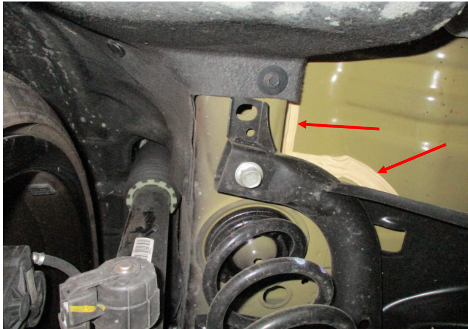
Photo 19 shows the chassis/structure body at the underside rear left of the Motor Car. The original factory sealant (arrowed) at the joints along the chassis/structural body was untouched, indicating no work was done on the chassis/structural body of the Motor Car and that the chassis/structural body was originally fitted.
