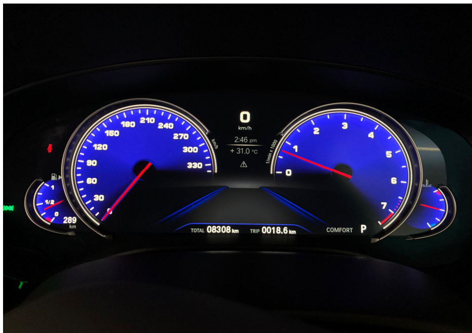
Photo 7 shows the respective warning lights no longer illuminated after the engine was started, indicating that there was no fault detected to the ABS, SRS, IAS, TPM and DSC systems of the Motor Car during the self-test. These electronic systems were hence in working condition at the time of my inspection.
