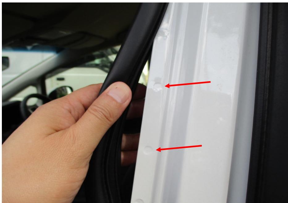
Photo 16 shows the left "B" Pillar of the Motor Car. I did not find any weld marks other than original spot weld marks (arrowed) on the non-detachable body panels of the Motor Car, indicating that there was no re-welding works carried out; and that the non-detachable body panels of the Motor Car were originally fitted.
