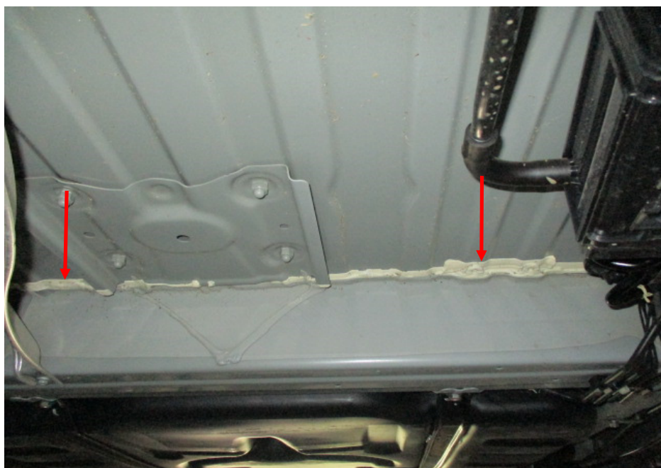
Photo 14 shows the floor board at the underside centre of the Motor Car. The original factory sealant (arrowed) at the joints of the non-detachable body panels was all untouched indicating no replacement of the non-detachable body panels was carried out.
