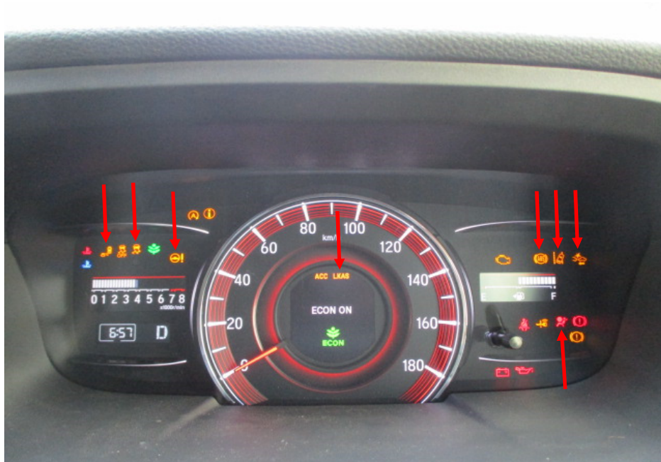
Photo 6 shows the warning lights for the various electronic safety features appearing on the instrument panel of the Motor Car during its self-test when the engine is cranked, in particular the ABS, SRS, EPS, VSA, BSI, LKAS, RDM, CMBS lights (arrowed).
