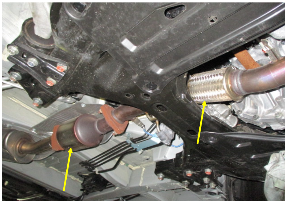
Photo 12 shows the Motor Car's catalytic converters (arrowed). My examination of the Motor Car's exhaust system revealed no sign(s) or indication(s) of any cut or weld marks along its exhaust pipes and on its rear muffler.
