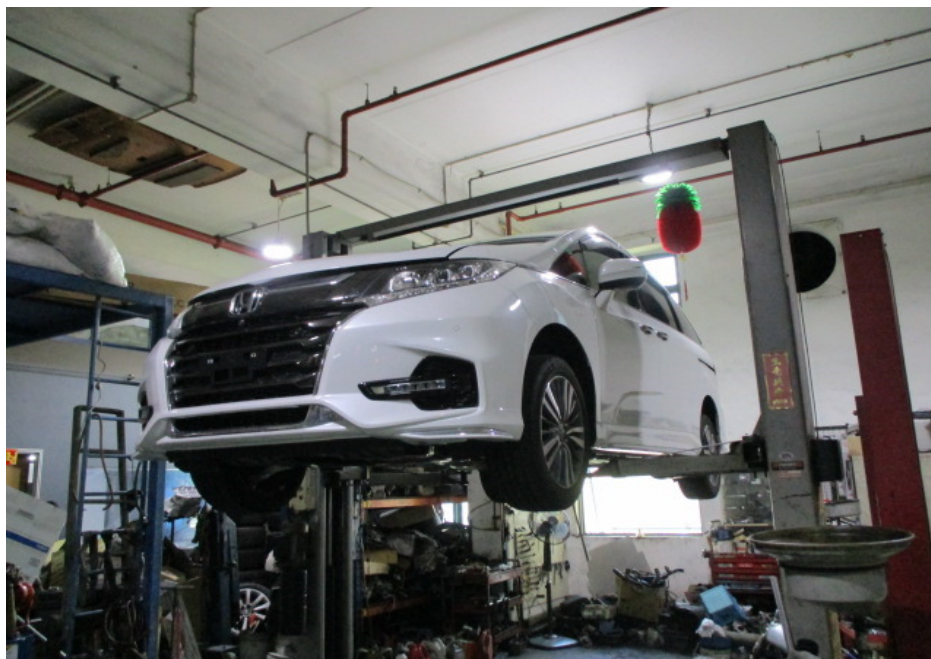
Photo 8 shows the Motor Car hoisted up for checks on its undercarriage. There was no sign(s) or indication(s) of fluid leakage and/or fluid stain(s). The undercarriage components of the Motor Car were also all observed to be intact and secured in an appropriate manner.
