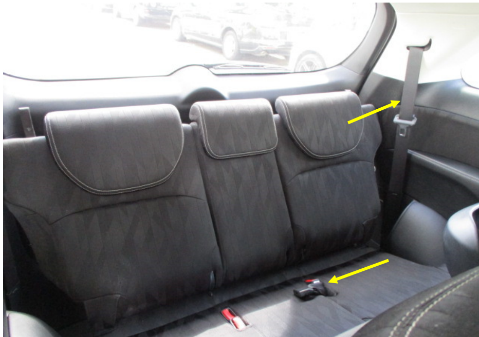
Photo 5 shows the rear seats (2 nd row) of the Motor Car. All the seats of the Motor Car were secured via seat rails to the floor board. They were also fitted with a retractable seat belt reel and a pre-tensioner (arrowed). The seat belts were all checked and able to be fastened securely to the respective pretension that was fitted on the side of each individual seat.
