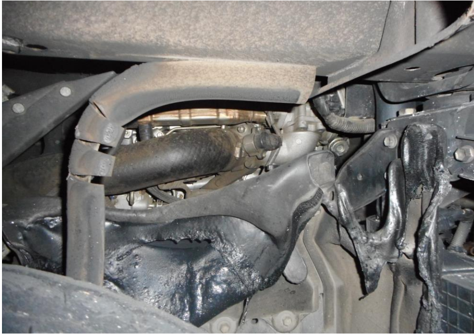
Photo 8 shows the engine compartment of the Insured Vehicle at the time of our inspection. The front cabin of the Insured Vehicle was not able to be lifted due to the damage it sustained from the fire, however visually the engine unit looks to be intact and was unaffected by the fire.
