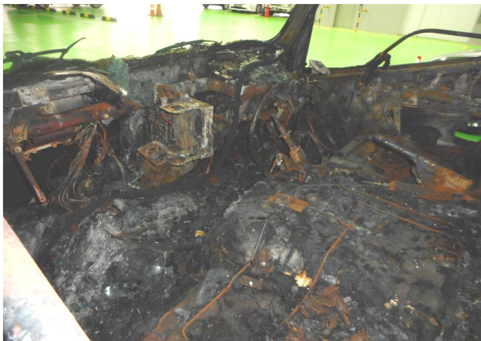
Photo 3 shows the close up view of the interior compartment of the Insured Vehicle. The interior compartment have been badly burnt by the fire.
