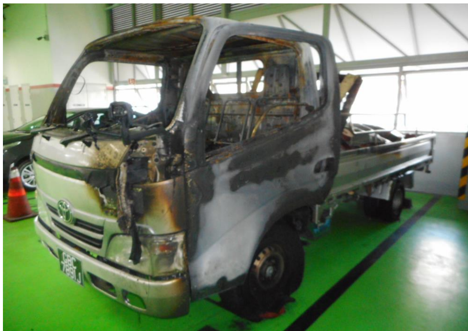
Photo 6 shows the left side of the Insured Vehicle at the time of our inspection. The fire damage to the Insured Vehicle was confined to its rear portion and interior compartment. The right rear cabin panel, handle railings and rear portion of the driver side door were amongst the parts that were observed to have been affected by the fire.
