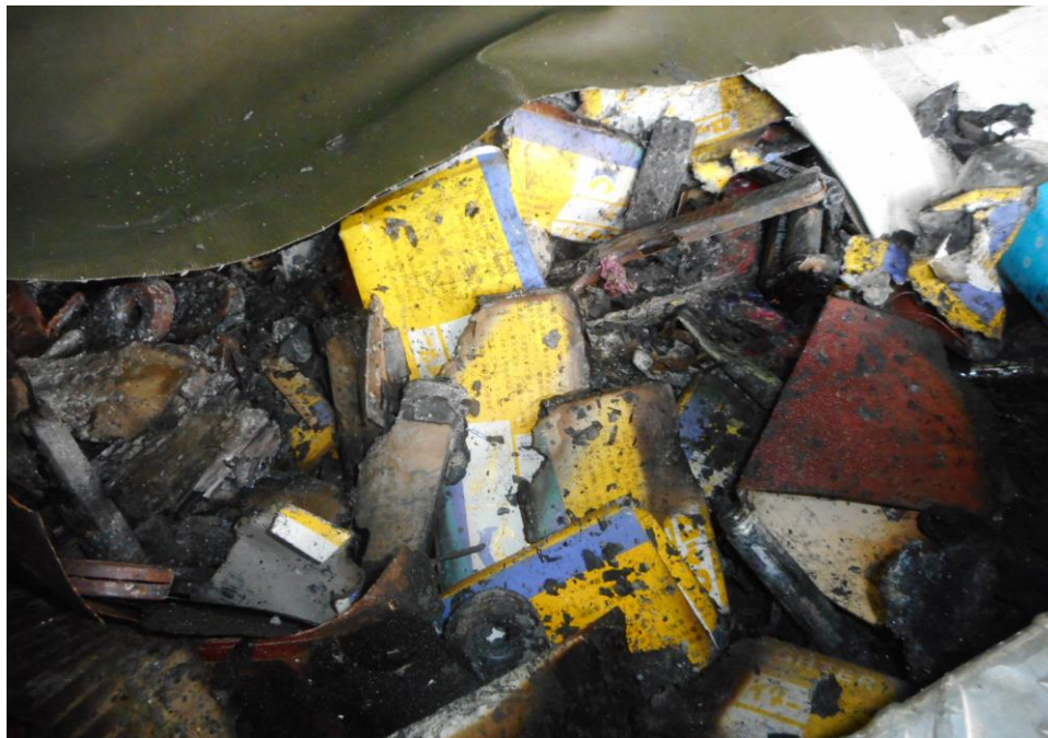
Photo 10 shows a closer view of the rear goods compartment of the Insured Vehicle at the time of our inspection. The rear cabin was significantly burnt and/or melted as a result of the fire. We also found remnants of burned sand paper, cardboard and various other items in the rear goods compartment.
