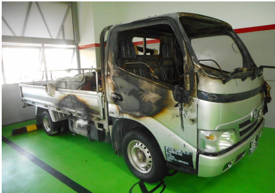
Photo 4 shows the right side of the Insured Vehicle at the time of our inspection. The fire damage to the Insured Vehicle was confined to its rear portion and interior compartment. The right rear cabin panel, handle railings and rear portion of the driver side door were amongst the parts that were observed to have been affected by the fire.
