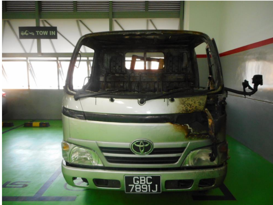
Photo 1 shows the front view of the Insured Vehicle at the time of our inspection. The fire damage to the Insured Vehicle was confined to its front cabin, interior compartment and rear portion.
