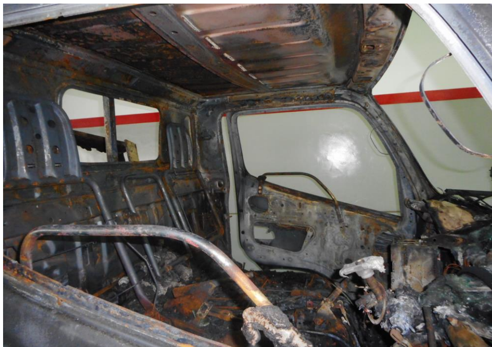
Photo 2 shows the general view of the interior compartment of the Insured Vehicle. The entire windscreen and the interior compartment have been badly burnt by the fire.
