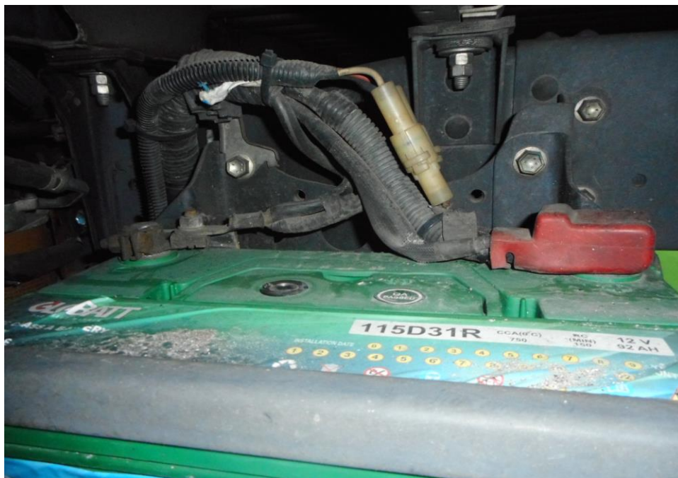
Photo 7 shows the battery unit of the Insured Vehicle at the time of our inspection. The battery unit and the battery terminal was unaffected by the fire damage to the Insured Vehicle.
