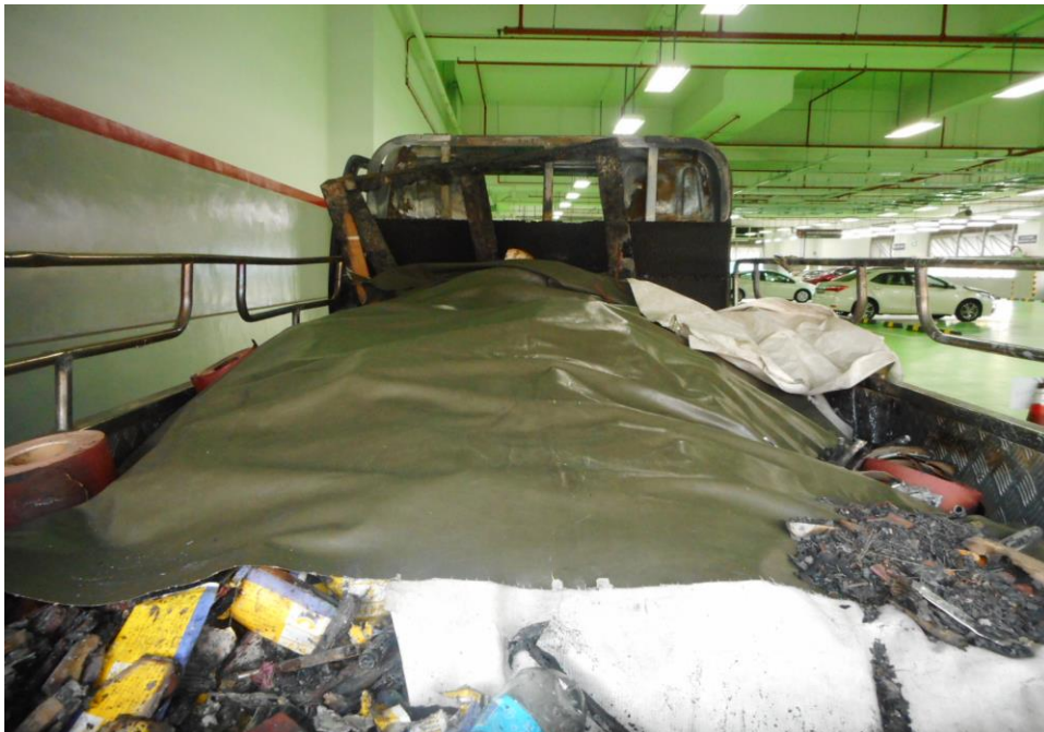
Photo 9 shows a closer view of the rear portion of the Insured Vehicle at the time of our inspection. The entire rear goods compartment, rear cabin panel, and sustained severe visible fire damage.
