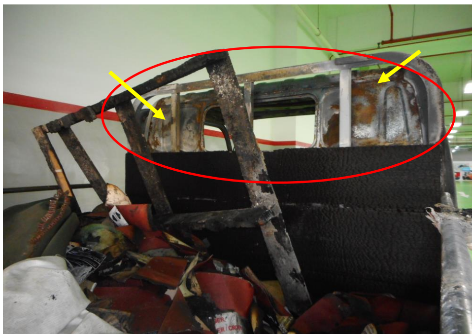
Photo 11 shows the fire damage at the rear portion of the Insured Vehicle. The high heat intensity burn marks (whitish burn marks) found on the exterior surface of the back portion of the front cabin (circled) and rust that had developed on the sides (red arrows) indicates that the fire to the Insured Vehicle had originated from the exterior of the Insured Vehicle. Indicating that the fire may have started from the rear goods compartment portion of the Insured Vehicle. This is also taking into consideration that there was no extensive fire damage at the interior of its engine compartment. Refer to photo 8 above.
