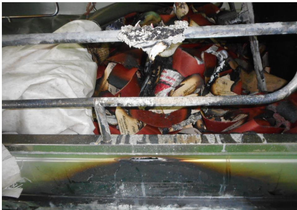
Photo 5 shows the close up view of the right side of the Insured Vehicle at the time of our inspection. The fire damage to the Insured Vehicle was confined to its rear portion and interior compartment. The right rear cabin panel and handle railings were amongst the parts that were observed to have been affected by the fire.
