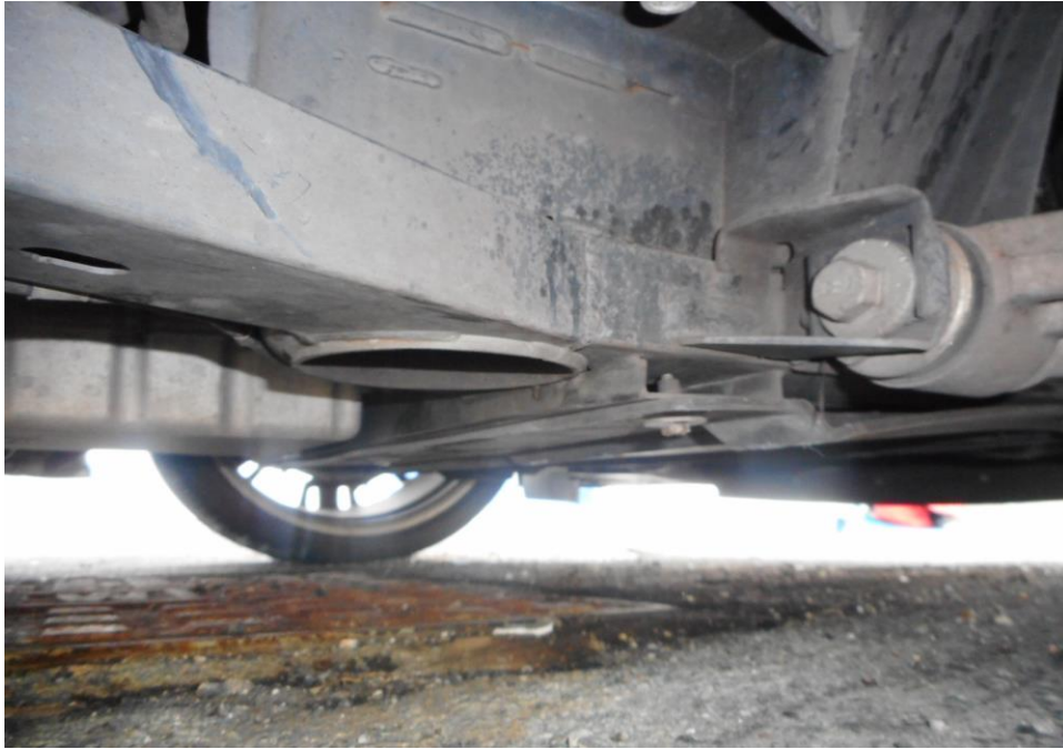
Photo 17 shows the undercarriage of the Motor Car, at the area where the engine housing and transmission housing are located. . I did not find any sign(s) or indication(s) of fluid leak and/or fluid stain(s) on the underside of the Motor Car.
