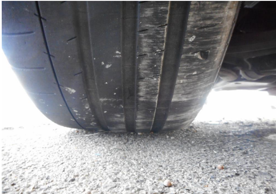
Photo 10 shows the condition of the front left tyres of the Motor Car, which were observed to be in serviceable condition with remaining, tread depth of approximately 3.5mm. There was also no tear, cut or burst mark(s) on the outer and the inner sidewalls as well as across the tread of the 4 tyres that were fitted on the Motor Car.
