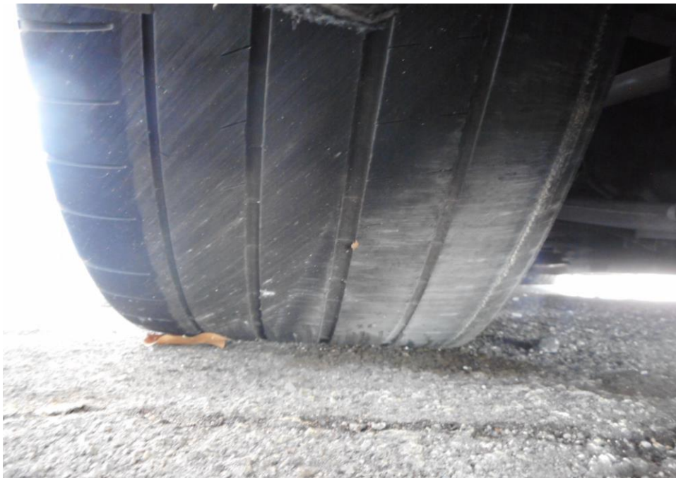
Photo 9 shows the condition of the rear left tyres of the Motor Car, which were observed to be in serviceable condition with remaining, tread depth of approximately 3.4mm. There was also no tear, cut or burst mark(s) on the outer and the inner sidewalls as well as across the tread of the 4 tyres that were fitted on the Motor Car.
