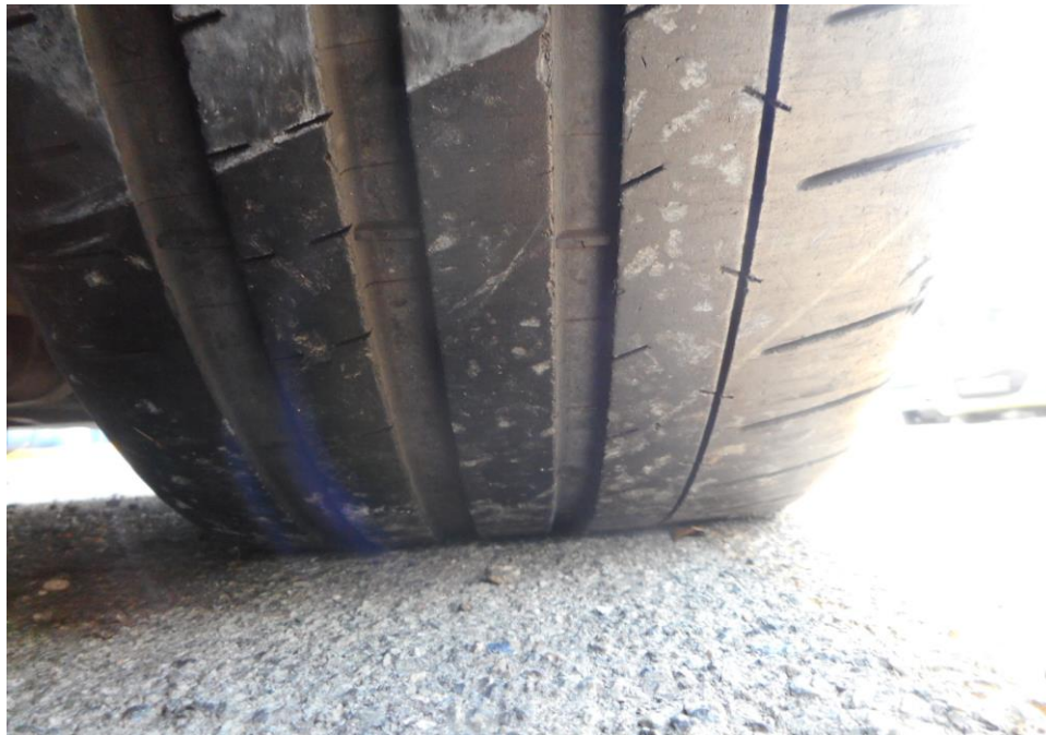
Photo 7 shows the condition of the front right tyre of the Motor Car, which was observed to be in serviceable condition with remaining tread depth of approximately 3.8mm. The tyre, which was wrapped around standard alloy wheel rim, was also observed to be sufficiently inflated for vehicular operation. There was no tear, cut or burst mark(s) on the outer and the inner sidewalls as well as across the tread of the 4 tyres that were fitted on the Motor Car.
