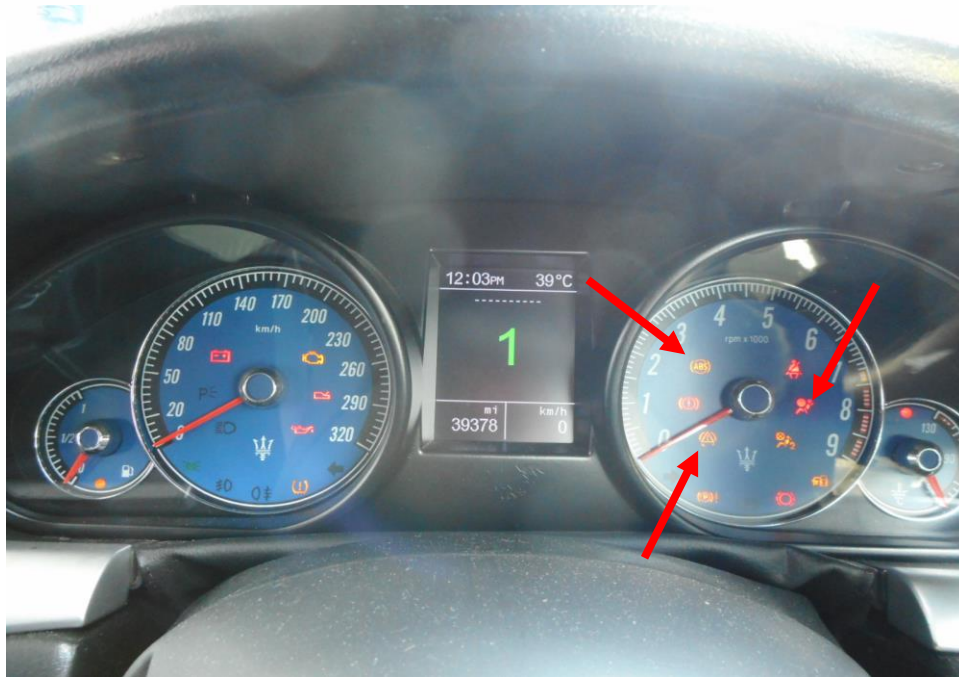
Photo 25 shows the warning light for Anti-Lock Brake System (ABS) and Supplemental Restraint System (SRS) and Traction Control System (TC) appearing on the instrument panel of the Motor Car during the self-test of its various electronic operating systems when its engine was cranked.
