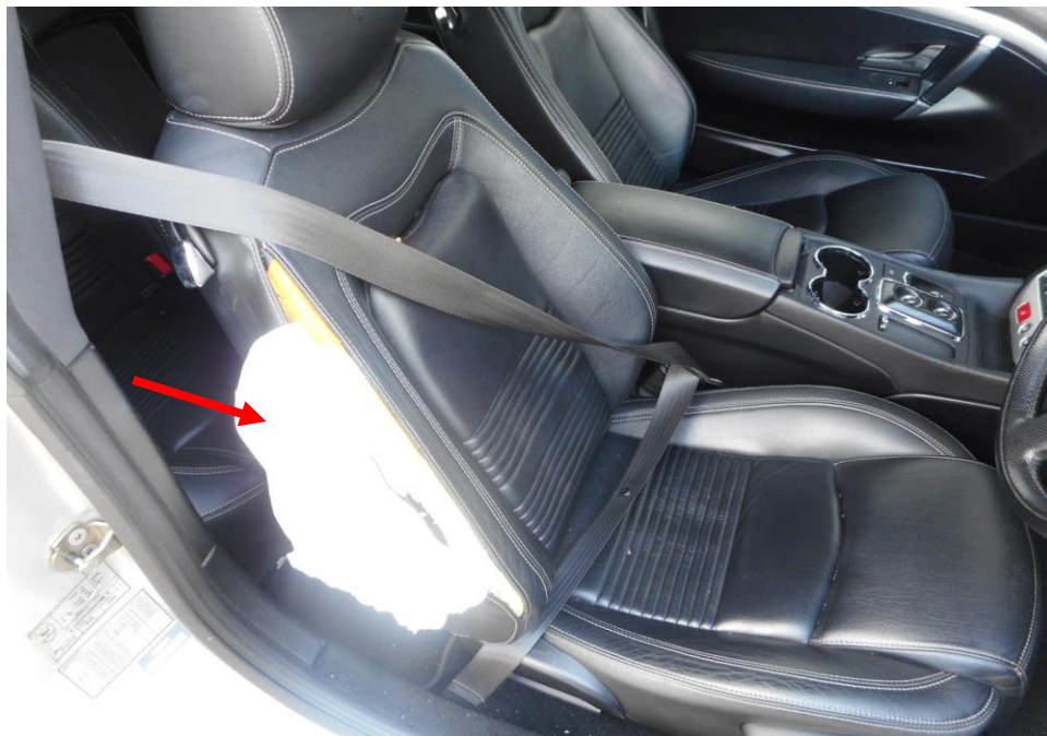
Photo 11 shows the deployment of the Supplemental Restraint System (SRS) airbag (arrowed) in the Motor Car as a result of the accident.
