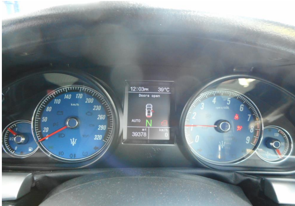
Photo 26 shows no warning lights illuminated on the instrument panel of the Motor Car after the engine was cranked. This would suggest that there was no abnormality to the various electronic operating systems of the Motor Car, like the ABS, SRS and TC.
