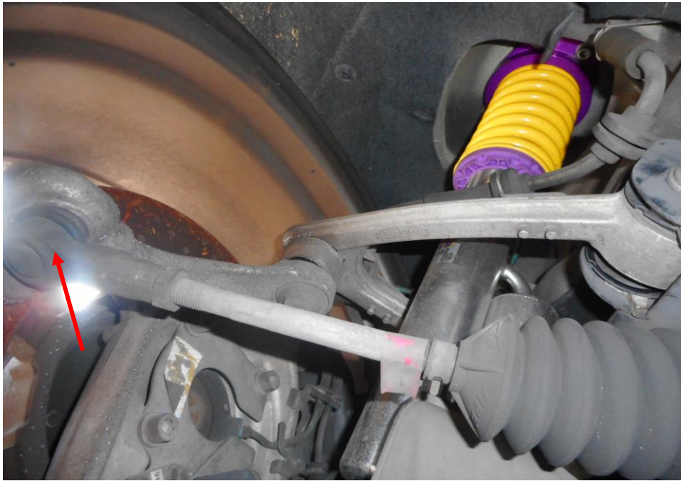
Photo 18 shows the various undercarriage components at the front right wheel of the Motor Car, in particular the steering tie rod end (arrowed). The various steering components were all found to be intact, suggesting that the steering system of the Motor Car was likely to be in serviceable condition at the material time of accident. There was also no sign of fluid stain(s) observed on the various undercarriage components.
