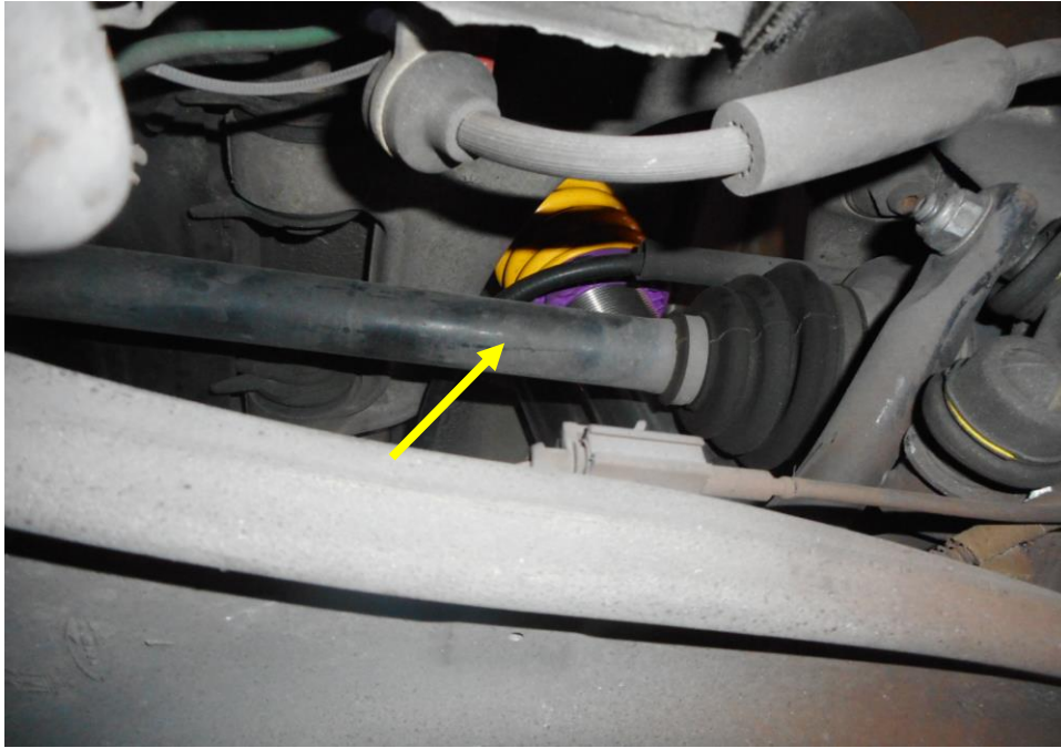
Photo 24 shows the various undercarriage components at the rear left wheel of the Motor Car, The drive shaft (yellow arrow) was found to be intact and there was no sign of fluid stain(s) observed on the various undercarriage components.
