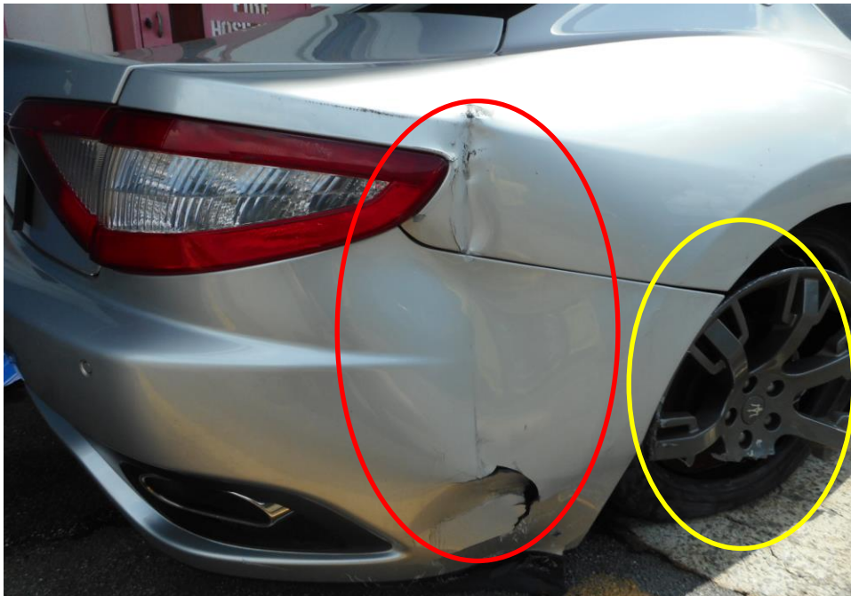
Photo 3 shows a close up view of the Motor Car's rear right portion at the time of my inspection. Its rear bumper and rear right fender (red circle), rear right rim (yellow circle) were damage at the time of my inspection.
