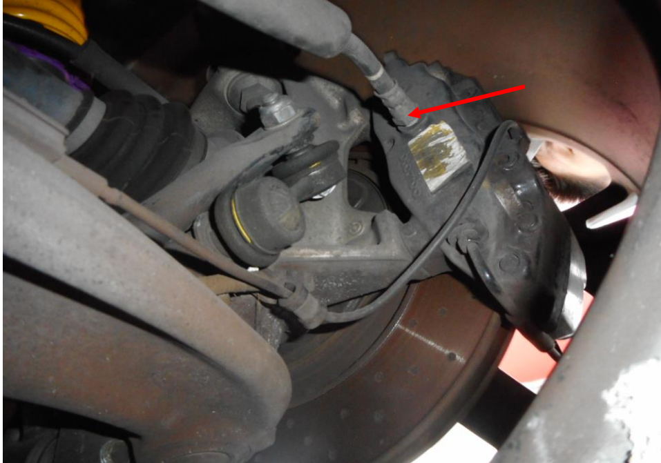
Photo 20 shows the brake pipe (arrowed) at the rear right wheel of the Motor Car. I did not observe any leakage of brake fluid at the time of my inspection of the Motor Car. My static tests of the Motor Car's braking system, along with my visual examination of the various mechanical components in the braking system, had indicated that there was no internal leakage of pressure/vacuum. Hence the braking system of the Motor Car was likely to be in serviceable condition at the material time of accident.
