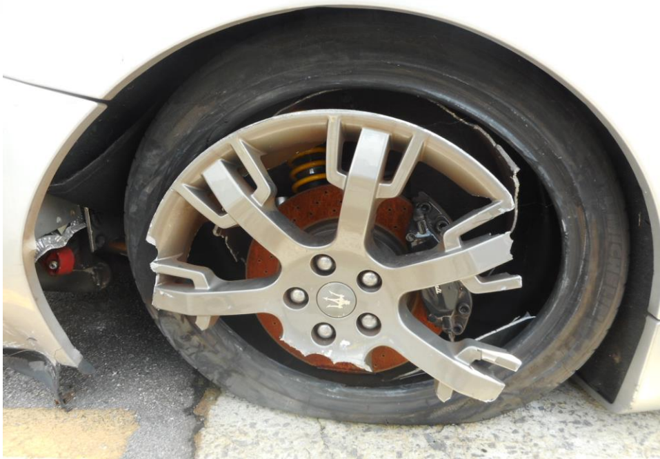
Photo 8 shows the condition of the rear right tyre of the Motor Car, which was observed to be in unserviceable condition. The tyre, which was wrapped around standard alloy wheel rim was slipped out due to the damaged to the rim as a result of the accident. There was no tear, cut or burst mark(s) on the outer and the inner sidewalls as well as across the tread of the tyre with remaining tread depth of approximately 4mm.
