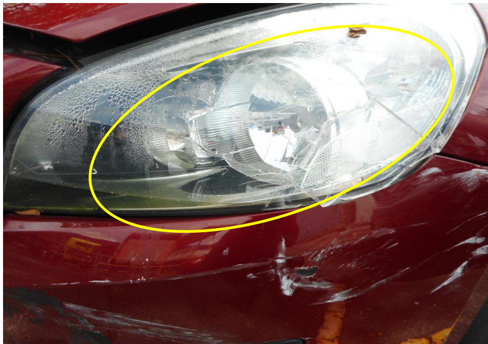
Photo 5 shows the close up view of the Motor Car's front body at the time of my inspection. The Motor Car was observed to have sustained damage at its front left headlamps (circled) as a result of the accident.
