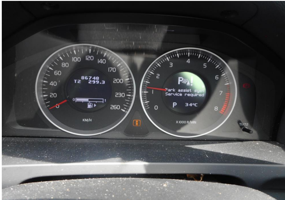
Photo 27 shows no warning lights illuminated on the instrument panel of the Motor Car after the engine was cranked. This would suggest that there was no abnormality to the electronic operating system of the Motor Car, like the ABS, TC and SRS etc.
