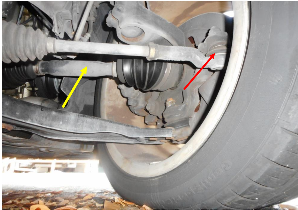
Photo 24 shows the various undercarriage components at the front right wheel of the Motor Car, in particular the steering tie rod (red arrow) and drive shaft (yellow arrow). The various steering components were all found to be intact, suggesting that the steering system of the Motor Car was likely to be in serviceable condition at the material time of accident. There was also no sign of fluid stain observed on the various undercarriage components at the front right wheel of the Motor Car.
