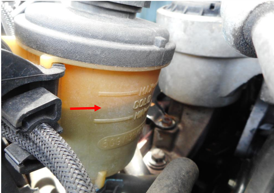
Photo 17 shows the power steering fluid reservoir of the Motor Car at the time of my inspection. The power steering fluid was observed to be of sufficient level (arrowed) and without any visible contamination.
