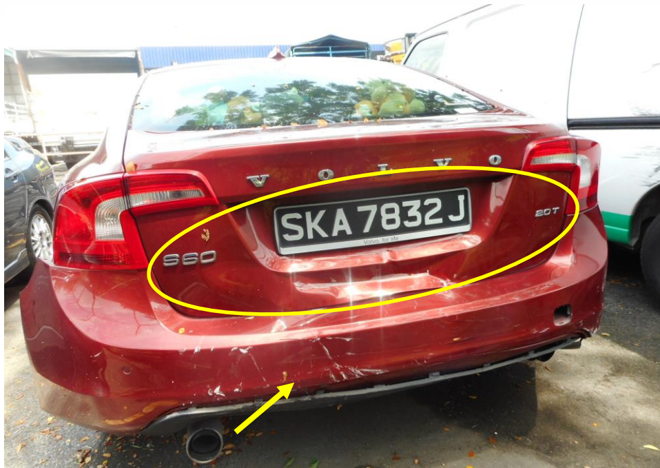
Photo 6 shows the general view of the Motor Car's rear body at the time of my inspection. The Motor Car rear was observed to have sustained damage at its rear boot (circled) and rear bumper (arrowed) as a result of the accident.
