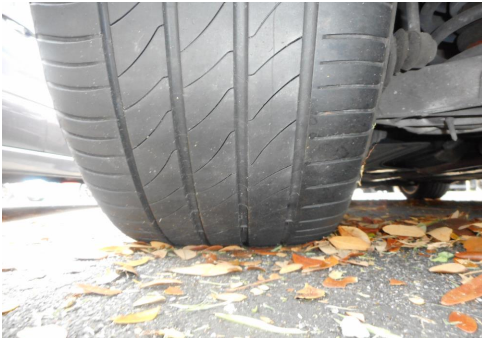
Photo 11 shows the condition of the rear left tyre of the Motor Car, which was observed to be in serviceable condition with remaining tread depth of approximately 4.1mm. The tyre, which was wrapped around steel wheel rim, was also observed to be sufficiently inflated for vehicular operation. The 4 tyres of the Motor Car were wrapped around standard steel wheel rims.
