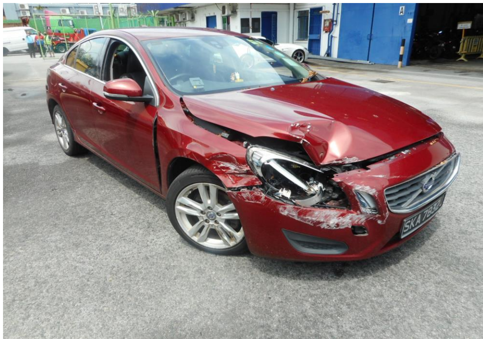
Photo 23 shows the front right wheel of the Motor Car turned to its full left. During my steering system test, I did not experience any abnormal free play and/or resistance when I had turned the steering wheel towards the left and right. This would suggest that the steering system of the Motor Car was likely to be in serviceable condition at the material time of accident.
