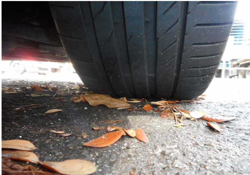
Photo 9 shows the condition of the front right tyre of the Motor Car, which was observed to be in serviceable condition with remaining tread depth of approximately 4.9mm. The tyre was sufficiently inflated for vehicular operation with no tear, cut or burst mark(s) on the outer and the inner sidewalls as well as across the tread. The 4 tyres of the Motor Car were wrapped around standard steel wheel rims without any damage.
