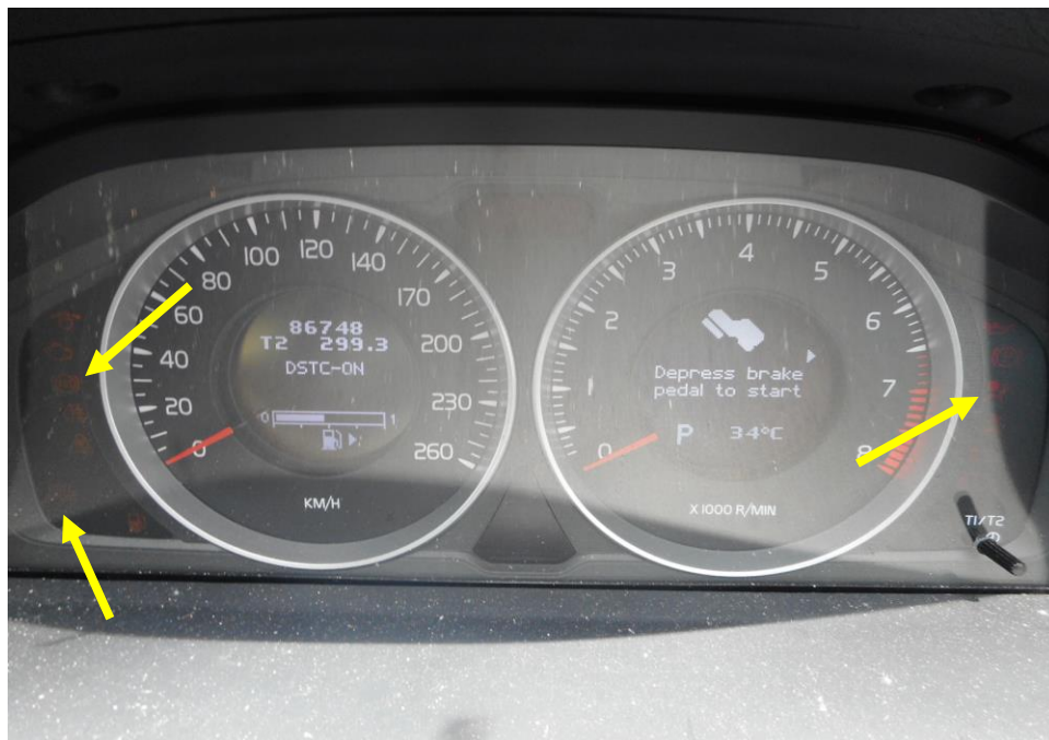
Photo 26 shows the warning light for Anti-Lock Brake System (ABS), Traction Control System (TC) and Supplemental Restraint System (SRS) (arrowed) appearing on the instrument panel of the Motor Car during the self-test of its various electronic operating systems when its engine was cranked.
