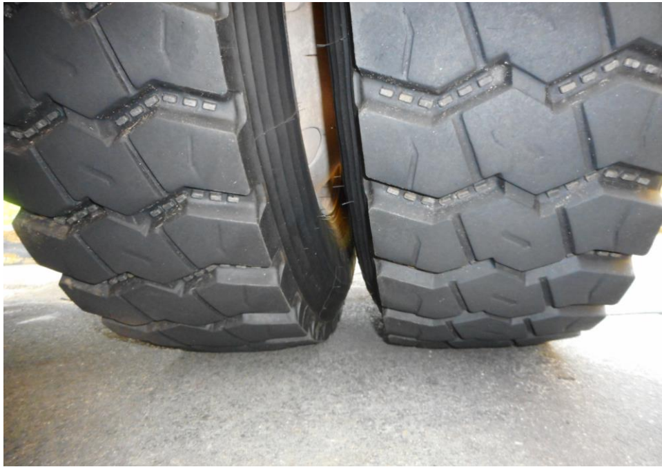
Photo 10 shows the condition of the rear left tyres of the Oil Tanker, which was observed to be in serviceable condition with remaining tread depth of approximately 15mm. The tyres, which were wrapped around standard steel wheel rim, were also observed to be sufficiently inflated for vehicular operation. There was also no damage found on all 10 steel wheel rims of the Oil Tanker.
