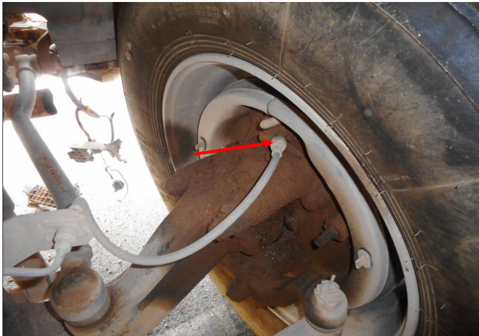
Photo 21 shows the brake pipe (arrowed) at the front right wheel of the Oil Tanker. I did not observe any leakage of brake fluid at the time of my inspection of the Oil Tanker. My static tests of the Oil Tanker's braking system, along with my visual examination of the various mechanical components in the braking system had indicated that there was no internal leakage of pressure/vacuum. Hence the braking system of the Oil Tanker was likely to be in serviceable condition at the material time of accident.
