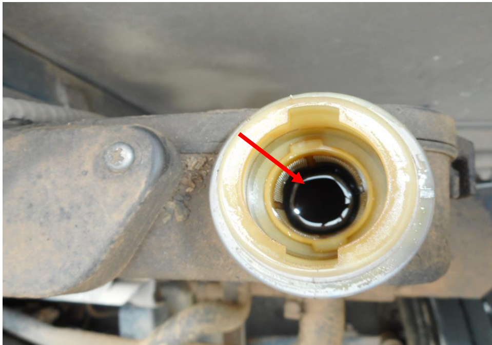
Photo 16 shows the power steering reservoir of the Oil Tanker at the time of my inspection. The steering fluid was observed to be of sufficient level (arrowed) and without any visible contamination.
