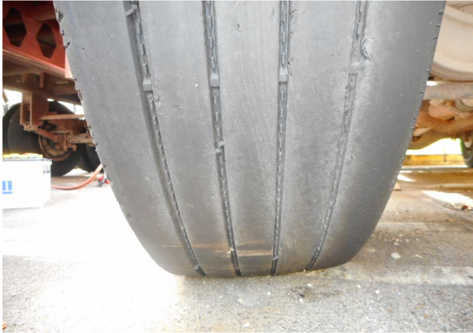
Photo 8 shows the condition of the front right tyre of the Oil Tanker, which was observed to be in serviceable condition with remaining tread depth of approximately 4.6 mm. The tyre, which was wrapped around standard steel wheel rim, was also observed to be sufficiently inflated for vehicular operation. There was no tear, cut or burst mark(s) on the outer and the inner sidewalls as well as across the tread of the 10 tyres that were fitted on the Oil Tanker.
