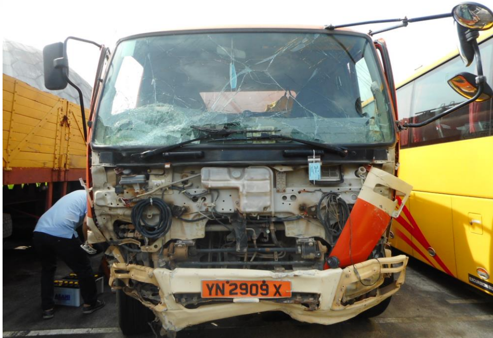
Photo 2 shows a general view of the front body of the Oil Tanker at the time of my inspection. The Oil Tanker was observed to have sustained damage at its frontal portion. Its front windscreen and front body panel were amongst the body parts that were damaged as a result of the accident.
