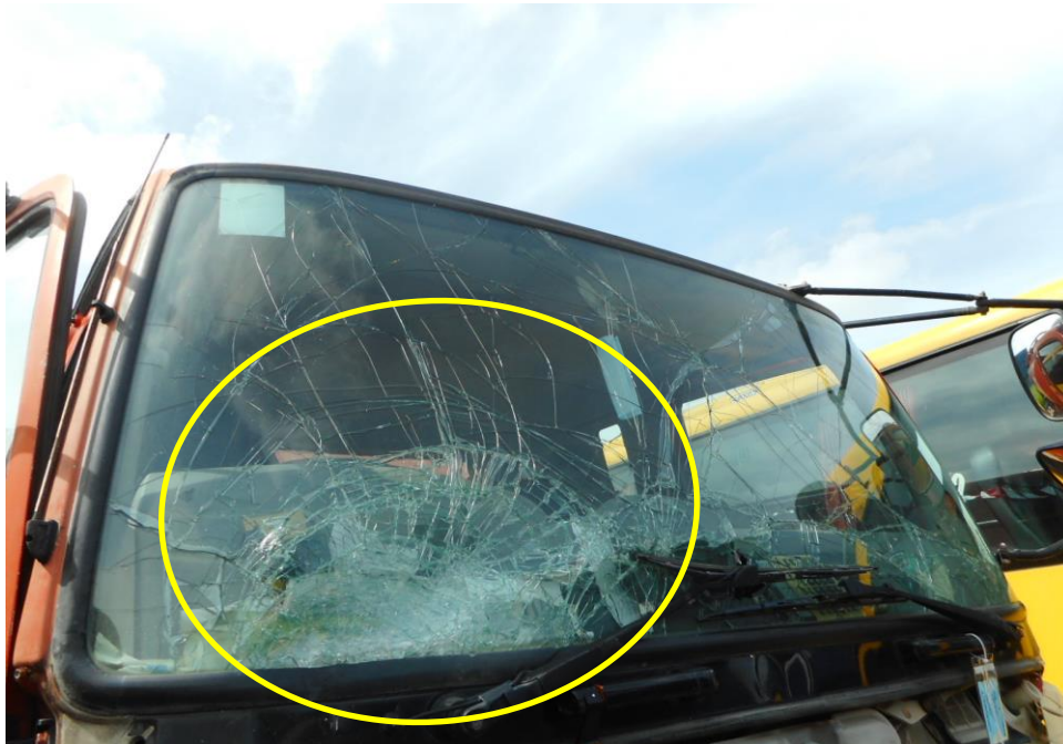
Photo 3 shows the close up view of the Oil Tanker front body at the time of my inspection. The Oil Tanker was observed to have sustained damage at its front windscreen (circled), as a result of the accident.
