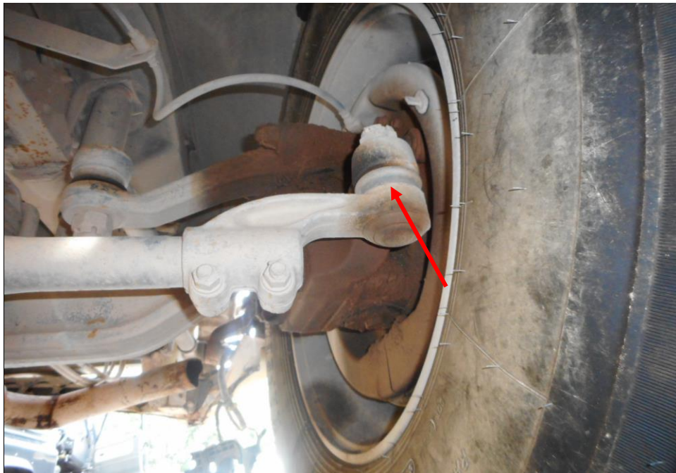
Photo 23 shows the various undercarriage components at the front right wheel of the Oil Tanker, in particular the steering tie rod end (arrowed). The various steering components were all found to be intact, suggesting that the steering system of the Oil Tanker was likely to be in serviceable condition at the material time of accident. There was also no sign of fluid stain(s) observed on the various undercarriage components.
