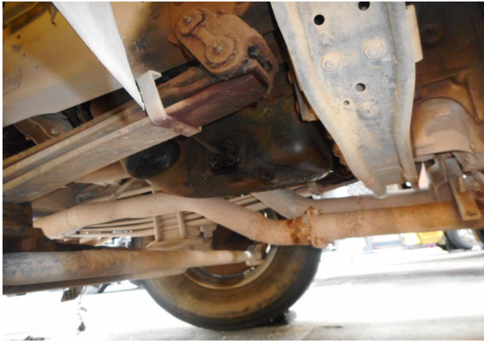
Photo 17 shows the undercarriage of the Oil Tanker, at the area where the engine housing located. I did not find any sign(s) or indication(s) of fluid leak and/or fluid stain(s) on the underside of the Oil Tanker.
