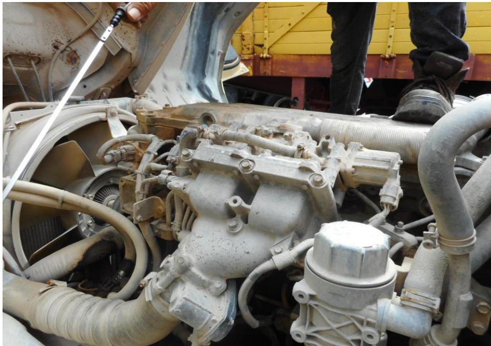
Photo 12 shows a general view of the Oil Tanker's engine compartment, which was accessed by lifting the front cabin of the Oil Tanker. The various parts and components inside the engine compartment were unaffected by the accident. There was also no sign(s) or indication(s) of fresh fluid leakage and/or fluid stain within the engine compartment
