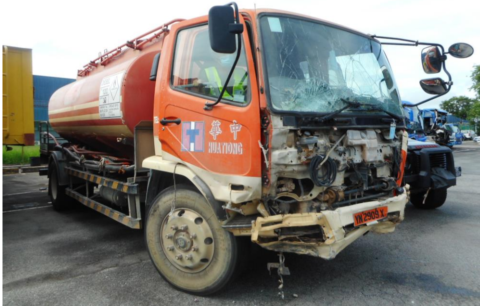
Photo 26 shows the front right wheel of the Oil Tanker turned to its full left. During my steering system test, I did not experience any abnormal free play and/or resistance when I had turned the steering wheel towards full left and full right. This would suggest that the steering system of the Oil Tanker was likely to be in serviceable condition at the material time of accident.
