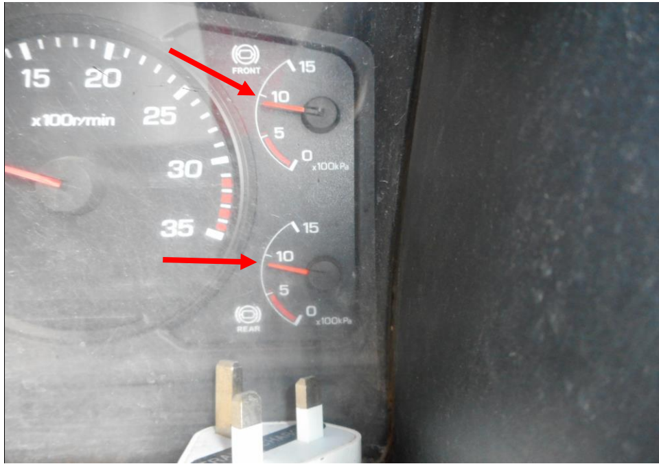
Photo 13 shows the air in the air brake cylinders of the Oil Tanker at the time of my inspection. The air in the cylinder was observed to be of sufficient level & serviceable at the time of the accident.
