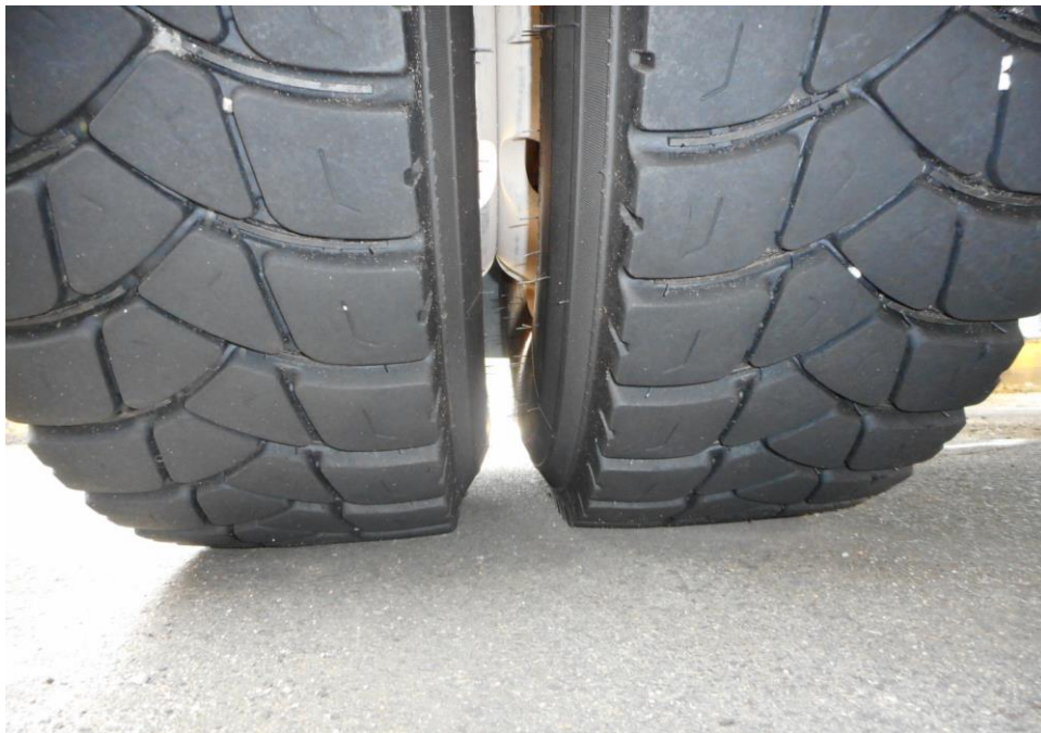
Photo 9 shows the condition of the rear right tyre of the Oil Tanker, which was observed to be in serviceable condition with remaining tread depth of approximately 9mm. The tyre, which was wrapped around standard steel wheel rim, was also observed to be sufficiently inflated for vehicular operation.
