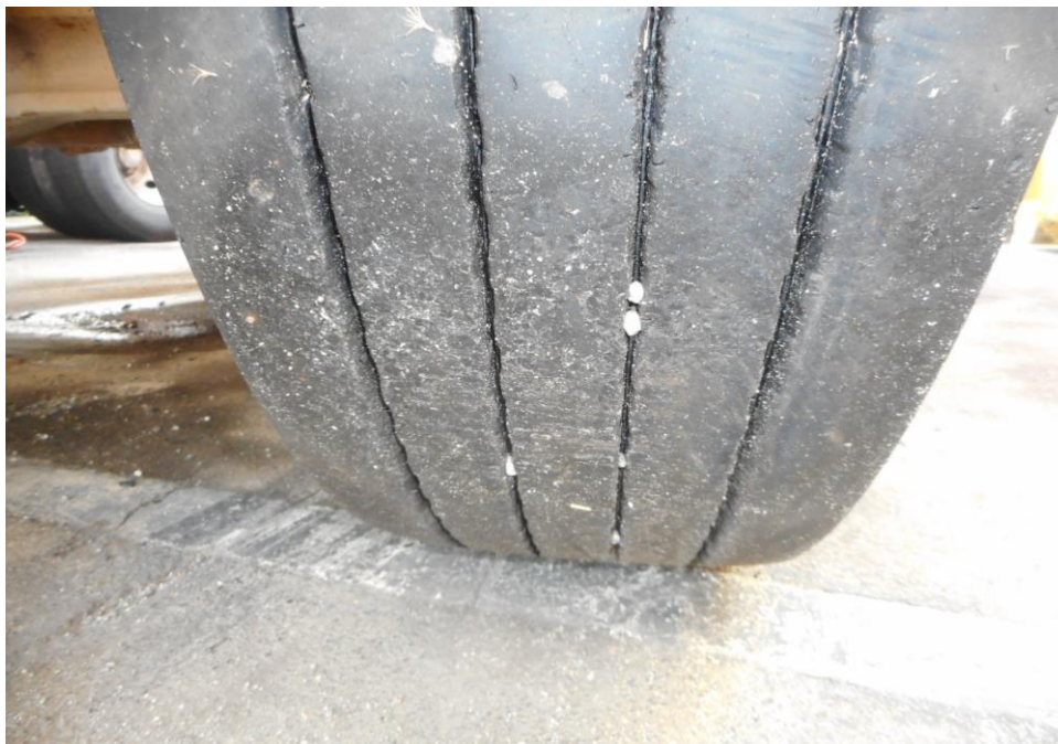
Photo 11 shows the condition of the front left tyres of the Oil Tanker, which were observed to be in serviceable condition with remaining tread depth of approximately 6.9mm. There was also no tear, cut or burst mark(s) on the outer and the inner sidewalls as well as across the tread of the 10 tyres that were fitted on the Oil Tanker.
