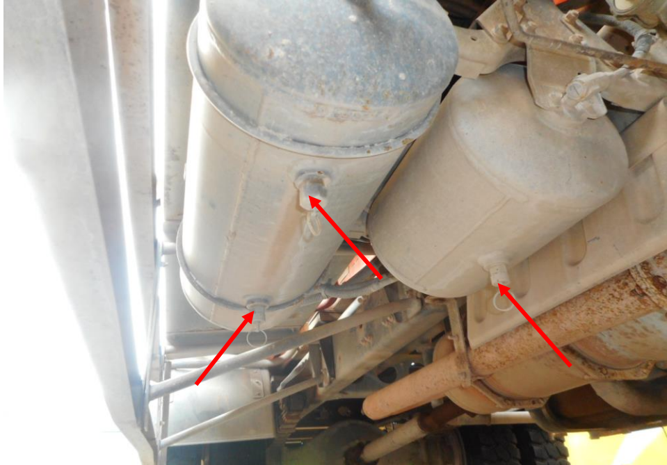
Photo 22 shows the air brake cylinders (arrowed) at the undercarriage of the Oil Tanker. I did not observe any leakage of air brake fluid at the time of my inspection of the Oil Tanker. My static tests of the Oil Tanker's braking system, along with my visual examination of the various mechanical components in the braking system had indicated that there was no internal leakage of pressure/vacuum. Hence the braking system of the Oil Tanker was likely to be in serviceable condition at the material time of accident.
