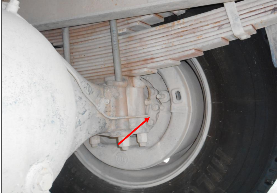
Photo 18 shows the brake pipe (arrowed) at the rear right wheel of the Oil Tanker. I did not observe any leakage of brake fluid at the time of my inspection of the Oil Tanker. My static tests of the Oil Tanker's braking system, along with my visual examination of the various mechanical components in the braking system, had indicated that there was no internal leakage of pressure/vacuum. Hence the braking system of the Oil Tanker was likely to be in serviceable condition at the material time of accident.
