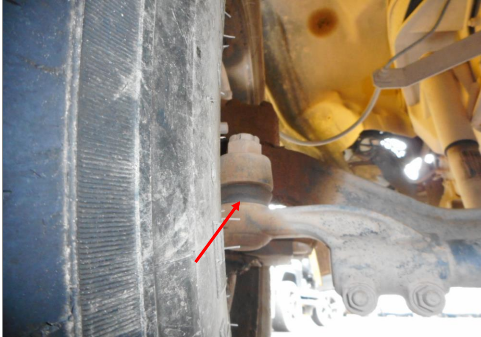
Photo 24 shows the various undercarriage components at the front left wheel of the Oil Tanker, in particular the steering tie rod end (arrowed). The various undercarriage components of the Oil Tanker were all found to be intact without any visible damage. There was also no sign of fluid stain(s) observed on the various undercarriage components.
