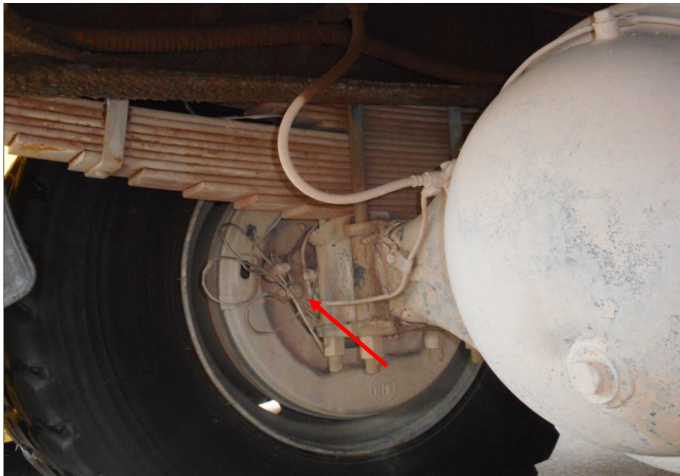
Photo 19 shows the brake pipe (arrowed) at the rear left wheel of the Oil Tanker. I did not observe any leakage of brake fluid at the time of my inspection of the Oil Tanker. My static tests of the Oil Tanker's braking system, along with my visual examination of the various mechanical components in the braking system, had indicated that there was no internal leakage of pressure/vacuum. Hence the braking system of the Oil Tanker was likely to be in serviceable condition at the material time of accident.
