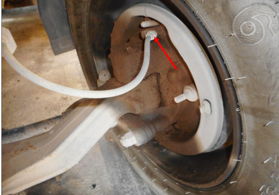
Photo 20 shows the brake pipe (arrowed) at the front left wheel of the Oil Tanker. I did not observe any leakage of brake fluid at the time of my inspection of the Oil Tanker. My static tests of the Oil Tanker's braking system, along with my visual examination of the various mechanical components in the braking system, had indicated that there was no internal leakage of pressure/vacuum. Hence the braking system of the Oil Tanker was likely to be in serviceable condition at the material time of accident.
