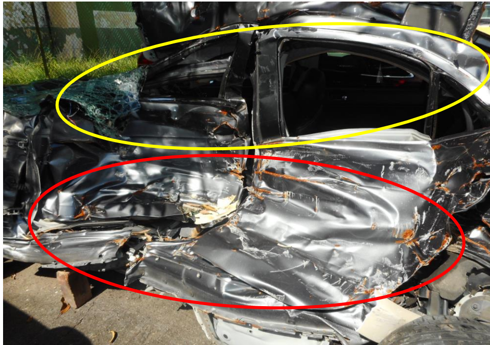
Photo 5 shows a close up view of the left portion of the Motor Car at the time of my inspection. The left side of the Motor Car had sustained extensive impact, it's both left doors (red circle), whole body panel structure and both left windscreens (yellow circle) was observed to have been damaged as a result of the accident.
