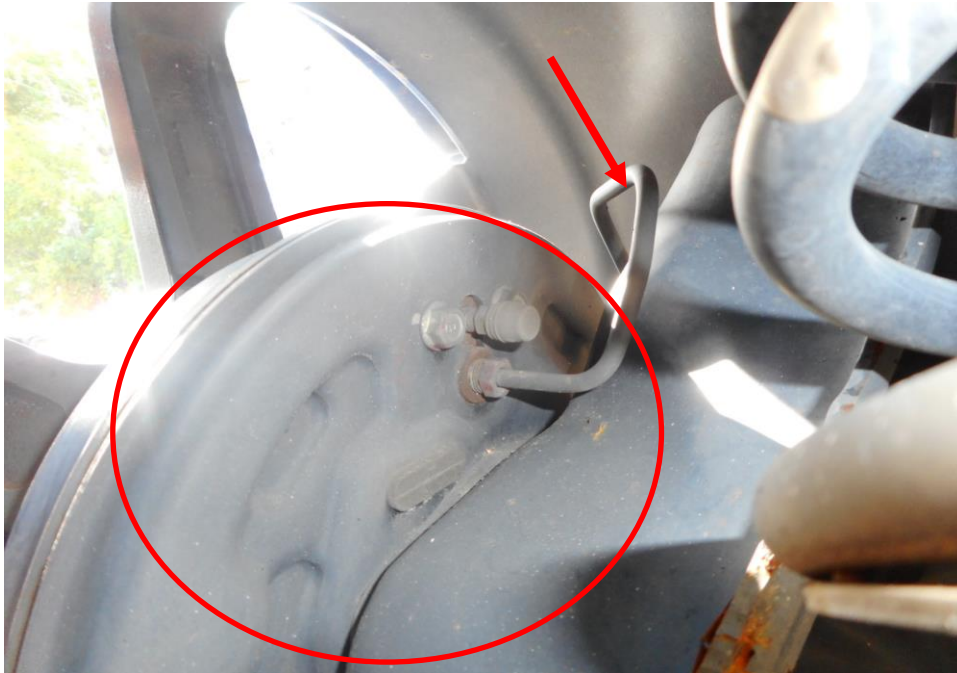
Photo 19 shows the brake drum (circled) and brake hose/pipe (arrowed) at the rear left wheel of the Motor Car and it was observed to be intact
