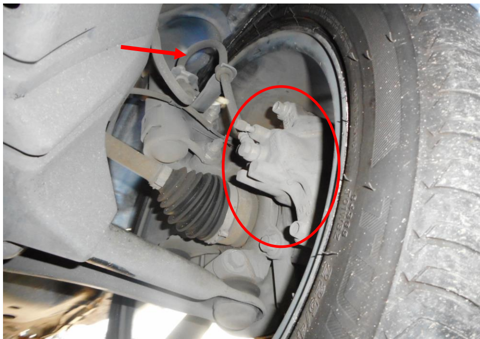
Photo 22 shows the brake hose/pipe (arrowed) at the front left wheel of the Motor Car. No leakage of brake fluid was observed. Visual examination of the various components of the braking system like the brake caliper (circled), brake booster, brake pedal etc had revealed all to be intact and without visible damage at the time of accident. There was also no sign of fluid stain(s) observed on the various undercarriage components.
