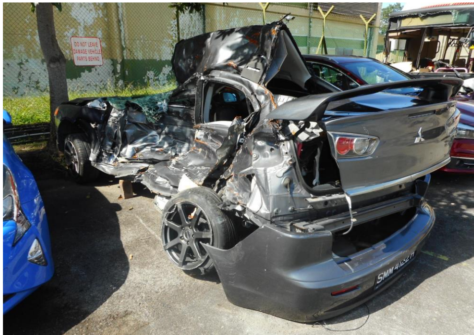
Photo 4 shows a general view of the left portion of the Motor Car at the time of my inspection. The left side of the Motor Car had sustained extensive impact, its doors and the whole body panel structure was observed to have been damaged as a result of the accident.
