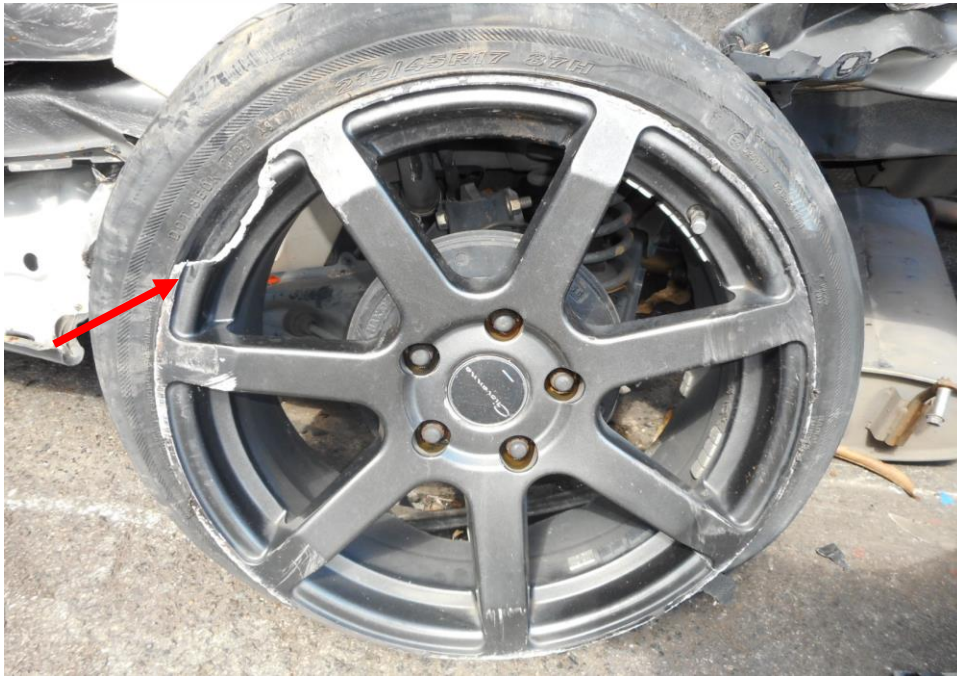
Photo 11 shows the condition of the rear left tyre of the Motor Car, which was observed to be in serviceable condition with remaining tread depth of approximately 5.5mm. The tyre was also observed to be sufficiently inflated for vehicular operation with no tear, cut or burst mark(s), however observed to be deflated due to damage to the rims (arrowed).
