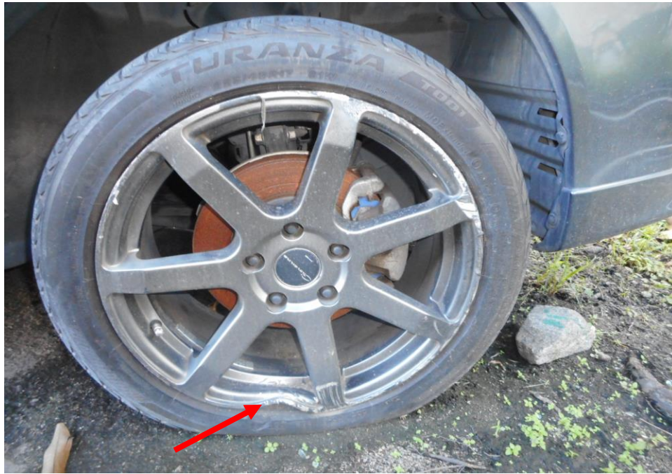
Photo 9 shows the condition of the front right tyre of the Motor Car, which was observed to be in serviceable condition with remaining tread depth of approximately 5.3mm. There was also no tear, cut or burst mark(s) on the outer and the inner sidewalls as well as across the tread of the Motor Car's 4 tyres, however observed to be deflated due to damage to the rims (arrowed).
