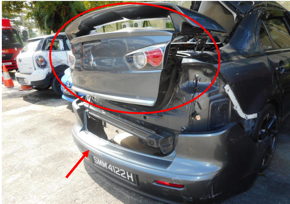
Photo 7 shows a general view of the rear portion of the Motor Car at the time of my inspection. The rear portion boot (circled) and bumper (arrowed) of the Motor Car was observed to have been damaged as well from the induced impact by the accident.
