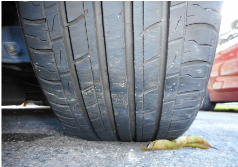
Photo 10 shows the condition of the rear right tyre of the Motor Car, which was observed to be in serviceable condition with remaining tread depth of approximately 5.6mm. The tyre was also observed to be sufficiently inflated for vehicular operation with no tear, cut or burst mark(s).
