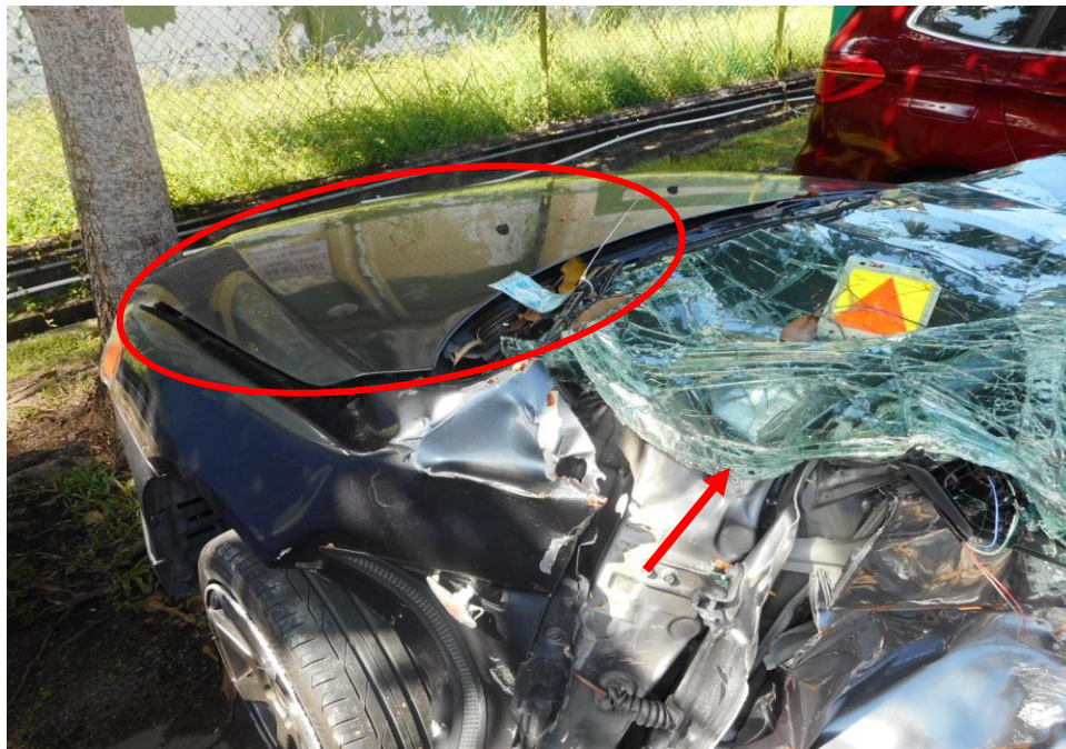
Photo 2 shows a close up view of the front portion of the Motor Car at the time of my inspection. The front bonnet (circled) and front windscreen (arrowed) was observed to have been damaged as a result of the accident.
