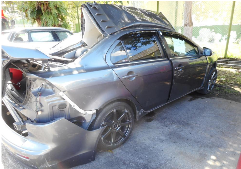
Photo 6 shows a general view of the right portion of the Motor Car at the time of my inspection. The right body panel of the Motor Car was relatively intact with minor dents on the panels as a result of the accident.
