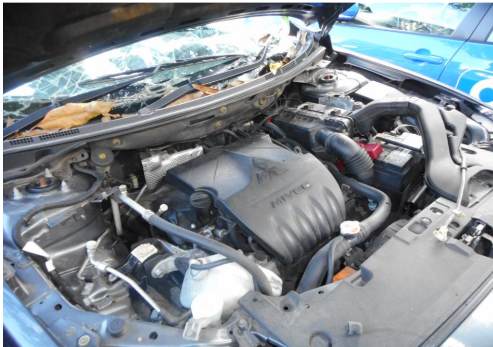
Photo 13 shows a general view of the Motor Car's engine compartment, which was accessed by lifting the front cabin of the Motor Car. The various parts and components inside the engine compartment were unaffected by the accident. However, the intake pipe and ignition system was observed to be damaged due to the induced impact from the accident. There was also no sign(s) or indication(s) of fresh fluid leakage and/or fluid stain within the engine compartment
