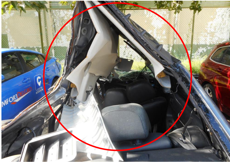
Photo 3 shows a close up view of the roof portion of the Motor Car at the time of my inspection. The roof of the Motor Car was observed to have been damaged as a result of the induced impact from the accident (circled)
