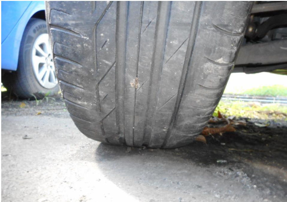
Photo 12 shows the condition of the front left tyre of the Motor Car, which was observed to be in serviceable condition with remaining tread depth of approximately 5.5mm. The tyre was also observed to be sufficiently inflated for vehicular operation with no tear, cut or burst mark(s).
