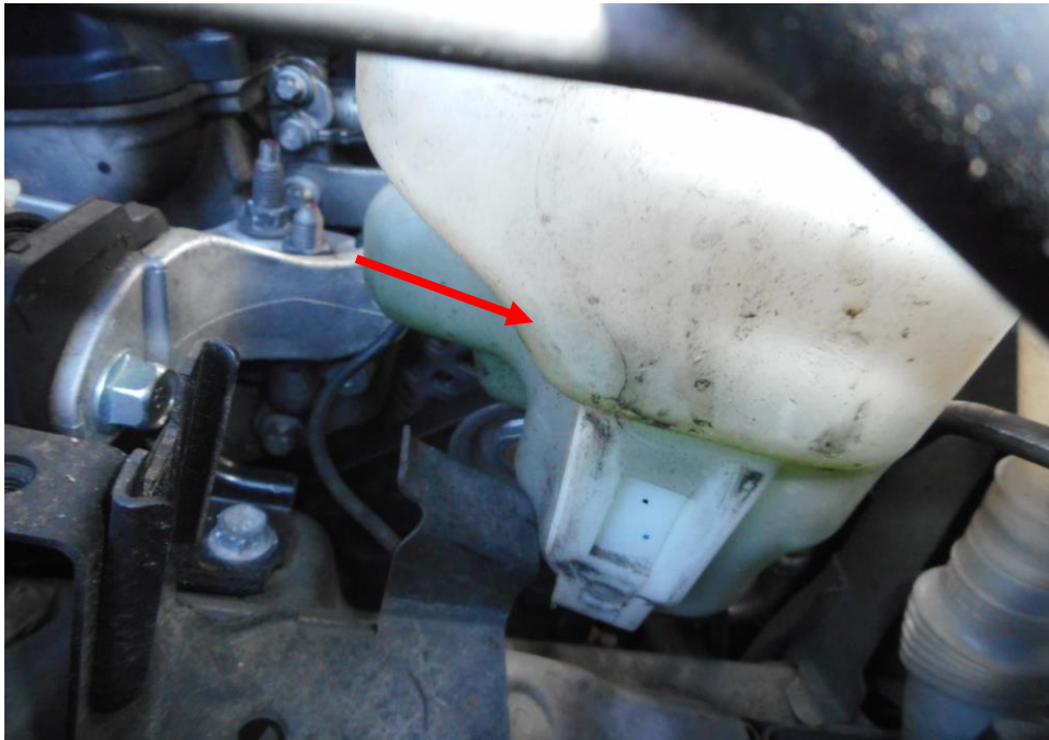
Photo 16 shows the engine coolant reservoir of the Motor Car at the time of my inspection. The engine coolant was observed to be of sufficient level (arrowed) and without any visible contamination.
