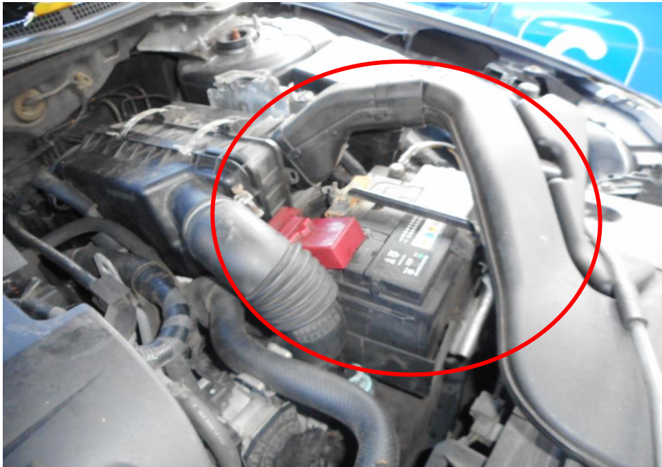
Photo 14 shows a close up view of the Motor Car's engine compartment, which was accessed by lifting the front cabin of the Motor Car. The intake pipe and ignition system (circled) was observed to be damaged due to the induced impact from the accident.
