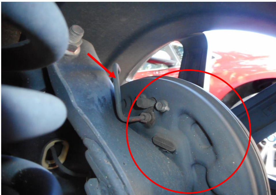
Photo 20 shows the brake drum (circled) brake hose/pipe (arrowed) at the rear right wheel of the Motor Car and it was observed to be intact
