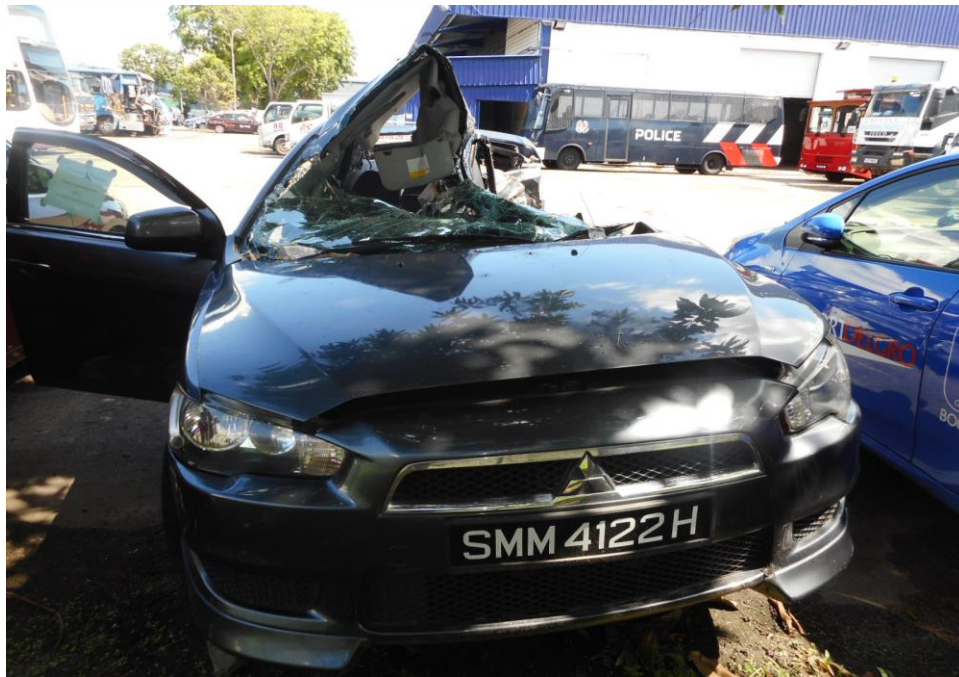
Photo 1 shows a general view of the front portion of the Motor Car at the time of my inspection. The Motor Car was also observed to have sustained extensive major impact damage at its left portion, body parts around the whole Motor Car had sustained damage as well. The front bonnet and rear boot and roof were also observed to have been damaged as a result of the accident.
