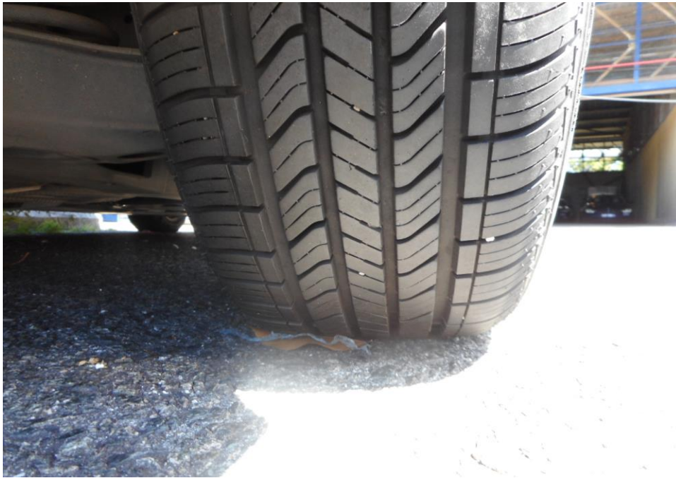
Photo 8 shows the condition of the rear right tyre of the Motor Taxi, which was observed to be in serviceable condition with remaining tread depth of approximately 6.9mm. The tyre, which was wrapped around standard alloy wheel rim, was also observed to be sufficiently inflated for vehicular operation.
