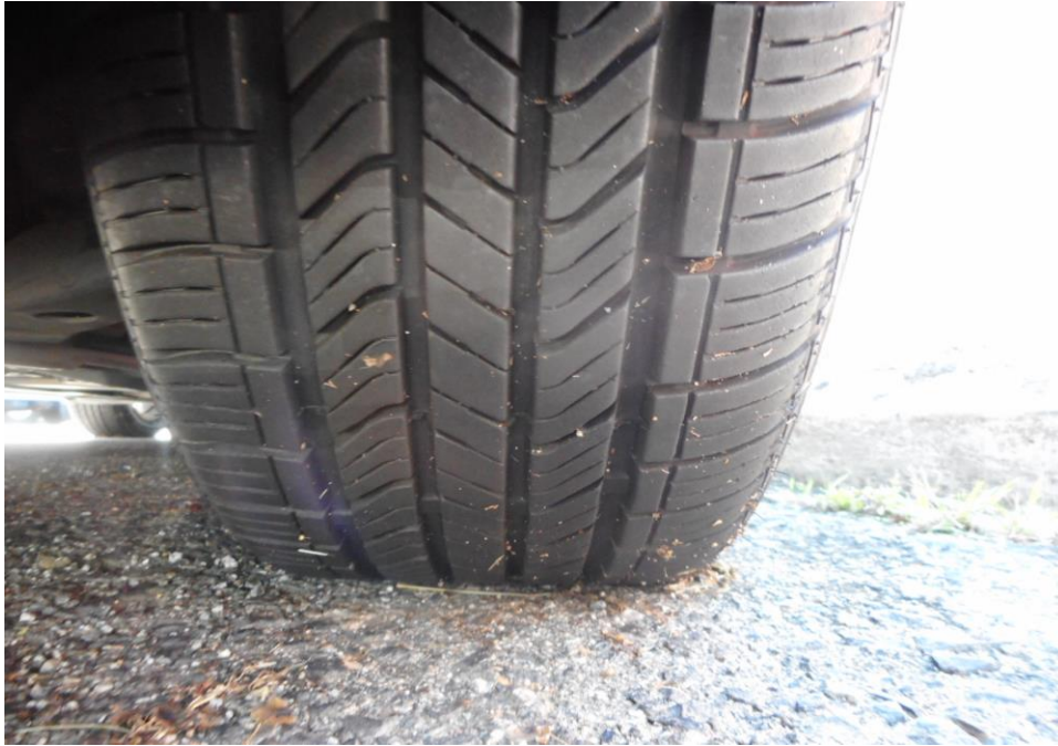
Photo 10 shows the condition of the rear right tyres of the Motor Taxi, which were observed to be in serviceable condition with remaining, tread depth of approximately 6.4mm. There was also no tear, cut or burst mark(s) on the outer and the inner sidewalls as well as across the tread of the 4 tyres that were fitted on the Motor Taxi.
