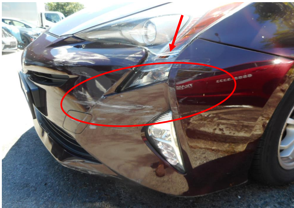
Photo 3 shows a close up view of the front body of the Motor Taxi at the time of my inspection. The Motor Taxi was observed to visually sustain damage at its front bumper (circled) and front left headlamp (arrowed) at the time of inspection.
