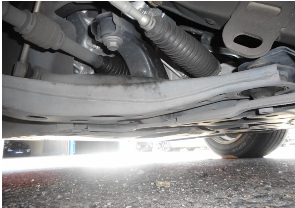
Photo 15 shows the undercarriage of the Motor Taxi, at the area where the engine housing and transmission housing are located. . I did not find any sign(s) or indication(s) of fluid leak and/or fluid stain(s) on the underside of the Motor Taxi.
