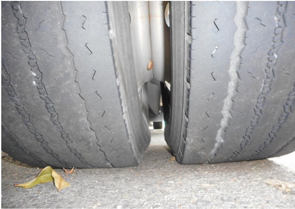
Photo 8 shows the condition of the rear right tyres of the Motor Lorry, which was observed to be in serviceable condition with remaining, tread depth of approximately 2.7mm. The tyres, which were wrapped around standard steel wheel rim, were also observed to be sufficiently inflated for vehicular operation. There was also no damage found on all 6 steel wheel rims of the Motor Lorry.
