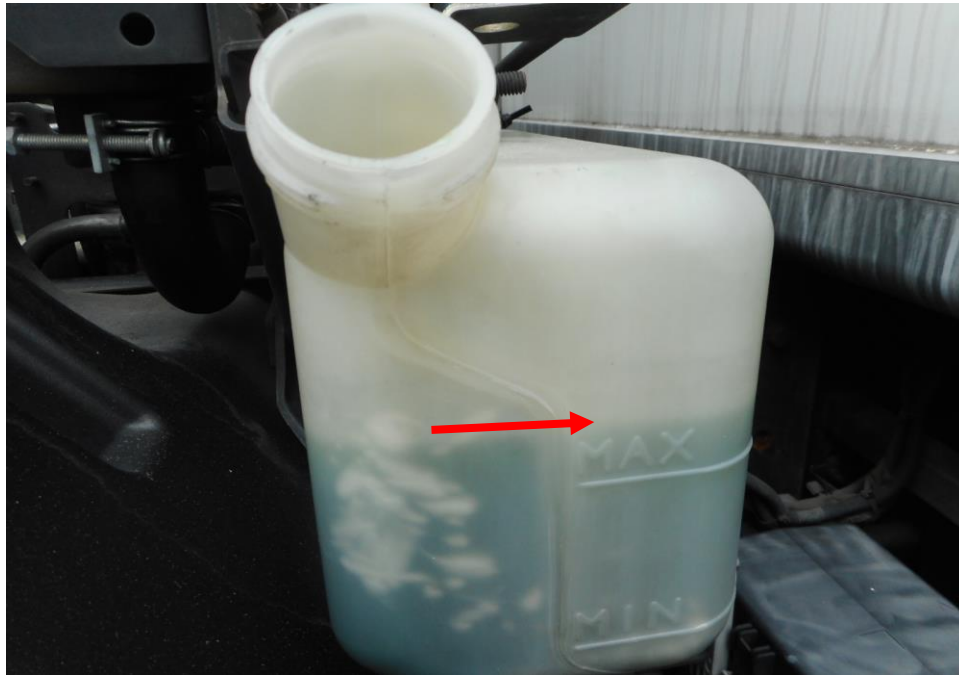
Photo 13 shows the engine coolant reservoir of the Motor Lorry at the time of my inspection. The engine coolant was observed to be of sufficient level (arrowed) and without any visible contamination.
