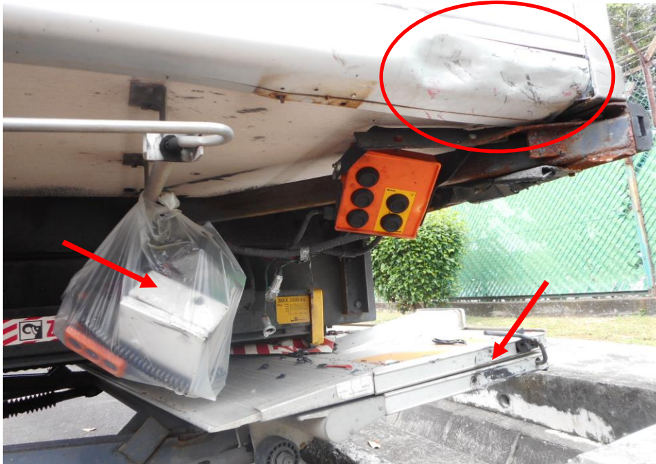
Photo 4 shows a close up view of the left body of the Motor Lorry at the time of my inspection. The Motor Lorry was observed to have sustained damage at its left side body panel (circled) and rear tailgate (arrowed) as a result of the accident.
