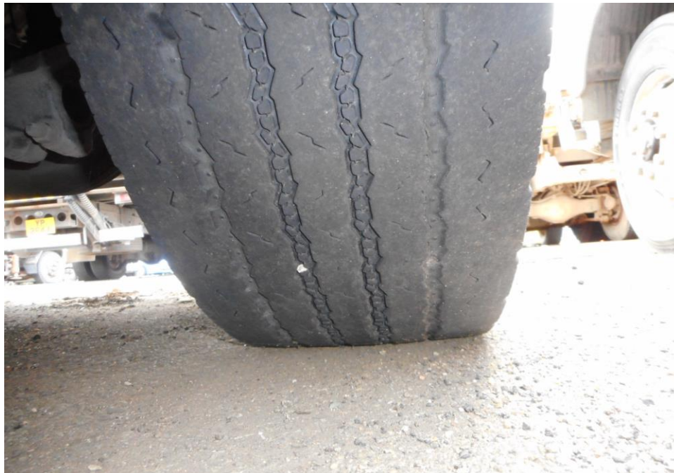
Photo 7 shows the condition of the front right tyre of the Motor Lorry, which was observed to be in serviceable condition with remaining tread depth of approximately 3.8mm. The tyre, which was wrapped around standard steel wheel rim, was also observed to be sufficiently inflated for vehicular operation. There was no tear, cut or burst mark(s) on the outer and the inner sidewalls as well as across the tread of the 6 tyres that were fitted on the Motor Lorry.
