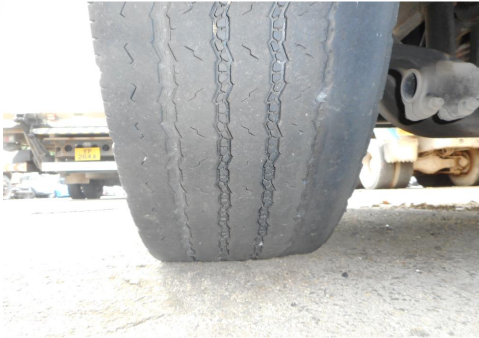
Photo 10 shows the condition of the front left tyre of the Motor Lorry, which were observed to be in serviceable condition with remaining, tread depth of approximately 4.3mm. There was also no tear, cut or burst mark(s) on the outer and the inner sidewalls as well as across the tread of the 6 tyres that were fitted on the Motor Lorry.
