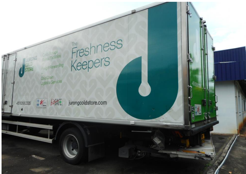
Photo 3 shows a general view of the left body of the Motor Lorry at the time of my inspection. The Motor Lorry was observed to have sustained damage at its left side body panel and rear tailgate as a result of the accident.
