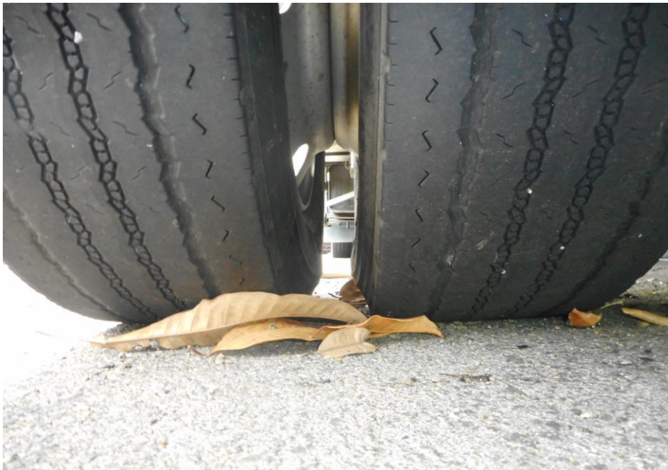
Photo 9 the condition of the rear left tyres of the Motor Lorry, which was observed to be in serviceable condition with remaining, tread depth of approximately 3.7mm. The tyres, which were wrapped around standard steel wheel rim, were also observed to be sufficiently inflated for vehicular operation. There was also no damage found on all 6 steel wheel rims of the Motor Lorry.
