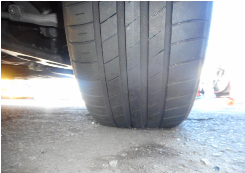
Photo 6 shows the condition of the front right tyre of the Motor Car, which was observed to be in serviceable condition with remaining tread depth of approximately 5.5mm. The tyre, which was wrapped around standard alloy wheel rim, was also observed to be sufficiently inflated for vehicular operation. There was no tear, cut or burst mark(s) on the outer and the inner sidewalls as well as across the tread of the 4 tyres that were fitted on the Motor Car.
