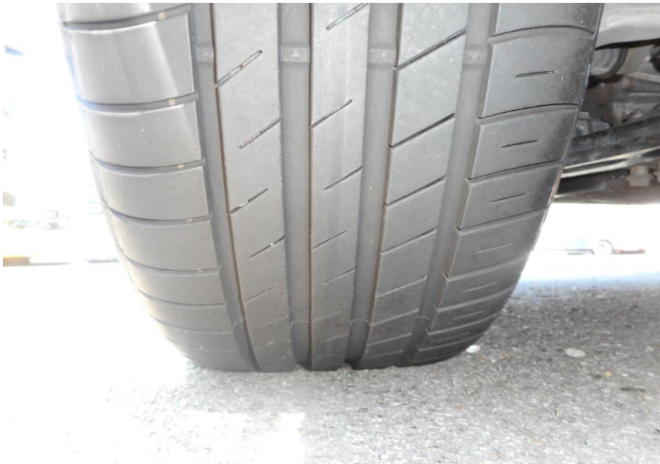
Photo 9 shows the condition of the rear right tyres of the Motor Car, which were observed to be in serviceable condition with remaining, tread depth of approximately 5.4mm. There was also no tear, cut or burst mark(s) on the outer and the inner sidewalls as well as across the tread of the 4 tyres that were fitted on the Motor Car.
