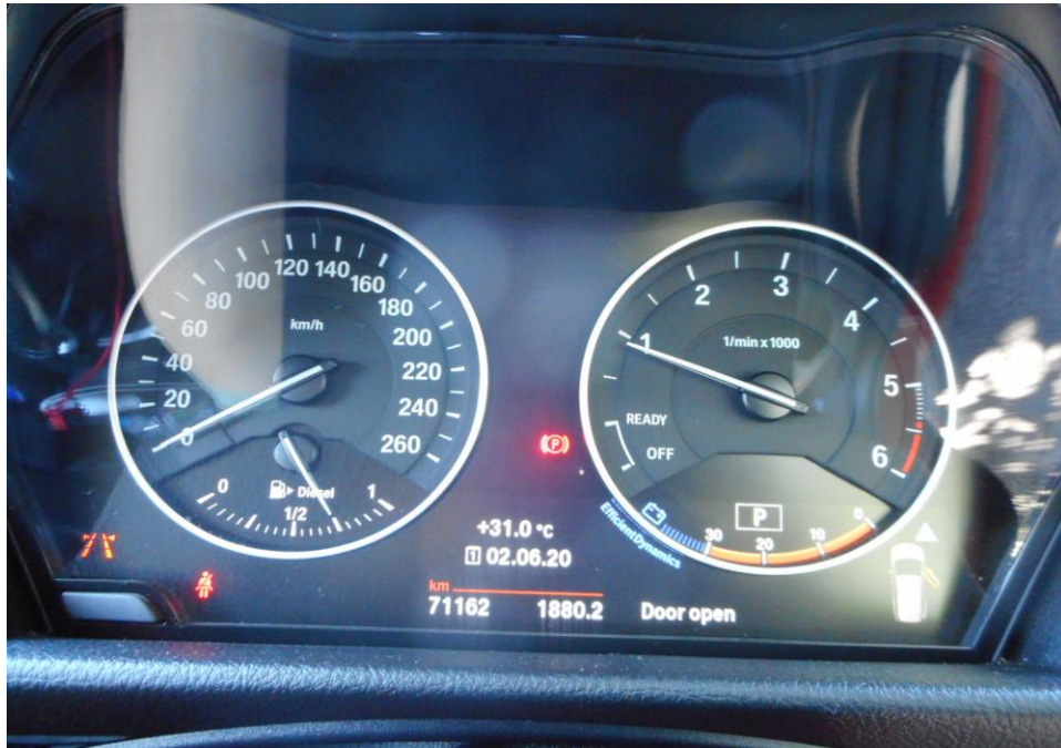
Photo 23 shows no warning lights illuminated on the instrument panel of the Motor Car after the engine was cranked. This would suggest that there was no abnormality to the various electronic operating systems of the Motor Car, like the ABS, TC, SRS and EPS.
