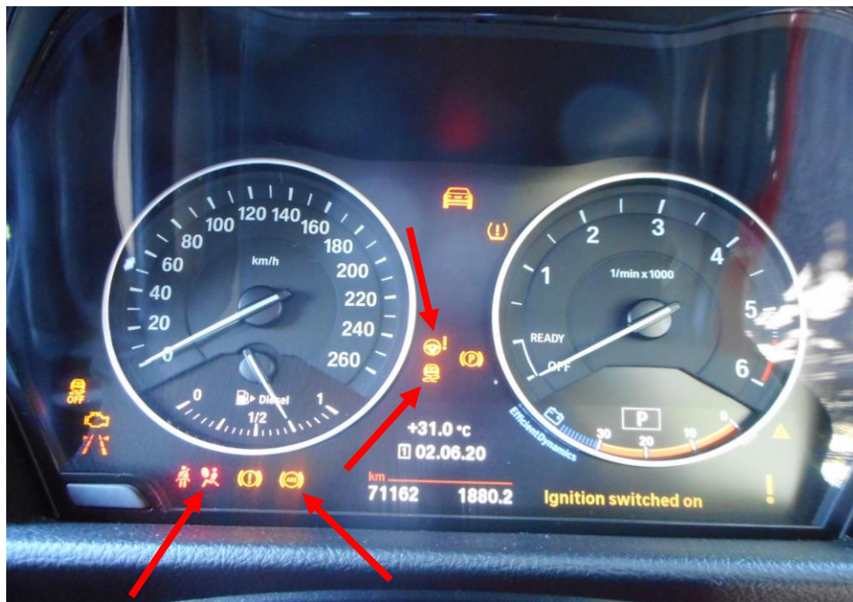
Photo 22 shows the warning light for Anti-Lock Brake System (ABS), Traction Control (TC), Supplemental Restraint System (SRS) and Electric Power Steering System (EPS) appearing on the instrument panel of the Motor Car during the self-test of its various electronic operating systems when its engine was cranked.
