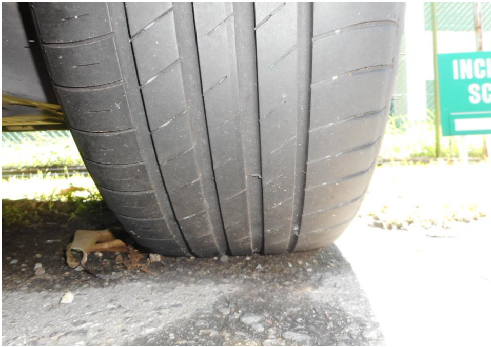
Photo 8 shows the condition of the rear left tyres of the Motor Car, which was observed to be in serviceable condition with remaining tread depth of approximately 4.4mm. The tyres, which were wrapped around standard alloy wheel rim, were also observed to be sufficiently inflated for vehicular operation. There was also no damage found on all 4 alloy wheel rims of the Motor Car.
