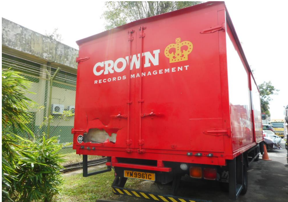
Photo 3 shows a general view of the rear body of the Motor Lorry at the time of my inspection. The Motor Lorry was observed to have sustained damage at its rear portion. Its rear left door panel, rear guard rail and rear left brake lamp was damaged as a result of the accident.
