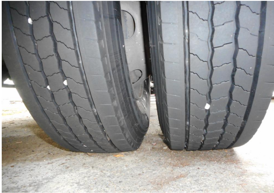
Photo 8 shows the condition of the rear right tyres of the Motor Lorry, which was observed to be in serviceable condition with remaining, tread depth of approximately 10.8mm. The tyres, which were wrapped around standard steel wheel rim, were also observed to be sufficiently inflated for vehicular operation. There was also no damage found on all 6 steel wheel rims of the Motor Lorry.
