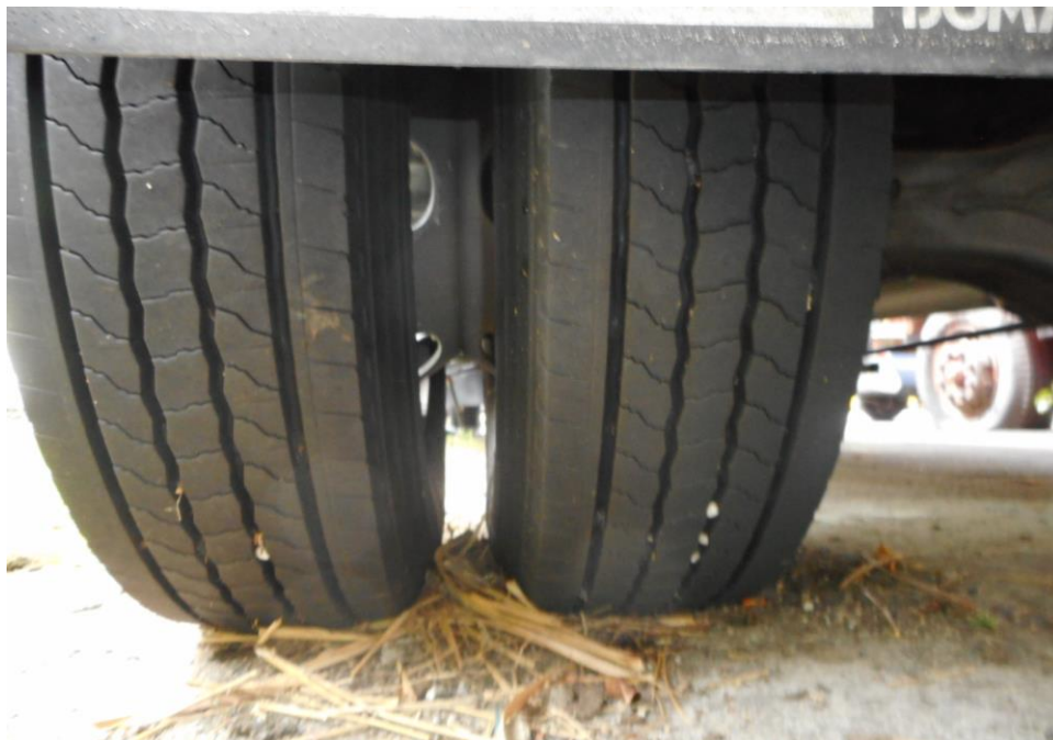
Photo 9 the condition of the rear left tyres of the Motor Lorry, which was observed to be in serviceable condition with remaining, tread depth of approximately 10.9mm. The tyres, which were wrapped around standard steel wheel rim, were also observed to be sufficiently inflated for vehicular operation. There was also no damage found on all 6 steel wheel rims of the Motor Lorry.
