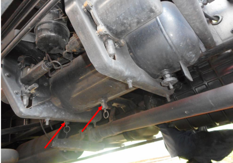
Photo 22 shows the air brake cylinders (arrowed) at the undercarriage of the Motor Lorry. I did not observe any leakage of air brake fluid at the time of my inspection of the Motor Lorry. My static tests of the Motor Lorry's braking system, along with my visual examination of the various mechanical components in the braking system had indicated that there was no internal leakage of pressure/vacuum. Hence the braking system of the Motor Lorry was likely to be in serviceable condition at the material time of accident.
