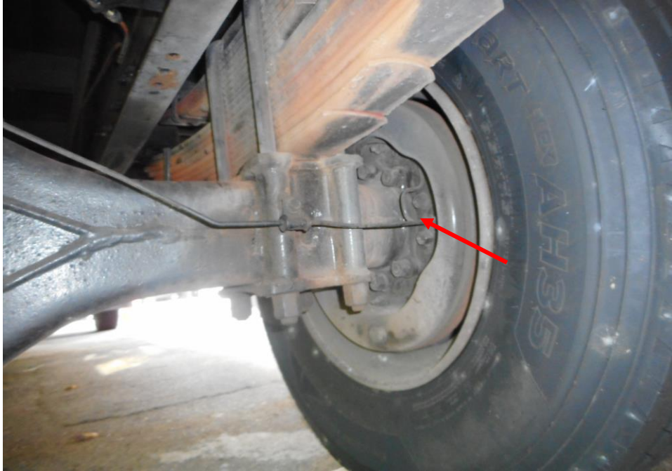
Photo 20 shows the brake pipe (arrowed) at the rear right wheel of the Motor Lorry. I did not observe any leakage of brake fluid at the time of my inspection of the Motor Lorry. My static tests of the Motor Lorry's braking system, along with my visual examination of the various mechanical components in the braking system, had indicated that there was no internal leakage of pressure/vacuum. Hence the braking system of the Motor Lorry was likely to be in serviceable condition at the material time of accident.
