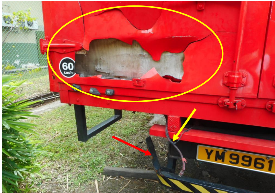
Photo 4 shows a close up view of the left body of the Motor Lorry at the time of my inspection. The Motor Lorry was observed to have sustained damage at its rear portion. Its rear left door panel (circled), rear guard rail (red arrow) and rear left brake lamp (yellow arrowed) was damaged as a result of the accident.
