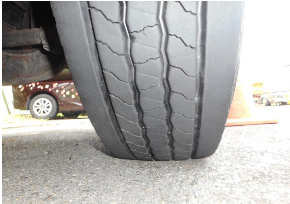
Photo 7 shows the condition of the front right tyre of the Motor Lorry, which was observed to be in serviceable condition with remaining tread depth of approximately 11.8mm. The tyre, which was wrapped around standard steel wheel rim, was also observed to be sufficiently inflated for vehicular operation. There was no tear, cut or burst mark(s) on the outer and the inner sidewalls as well as across the tread of the 6 tyres that were fitted on the Motor Lorry.
