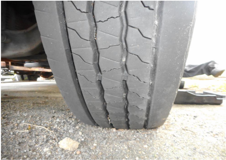
Photo 10 shows the condition of the front left tyre of the Motor Lorry, which were observed to be in serviceable condition with remaining, tread depth of approximately 11.8mm. There was also no tear, cut or burst mark(s) on the outer and the inner sidewalls as well as across the tread of the 6 tyres that were fitted on the Motor Lorry.
