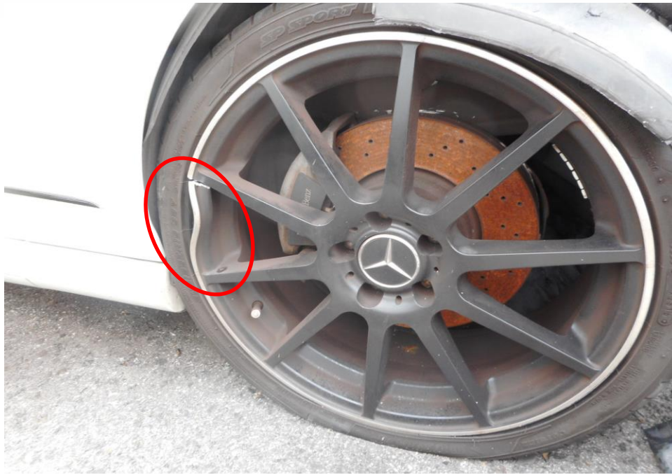
Photo 9 shows the condition of the front right tyre of the Motor Car, which was observed to be in unserviceable condition with deflated tyre which was a result of the damaged rim (circled) as a result of the accident. The remaining tread depth was approximately 5.7mm.
