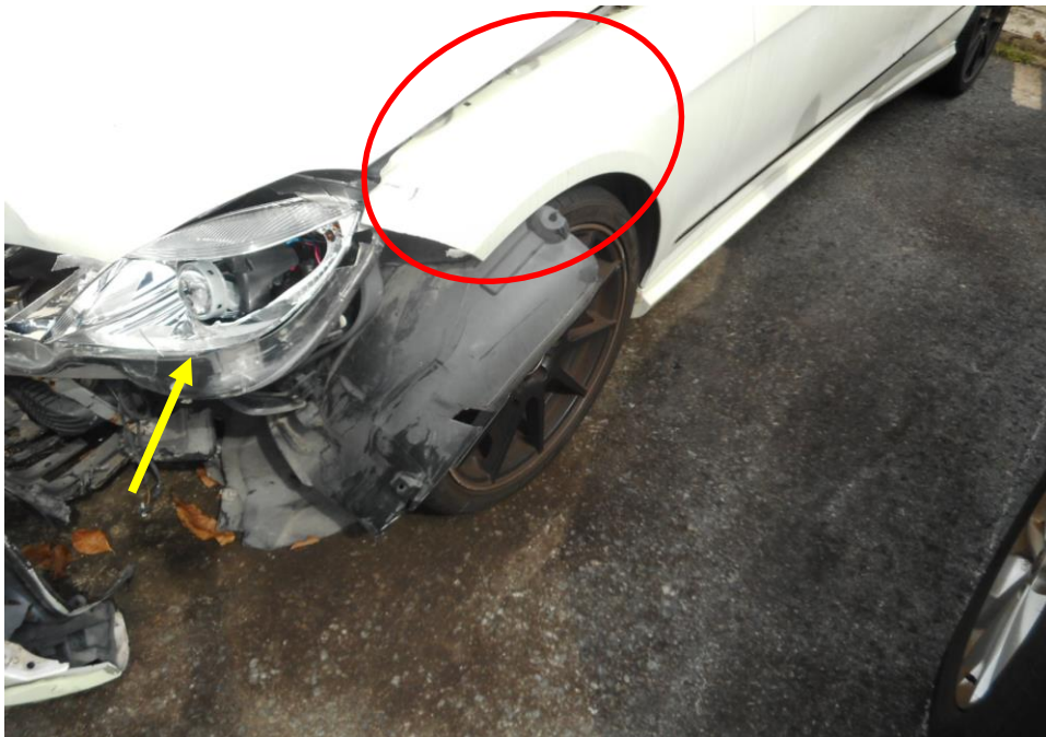
Photo 8 shows a close up view of the Motor Car's engine compartment at the time of my inspection. The Motor car was observed to have sustained damage at its left portion. Its front left fender (red circle) and front left headlamp (yellow arrow) was damaged as a result of the accident.
