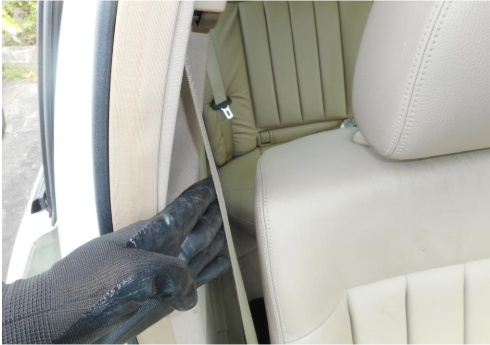
Photo 24 shows that the seat belt on the right seat was unworn at the material time of accident as the safety pre-tensioners was activated at the moment of impact and caused the seat belts to be locked into the last position.
