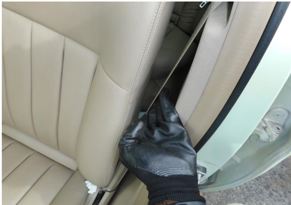
Photo 23 shows that the seat belt on the left seat was unworn at the material time of accident as the safety pre-tensioners was activated at the moment of impact and caused the seat belts to be locked into the last position.
