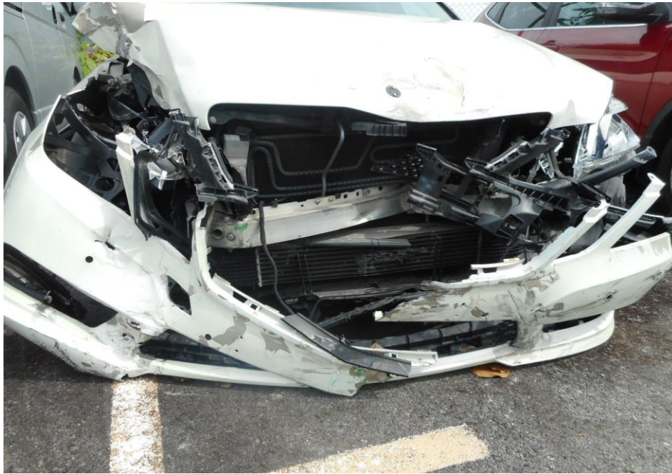
Photo 5 shows the close up view of the Motor Car's front body at the time of my inspection. The Motor car was observed to have sustained damage at its front portion. Its front bumper, front left and right fender, front left and right headlamp was amongst the body parts and various components in the engine compartments were also damaged as a result of the accident.
