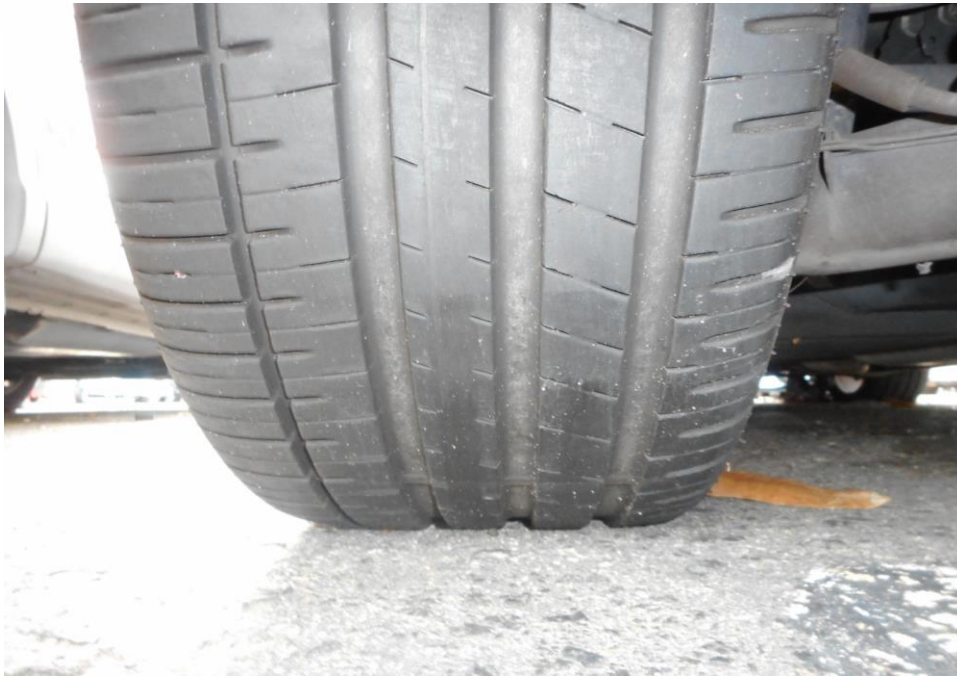
Photo 11 shows the condition of the rear left tyre of the Motor Car, which was observed to be in serviceable condition with remaining tread depth of approximately 5.9mm. The tyre was also observed to be sufficiently inflated for vehicular operation with no tear, cut or burst mark(s).
