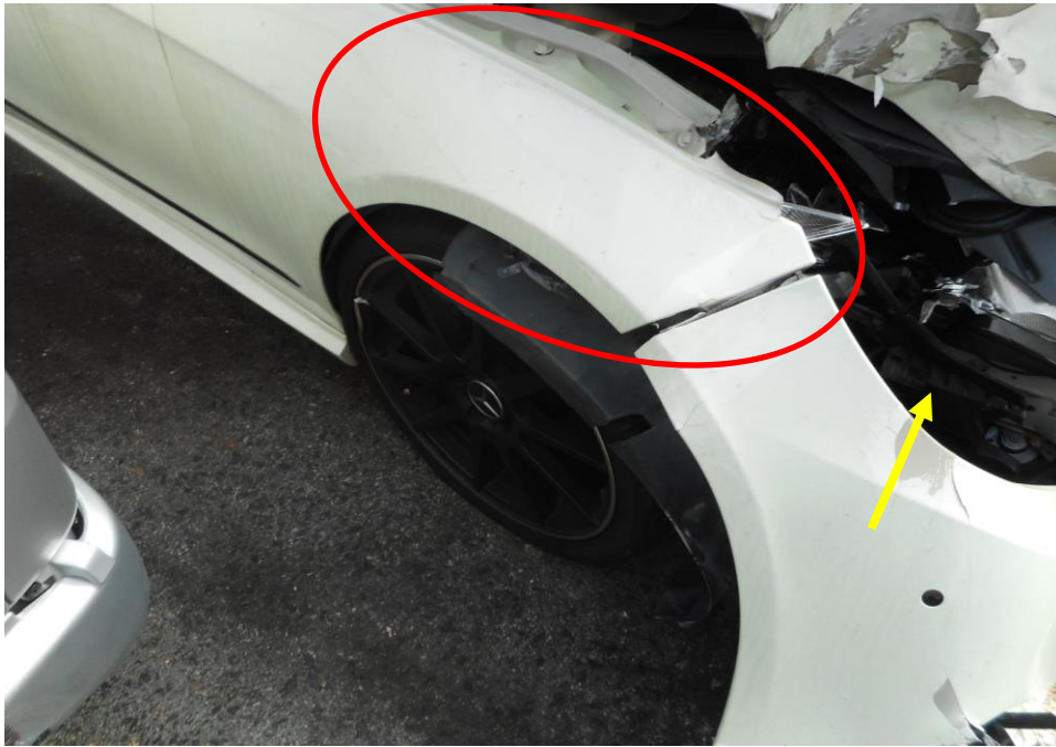
Photo 7 shows a close up view of the Motor Car's engine compartment at the time of my inspection. The Motor car was observed to have sustained damage at its right portion. Its front right fender (red circle) and front right headlamp (yellow arrow) was damaged as a result of the accident.
