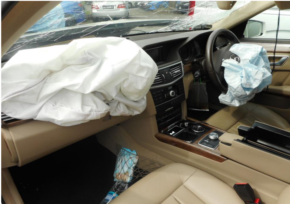
Photo 13 shows the deployment of the Supplemental Restraint System (SRS) airbag (arrowed) in the Motor Car as a result of the accident.
