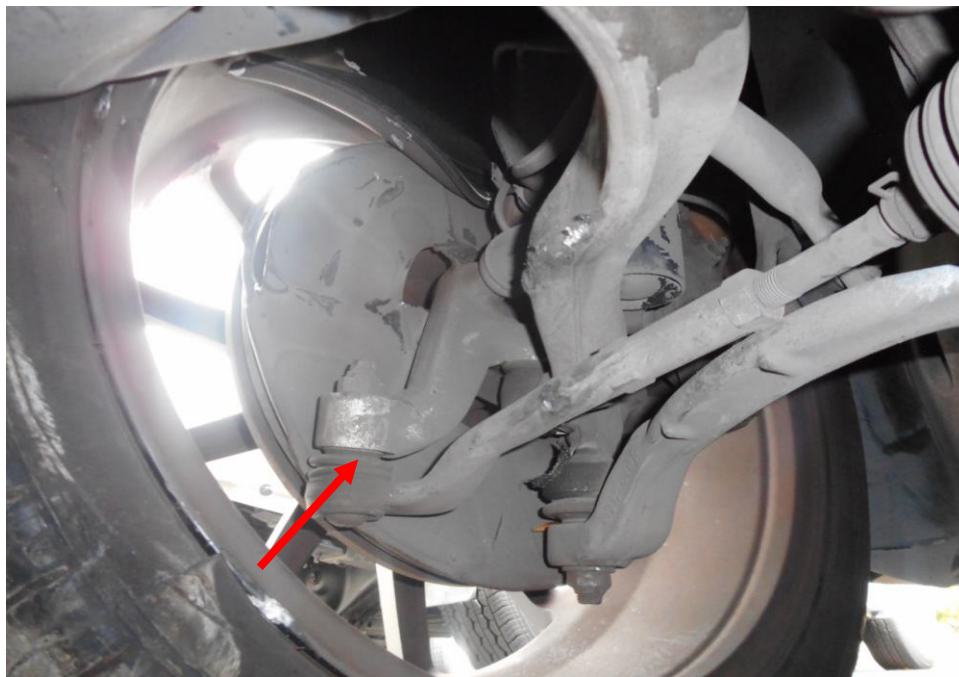
Photo 20 shows the various undercarriage components at the front right wheel of the Motor Car, in particular the steering tie rod end (arrowed). The various steering components were all found to be intact, suggesting that the steering system of the Motor Car was likely to be in serviceable condition at the material time of accident. There was also no sign of fluid stain(s) observed on the various undercarriage components.
