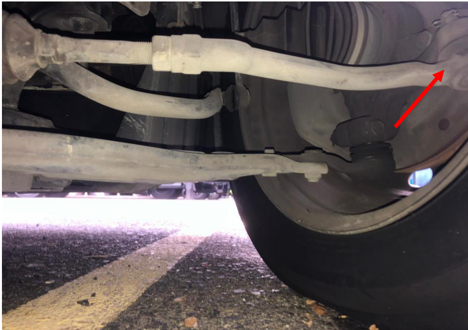
Photo 20 shows the various undercarriage components at the front right wheel of the Motor Taxi, in particular the steering tie rod (red arrow) and drive shaft (yellow arrow). The various steering components were all found to be intact, suggesting that the steering system of the Motor Taxi was likely to be in serviceable condition at the material time of accident. There was also no sign of fluid stain observed on the various undercarriage components at the front right wheel of the Motor Taxi.
