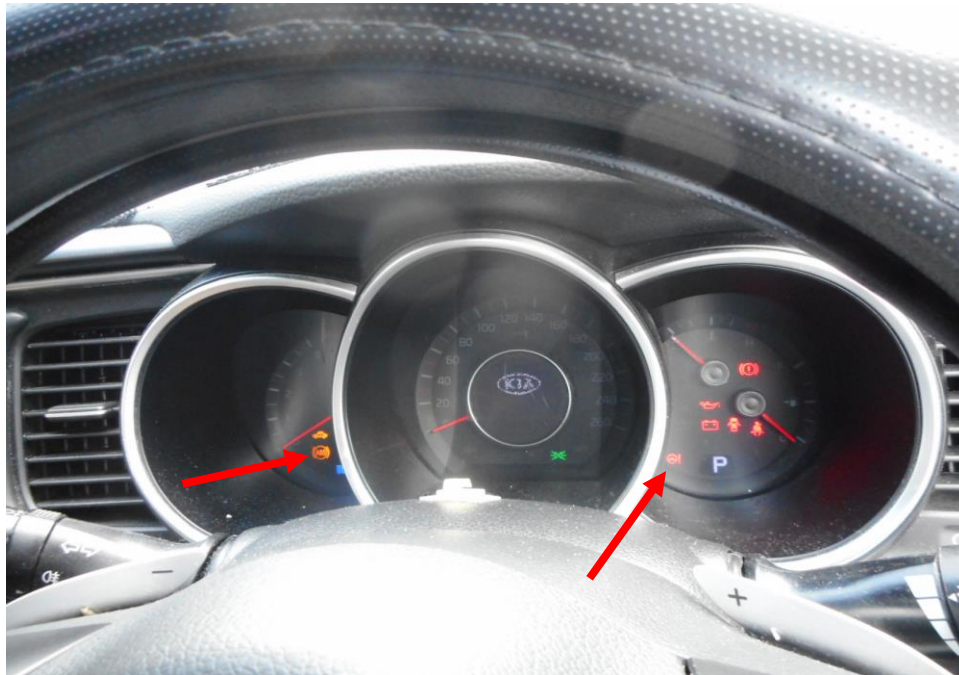
Photo 22 shows the warning light for Anti-Lock Brake System (ABS) and Power Steering System (EPS) (arrowed) appearing on the instrument panel of the Motor Taxi during the self-test of its various electronic operating systems when its engine was cranked.
