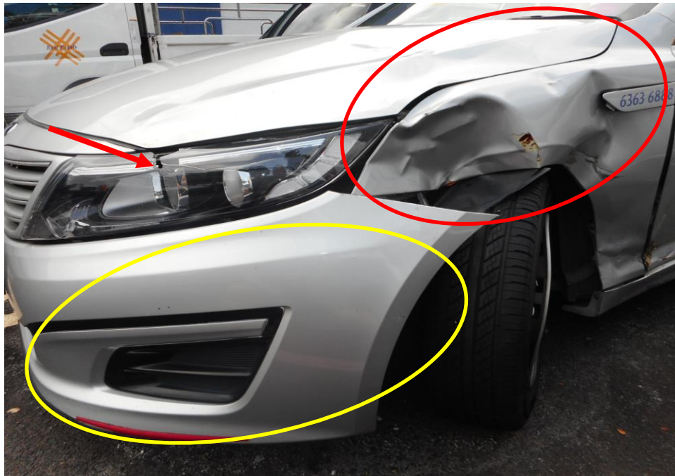
Photo 4 shows the close up view of the Motor Taxi's front left body at the time of my inspection. The Motor Taxi was observed to have sustained damage at its front left headlamp (arrowed) front left fender (red circle) and front bumper (yellow circle) as a result of the accident.
