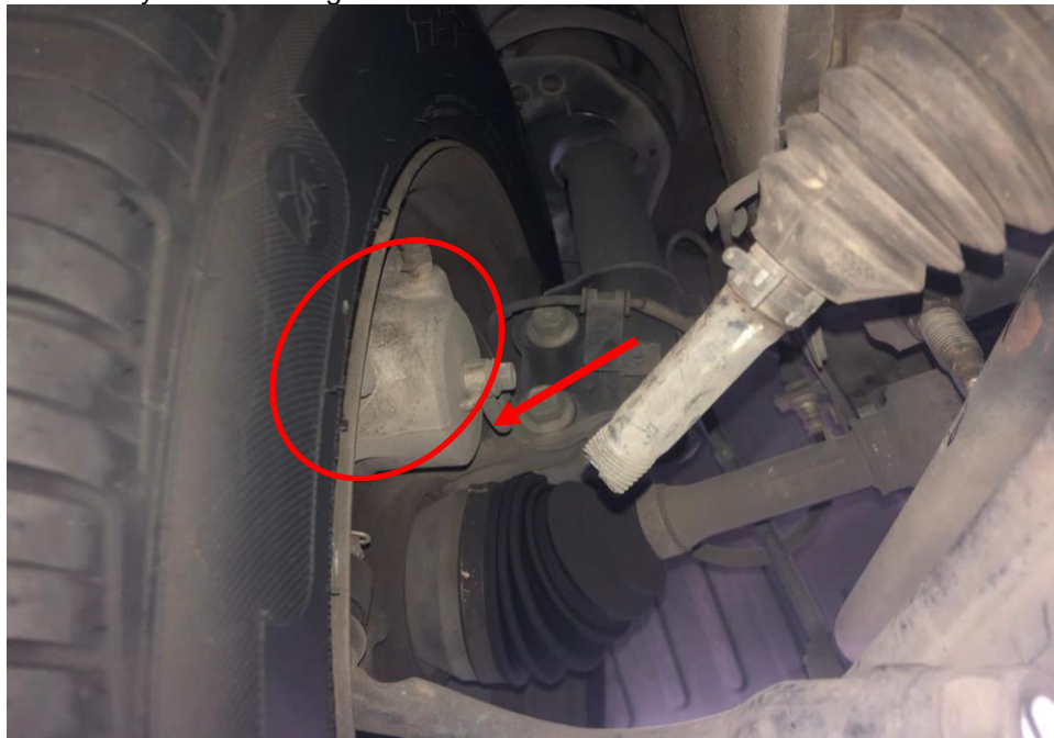
Photo 19 shows the brake hose/pipe (arrowed) at the front left wheel of the Motor Taxi. No leakage of brake fluid was observed. Visual examination of the various components of the braking system like the brake caliper (circled), brake booster, brake pedal etc had revealed all to be intact and without visible damage.
