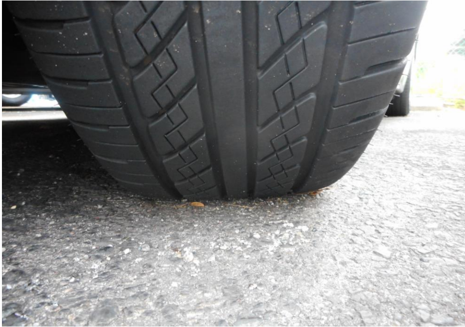
Photo 10 shows the condition of the front left tyre of the Motor Taxi, which was observed to be in serviceable condition with remaining tread depth of approximately 5mm. There was also no tear, cut or burst mark(s) on the outer and the inner sidewalls as well as across the tread of the Motor Taxi's 4 tyres.
