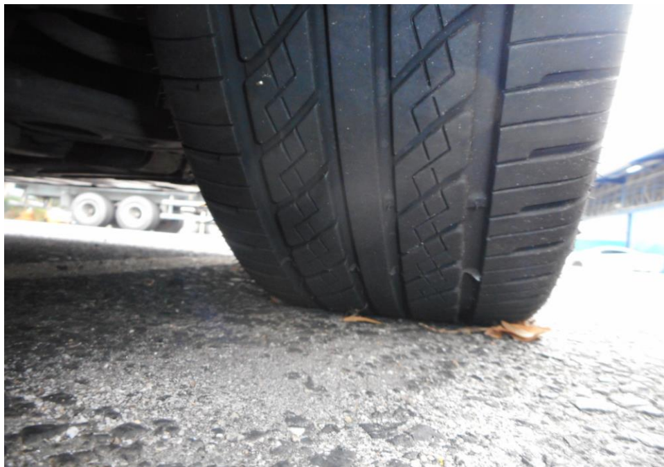
Photo 7 shows the condition of the front right tyre of the Motor Taxi, which was observed to be in serviceable condition with remaining tread depth of approximately 5.4mm. The tyre was sufficiently inflated for vehicular operation with no tear, cut or burst mark(s) on the outer and the inner sidewalls as well as across the tread. The 4 tyres of the Motor Taxi were wrapped around standard steel wheel rims without any damage.
