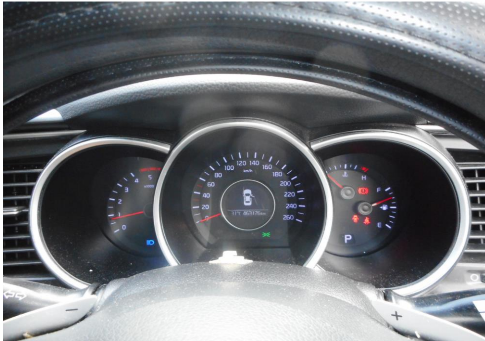
Photo 23 shows no warning lights illuminated on the instrument panel of the Motor Taxi after the engine was cranked. This would suggest that there was no abnormality to the electronic operating system of the Motor Taxi, like the ABS and EPS etc.
