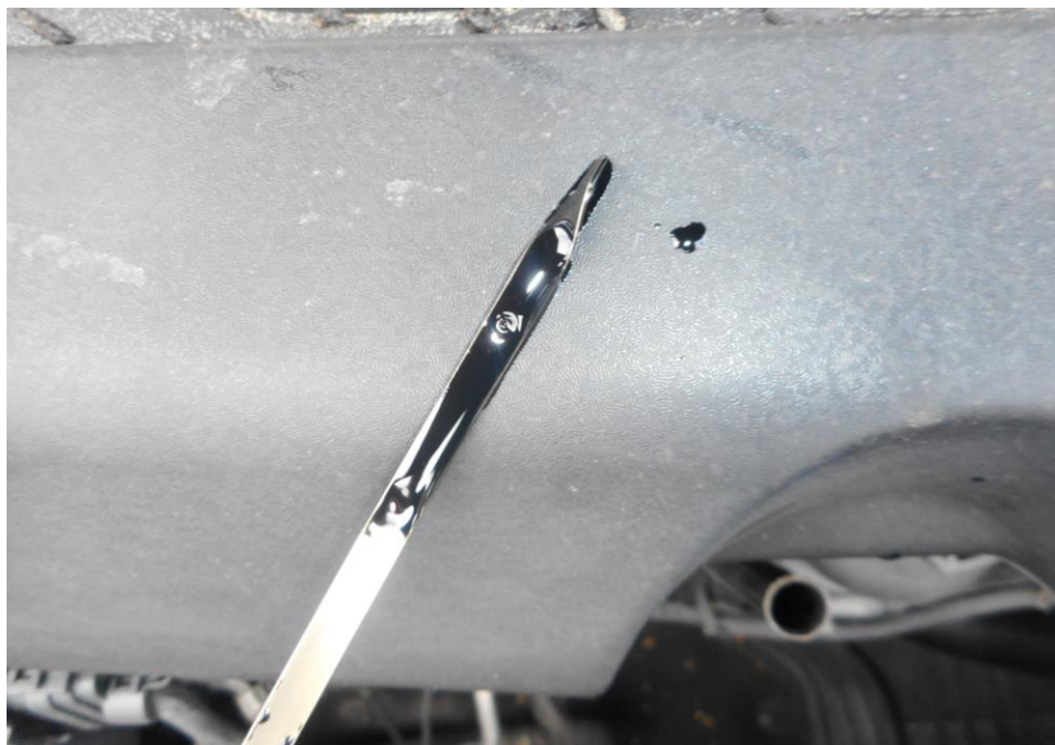
Photo 14 shows the engine oil dip stick of the Motor Taxi at the time of my inspection. The engine oil was observed to be of sufficient level and without any visible contamination.
