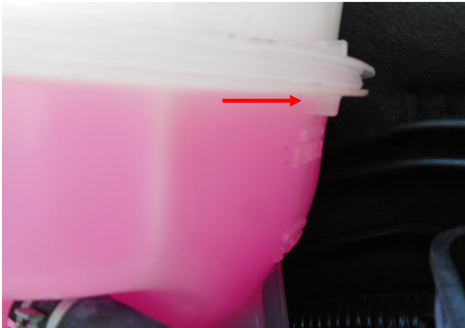
Photo 14 shows the engine coolant reservoir of the Mini Bus at the time of my inspection. The engine coolant was observed to be of sufficient level and without any visible contamination.
