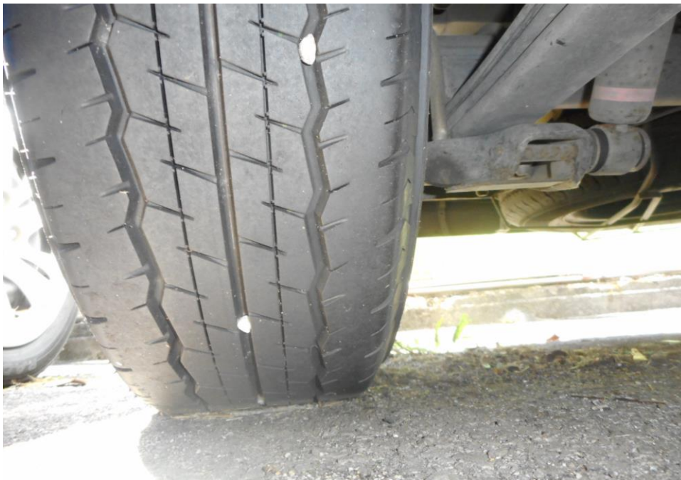
Photo 9 shows the condition of the rear right tyre of the Mini Bus, which was observed to be in serviceable condition with remaining tread depth of approximately 7.2mm. The tyre, which was wrapped around standard steel wheel rim, it was observed to be sufficiently inflated for vehicular operation.
