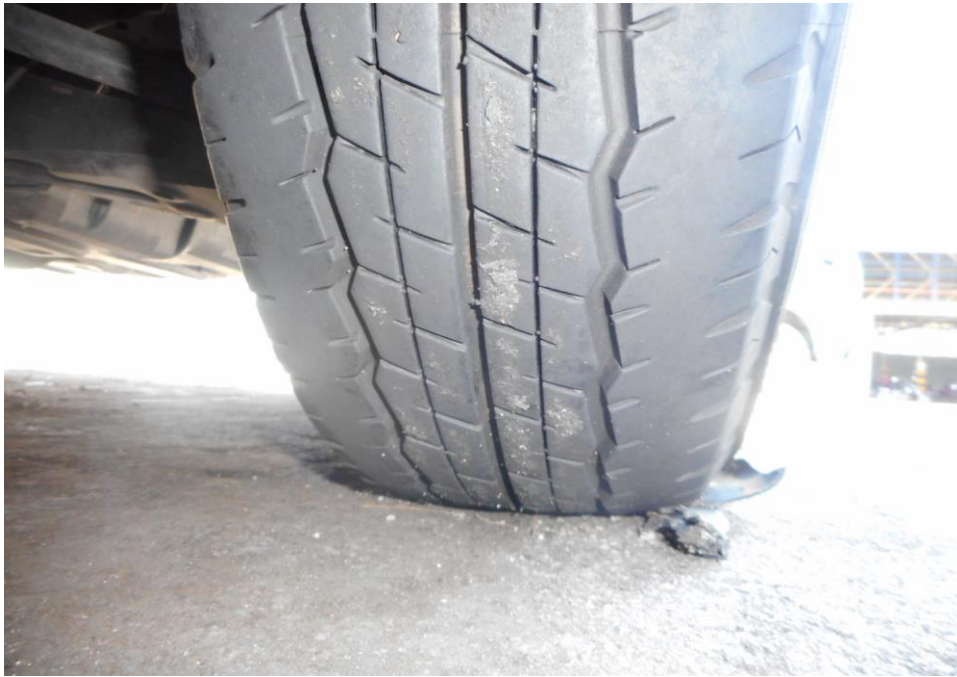
Photo 8 shows the condition of the front right tyre of the Mini Bus, which was observed to be in serviceable condition with remaining tread depth of approximately 7.9mm. The tyre, which was wrapped around standard steel wheel rim, was also observed to be sufficiently inflated for vehicular operation. There was no tear, cut or burst mark(s) on the outer and the inner sidewalls as well as across the tread of the 4 tyres that were fitted on the Mini Bus.
