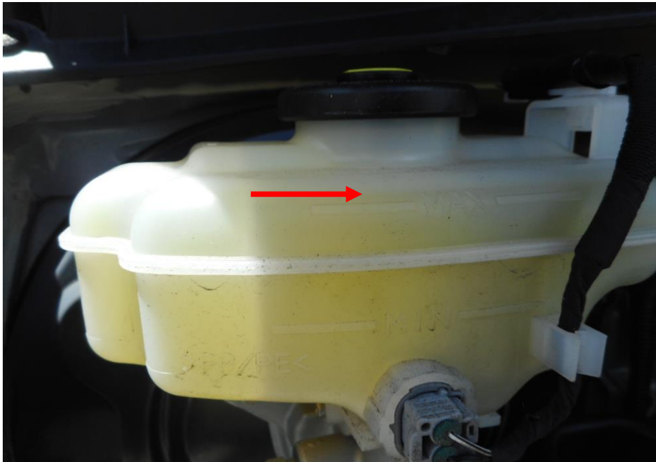
Photo 13 shows the brake fluid reservoir of the Mini Bus at the time of my inspection. The brake fluid was observed to be of sufficient level (arrowed) and without any visible contamination.
