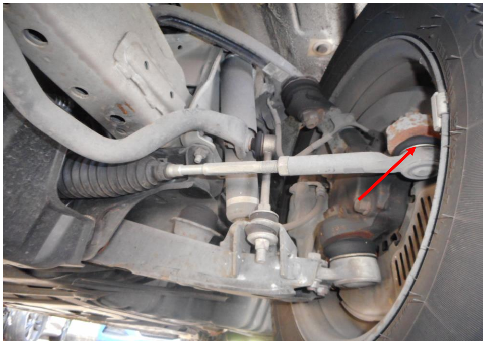
Photo 19 shows the various undercarriage components at the front left wheel of the Mini Bus, in particular the steering tie rod end (arrowed). The various undercarriage components of the Mini Bus were all found to be intact without any visible damage. There was also no sign of fluid stain(s) observed on the various undercarriage components.
