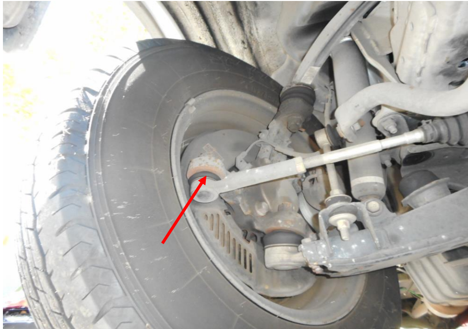
Photo 18 shows the various undercarriage components at the front right wheel of the Mini Bus, in particular the steering tie rod end (arrowed). The various steering components were all found to be intact, suggesting that the steering system of the Mini Bus was likely to be in serviceable condition at the material time of accident. There was also no sign of fluid stain(s) observed on the various undercarriage components.
