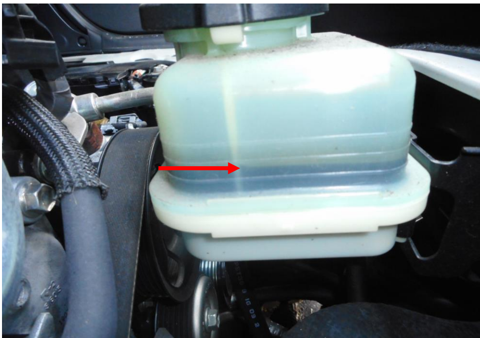
Photo 16 shows the power steering fluid of the Mini Bus at the time of my inspection. The power steering fluid was observed to be of sufficient level (arrowed) and without any visible contamination.
