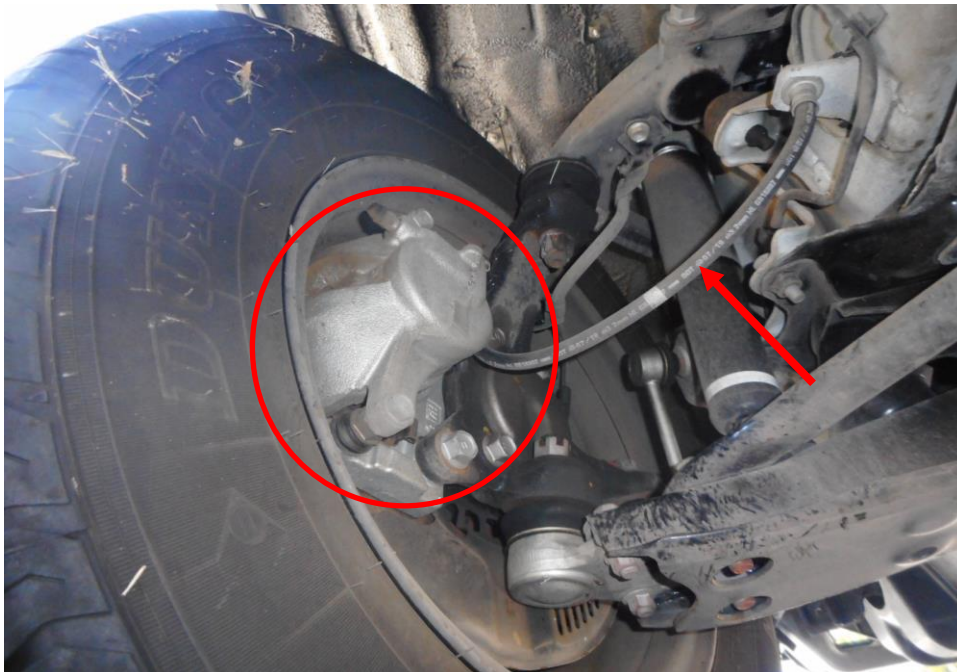
Photo 23 shows the brake hose/pipe (arrowed) at the front left wheel of the Mini Bus. No leakage of brake fluid was observed. Visual examination of the various components of the braking system like the brake caliper (circled), brake booster, brake pedal etc had revealed all to be intact and without visible damage at the time of accident. There was also no sign of fluid stain(s) observed on the various undercarriage components.
