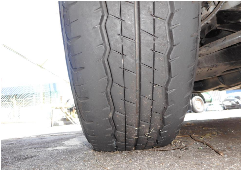
Photo 11 shows the condition of the rear right tyres of the Mini Bus, which were observed to be in serviceable condition with remaining, tread depth of approximately 7.6mm. There was also no tear, cut or burst mark(s) on the outer and the inner sidewalls as well as across the tread of the 4 tyres that were fitted on the Mini Bus.
