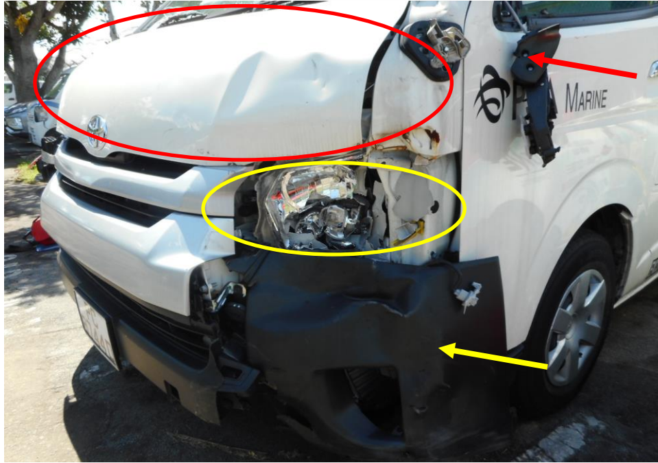
Photo 4 shows a close up view of the Mini Bus's frontal portion at the time of my inspection. It appeared to have sustained damage at its frontal portion. Its front bonnet (red circle), front bumper (yellow arrow), left rear view mirror (red arrow) and front left head lamp (yellow circle) were damage at the time of my inspection.
