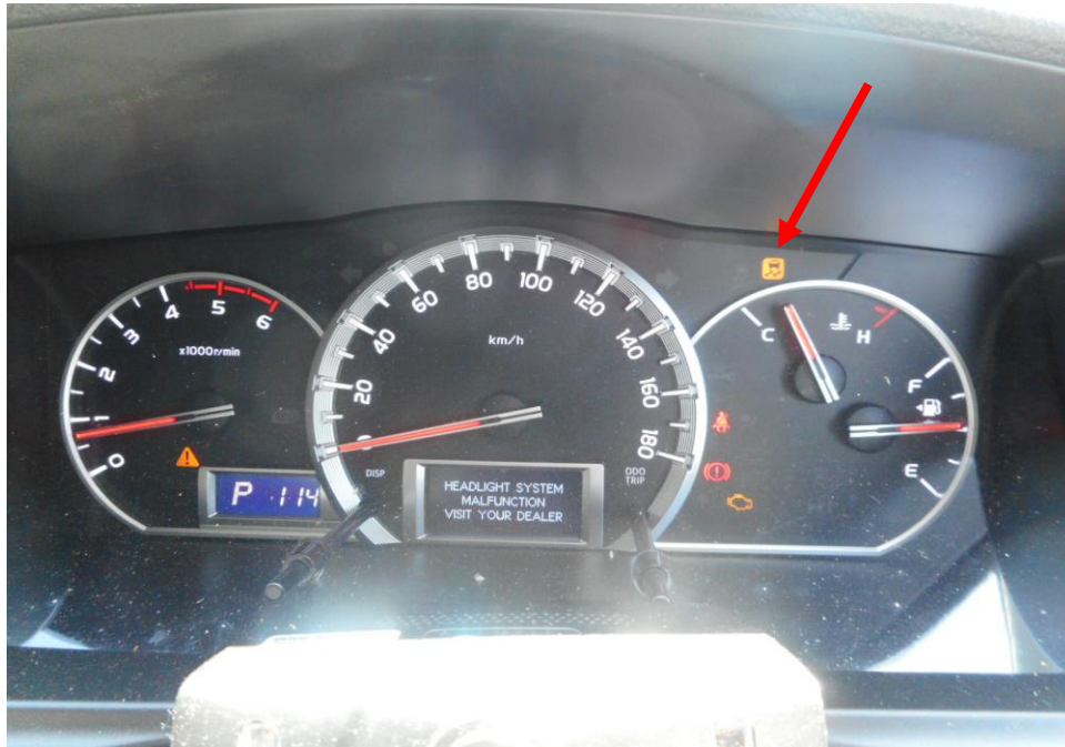
Photo 25 shows no warning lights illuminated on the instrument panel of the Mini Bus after the engine was cranked. This would suggest that there was no abnormality to the electronic operating system of the Mini Bus, like the ABS and SRS etc. However the Traction Control System (TC) light remained illuminated on likely caused by the result of the accident.
