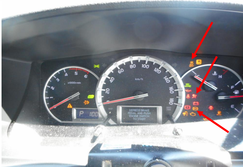
Photo 24 shows the warning light for Anti-Lock Brake System (ABS) and Supplemental Restraint System (SRS) and Traction Control System (TC) (arrowed) appearing on the instrument panel of the Mini Bus during the self-test of its various electronic operating systems when its engine was cranked.
