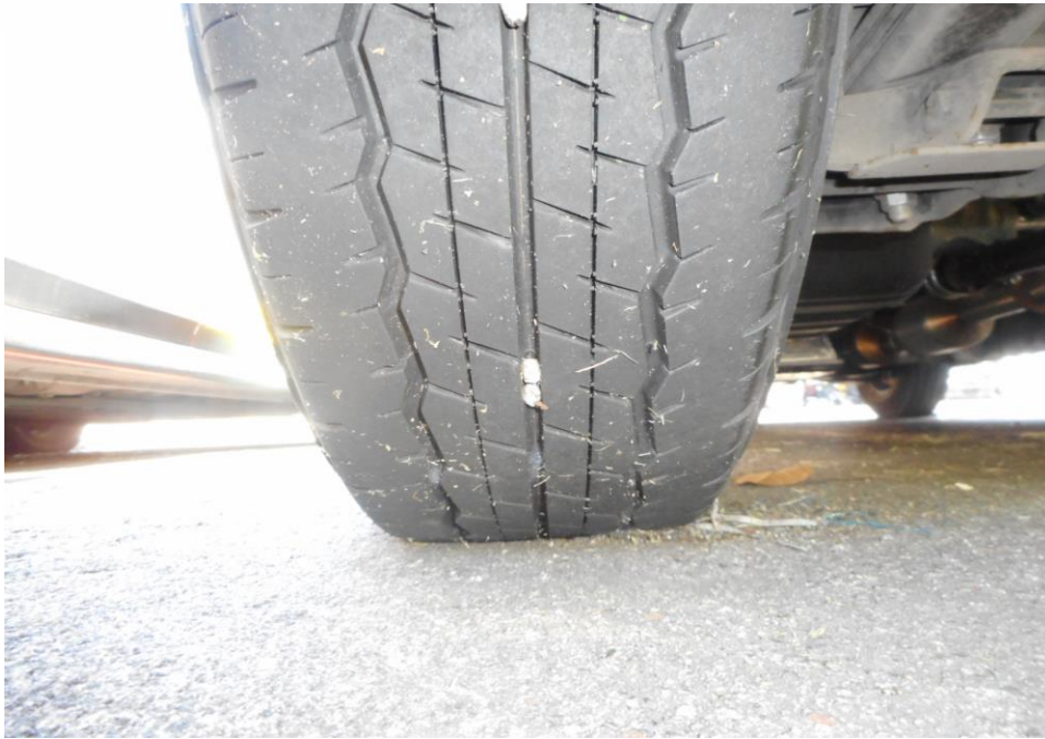
Photo 10 shows the condition of the rear left tyres of the Mini Bus, which was observed to be in serviceable condition with remaining tread depth of approximately 7mm. The tyres, which were wrapped around standard steel wheel rim, were also observed to be sufficiently inflated for vehicular operation. There was also no damage found on all 4 steel wheel rims of the Mini Bus.
