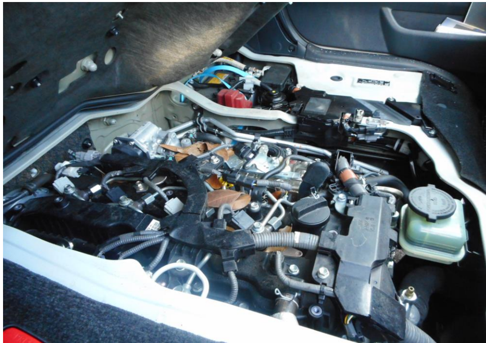
Photo 12 shows a general view of the Mini Bus's engine compartment, which was accessed by lifting the front cabin of the Mini Bus. The various parts and components inside the engine compartment were unaffected by the accident. There was also no sign(s) or indication(s) of fresh fluid leakage and/or fluid stain within the engine compartment
