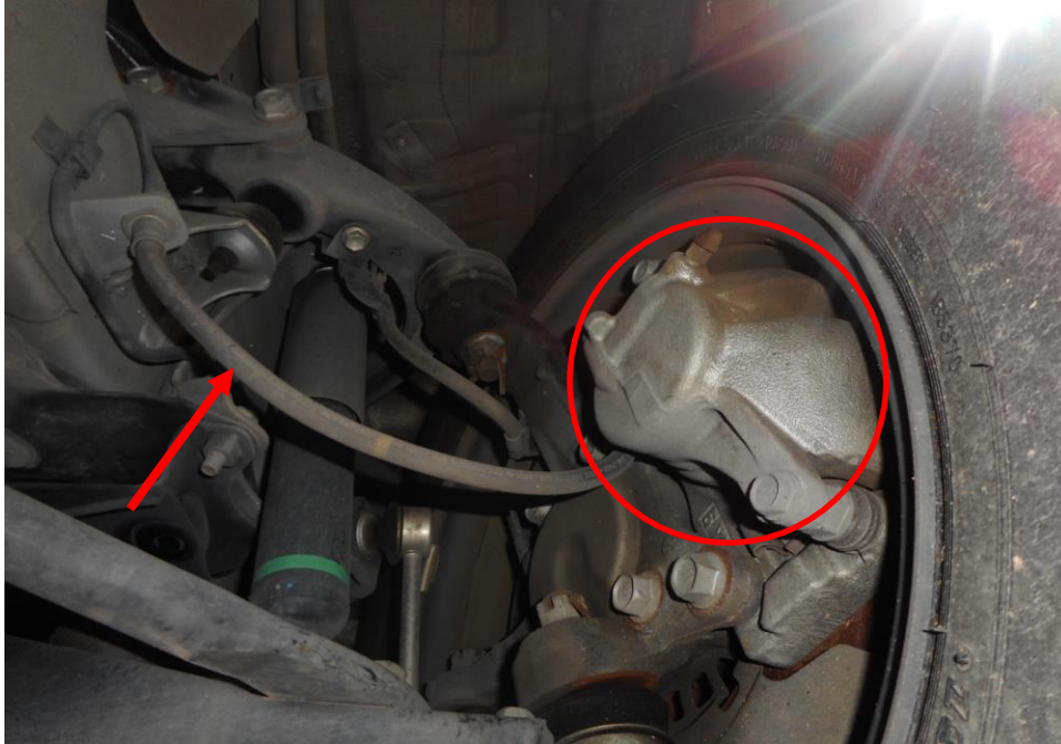
Photo 21 shows the brake hose/pipe (arrowed) at the front right wheel of the Mini Bus. No leakage of brake fluid was observed. Visual examination of the various components of the braking system like the brake caliper (circled), brake booster, brake pedal etc had revealed all to be intact and without visible damage at the time of accident. There was also no sign of fluid stain(s) observed on the various undercarriage components.
