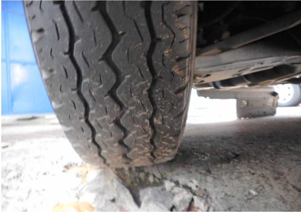
Photo 10 shows the condition of the rear right tyres of the Mini Bus, which were observed to be in serviceable condition with remaining, tread depth of approximately 5.7mm. There was also no tear, cut or burst mark(s) on the outer and the inner sidewalls as well as across the tread of the 4 tyres that were fitted on the Mini Bus.
