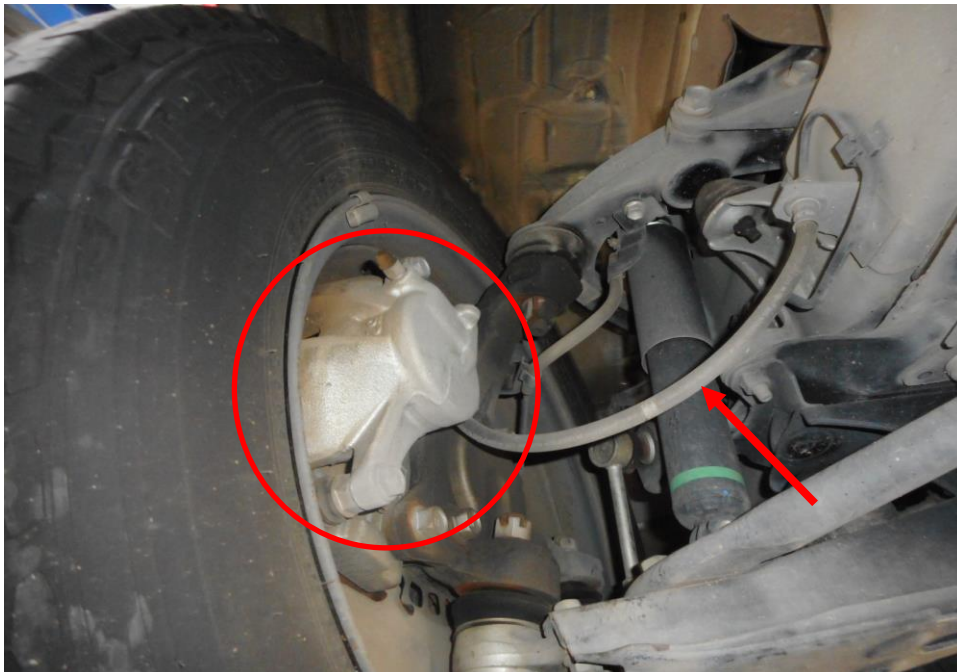
Photo 22 shows the brake hose/pipe (arrowed) at the front left wheel of the Mini Bus. No leakage of brake fluid was observed. Visual examination of the various components of the braking system like the brake caliper (circled), brake booster, brake pedal etc had revealed all to be intact and without visible damage at the time of accident. There was also no sign of fluid stain(s) observed on the various undercarriage components.
