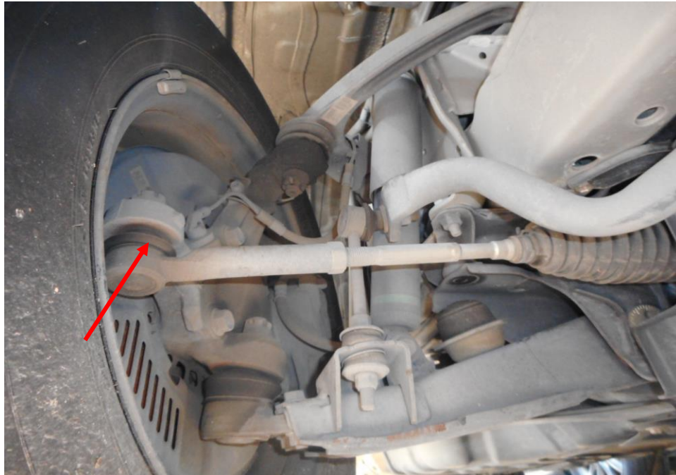
Photo 17 shows the various undercarriage components at the front right wheel of the Mini Bus, in particular the steering tie rod end (arrowed). The various steering components were all found to be intact, suggesting that the steering system of the Mini Bus was likely to be in serviceable condition at the material time of accident. There was also no sign of fluid stain(s) observed on the various undercarriage components.
