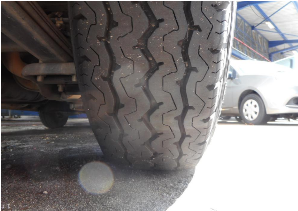
Photo 8 shows the condition of the rear right tyre of the Mini Bus, which was observed to be in serviceable condition with remaining tread depth of approximately 6mm. The tyre, which was wrapped around standard steel wheel rim, it was observed to be sufficiently inflated for vehicular operation.
