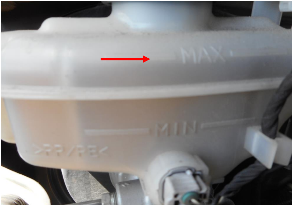
Photo 12 shows the brake fluid reservoir of the Mini Bus at the time of my inspection. The brake fluid was observed to be of sufficient level (arrowed) and without any visible contamination.
