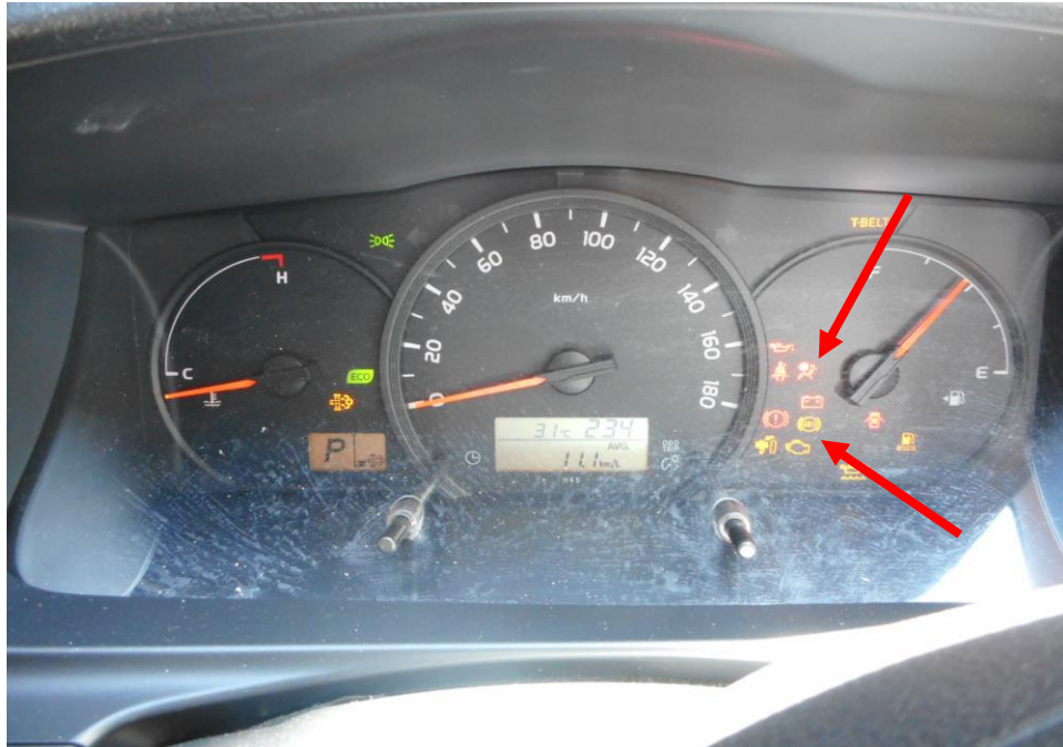
Photo 24 shows the warning light for Anti-Lock Brake System (ABS) and Supplemental Restraint System (SRS) (arrowed) appearing on the instrument panel of the Mini Bus during the self-test of its various electronic operating systems when its engine was cranked.
