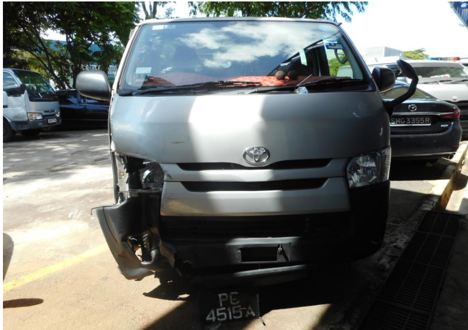
Photo 2 shows a general view of the Mini Bus's frontal portion at the time of my inspection. It appeared to have sustained damage at its frontal portion. Its front bumper, front bonnet and front right head lamp were damage at the time of my inspection.
