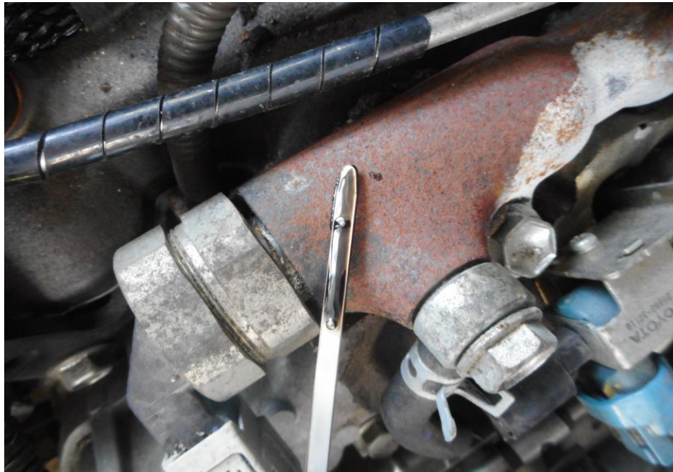
Photo 14 shows the engine oil dip stick of the Mini Bus at the time of my inspection. The engine oil was observed to be of sufficient level and without any visible contamination.
