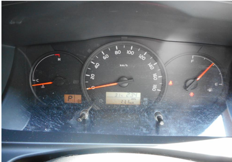
Photo 25 shows no warning lights illuminated on the instrument panel of the Mini Bus after the engine was cranked. This would suggest that there was no abnormality to the electronic operating system of the Mini Bus, like the ABS and SRS etc.
