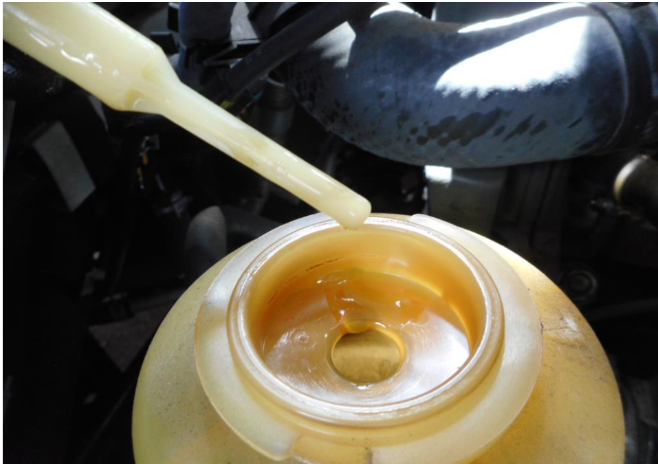
Photo 15 shows the power steering fluid dip stick of the Mini Bus at the time of my inspection. The power steering fluid was observed to be of sufficient level and without any visible contamination.
