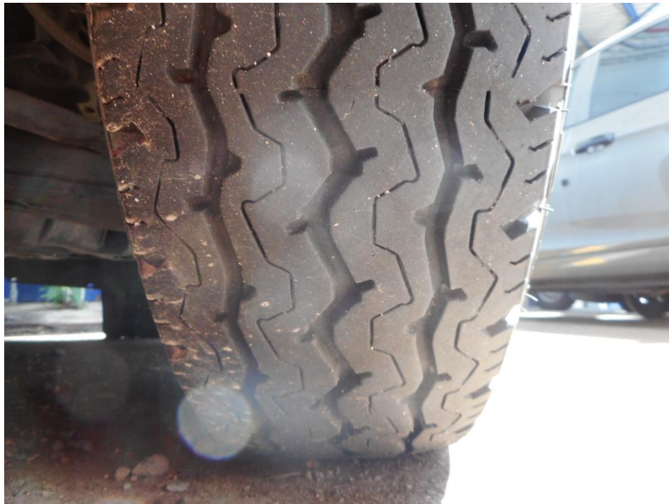
Photo 7 shows the condition of the front right tyre of the Mini Bus, which was observed to be in serviceable condition with remaining tread depth of approximately 6.9mm. The tyre, which was wrapped around standard steel wheel rim, was also observed to be sufficiently inflated for vehicular operation. There was no tear, cut or burst mark(s) on the outer and the inner sidewalls as well as across the tread of the 4 tyres that were fitted on the Mini Bus.
