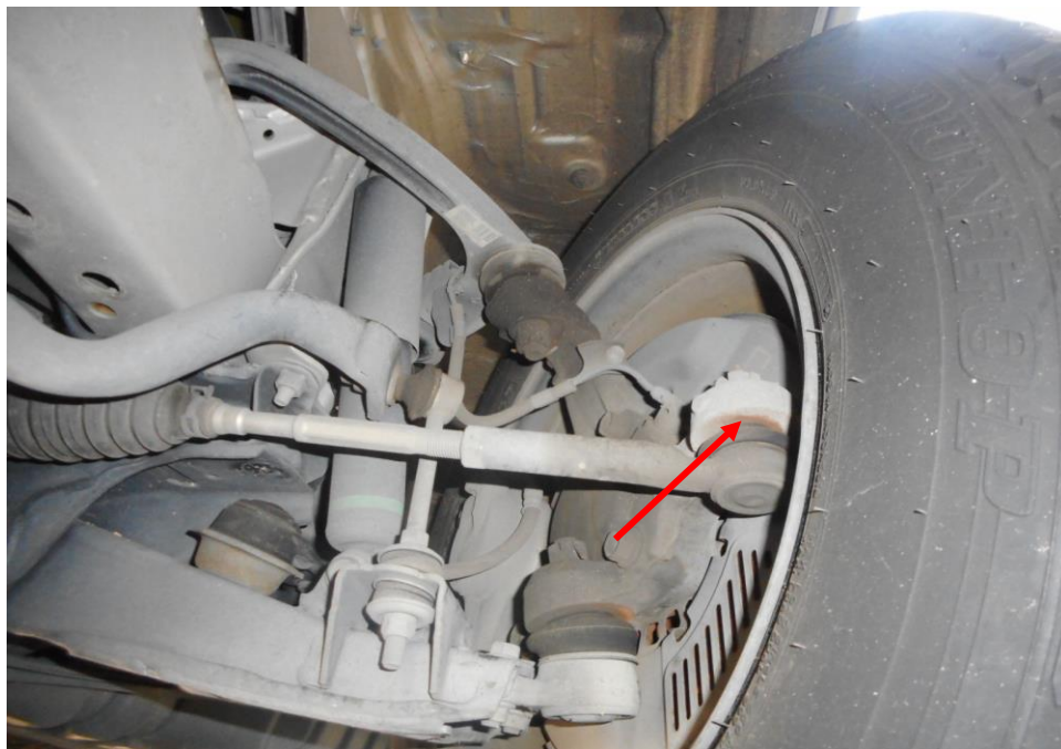
Photo 18 shows the various undercarriage components at the front left wheel of the Mini Bus, in particular the steering tie rod end (arrowed). The various undercarriage components of the Mini Bus were all found to be intact without any visible damage. There was also no sign of fluid stain(s) observed on the various undercarriage components.
