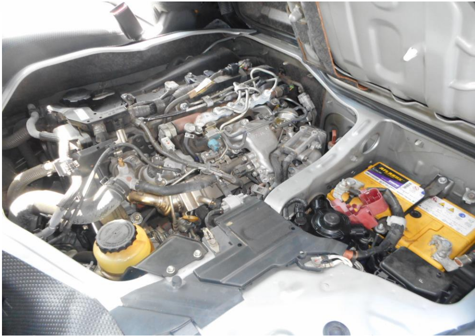
Photo 11 shows a general view of the Mini Bus's engine compartment, which was accessed by lifting the front cabin of the Mini Bus. The various parts and components inside the engine compartment were unaffected by the accident. There was also no sign(s) or indication(s) of fresh fluid leakage and/or fluid stain within the engine compartment
