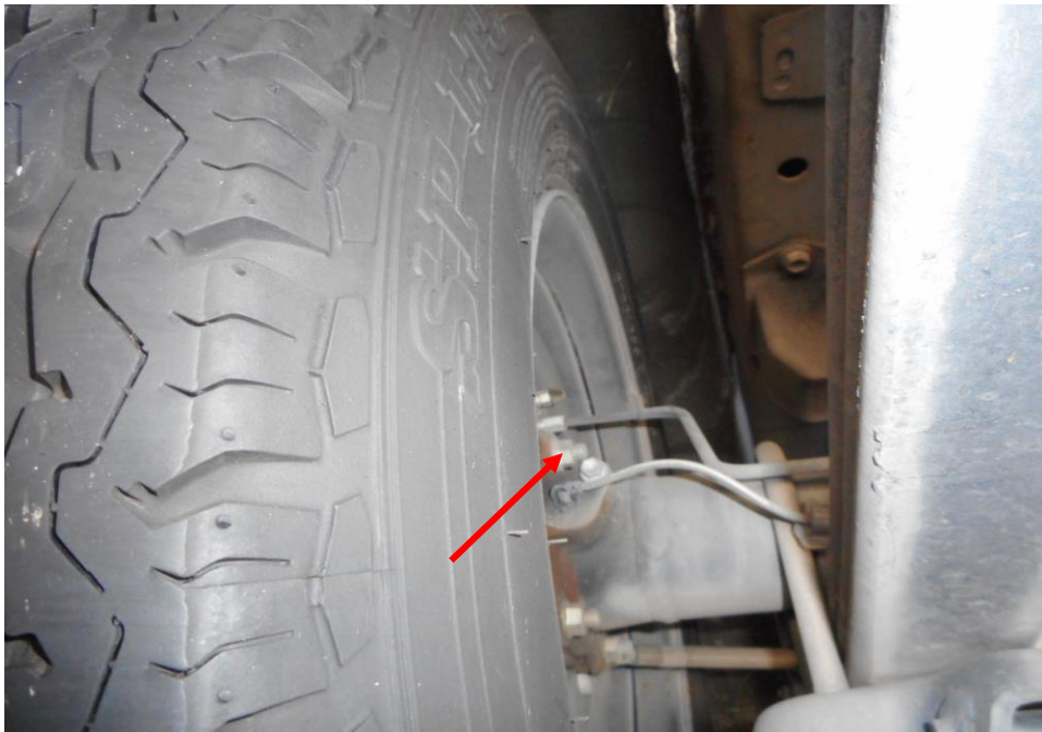
Photo 20 shows the brake pipe (arrowed) at the rear left wheel of the Mini Bus. I did not observe any leakage of brake fluid at the time of my inspection of the Mini Bus. My static tests of the Mini Bus's braking system, along with my visual examination of the various mechanical components in the braking system had indicated that there was no internal leakage of pressure/vacuum. Hence the braking system of the Mini Bus was likely to be in serviceable condition at the material time of accident.
