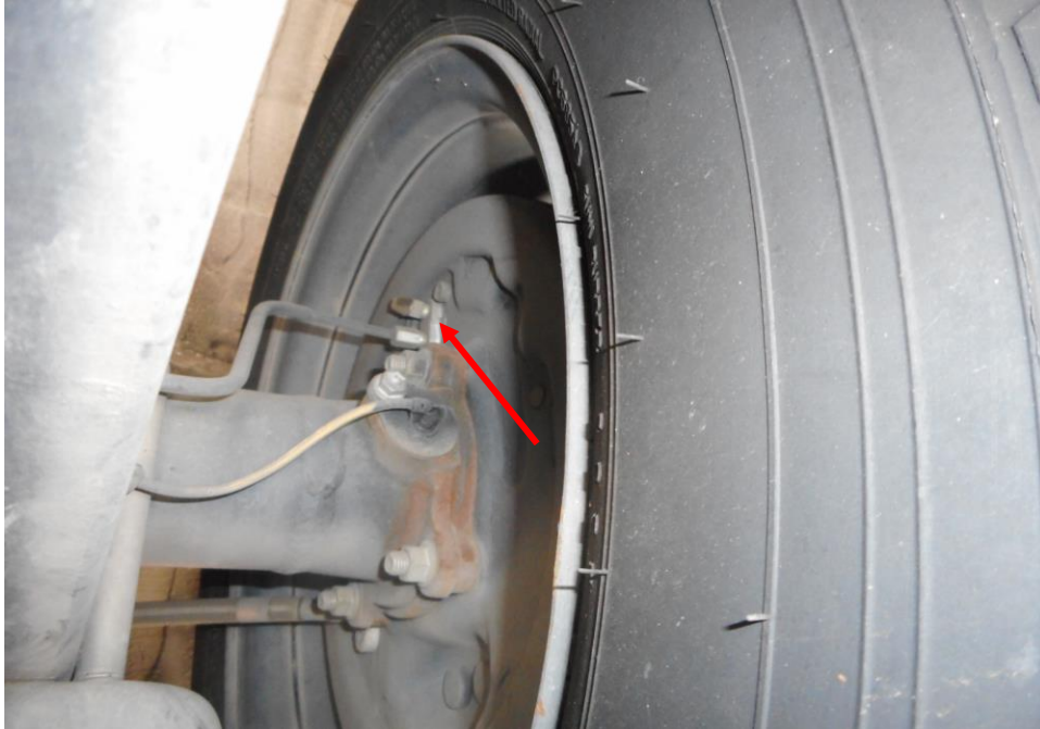
Photo 19 shows the brake pipe (arrowed) at the rear right wheel of the Mini Bus. I did not observe any leakage of brake fluid at the time of my inspection of the Mini Bus. My static tests of the Mini Bus's braking system, along with my visual examination of the various mechanical components in the braking system, had indicated that there was no internal leakage of pressure/vacuum. Hence the braking system of the Mini Bus was likely to be in serviceable condition at the material time of accident.
