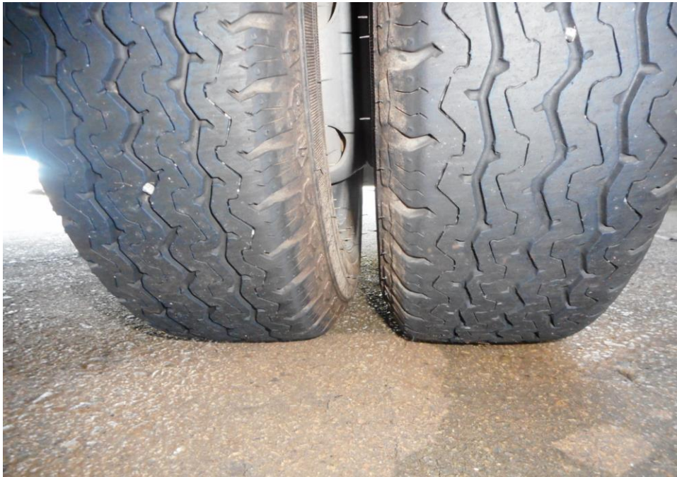
Photo 10 shows the condition of the rear left tyres of the Motor Lorry, which was observed to be in serviceable condition with remaining tread depth of approximately 4.1mm. The tyres, which were wrapped around standard steel wheel rim, were also observed to be sufficiently inflated for vehicular operation. There was also no damage found on all 6 steel wheel rims of the Motor Lorry.
