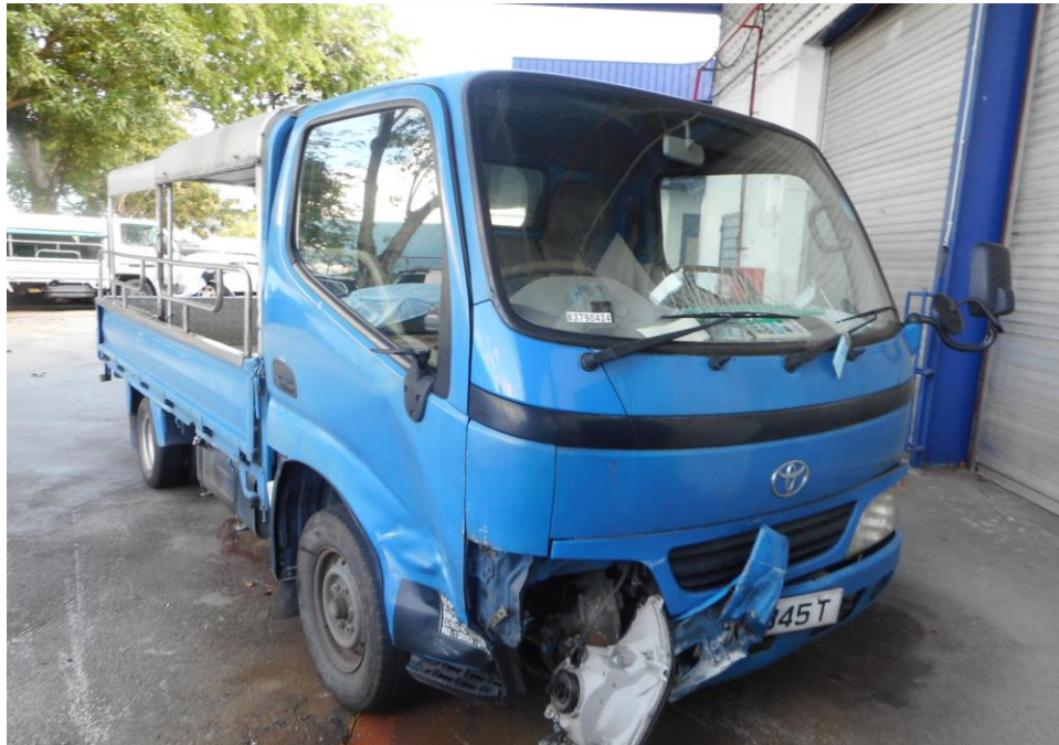
Photo 4 shows a general view of the Motor Lorry's right portion at the time of my inspection. It appeared to have sustained moderate damage at its right rear view mirror and right door panel were damage at the time of my inspection.
