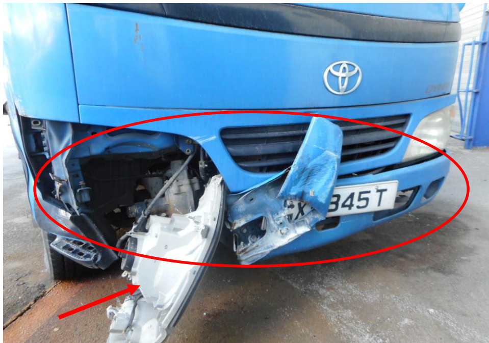
Photo 3 shows a close up view of the Motor Lorry's frontal portion at the time of my inspection. It appeared to have sustained moderate damage at its frontal portion. Its front bumper (circled) and front right headlamp (arrowed) were damage at the time of my inspection.
