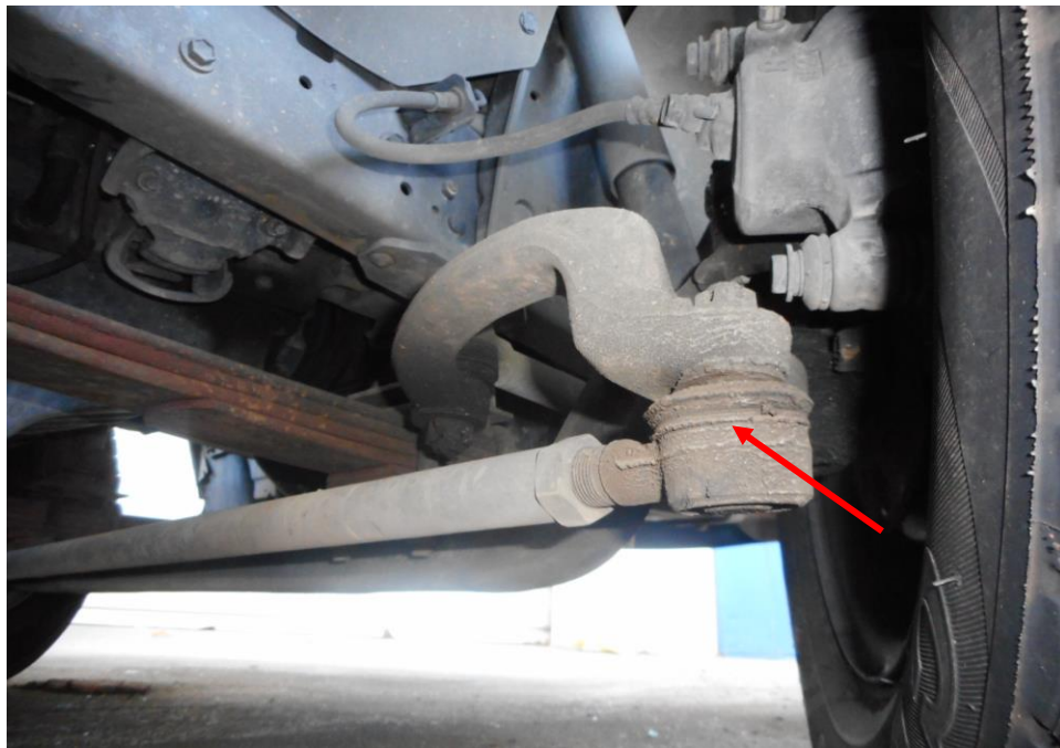
Photo 17 shows the various undercarriage components at the front right wheel of the Motor Lorry, in particular the steering tie rod end (arrowed). The various steering components were all found to be intact, suggesting that the steering system of the Motor Lorry was likely to be in serviceable condition at the material time of accident. There was also no sign of fluid stain(s) observed on the various undercarriage components.
