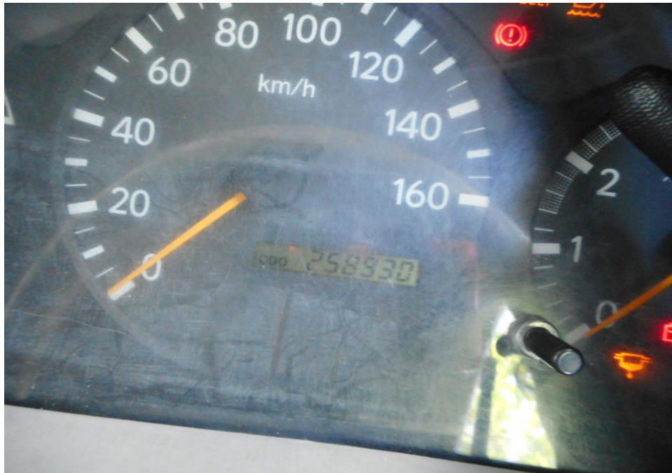
Photo 1 shows a general view of the instrument cluster of the Motor Lorry at the time of my inspection. The mileage of the Motor Lorry was 258,930km
