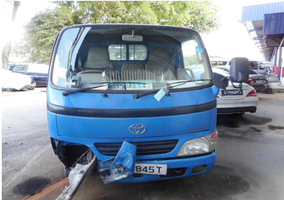
Photo 2 shows a general view of the Motor Lorry's frontal portion at the time of my inspection. It appeared to have sustained moderate damage at its frontal and right portion. Its front bumper, front right headlamp, right rear view mirror and right door panel were damage at the time of my inspection.
