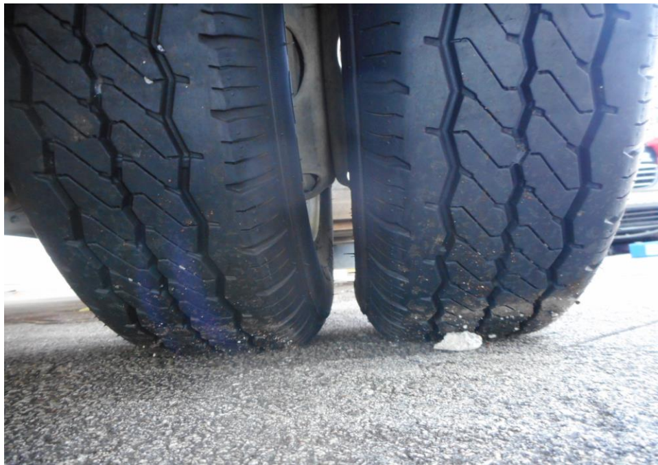
Photo 9 shows the condition of the rear right tyre of the Motor Lorry, which was observed to be in serviceable condition with remaining tread depth of approximately 5.4mm. The tyre, which was wrapped around standard steel wheel rim, was also observed to be sufficiently inflated for vehicular operation.
