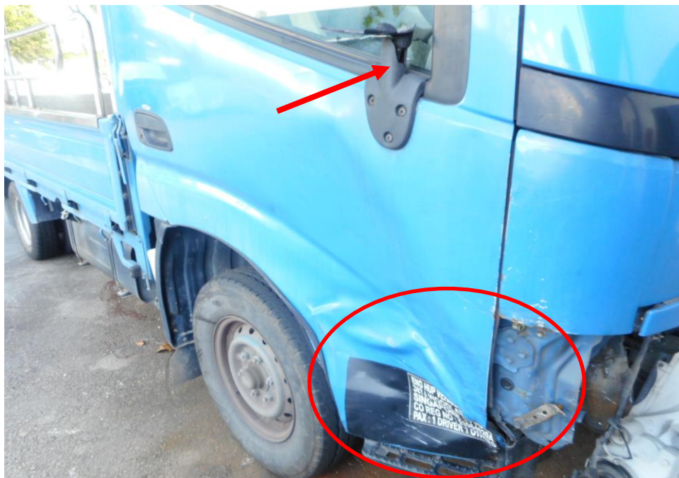
Photo 5 shows a close up view of the Motor Lorry's right portion at the time of my inspection. It appeared to have sustained moderate damage at its right rear view mirror (arrowed) and right door panel (circled) were damage at the time of my inspection.
