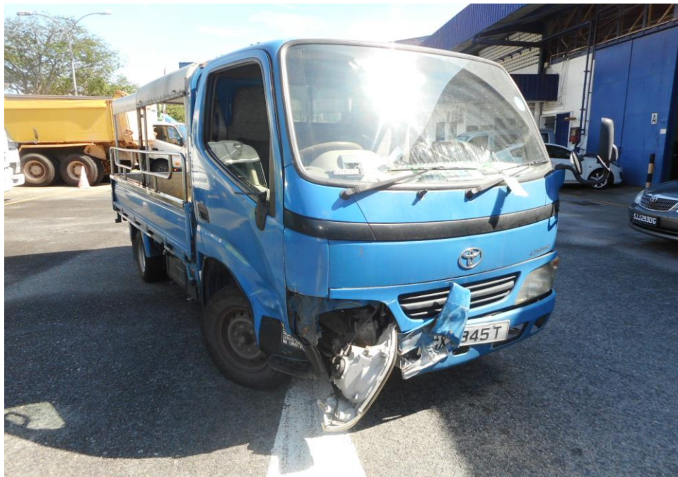
Photo 23 shows the front left wheel of the Motor Lorry turned to its full right. During my steering system test, I did not experience any abnormal free play and/or resistance when I had turned the steering wheel towards full left and full right. This would suggest that the steering system of the Motor Lorry was likely to be in serviceable condition at the material time of accident.
