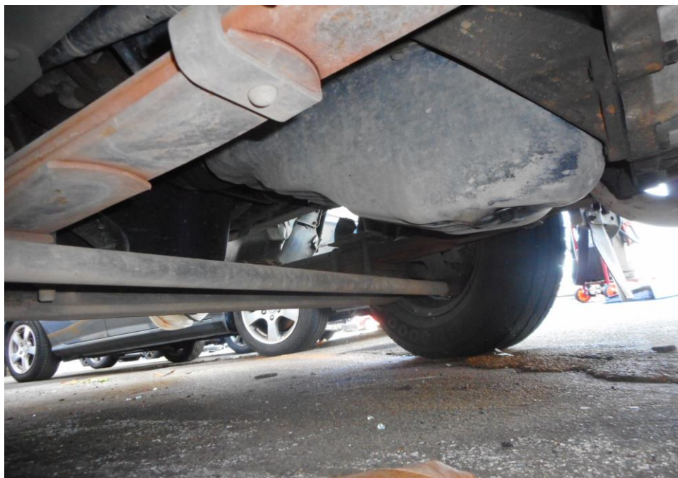
Photo 16 shows the undercarriage of the Motor Lorry, at the area where the engine housing and transmission housing are located. Observed was minor old engine oil stain on the housing of the engine oil sump
