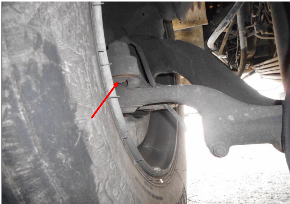
Photo 28 shows the various undercarriage components at the front left wheel of the Motor Trailer, in particular the steering tie rod end (arrowed). The various undercarriage components of the Motor Trailer were all found to be intact without any visible damage. There was also no sign of fluid stain(s) observed on the various undercarriage components.
