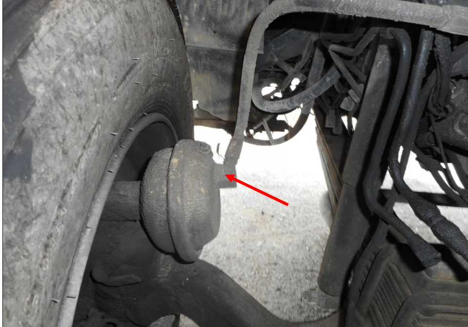
Photo 25 shows the brake pipe (arrowed) at the front left wheel of the Motor Trailer. I did not observe any leakage of brake fluid at the time of my inspection of the Motor Trailer. My visual examination of the various mechanical components in the braking system had indicated that there was no internal leakage of pressure/vacuum and there components were generally in good condition.
