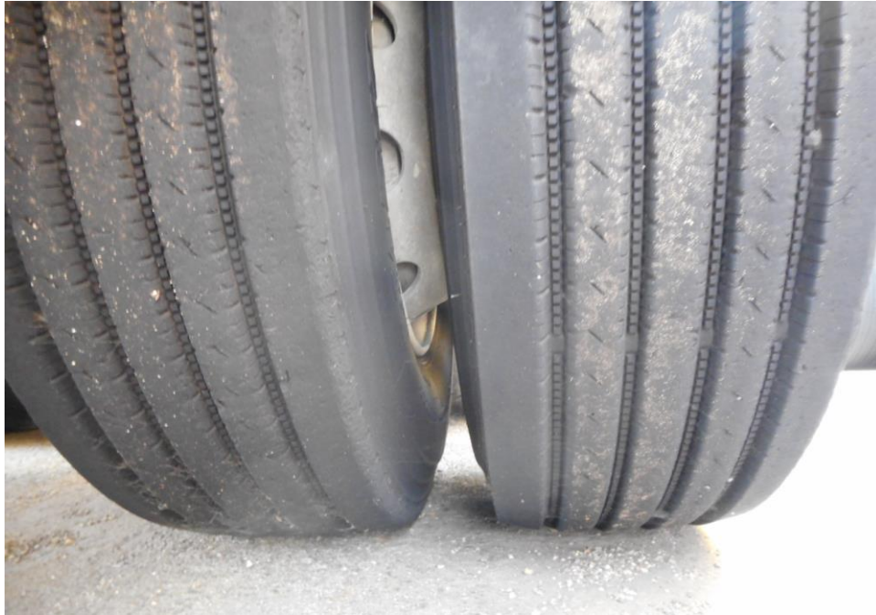
Photo 15 shows the condition of the left tyres of the trailer, which was observed to be in serviceable condition with remaining tread depth of approximately 9.3mm. The tyres, which were wrapped around standard steel wheel rim, were also observed to be sufficiently inflated for vehicular operation. There was also no damage found on all 6 steel wheel rims of the Motor Trailer.
