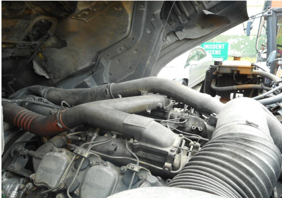
Photo 16 shows a general view of the Motor Trailer's engine compartment, which was accessed by lifting the front cabin of the Motor Trailer. The various parts and components inside the engine compartment were unaffected by the accident. There was also no sign(s) or indication(s) of fresh fluid leakage and/or fluid stain within the engine compartment
