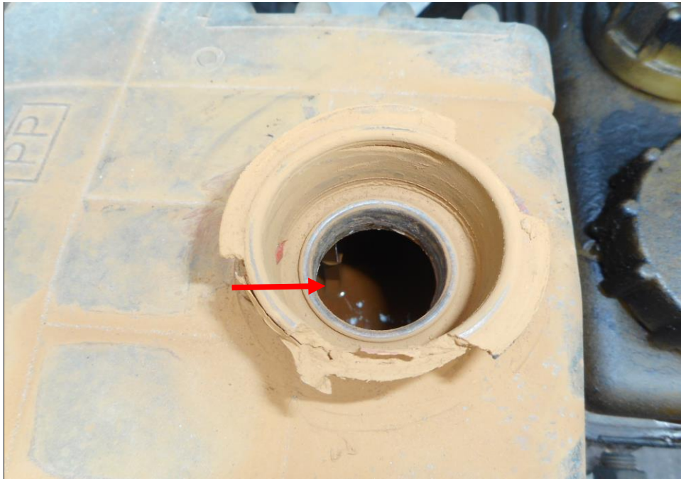
Photo 18 shows the engine coolant reservoir of the Motor Trailer at the time of my inspection. The engine coolant was observed to be of sufficient level (arrowed) and without any visible contamination.
