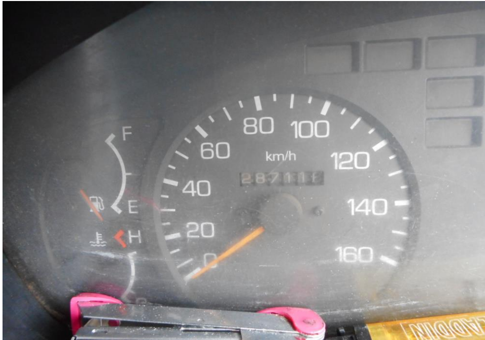
Photo 1 shows a general view of the instrument cluster of the Motor Trailer at the time of my inspection. The mileage of the Motor Trailer was 287,118km
