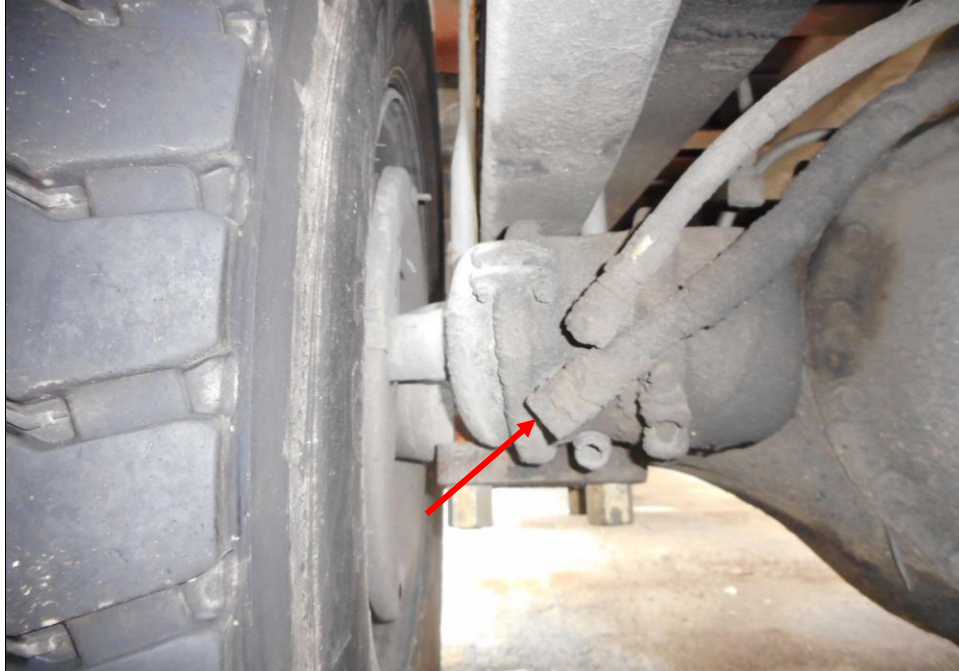
Photo 23 shows the brake pipe (arrowed) at the rear left wheel of the Motor Trailer. I did not observe any leakage of brake fluid at the time of my inspection of the Motor Trailer. My static tests of the Motor Trailer's braking system, along with my visual examination of the various mechanical components in the braking system, had indicated that there was no internal leakage of pressure/vacuum and there components were generally in good condition.
