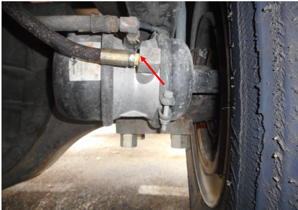
Photo 22 shows the brake pipe (arrowed) at the rear right wheel of the Motor Trailer. I did not observe any leakage of brake fluid at the time of my inspection of the Motor Trailer. My visual examination of the various mechanical components in the braking system, had indicated that there was no internal leakage of pressure/vacuum and there components were generally in good condition.
