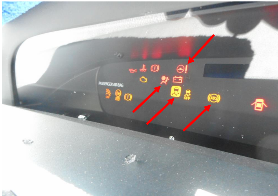
Photo 23 shows the warning light for Anti-Lock Brake System (ABS), Supplemental Restraint System (SRS), Traction Control System (TC) and Electric Power Steering System (EPS) appearing on the instrument panel of the Motor Taxi during the self-test of its various electronic operating systems when its engine was cranked.
