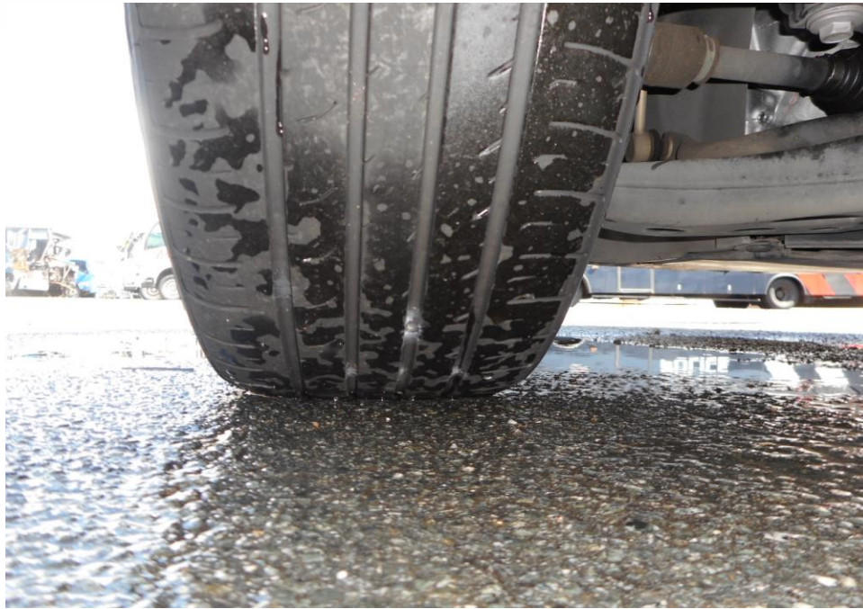
Photo 10 shows the condition of the rear right tyres of the Motor Taxi, which were observed to be in serviceable condition with remaining, tread depth of approximately 3.7mm. There was also no tear, cut or burst mark(s) on the outer and the inner sidewalls as well as across the tread of the 4 tyres that were fitted on the Motor Taxi.
