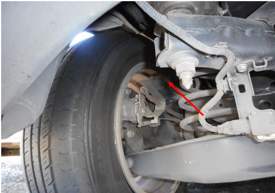
Photo 19 shows the brake pipe (arrowed) at the rear left wheel of the Motor Taxi. I did not observe any leakage of brake fluid at the time of my inspection of the Motor Taxi. My static tests of the Motor Taxi's braking system, along with my visual examination of the various mechanical components in the braking system had indicated that there was no internal leakage of pressure/vacuum. Hence the braking system of the Motor Taxi was likely to be in serviceable condition at the material time of accident.
