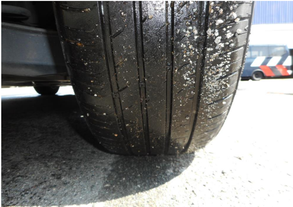
Photo 8 shows the condition of the rear right tyre of the Motor Taxi, which was observed to be in serviceable condition with remaining tread depth of approximately 4.6mm. The tyre, which was wrapped around standard alloy wheel rim, was also observed to be sufficiently inflated for vehicular operation.
