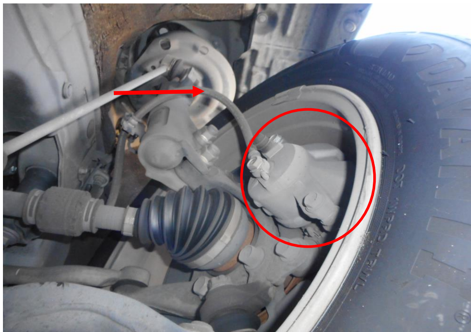
Photo 21 shows the brake hose/pipe (arrowed) at the front left wheel of the Motor Taxi. No leakage of brake fluid was observed. Visual examination of the various components of the braking system like the brake caliper (circled), brake booster, brake pedal etc had revealed all to be intact and without visible damage at the time of accident. There was also no sign of fluid stain(s) observed on the various undercarriage components.
