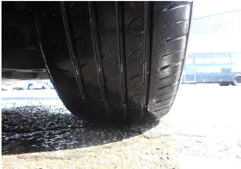
Photo 7 shows the condition of the front right tyre of the Motor Taxi, which was observed to be in serviceable condition with remaining tread depth of approximately 3.5mm. The tyre, which was wrapped around standard alloy wheel rim, was also observed to be sufficiently inflated for vehicular operation. There was no tear, cut or burst mark(s) on the outer and the inner sidewalls as well as across the tread of the 4 tyres that were fitted on the Motor Taxi.
