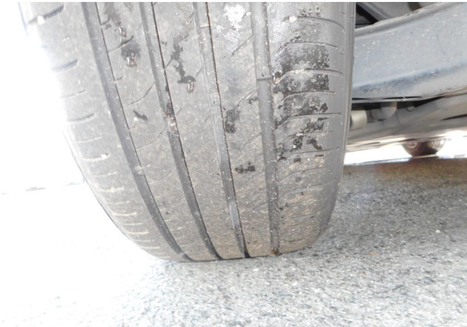
Photo 9 shows the condition of the rear left tyres of the Motor Taxi, which was observed to be in serviceable condition with remaining tread depth of approximately 4.9mm. The tyres, which were wrapped around standard alloy wheel rim, were also observed to be sufficiently inflated for vehicular operation. There was also no damage found on all 4 alloy wheel rims of the Motor Taxi.
