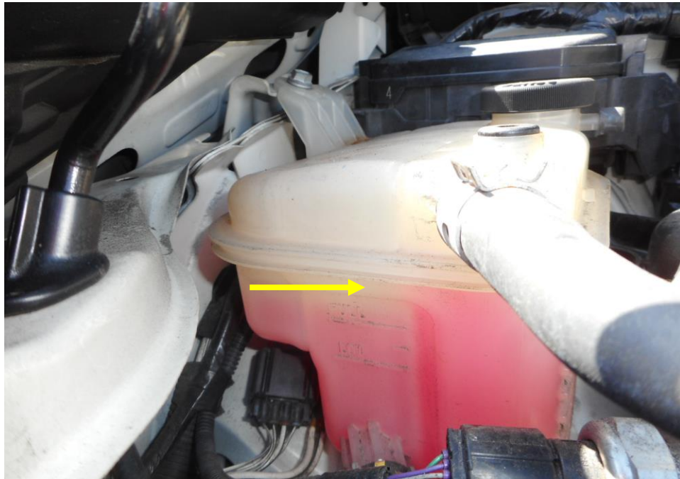
Photo 13 shows the engine coolant reservoir of the Motor Taxi at the time of my inspection. The engine coolant was observed to be of sufficient level (arrowed) and without any visible contamination.
