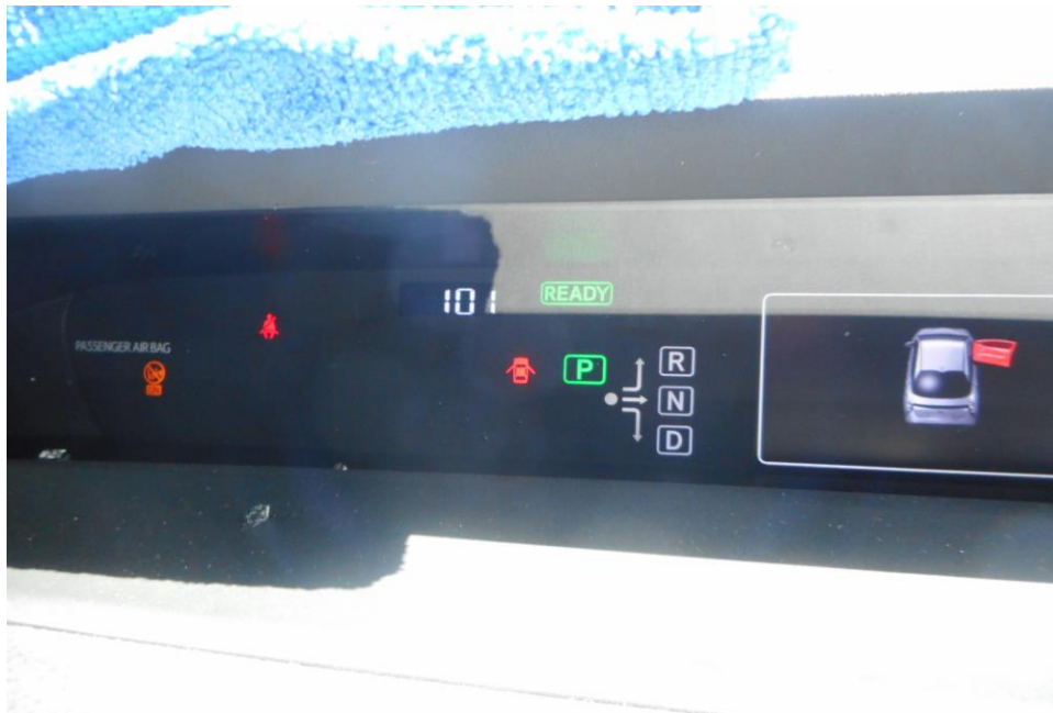
Photo 24 shows no warning lights illuminated on the instrument panel of the Motor Taxi after the engine was cranked. This would suggest that there was no abnormality to the various electronic operating systems of the Motor Taxi, like the ABS, SRS, TC and EPS.
