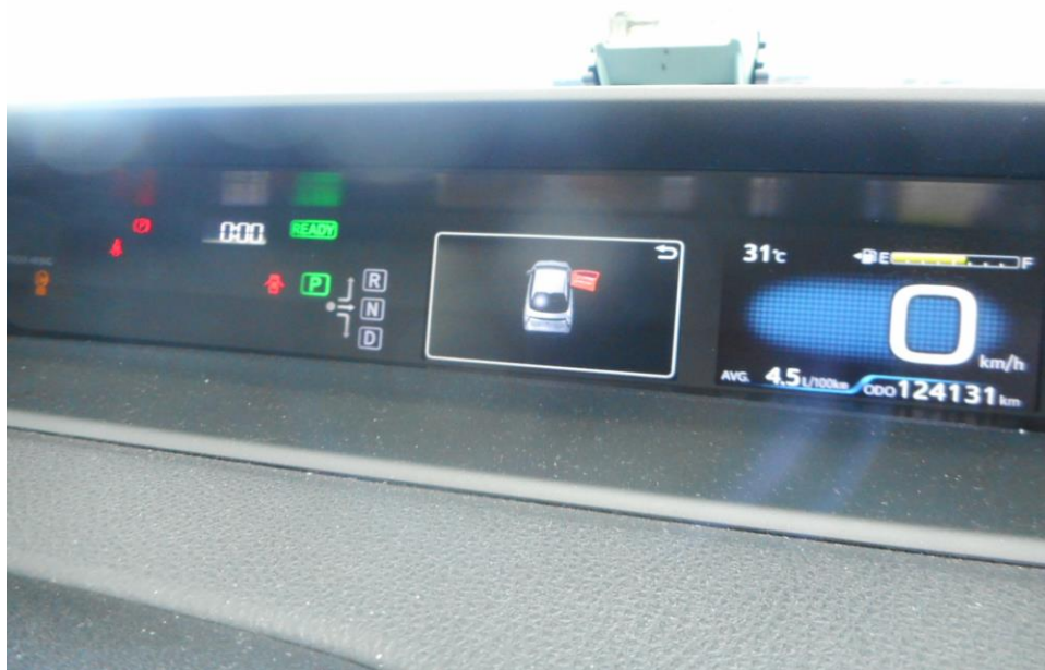
Photo 21 shows no warning lights illuminated on the instrument panel of the Motor Taxi after the engine was cranked. This would suggest that there was no abnormality to the various electronic operating systems of the Motor Taxi, like the ABS, EPS, TC and SRS etc.
