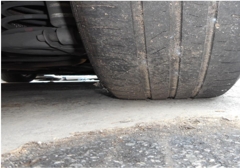
Photo 6 shows the condition of the rear right tyre of the Motor Taxi, which was observed to be in serviceable condition with remaining tread depth of approximately 3.4mm. The tyre was also observed to be sufficiently inflated for vehicular operation with no tear, cut or burst mark(s).
