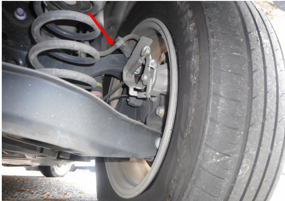
Photo 16 shows the brake hose/pipe (arrowed) at the rear right wheel of the Motor Taxi. I did not observe any leakage of brake fluid at the time of my inspection of the Motor Taxi. Static tests of the Motor Taxi's braking system had indicated that there was no internal leakage of pressure/vacuum. The undercarriage components of the Motor Taxi were also all found to be intact and without any visible damage.
