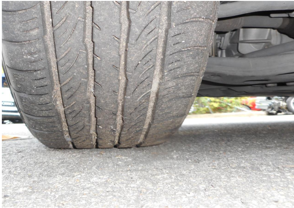
Photo 8 shows the condition of the front left tyre of the Motor Taxi, which was observed to be in serviceable condition with remaining tread depth of approximately 3.8mm. The tyre was also observed to be sufficiently inflated for vehicular operation with no tear, cut or burst mark(s).
