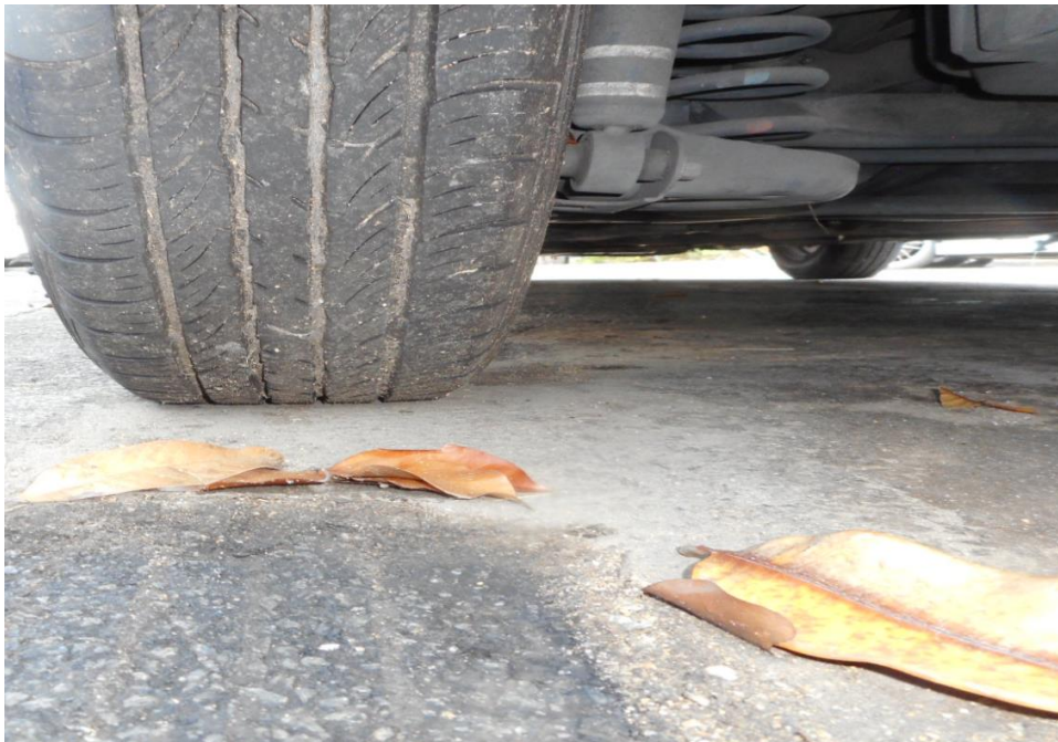
Photo 7 shows the condition of the rear left tyre of the Motor Taxi, which was observed to be in serviceable condition with remaining tread depth of approximately 3.4mm. The tyre was also observed to be sufficiently inflated for vehicular operation with no tear, cut or burst mark(s).
