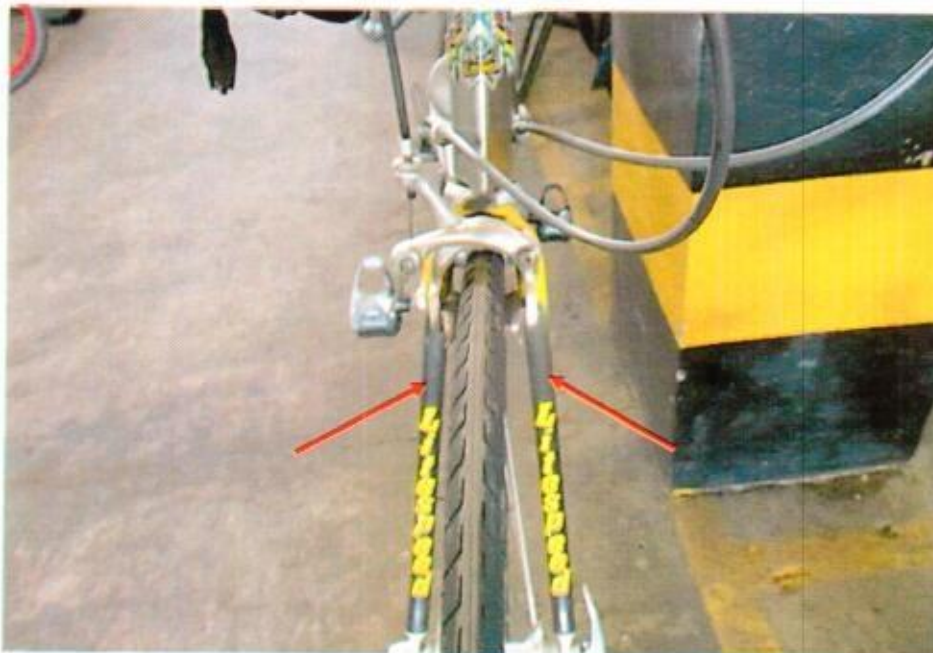
Photo 15 shows the front fork (arrowed) of the Bicycle. The front fork and fork bracket of the Bicycle were both found to be intact and undamaged. Turning the Bicycle's handle bar towards the left and right did not produce any abnormal free play. The steering system of the Bicycle was in serviceable condition at the time of our inspection.
