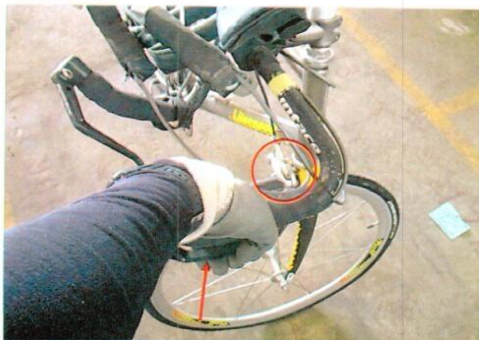
Photo 18 shows a static brake test conducted on the Bicycle's front brake. There was some resistance felt upon pressing the left hand brake lever (arrowed). It also shows that the front brake clamps responded to the gripping action (circled) after depressing the left hand brake lever.
