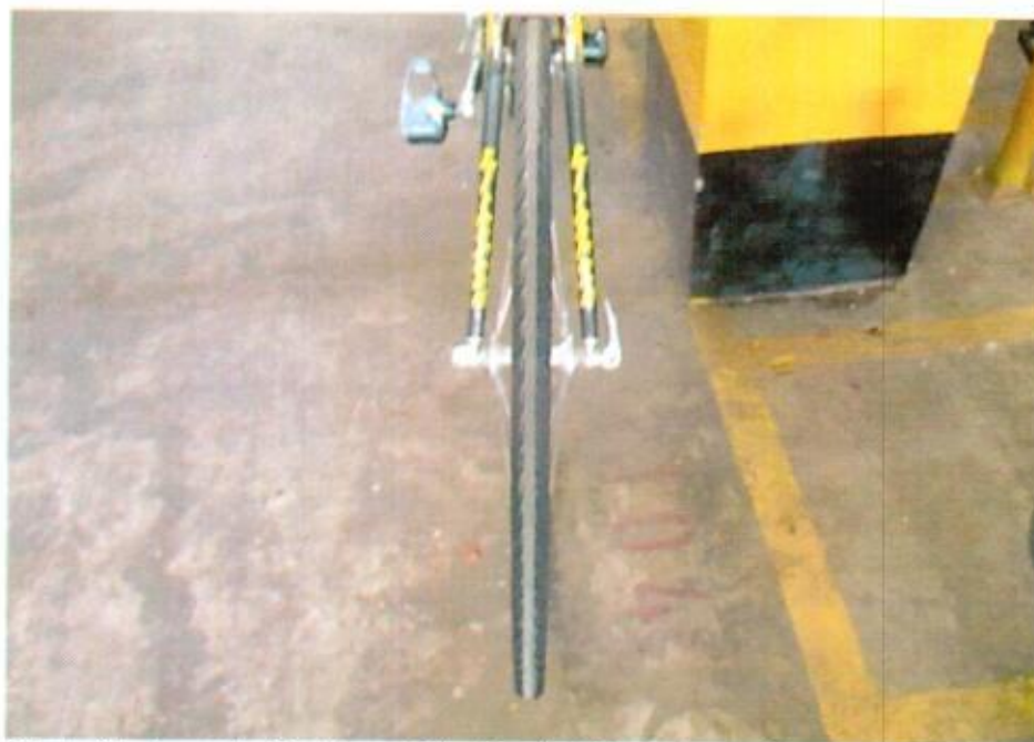
Photo 11 shows the front tyre of the Bicycle. The pattern of the tread was clearly visible. There was no tear, burst mark(s) and/or punctured hole(s) on the sidewalls as well as across the tread of the front tyre.
