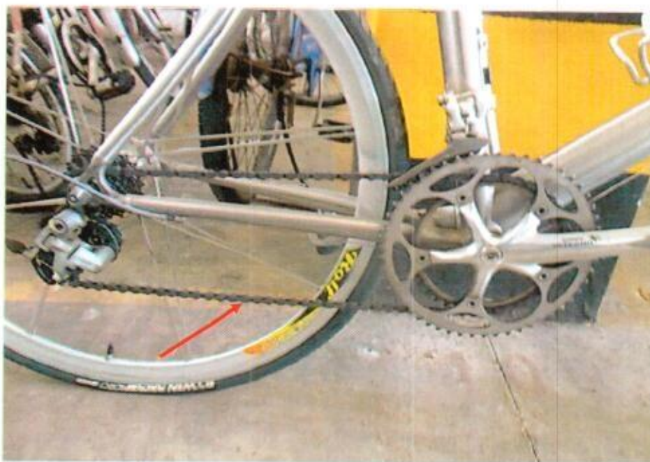
Photo 13 shows the general view of the gear train of the Bicycle, which was observed to be intact with no misalignment. It was also adequately lubricated for operating purposes (arrowed).
