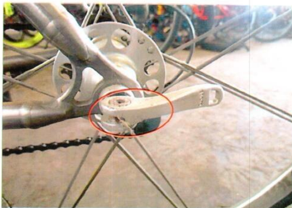
Photo 9 shows the damages of grazing nature on the left rear axle lever (circled) of the Bicycle at the time of our inspection.
