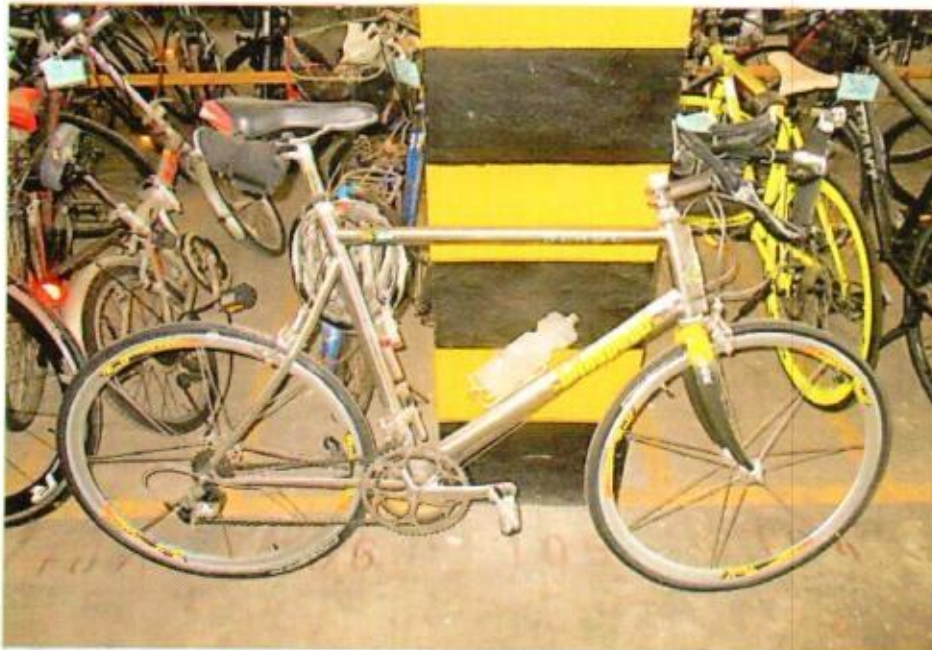
Photo 4 shows the right body of the Bicycle at time of our inspection. The bicycle had sustained damages all around. The body parts that were found to have been damaged include its brake levers, handlebars, left pedal and seat, amongst others as a result of the accident.
