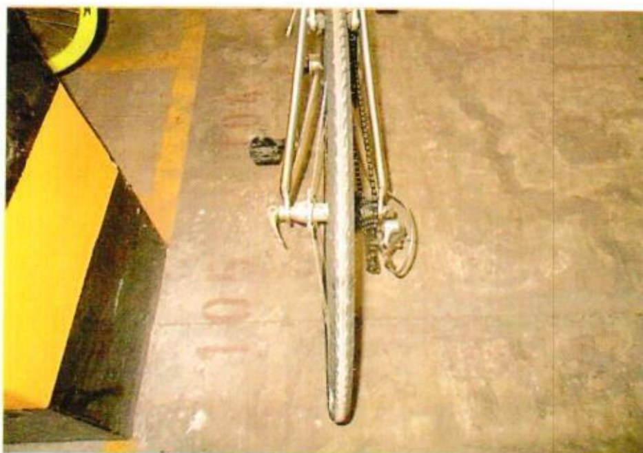
Photo 12 shows the rear tyre of the Motorcycle. The pattern of the tread was clearly visible. There was no tear, burst mark(s) and/or punctured hole(s) on the sidewalls as well as across the tread of the front tyre. However the rear tyre was observed to be deflated.
