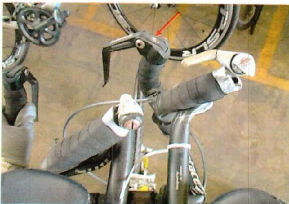
Photo 6 shows the damaged rear brake lever (arrowed) of the Bicycle at the time of our inspection.
