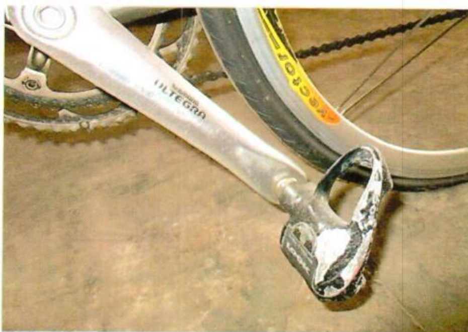
Photo 8 shows the damaged left pedal of the Bicycle at the time of our inspection.
