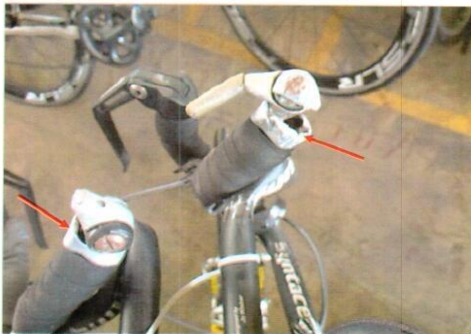
Photo 7 shows the damaged handlebars (arrowed) of the Bicycle at the time of our inspection.
