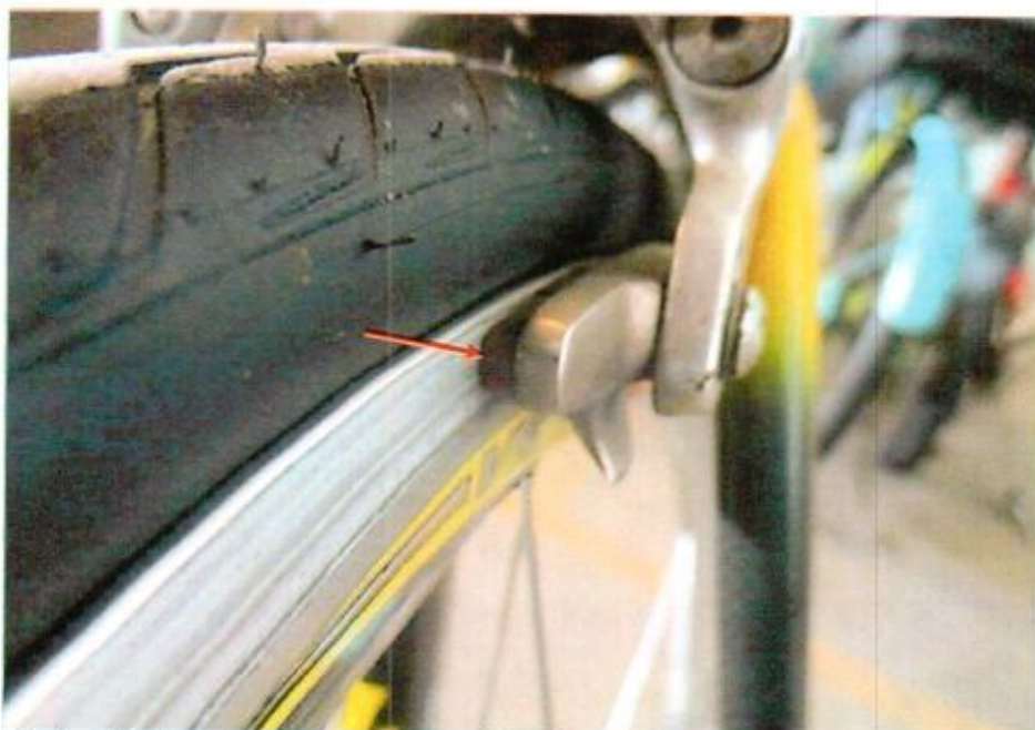
Photo 19 shows a close up view of the front brake clamps responding to the gripping action. The rubber brake blocks pressed against the front wheel rim upon depressing the left hand brake lever (arrowed). This had appeared to indicate that the front brake was in serviceable condition.
