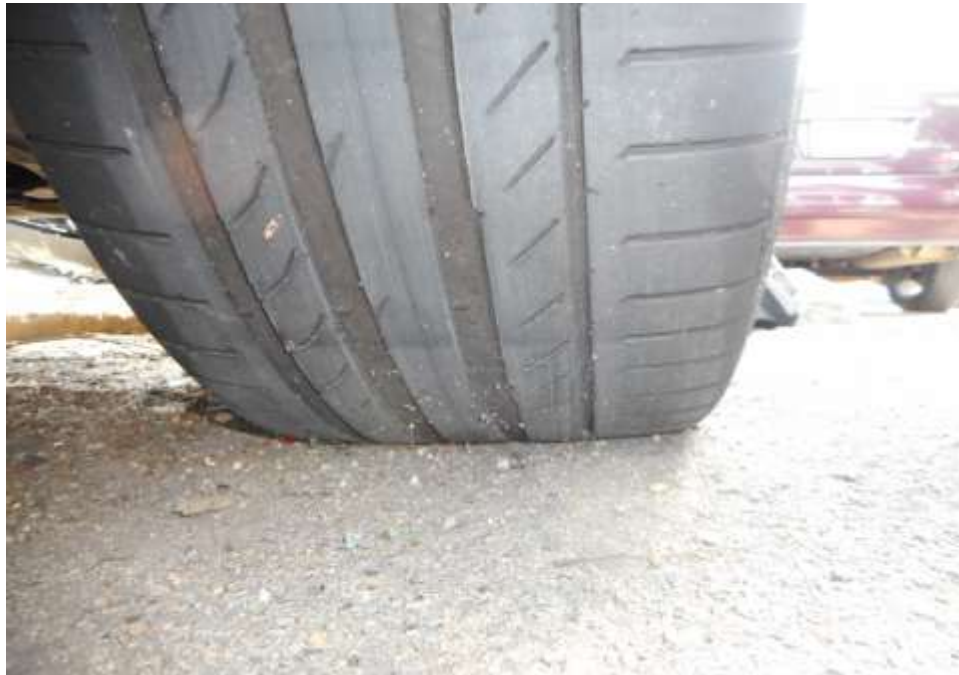
Photo 7 shows the condition of the front right tyre of the Motor Car, which was observed to be in serviceable condition with remaining tread depth of approximately 5mm. The tyre, which was wrapped around alloy wheel rim, was also observed to be sufficiently inflated for vehicular operation.
