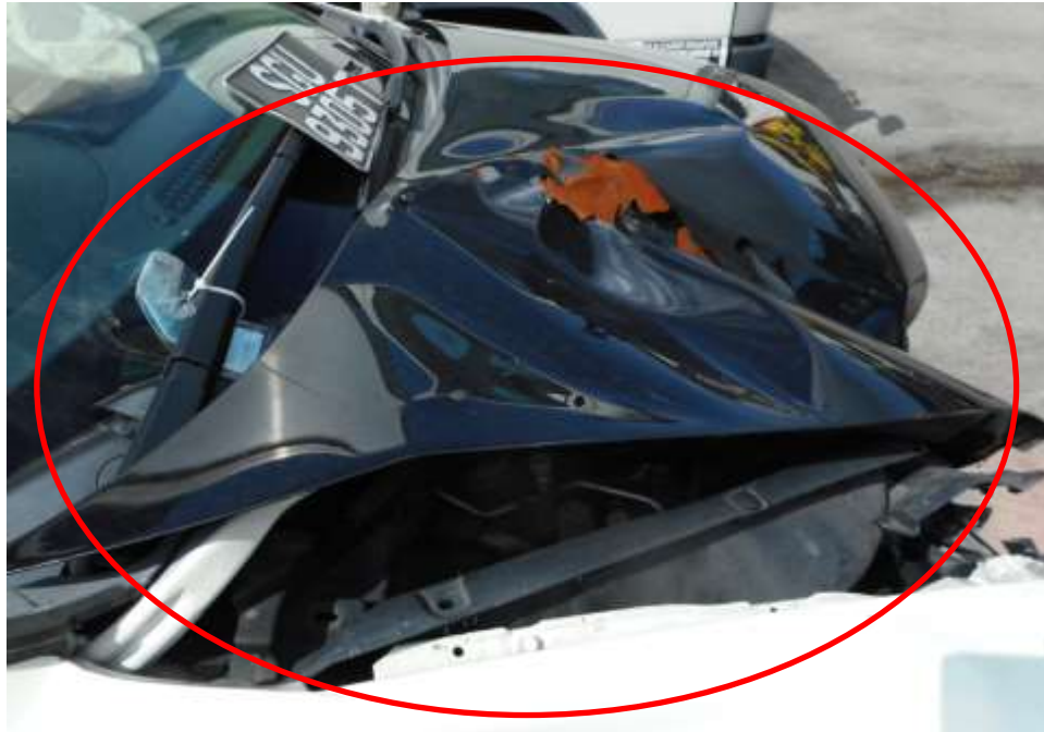
Photo 12 shows a close up view of the damaged front bonnet lock mechanism and the structure of the engine compartment of the Motor Car at the time of my inspection resulting it unable to open a result of the accident. (circled) (Unable to open)
