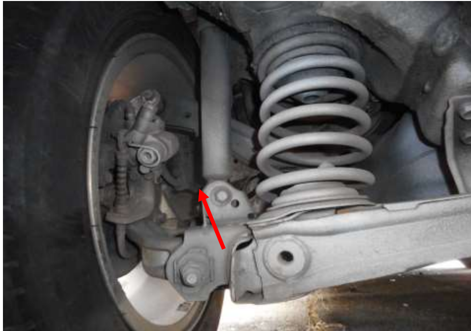
Photo 13 shows the brake hose/pipe (arrowed) at the rear left wheel of the Motor Car. No leakage of brake fluid was observed. Visual examination of the various components of the braking system like the drum brake, brake booster, brake pedal etc. had revealed all to be intact and without visible damage.
