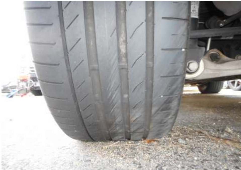
Photo 9 shows the condition of the rear left tyre of the Motor Car, which was observed to be in serviceable condition with remaining tread depth of approximately 4.4mm. The tyre was also observed to be sufficiently inflated for vehicular operation with no tear, cut or burst mark(s).
