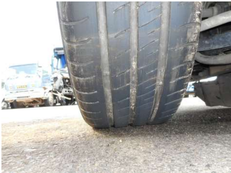
Photo 10 shows the condition of the front left tyre of the Motor Car, which was observed to be in serviceable condition with remaining tread depth of approximately 4.8mm. The tyre was also observed to be sufficiently inflated for vehicular operation with no tear, cut or burst mark(s).
