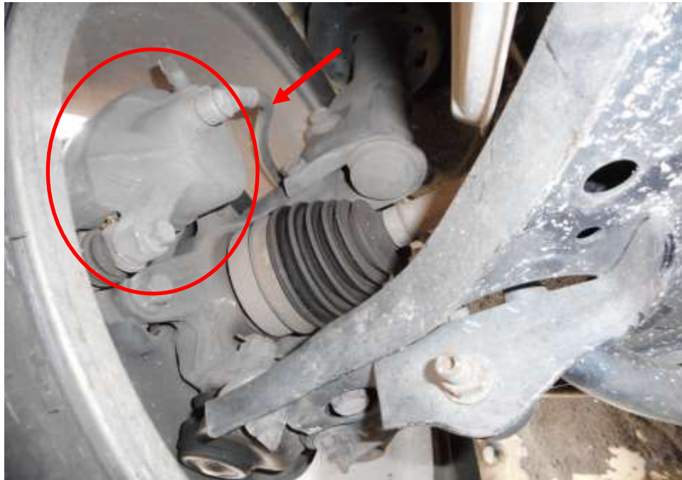
Photo 15 shows the brake hose/pipe (arrowed) at the front right wheel of the Motor Car. No leakage of brake fluid was observed. Visual examination of the various components of the braking system like the brake caliper (circled), brake booster, brake pedal etc had revealed all to be intact and without visible damage at the time of accident. There was also no sign of fluid stain(s) observed on the various undercarriage components.
