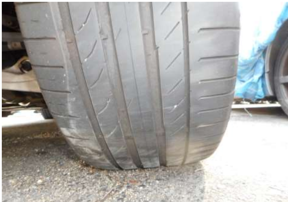
Photo 8 shows the condition of the rear right tyre of the Motor Car, which was observed to be in serviceable condition with remaining tread depth of approximately 4.2mm. The tyre was also observed to be sufficiently inflated for vehicular operation with no tear, cut or burst mark(s).
