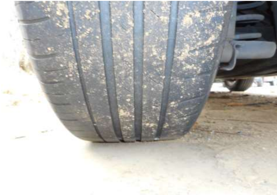
Photo 10 shows the condition of the rear left tyre of the Motor Car, which was observed to be in serviceable condition with remaining tread depth of approximately 3.9mm. The tyre, which was wrapped around steel wheel rim, was also observed to be sufficiently inflated for vehicular operation. The 4 tyres of the Motor Car were wrapped around standard steel wheel rims.
