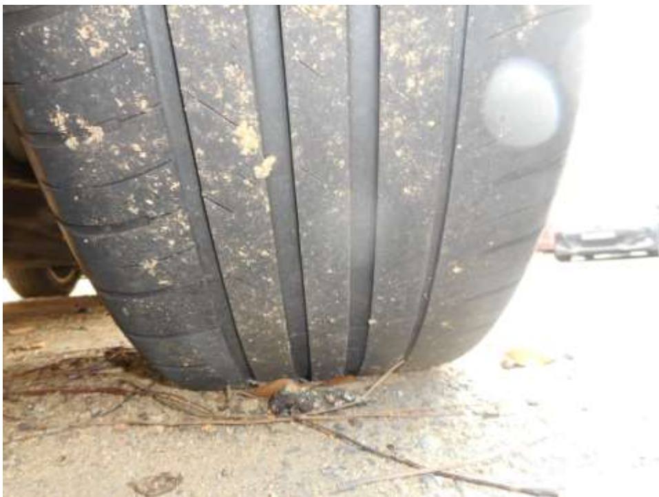
Photo 9 shows the condition of the rear right tyre of the Motor Car, which was observed to be in serviceable condition with remaining tread depth of approximately 4mm. The tyre was also observed to be sufficiently inflated for vehicular operation with no tear, cut or burst mark(s).
