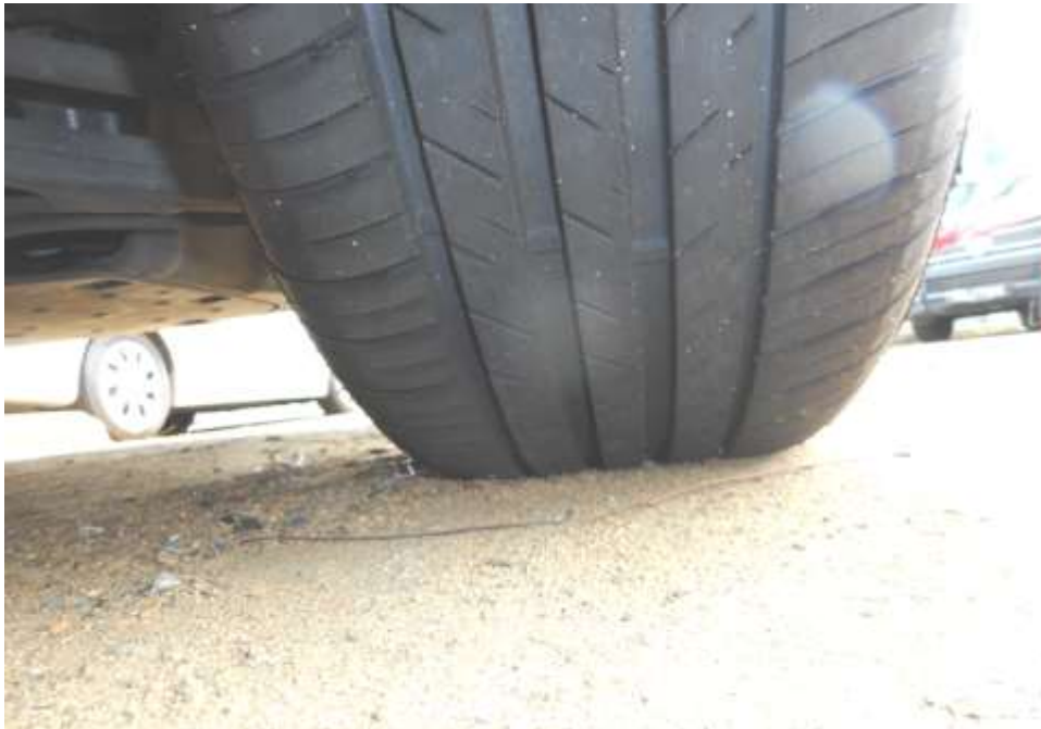
Photo 8 shows the condition of the front right tyre of the Motor Car, which was observed to be in serviceable condition with remaining tread depth of approximately 7mm. The tyre was sufficiently inflated for vehicular operation with no tear, cut or burst mark(s) on the outer and the inner sidewalls as well as across the tread. The 4 tyres of the Motor Car were wrapped around standard steel wheel rims without any damage.
