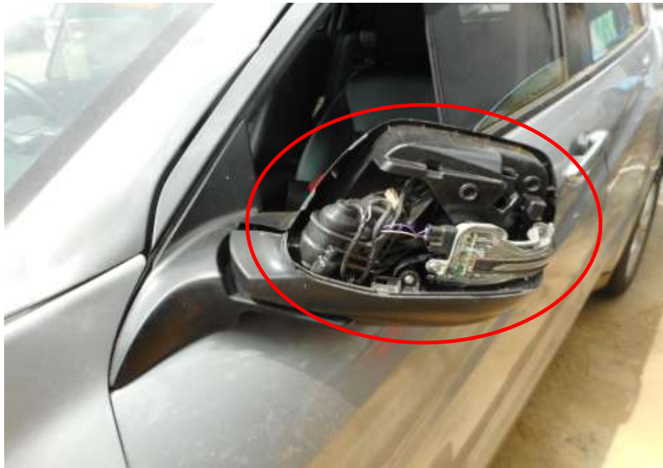
Photo 4 shows the close up view of the Motor Car's front body at the time of my inspection. The Motor Car was observed to have sustained damage at its front left rear view mirror (circled) as a result of the accident.
