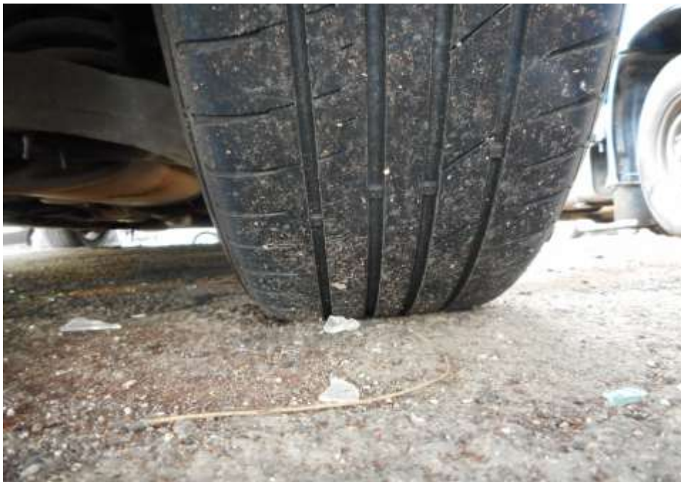
Photo 11 shows the condition of the rear right tyre of the Motor Car, which was observed to be in serviceable condition with remaining tread depth of approximately 4.8mm. The tyre was also observed to be sufficiently inflated for vehicular operation with no tear, cut or burst mark(s).
