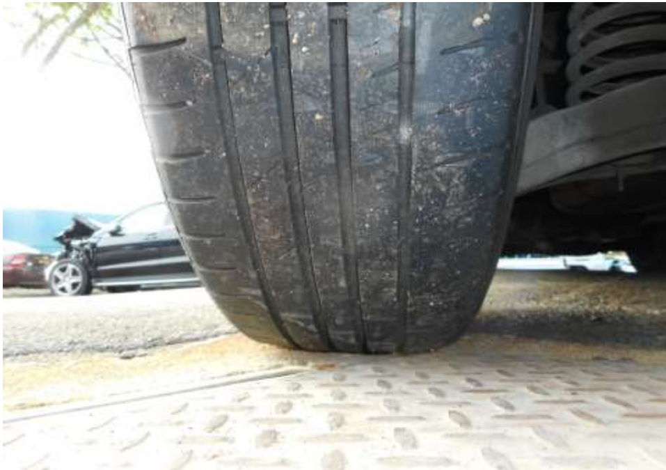
Photo 12 shows the condition of the rear left tyre of the Motor Car, which was observed to be in serviceable condition with remaining tread depth of approximately 4.1mm. The tyre, which was wrapped around steel wheel rim, was also observed to be sufficiently inflated for vehicular operation. The 4 tyres of the Motor Car were wrapped around standard steel wheel rims.
