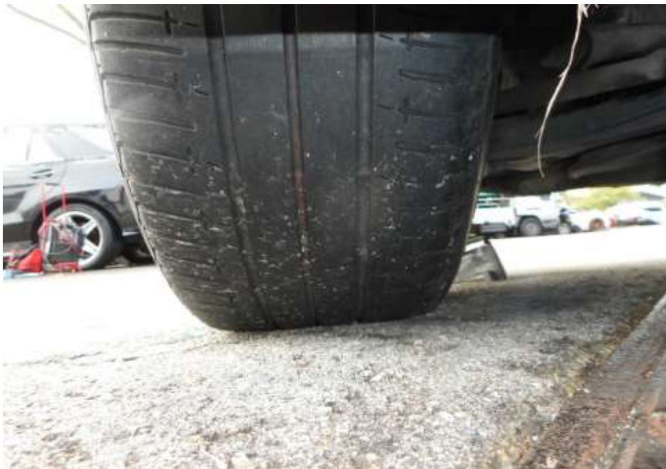
Photo 13 shows the condition of the front left tyre of the Motor Car, which was observed to be in serviceable condition with remaining tread depth of approximately 3mm. There was also no tear, cut or burst mark(s) on the outer and the inner sidewalls as well as across the tread of the Motor Car's 4 tyres.
