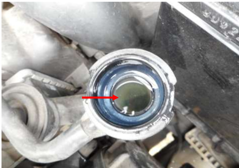
Photo 16 shows checks being carried out to the engine coolant of the Motor Car at the time of my inspection. The engine coolant was observed to be of sufficient level (arrowed) and without any visible contamination.
