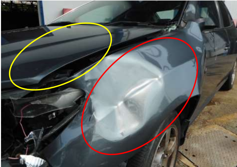
Photo 4 shows the close up view of the Motor Car's front body at the time of my inspection. The Motor Car was observed to have sustained damage at its front bonnet (yellow circle) and front left fender (red circle), as a result of the accident.
