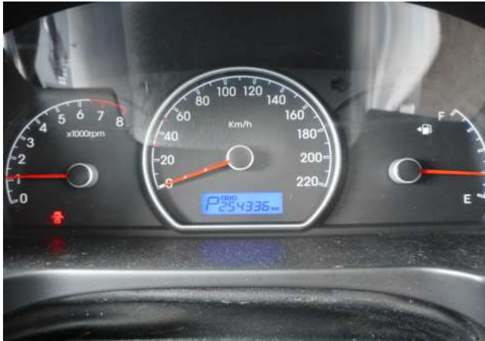
Photo 27 shows no warning lights illuminated on the instrument panel of the Motor Car after the engine was cranked. This would suggest that there was no abnormality to the electronic operating system of the Motor Car, like the ABS and EPS etc.
