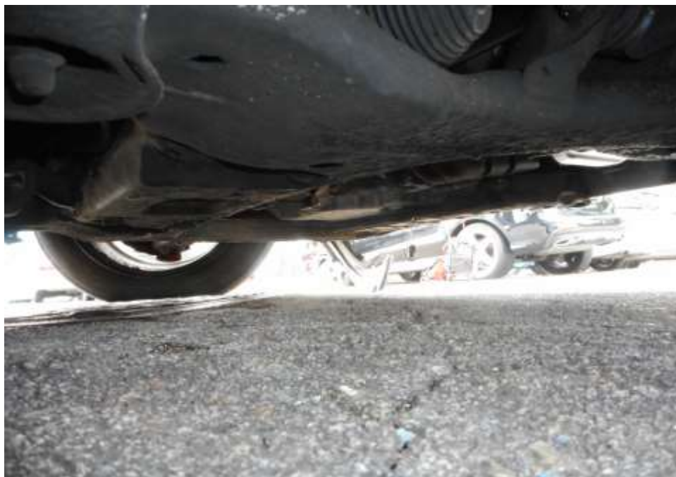
Photo 18 shows the undercarriage of the Motor Car, at the area where the engine housing and transmission housing are located. I did not find any sign(s) or indication(s) of fluid leak and/or fluid stain(s) on the underside of the Motor Car.
