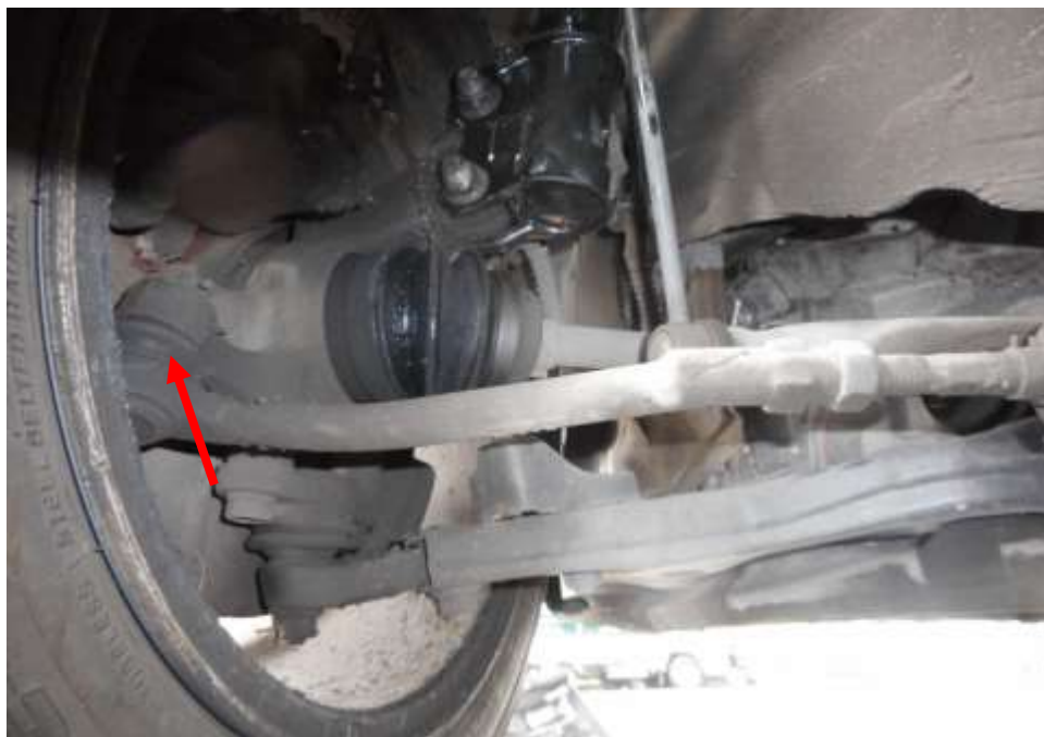
Photo 25 shows the various undercarriage components at the front left wheel of the Motor Car, which had included the steering tie rod (red arrow). The various undercarriage components of the Motor Car were all found to be intact without any visible damage.
