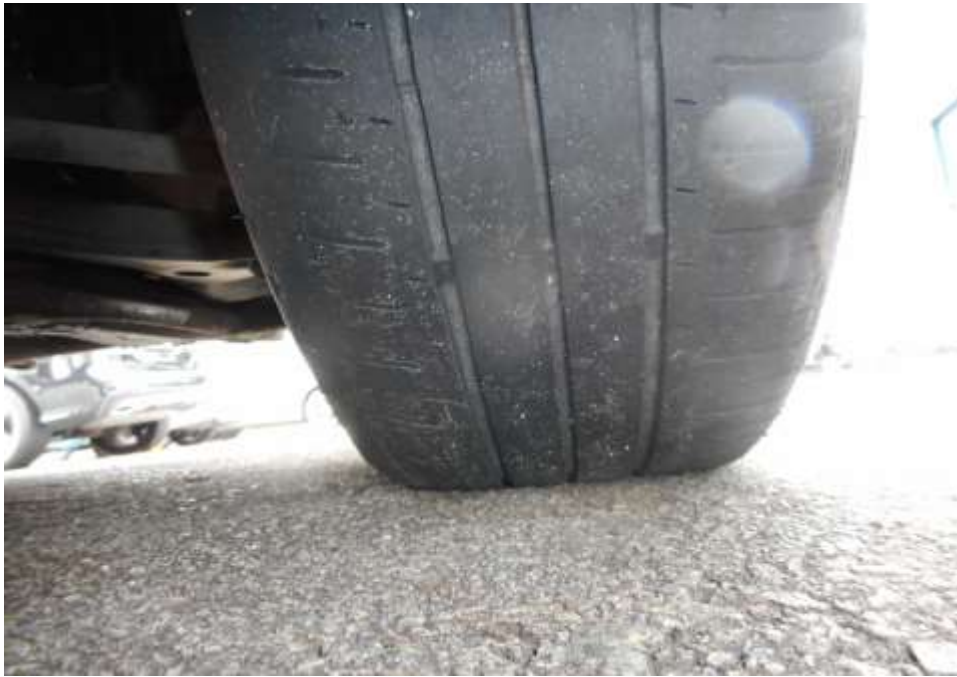
Photo 10 shows the condition of the front right tyre of the Motor Car, which was observed to be in serviceable condition with remaining tread depth of approximately 3.5mm. The tyre was sufficiently inflated for vehicular operation with no tear, cut or burst mark(s) on the outer and the inner sidewalls as well as across the tread. The 4 tyres of the Motor Car were wrapped around standard steel wheel rims without any damage.
