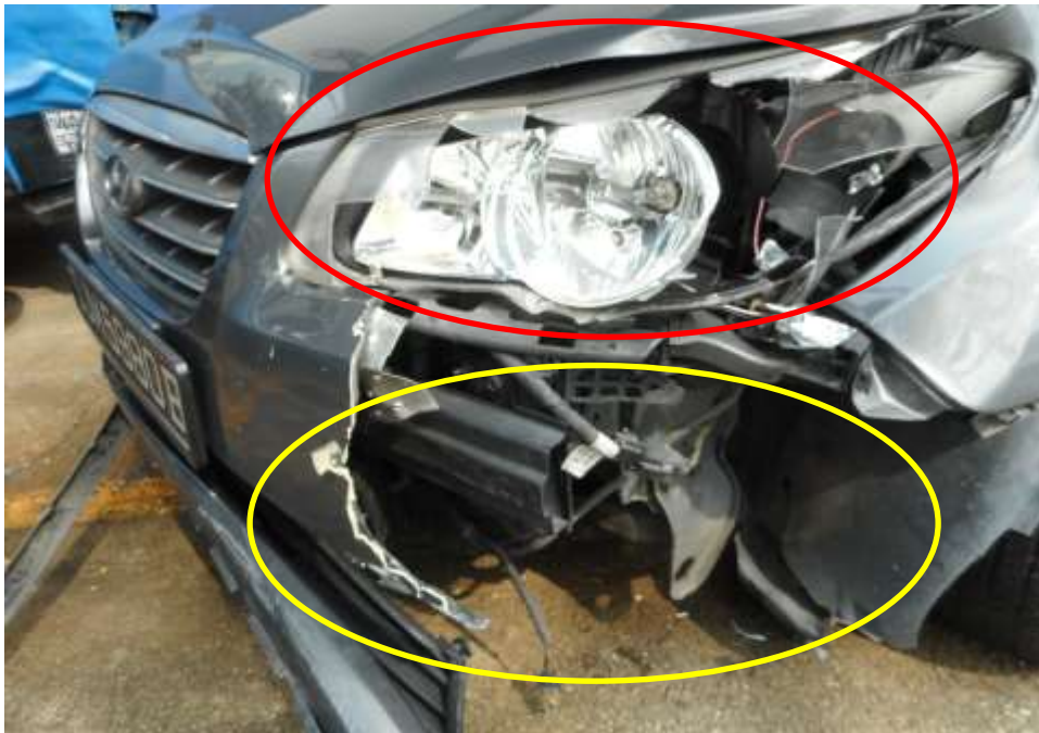
Photo 5 shows the close up view of the Motor Car's front body at the time of my inspection. The Motor Car was observed to have sustained damage at its front left headlamp (red circle) and front bumper (yellow circle) as a result of the accident.
