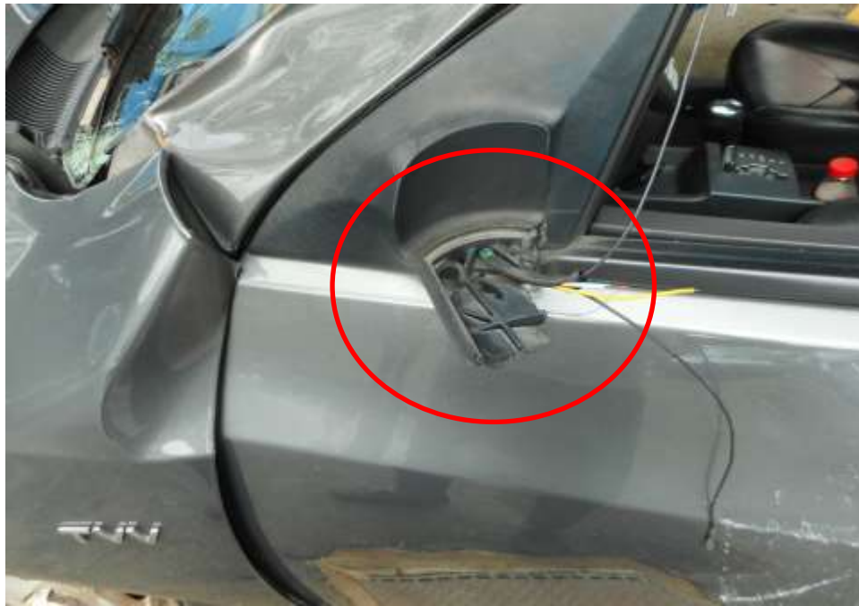
Photo 6 shows the close up view of the Motor Car's front body at the time of my inspection. The Motor Car was observed to have sustained damage at its front left rear view mirror (circled) as a result of the accident.
