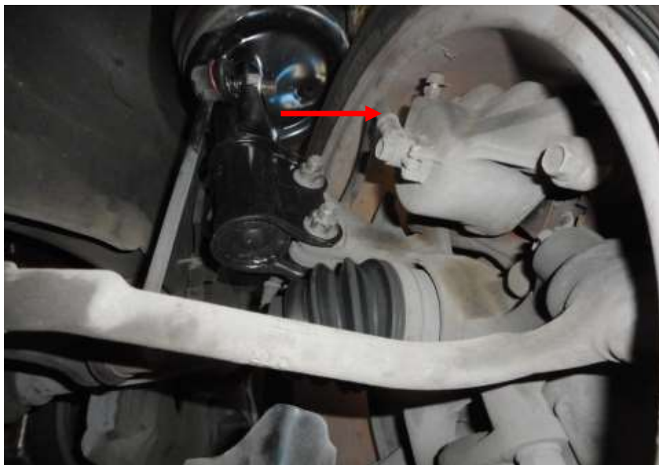
Photo 21 shows the brake hose/pipe (arrowed) at the front right wheel of the Motor Car. I did not observe any leakage of brake fluid at the time of my inspection of the Motor Car. Static tests of the Motor Car's braking system had indicated that there was no internal leakage of pressure/vacuum. The undercarriage components of the Motor Car were also all found to be intact and without any visible damage.
