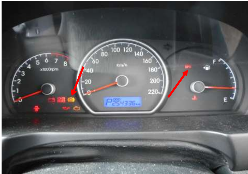
Photo 26 shows the warning light for Anti-Lock Brake System (ABS) and Power Steering System (EPS) (arrowed) appearing on the instrument panel of the Motor Car during the self-test of its various electronic operating systems when its engine was cranked.
