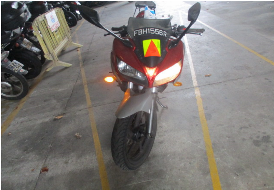
Photo 21 shows the front wheel of the Motorcycle turned towards its full right. Turning the Motorcycle's handle bar towards the right did not produce any abnormal free play and/or resistance. This would indicate that the steering system of the Motorcycle was in serviceable condition at the time of our inspection.
