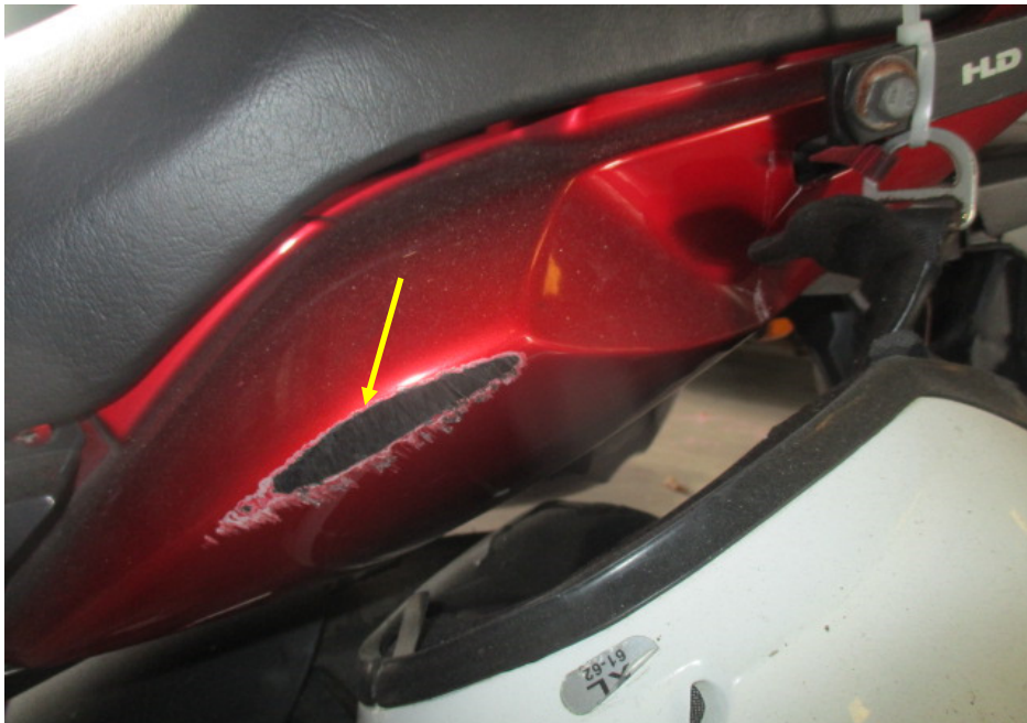
Photo 9 shows a closer view of the left rear side cover which was amongst the body parts of the Motorcycle that had sustained damages of grazing nature as a result of the accident (arrowed).
