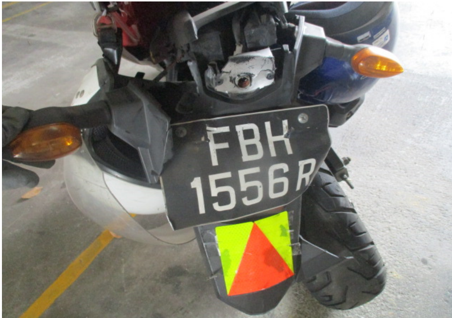
Photo 12 shows the rear mudguard, tail lamp and rear number plate of the Motorcycle that had sustained extensive damage as a result of the accident.
