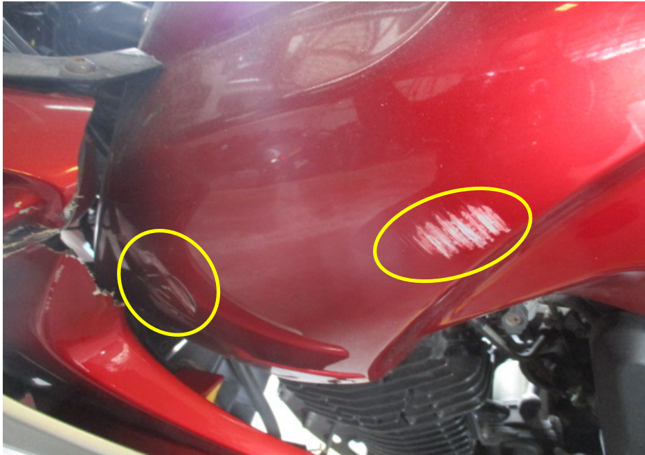
Photo 8 shows a closer view of the fuel tank (circled) which was amongst the body parts of the Motorcycle that had sustained damage as a result of the accident.
