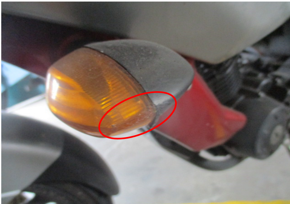
Photo 5 shows a closer view of the left front signal lamp (circled) which was amongst the body parts of the Motorcycle that had sustained damage as a result of the accident.
