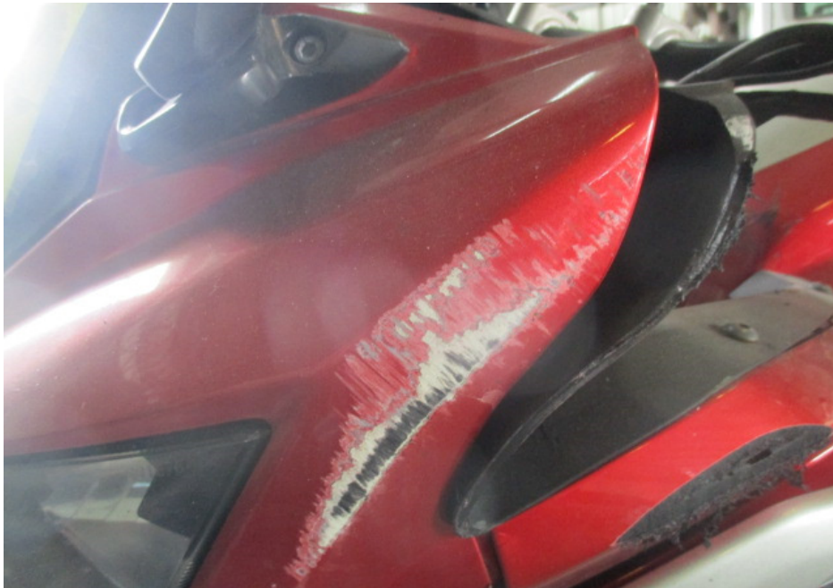
Photo 4 shows a close up view of the head cowl which was amongst the body parts at the front of the Motorcycle that had sustained damage as a result of the accident.
