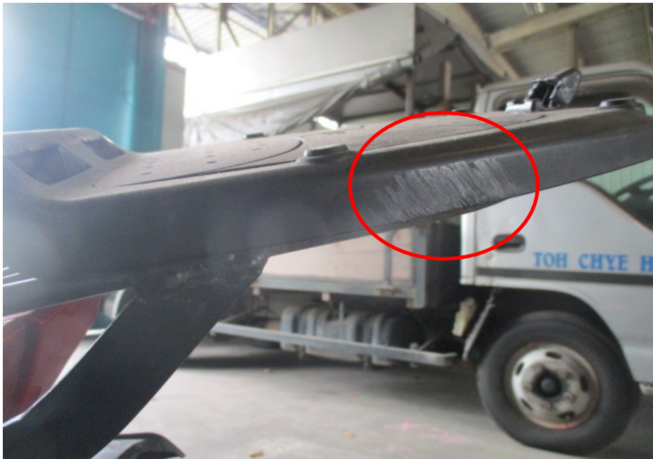
Photo 11 shows the top box rack (circled) of the Motorcycle that had sustained damage as a result of the accident.
