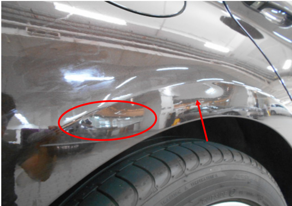
Photo 8 shows a closer view of the relatively light scratches (circled) and a minor dent (arrowed) at the right rear fender of the Third Party Vehicle, above the rear right wheel.
