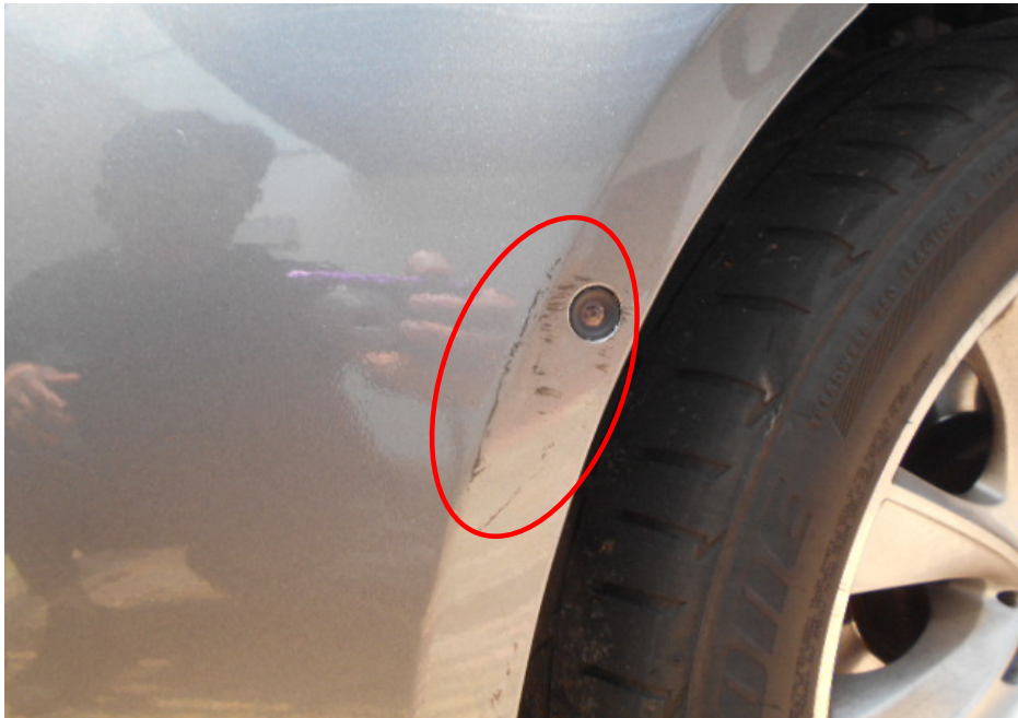
Photo 11 shows a close-up view of the relatively light scratches (circled) that I had observed on the left side of the Insured Vehicle's front bumper.
