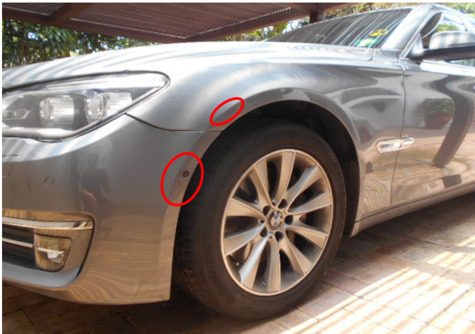
Photo 10 shows a general view of where the relatively light scratches (circled) were observed on the left front body of the Insured Vehicle. This was at the left side of the front bumper and at the left front fender, above the front left wheel.
