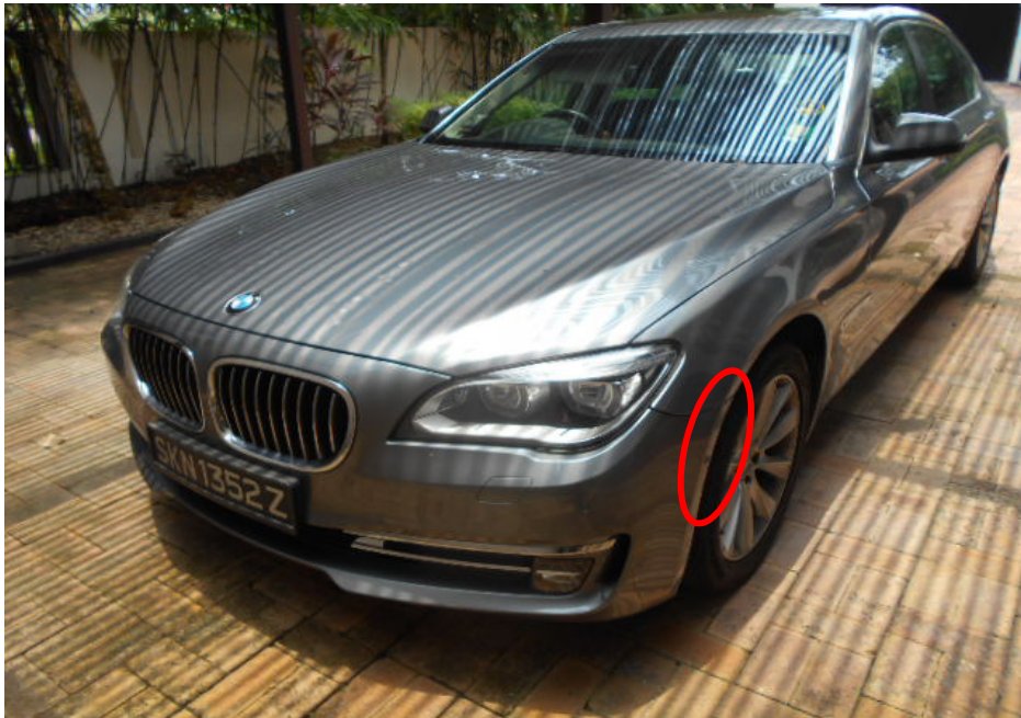
Photo 9 shows a general view of the left front body of the Insured Vehicle. At the time of my inspection, I had observed some relatively light scratches at the left side of the front bumper and at the left front fender, above the front left wheel of the Insured Vehicle. The damage observed at this body area (circled) of the Insured Vehicle had corresponded to the contact area on the Insured Vehicle (if indeed there was contact) that I had identified from my review of the video recording.
