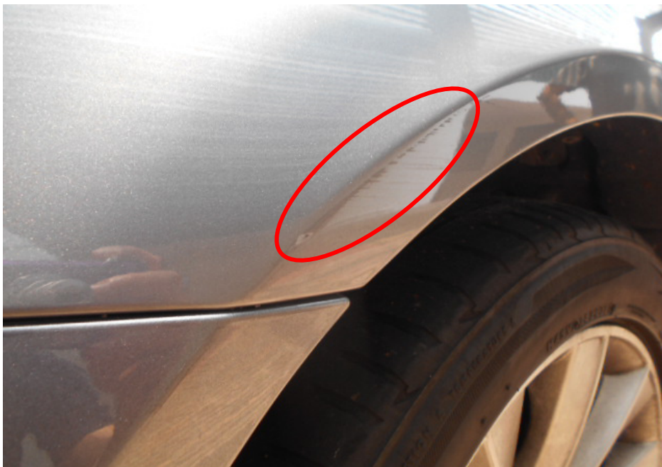
Photo 12 shows a close-up view of the relatively light scratches (circled) that I had observed on the left front fender of the Insured Vehicle's.
