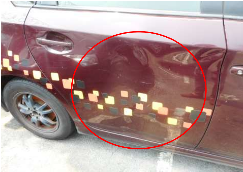
Photo 4 shows a close up view of the right body of the Motor Taxi at the time of my inspection. The Motor Taxi was observed to visually sustain damage at its right side door panel portion (circled).
