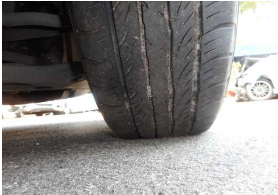
Photo 7 shows the condition of the front right tyre of the Motor Taxi, which was observed to be in serviceable condition with remaining tread depth of approximately 5.2mm. The tyre, which was wrapped around standard alloy wheel rim, was also observed to be sufficiently inflated for vehicular operation. There was no tear, cut or burst mark(s) on the outer and the inner sidewalls as well as across the tread of the 4 tyres that were fitted on the Motor Taxi.
