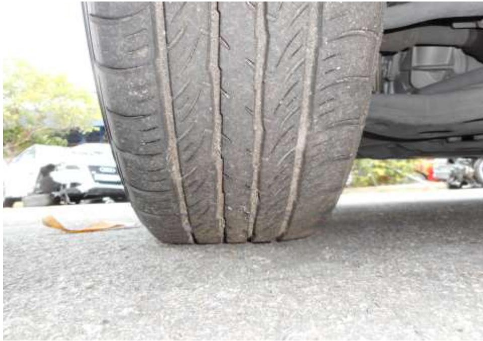
Photo 10 shows the condition of the rear right tyres of the Motor Taxi, which were observed to be in serviceable condition with remaining, tread depth of approximately 5.3mm. There was also no tear, cut or burst mark(s) on the outer and the inner sidewalls as well as across the tread of the 4 tyres that were fitted on the Motor Taxi.
