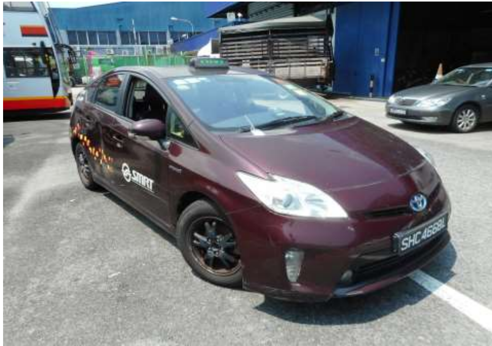
Photo 22 shows the front right wheel of the Motor Taxi turned to its full left. During my steering system test, I did not experience any abnormal free play and/or resistance when I had turned the steering wheel towards full left and full right. This would suggest that the steering system of the Motor Taxi was likely to be in serviceable condition at the material time of accident.
