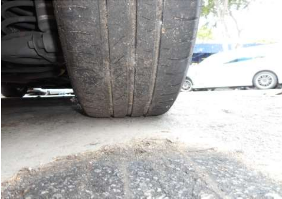
Photo 8 shows the condition of the rear right tyre of the Motor Taxi, which was observed to be in serviceable condition with remaining tread depth of approximately 4.2mm. The tyre, which was wrapped around standard alloy wheel rim, was also observed to be sufficiently inflated for vehicular operation.
