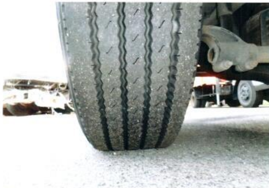
Photo 10 shows the condition of the front left tyre of the Motor Lorry, which were observed to be in serviceable condition with remaining tread depth of approximately 9.3mm. There was also no tear, cut or burst mark(s) on the outer and the inner sidewalls as well as across the tread of the 6 tyres that were fitted on the Motor Lorry.
