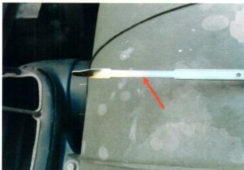
Photo 14 shows the engine oil dip stick of the Motor Lorry at the time of my inspection. The engine oil was observed to be of sufficient level (arrowed) and without any visible contamination.
