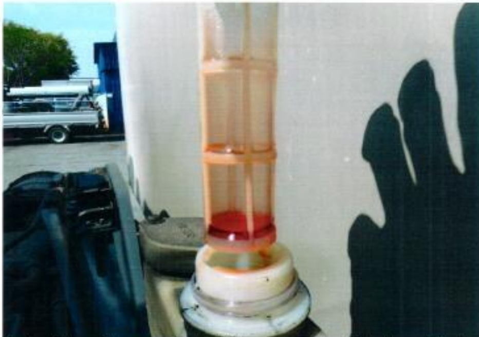
Photo 15 shows the power steering fluid reservoir of the Motor Lorry at the time of my inspection. The power steering fluid was observed to be of sufficient level and without any visible contamination.
