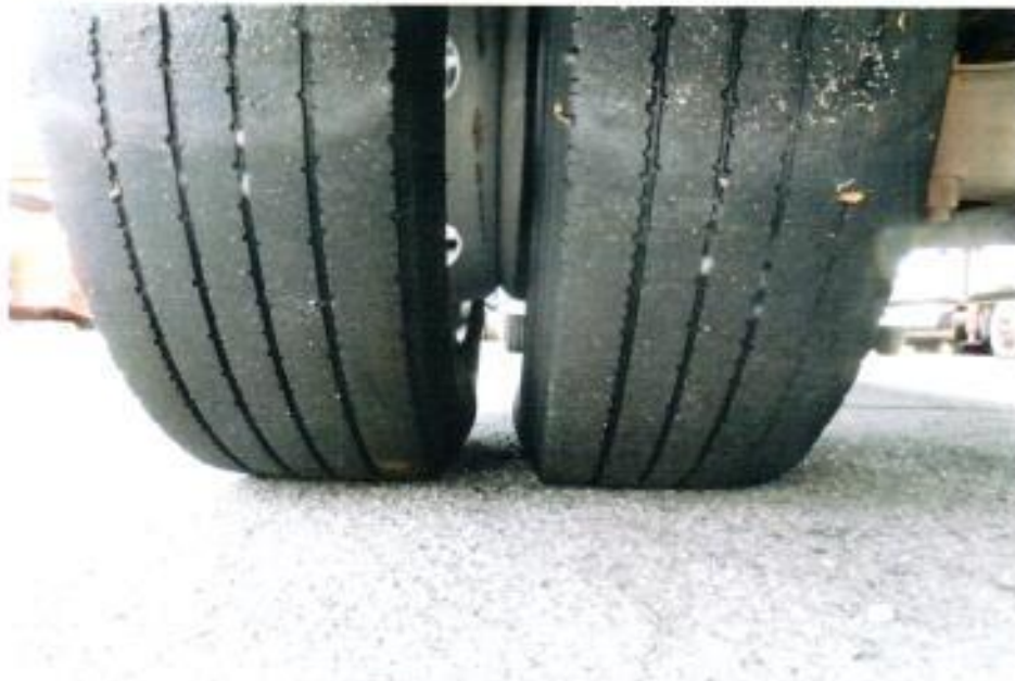
Photo 9 the condition of the rear left tyres of the Motor Lorry, which was observed to be in serviceable condition with remaining, tread depth of approximately 2.9mm. The tyres, which were wrapped around standard steel wheel rim, were also observed to be sufficiently inflated for vehicular operation. There was also no damage found on all 6 steel wheel rims of the Motor Lorry.
