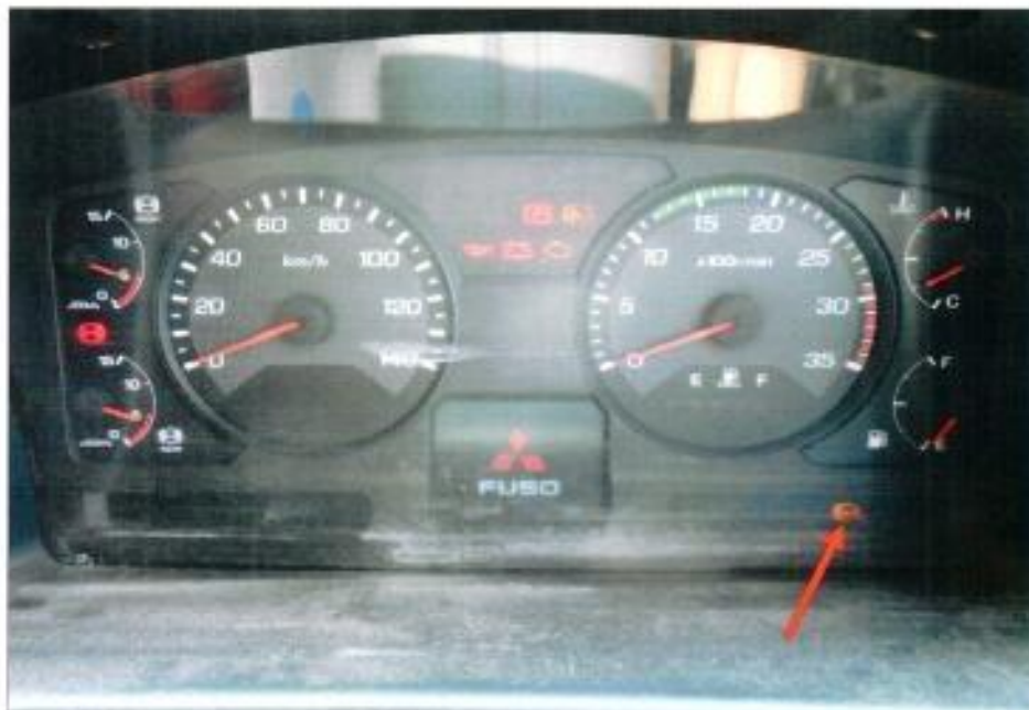
Photo 26 shows the warning light for Anti-Lock Brake System (ABS) (arrowed) appearing on the instrument panel of the Motor Lorry during the self-test of its various electronic operating systems when its engine was cranked.
