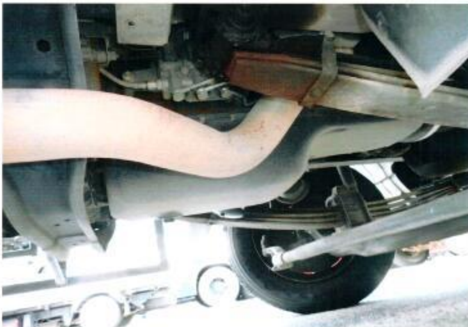
Photo 16 shows the undercarriage of the Motor Lorry, at the area where the engine housing and transmission housing are located. I did not observe any leakage or fluid stain on the underside of the Motor Lorry.
