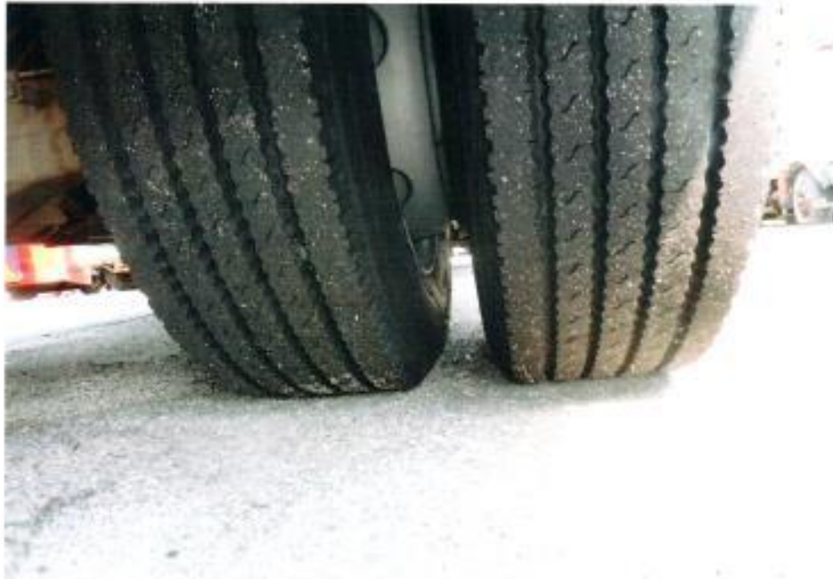
Photo 8 shows the condition of the rear right tyres of the Motor Lorry, which was observed to be in serviceable condition with remaining, tread depth of approximately 9.7mm. The tyres, which were wrapped around standard steel wheel rim, were also observed to be sufficiently inflated for vehicular operation. There was also no damage found on all 6 steel wheel rims of the Motor Lorry.
