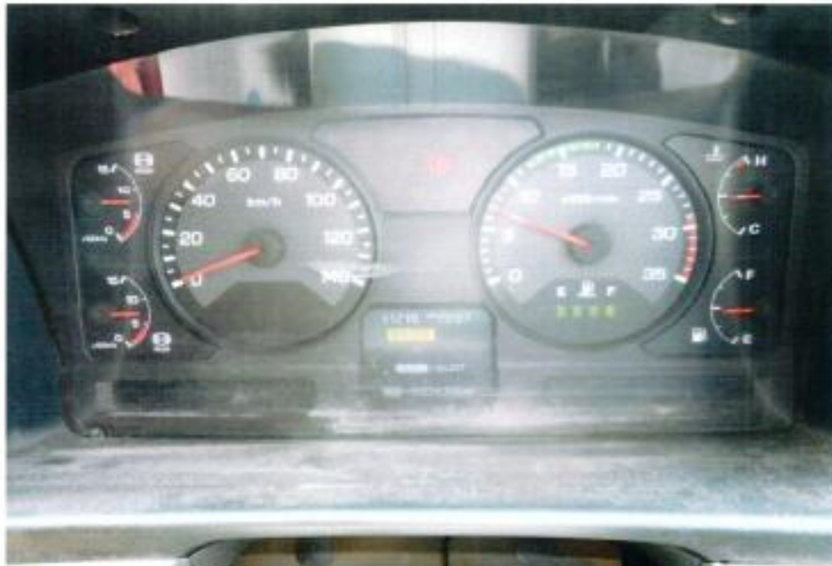
Photo 27 shows no warning lights illuminated on the instrument panel of the Motor Lorry after the engine was cranked. This would suggest that there was no abnormality to the electronic operating system of the Motor Lorry, like the ABS and etc.
