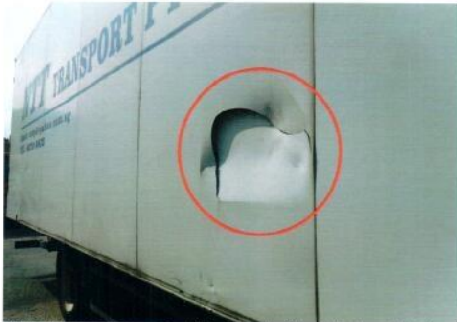
Photo 4 shows a close up view of the right body of the Motor Lorry at the time of my inspection. The Motor Lorry was observed to have sustained damage at its right portion. Its right side body panel (circled) was damaged as a result of the accident.
