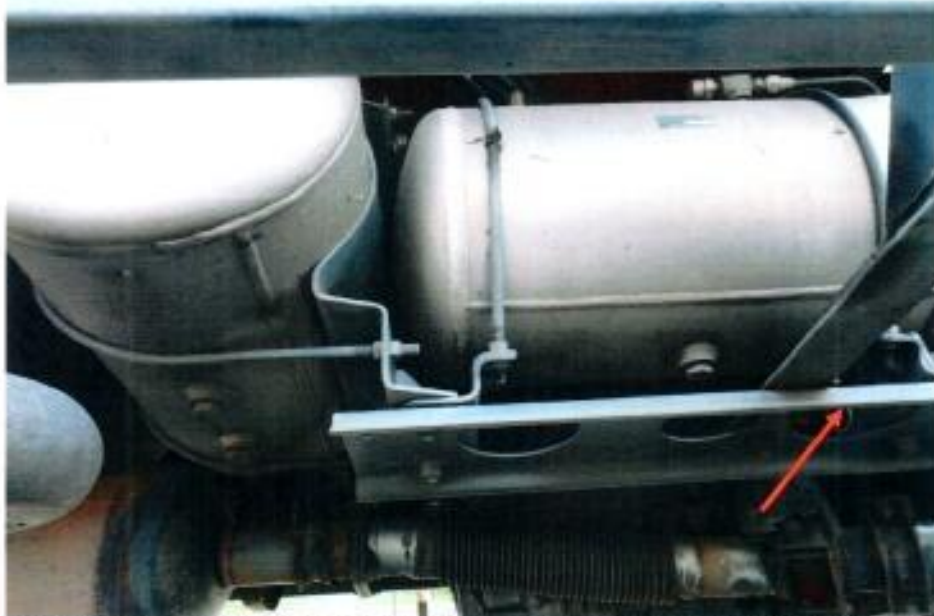
Photo 22 shows the air brake cylinders (arrowed) at the undercarriage of the Motor Lorry. I did not observe any leakage of air brake fluid at the time of my inspection of the Motor Lorry. My static tests of the Motor Lorry's braking system, along with my visual examination of the various mechanical components in the braking system had indicated that there was no internal leakage of pressure/vacuum. Hence the braking system of the Motor Lorry was likely to be in serviceable condition at the material time of accident.
