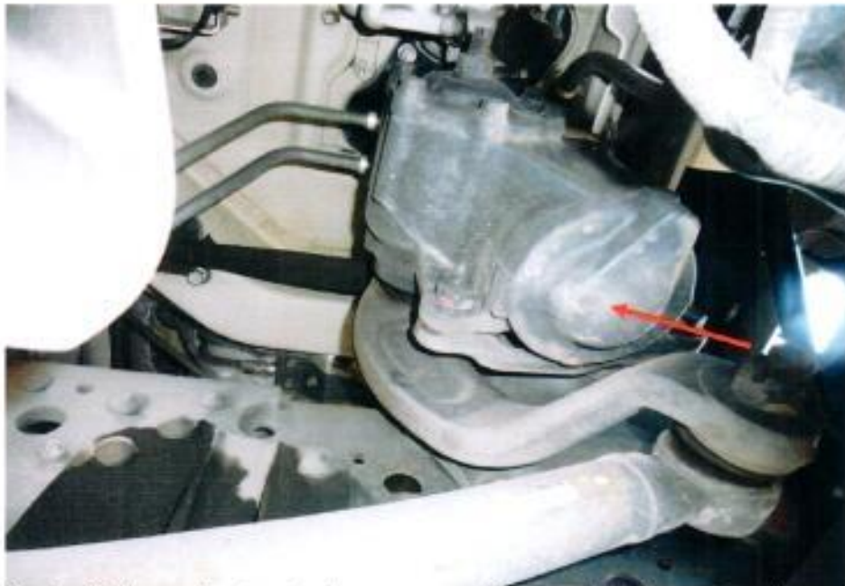
Photo 19 shows the steering box component (arrowed) at the undercarriage of the Motor Lorry was found to be intact without any visible damage. There was also no sign of fluid stain(s) observed on the various undercarriage components.
