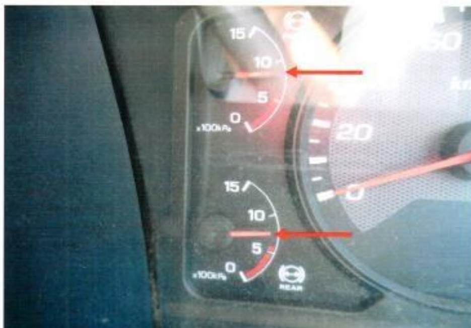
Photo 13 shows the air in the air brake cylinders of the Motor Lorry at the time of my inspection. The air in the cylinder (arrowed) was observed to be of sufficient level & serviceable at the time of the accident.
