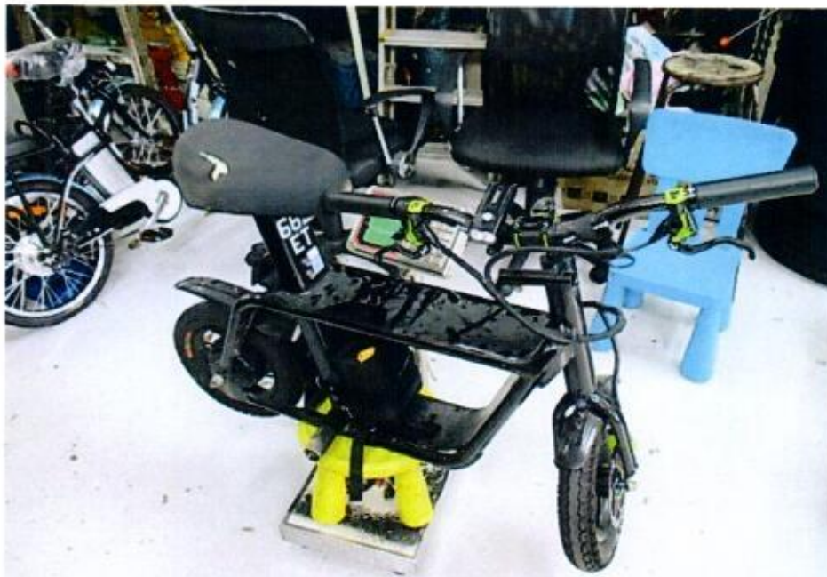
Photo 11 shows the electric scooter being weighed on a digital weighing scale. The yellow plastic chair supporting the electric scooter on the weighing scale was to prevent the tyres of the electric scooter from touching the ground during the weighing. The digital weighing scale was first calibrated to zero when the yellow plastic chair was placed on the scale.
