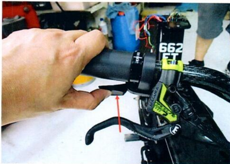
Photo 19 shows a closer view of the lever (arrowed) for the acceleration/movement function of the electric scooter being depressed. To maintain acceleration/movement, the lever will have to be continuously depressed. Once the lever is no longer depressed, electric power to the electric motor is cut off and the electric scooter will gradually come to a stop.
