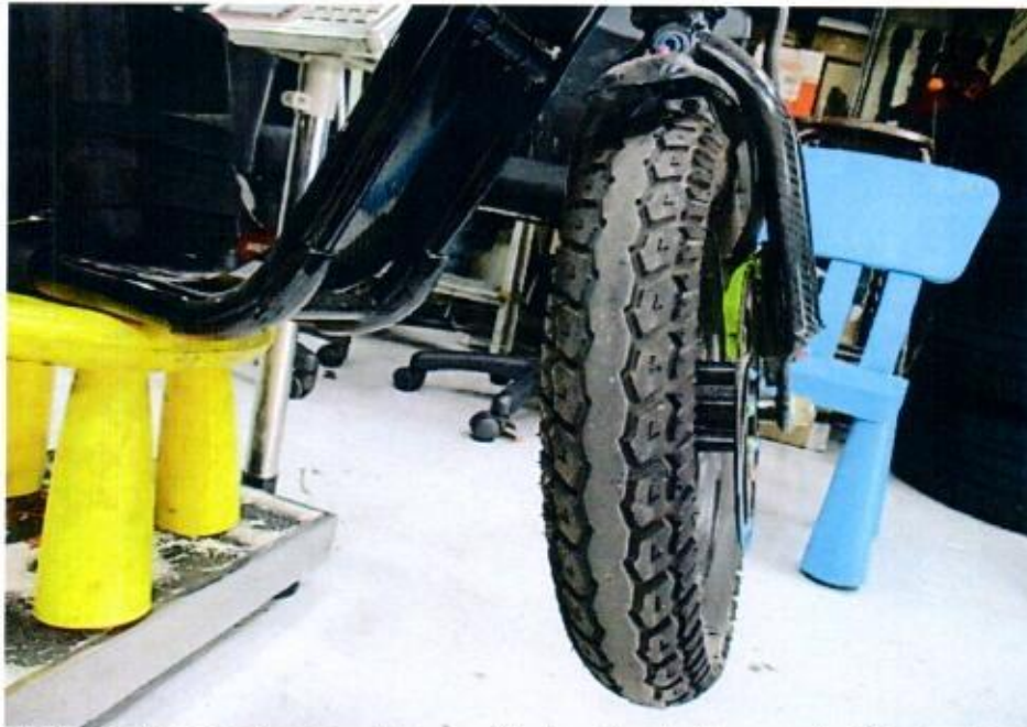
Photo 8 shows the front tyre that was fitted on the electric scooter. The front tyre was observed to be of serviceable condition with the tread pattern clearly visible. It was also sufficiently inflated for operational use.
