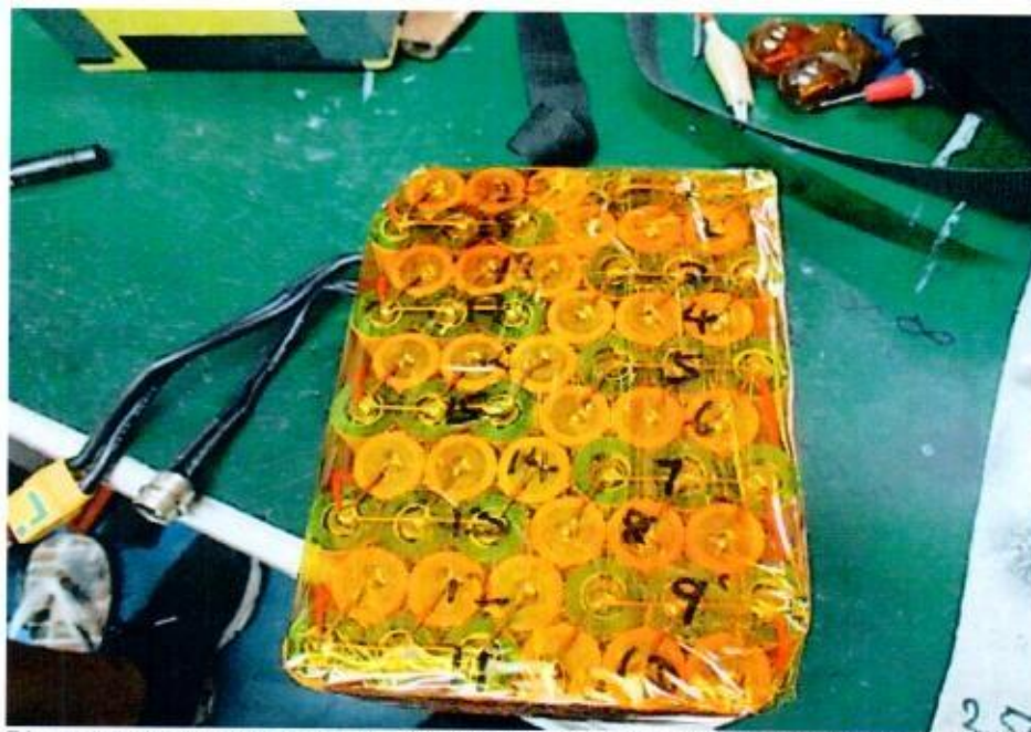
Photo 15 shows the battery pack that was fitted on the electric scooter. The battery pack was made up of 60 battery cells. This battery pack supplies the electric power to the electric motor in order for the electric scooter to accelerate/move.
