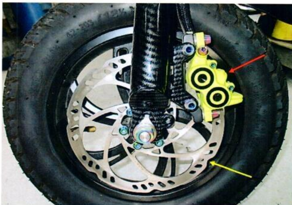
Photo 21 shows the braking components at the front wheel of the electric scooter. When the front brake lever of the electric scooter is depressed, the brake pad (red arrow) is pushed towards the brake disc (yellow arrow) via cable and spring. The brake pad clamps against the brake disc providing the frictional resistance to reduce the rotation of the front wheel, hence creating the braking effect for the electric scooter.
