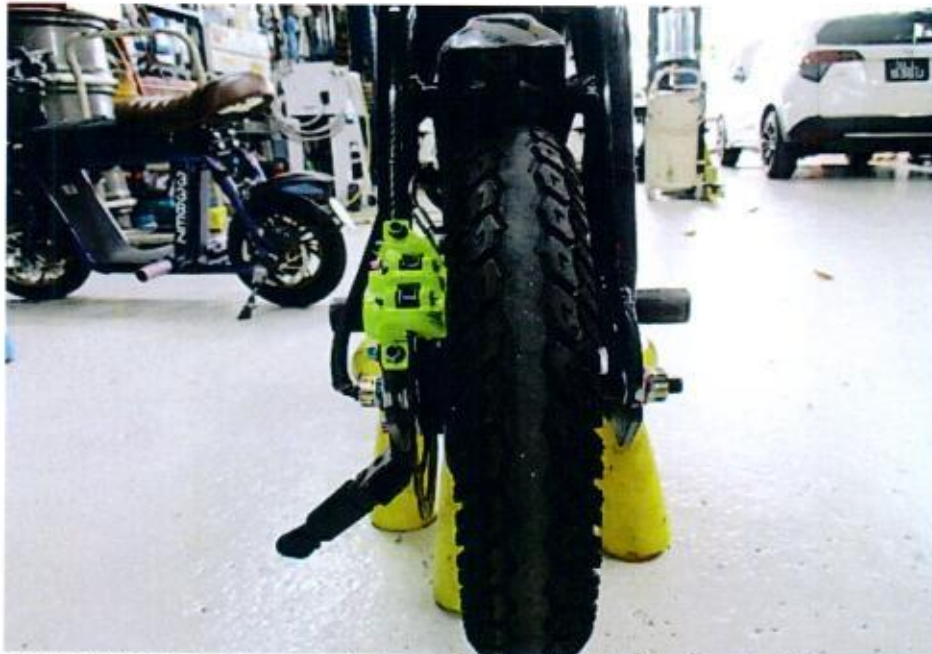
Photo 9 shows the rear tyre that was fitted on the electric scooter. The rear tyre was observed to be of serviceable condition with the tread pattern clearly visible. It was also sufficiently inflated for operational use.
