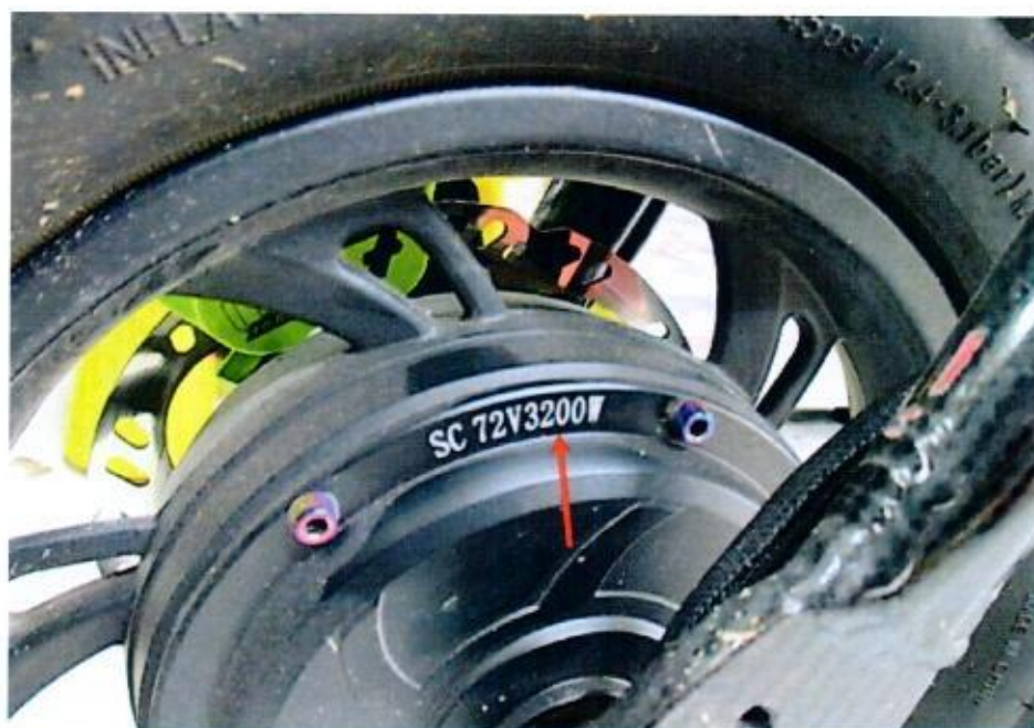
Photo 13 shows the electric motor that was fitted on the rear wheel of the electric scooter. The power rating of the electric motor was observed to be 3200 Watt (arrowed). The motor in this electric motor turns/rotates when electric power is supplied from the battery of the electric scooter.
