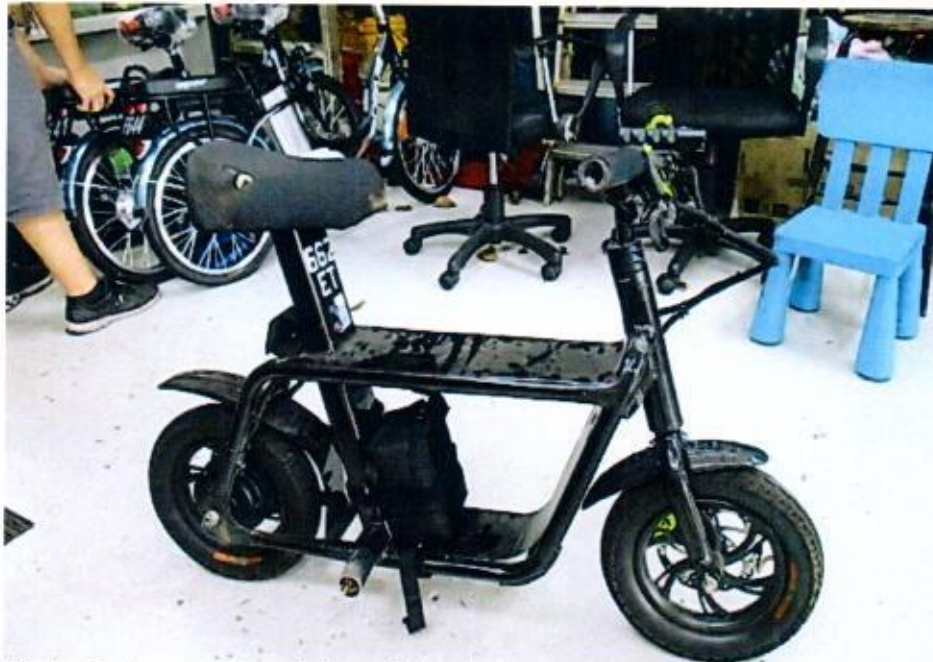
Photo 2 shows a general view of the electric scooter that I had inspected. The electric scooter was observed to have sustained relatively minor damage along its right side. The right side of the handlebar and right side leg rest were observed to be scratched/cut. The seat of the electric scooter was also torn.
