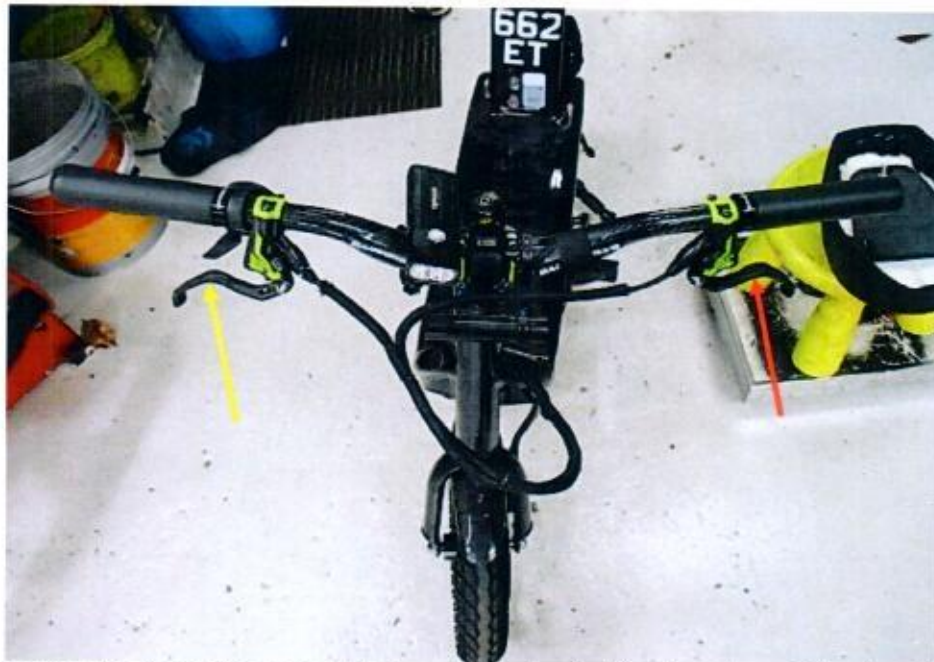
Photo 20 shows the levers that operates the braking function of the electric scooter. The lever (yellow arrow) at the right side of the handlebar operates the brake for the front wheel while the lever (red arrow) at the left side of the handlebar operates the brake for the rear wheel. The levers can be simultaneously depressed or individual depressed.
