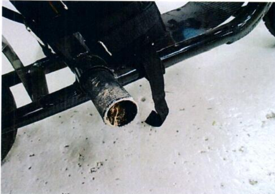
Photo 4 shows the footrest at the right side of the electric scooter, which was observed to be scratched/cut.
