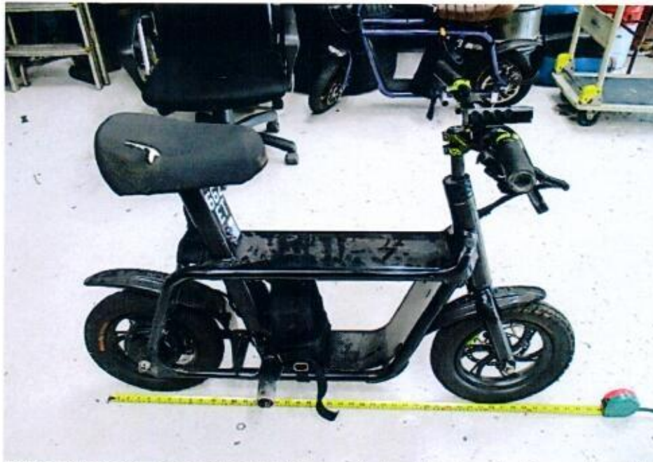
Photo 10 shows measurements being carried out to the electric scooter. The length of the electric scooter was measured to be 107cm while the width of the electric scooter was measured to be 65cm.
