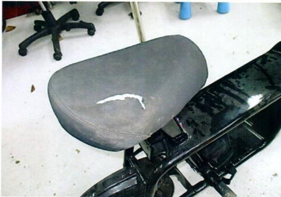
Photo 5 shows the seat cover of the electric scooter, which was observed to be torn.
