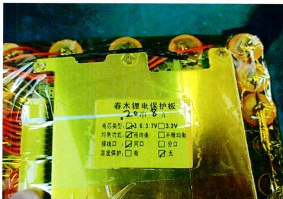
Photo 17 shows the information pasted on the battery pack of the electric scooter. The battery pack fitted on the electric scooter has 72 Volt.
