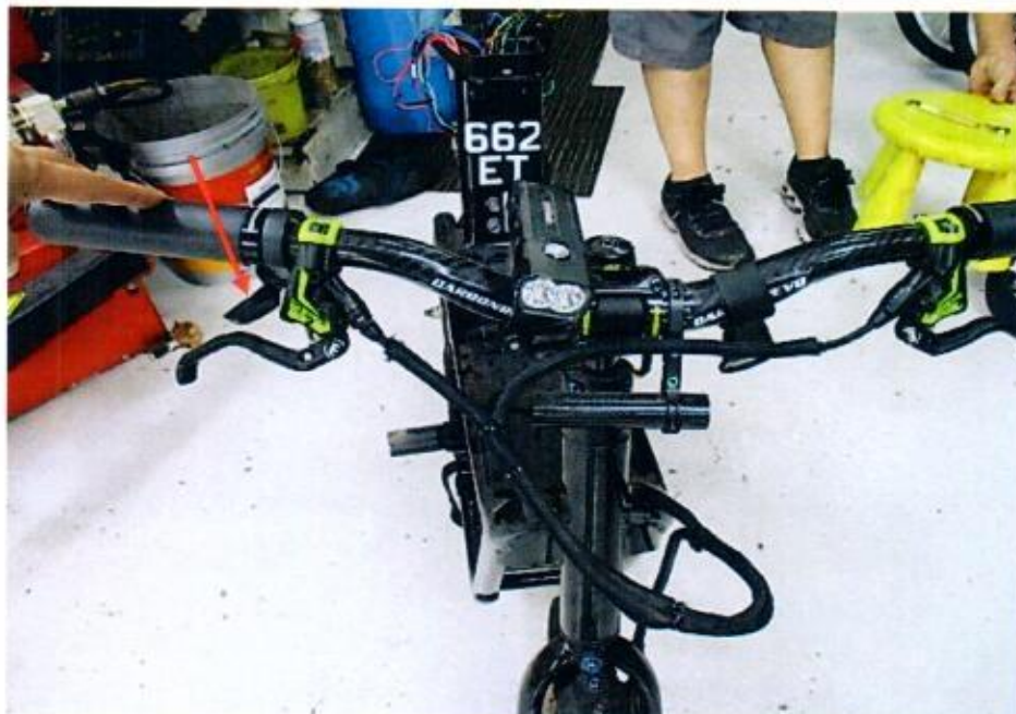
Photo 18 shows the lever (arrowed) for the acceleration/movement function of the electric scooter. When this lever is depressed, electric power from the battery pack of the electric scooter is supplied to the electric motor that is fitted at the rear wheel. The motor in the electric motor then turns/rotates resulting in the rear wheel of the electric scooter to also turn/rotate. This allows the electric scooter to accelerate/move.
