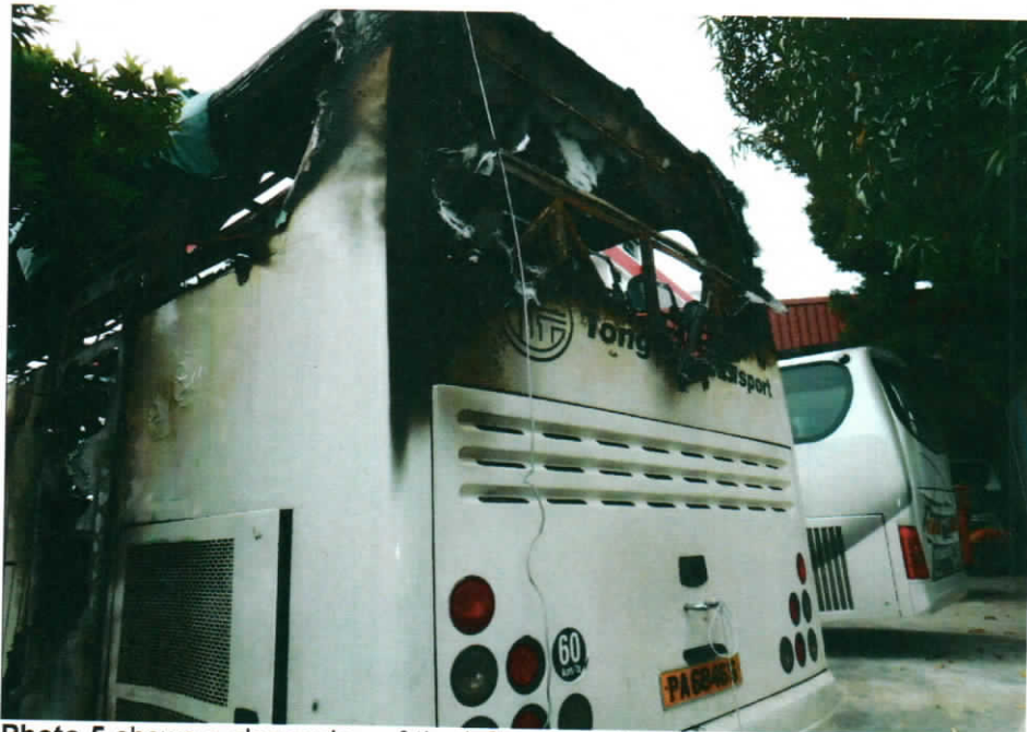
Photo 5 shows a closer view of the left rear portion of the Insured Vehicle at the time of our inspection. The fire damage was observed to be at its rear roof portion. The engine exterior compartment was observed to be unaffected by the fire.
