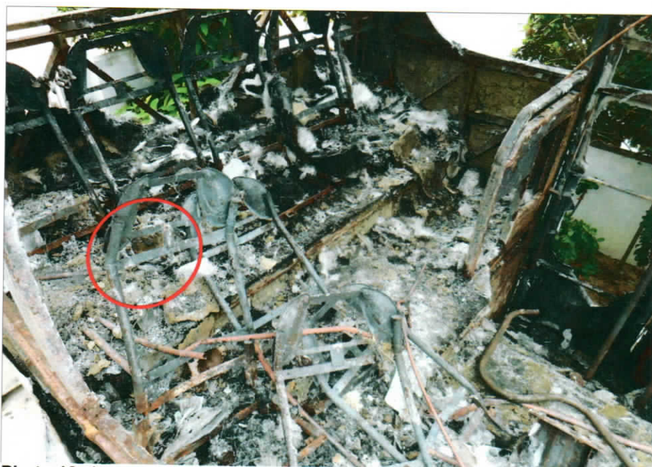
Photo 10 shows a general view of the interior portion. Observed the fan of the air extractor unit from the Insured Vehicle had fallen into the interior portion. Upon closer examination, we had found greenish residue on several burnt stretches of original extractor fan and factory fitted (circled).
