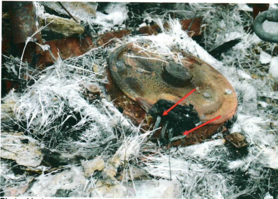
Photo 11 shows a closer view of the fallen original extractor fan from the air extractor unit, greenish residue was found on factory fitted wirings of the air extractor fan (arrowed) of the Insured Vehicle. This seems to suggest the occurrence of an electrical short circuit.
