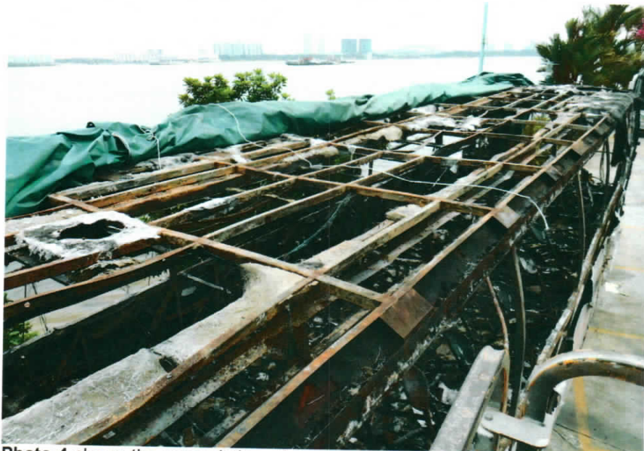
Photo 4 shows the general view of the top portion of the Insured Vehicle at the time of our inspection. The roof of the Insured Vehicle had sustained severe fire damage.
