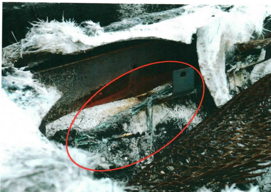
Photo 9 shows a close up view of the greenish residue found on several burnt stretches of original factory fitted wirings, around the rear roof portion of the air extractor unit (circled) of the Insured Vehicle. The presence of such greenish residue indicates internal heating of copper wires, a sign of an electrical short circuit occurring. The greenish residue is normally left behind from oxidation as a result of chemical reaction involving the copper wires.
