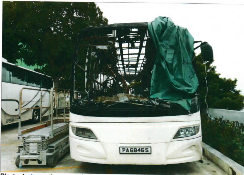
Photo 1 shows the general view of the front portion of the Insured Vehicle at the time of our inspection. The front portion of the Insured Vehicle was significantly affected by the fire.
