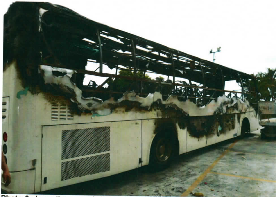
Photo 3 shows the general view of the right portion of the Insured Vehicle at the time of our inspection. The exterior body of the Insured Vehicle had sustained fire damage at the top portion as well as rear portion. Affected parts had included the side mirrors, roof, windows, rear panels, both windscreens and the rear roof air extractor unit
