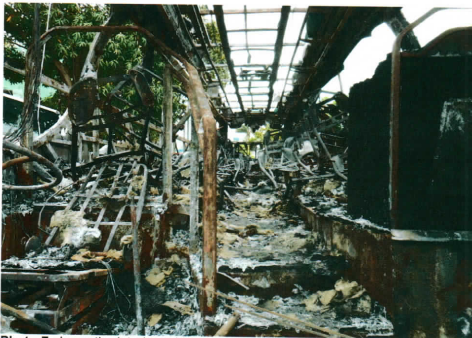
Photo 7 shows the interior cabin of the Insured Vehicle at the time of inspection. The interior rear cabin was completely burnt.
