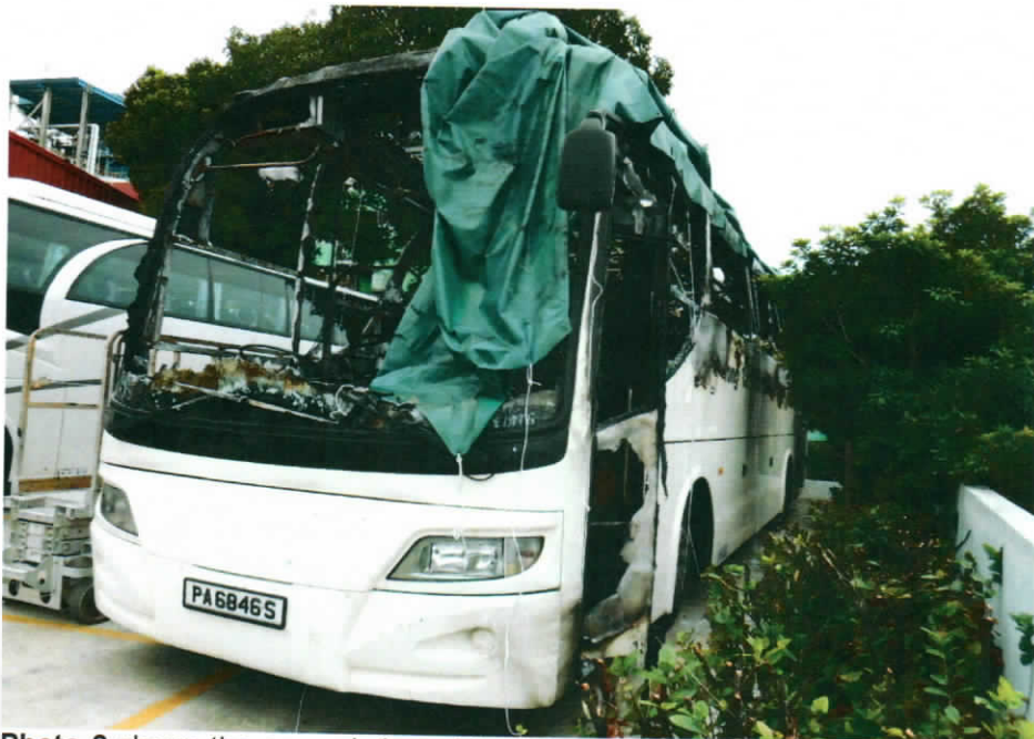
Photo 2 shows the general view of the left portion of the Insured Vehicle at the time of our inspection. The exterior body of the Insured Vehicle had sustained fire damage at the top portion as well as rear portion. Affected parts had included the side mirrors, roof, windows, rear panels, both windscreens and the rear roof air extractor unit.
