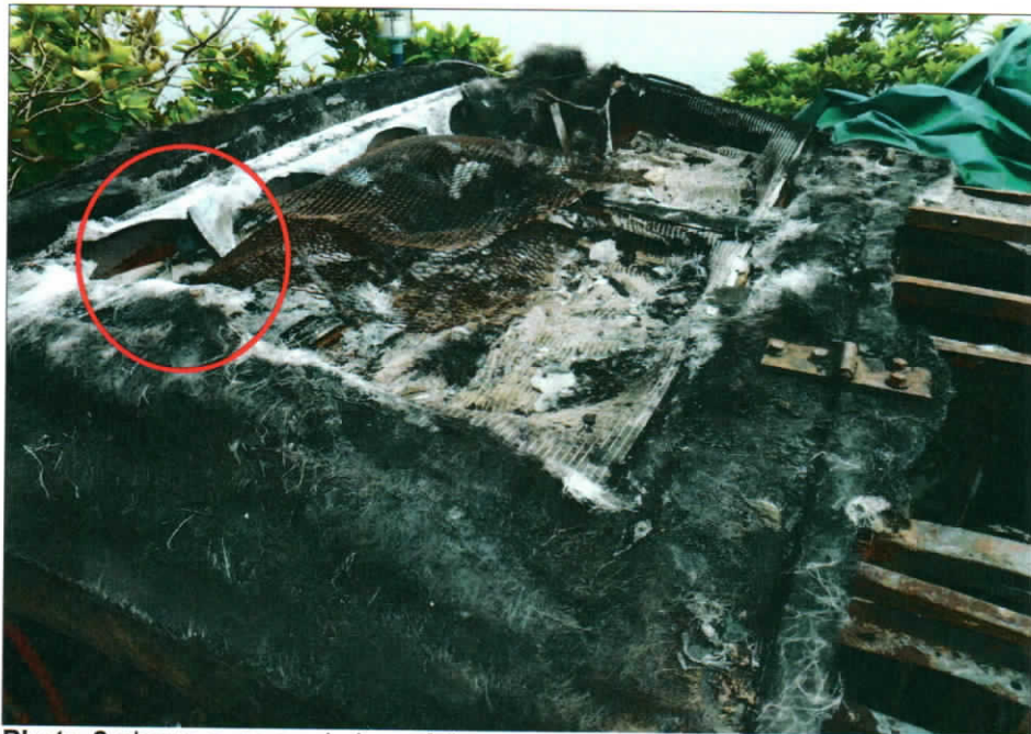
Photo 8 shows a general view of the rear roof portion of the air extractor unit of the Insured Vehicle. Upon closer examination, we had found greenish residue on several burnt stretches of original extractor fan and factory fitted wirings around the rear roof portion of where the air extractor unit is located with (circled).
